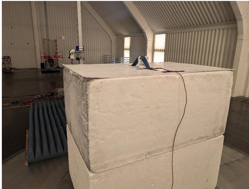
Photograph 4: Back View Radiated Emissions Worst-Case Configuration – Frequencies Over 1000 MHz
