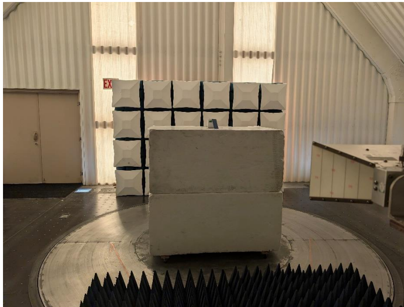
Photograph 3: Front View Radiated Emissions Worst-Case Configuration – Frequencies Over 1000 MHz
