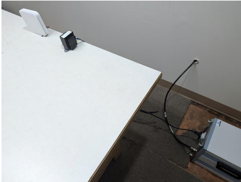
Photograph 5: Front View Conducted Emissions Worst-Case Configuration
