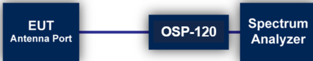
Figure 2: Direct Connection at the Antenna Port Test
