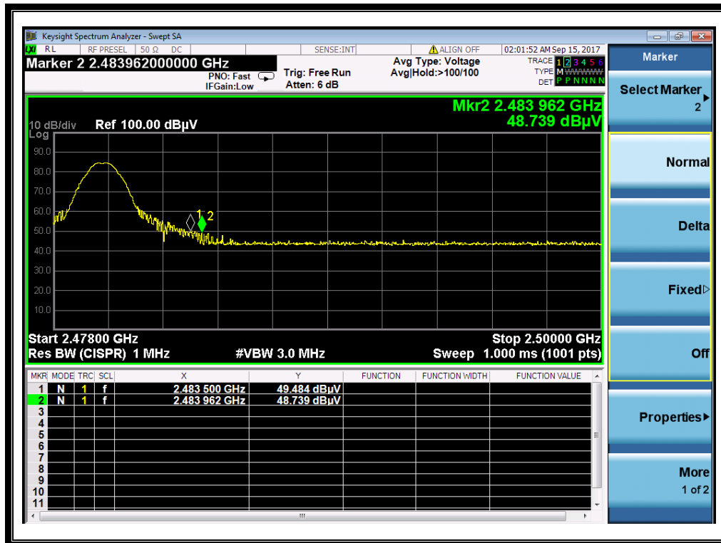
(Plot F1:Channel = 78 PEAK @ 8-DPSK Mode)
