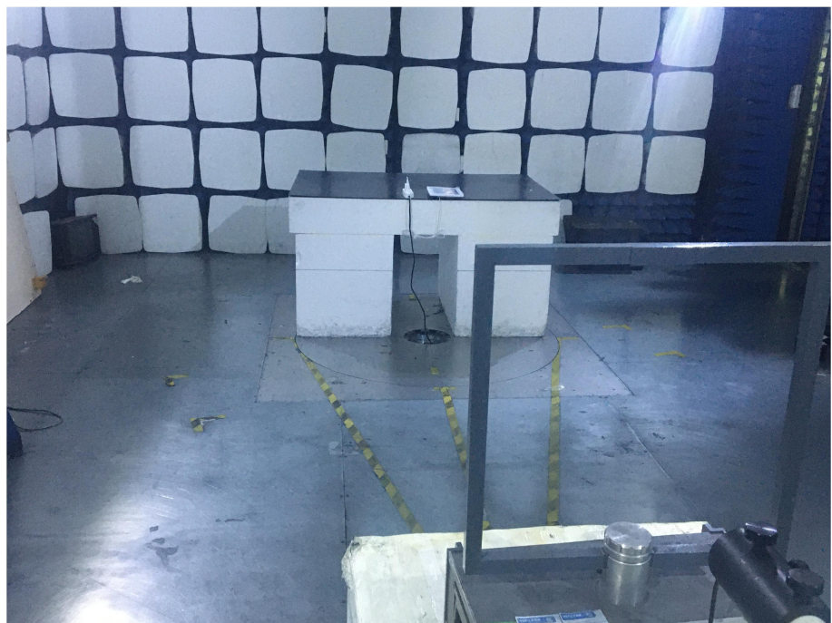
Radiation Emission Test Setup (Below 30MHz)
