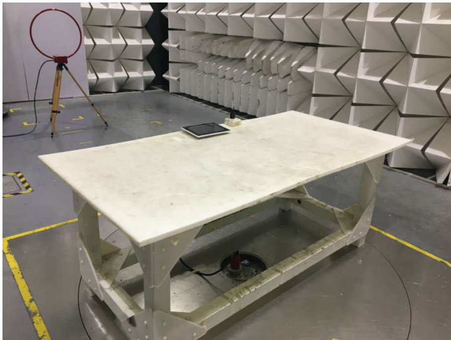
Radiated spurious emission Test Setup-1(Below 30MHz)
