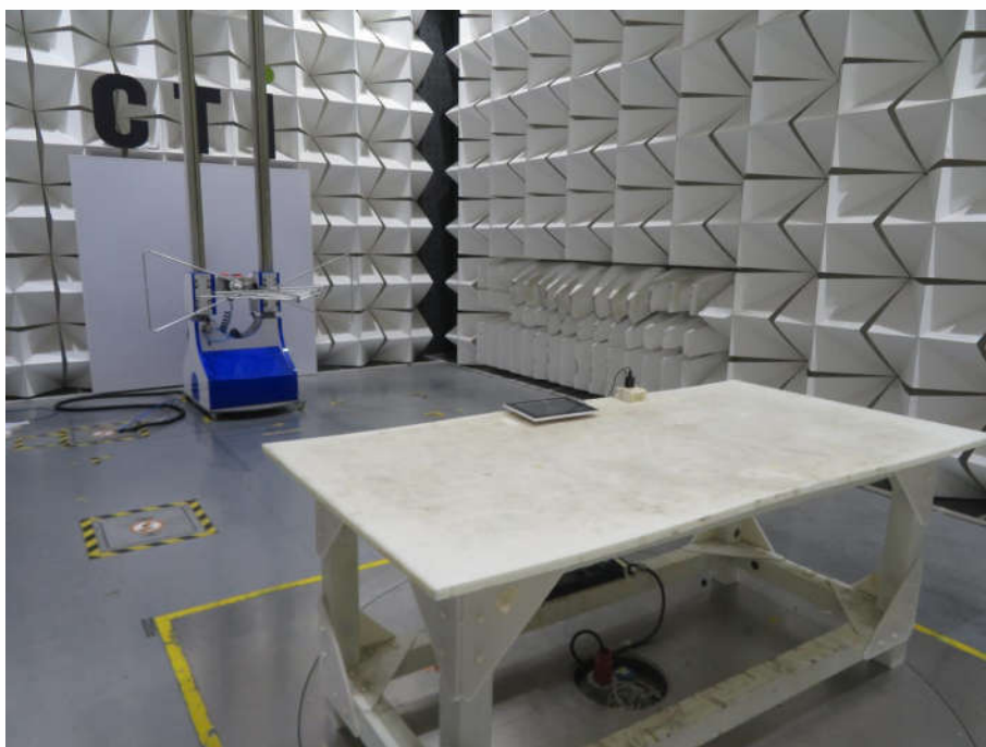
Radiated spurious emission Test Setup-2(Below 1GHz)
