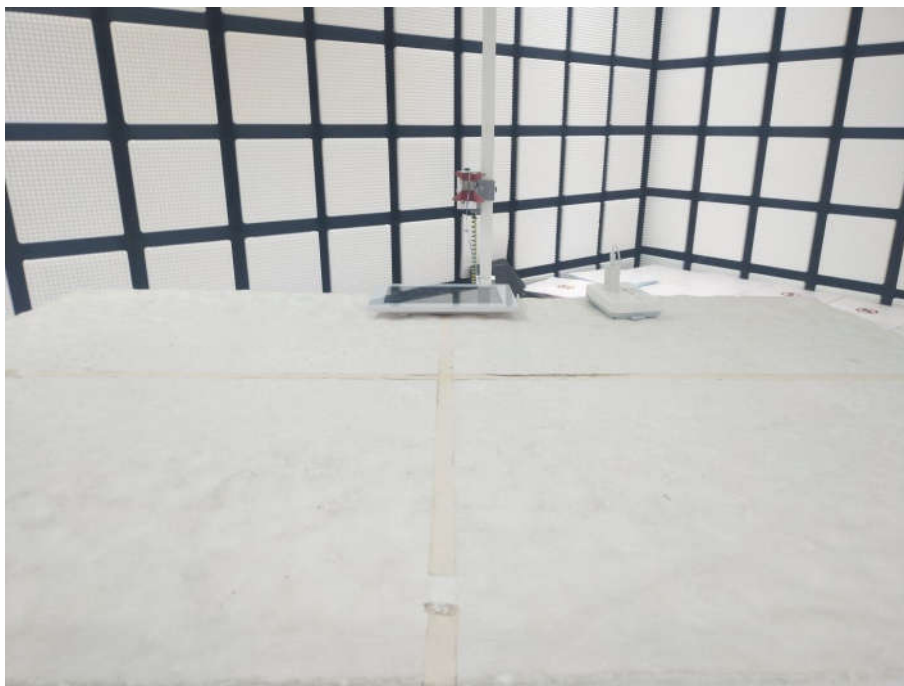
Radiated spurious emission Test Setup-2(Above 1GHz)
