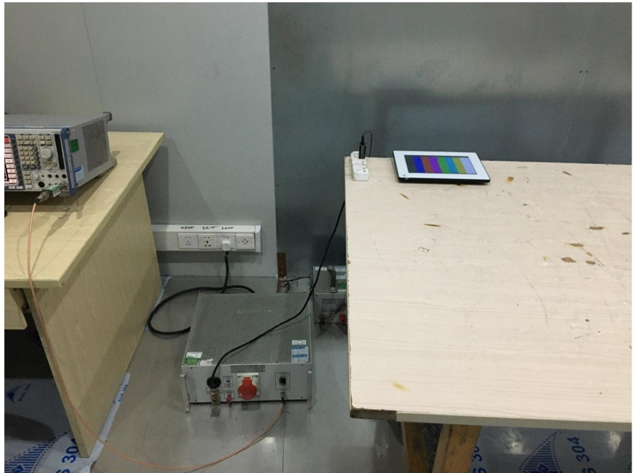
Conducted Emission Test Setup
