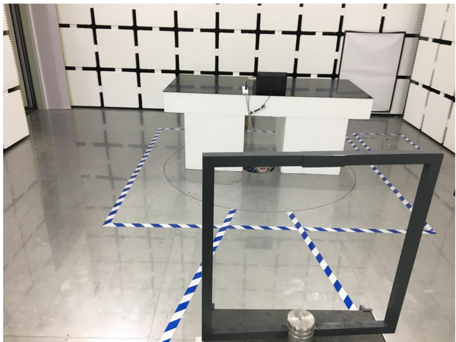
Radiation Emission Test Setup (Below 30MHz)
