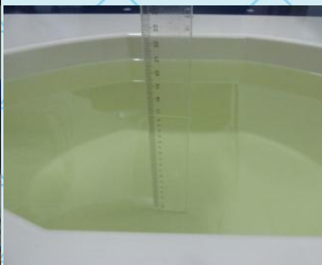
Photo 8: 2450MHz Liquid Depth \geq 15.0\text{cm}
