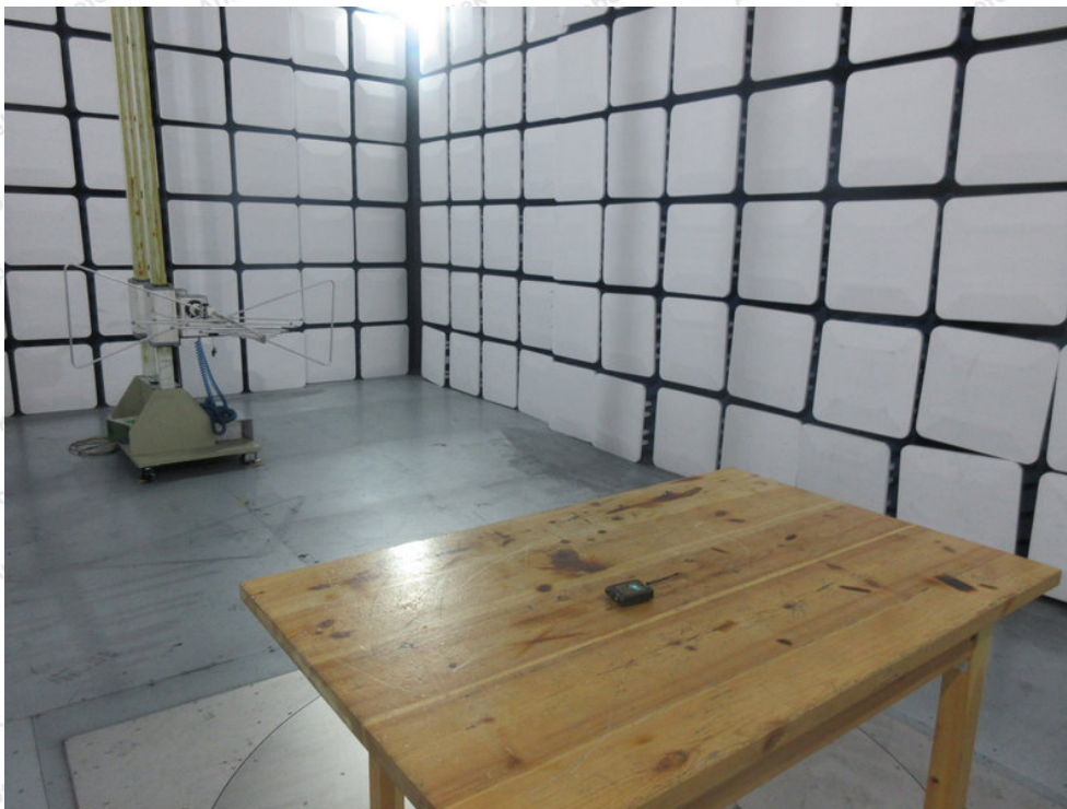
Photo of Radiation Emission Test
