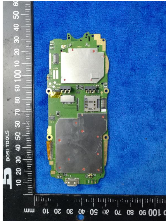
Mainboard with Shielding – Front View
