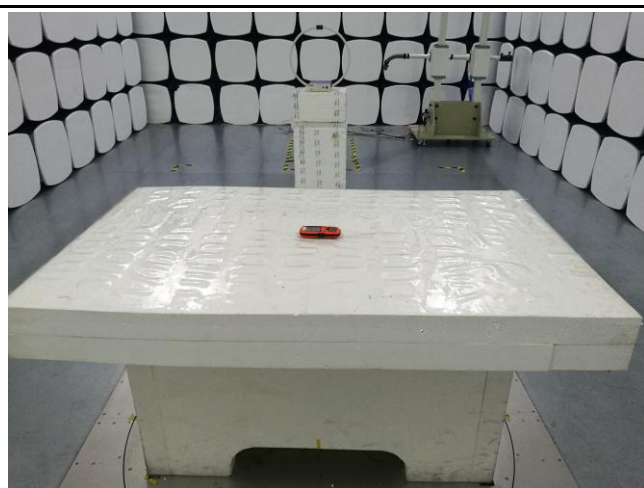
Radiated Emissions Test Setup 1MHz-30MHz
