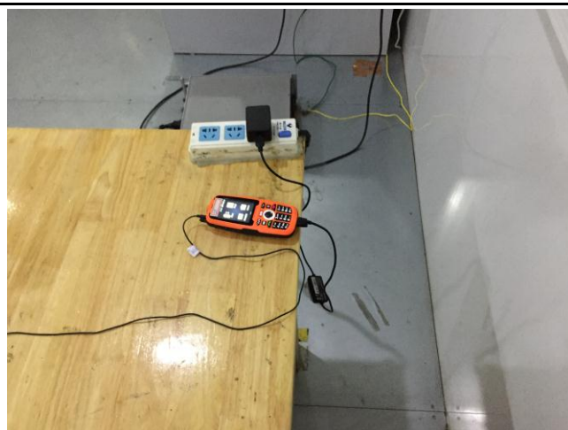
Conducted Emissions Test Setup – Side View
