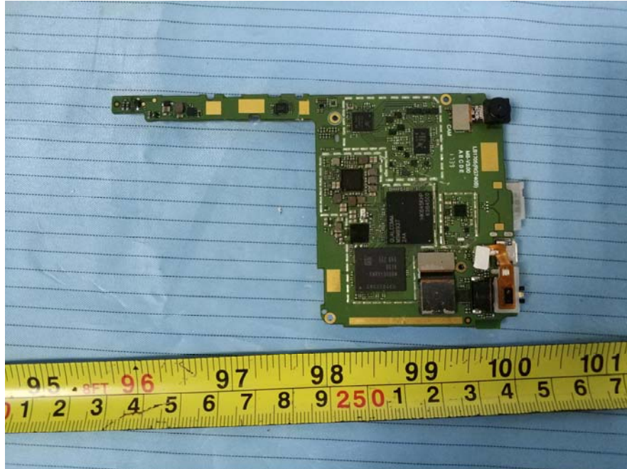
EUT –Main Board 1 Bottom Shielding off View
