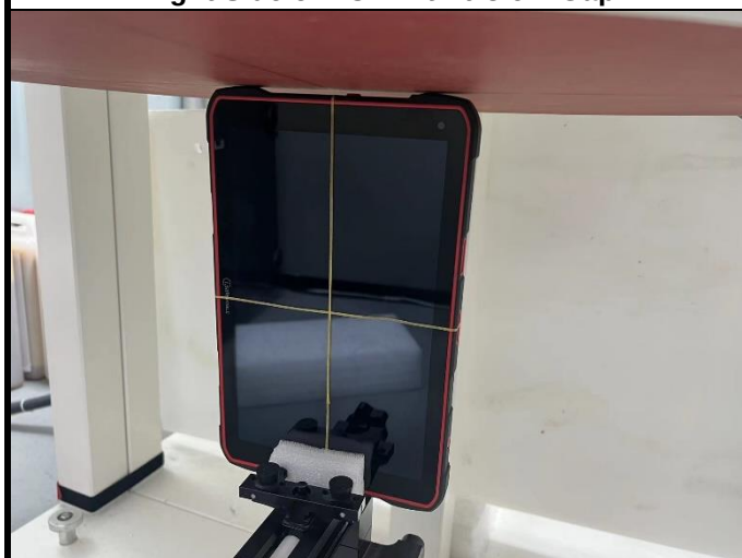
Top Side of EUT with 0 cm Gap
