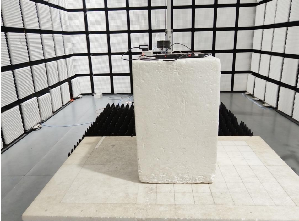
Radiated spurious emission Test Setup-2(Above 1GHz)
