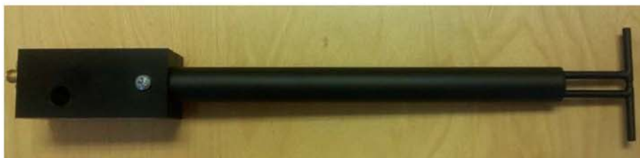
Figure 1 – MVG COMOSAR Validation Dipole
