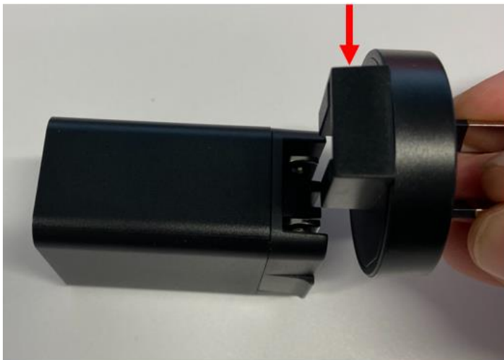
Align slots in adaptor to prongs and push down until adaptor is fully seated into back of AC Power Supply.
