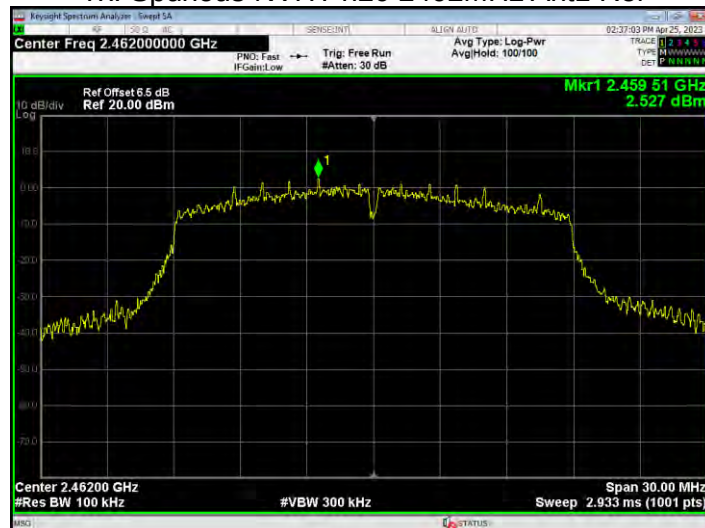
Tx. Spurious NVHT n20 2462MHz Ant1 Emission
