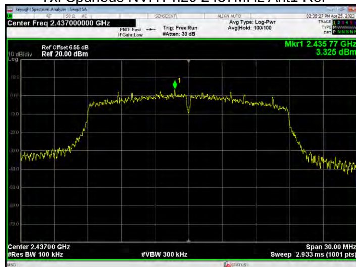
Tx. Spurious NVHT n20 2437MHz Ant1 Emission
