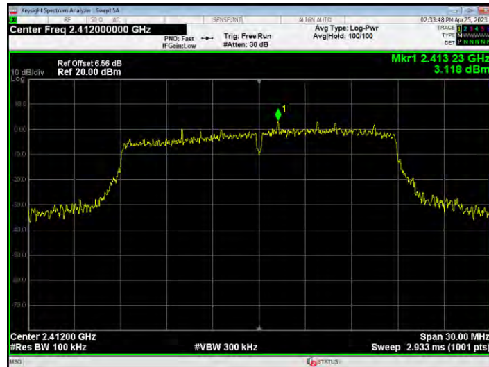
Tx. Spurious NVHT n20 2412MHz Ant1 Emission
