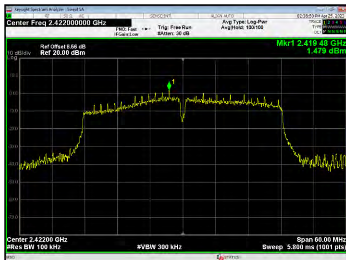
Tx. Spurious NVHT n40 2422MHz Ant1 Emission
