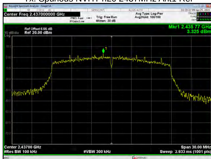
Tx. Spurious NVHT n20 2437MHz Ant1 Emission
