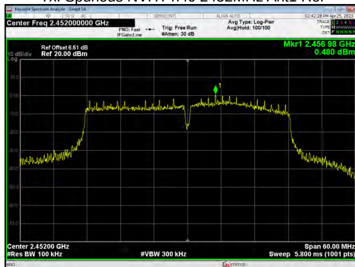
Tx. Spurious NVHT n40 2452MHz Ant1 Emission
