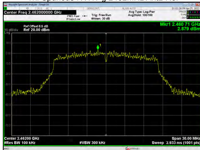
Tx. Spurious NVHT g 2462MHz Ant1 Emission
