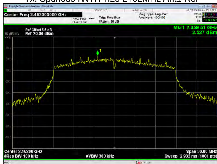
Tx. Spurious NVHT n20 2462MHz Ant1 Emission
