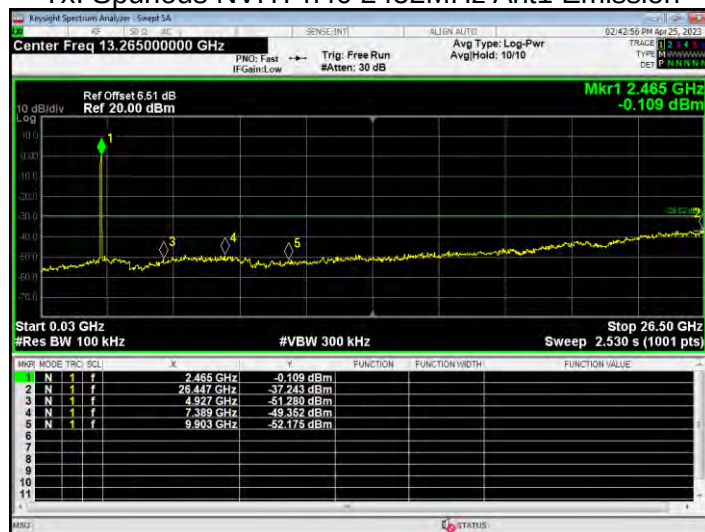
Tx. Spurious NVHT n40 2452MHz Ant1 Emission
