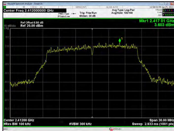
Tx. Spurious NVHT g 2412MHz Ant1 Emission
