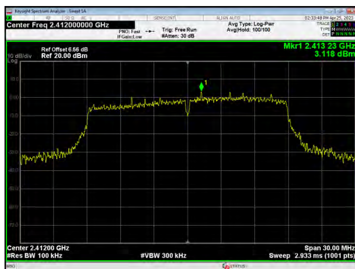
Tx. Spurious NVHT n20 2412MHz Ant1 Emission
