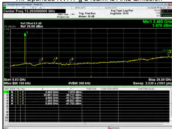
Tx. Spurious NVHT n20 2412MHz Ant1 Ref
