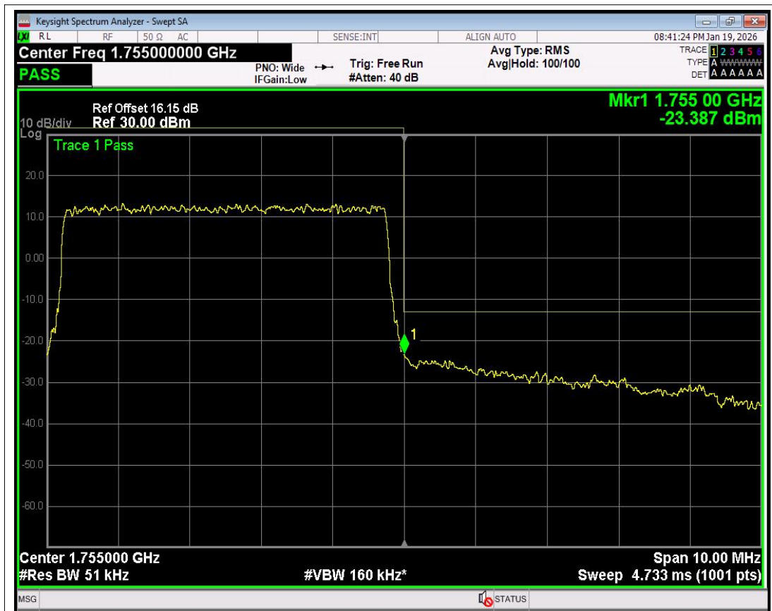
Band4 QPSK BW=5MHz Channel=20375 RB Size=25 Position=#0 NVNT
