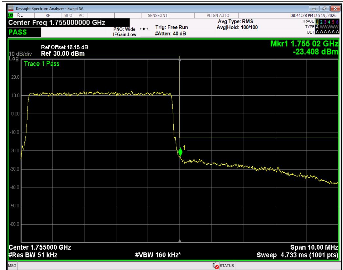
Band4 16QAM BW=5MHz Channel=20375 RB Size=25 Position=#0 NVNT
