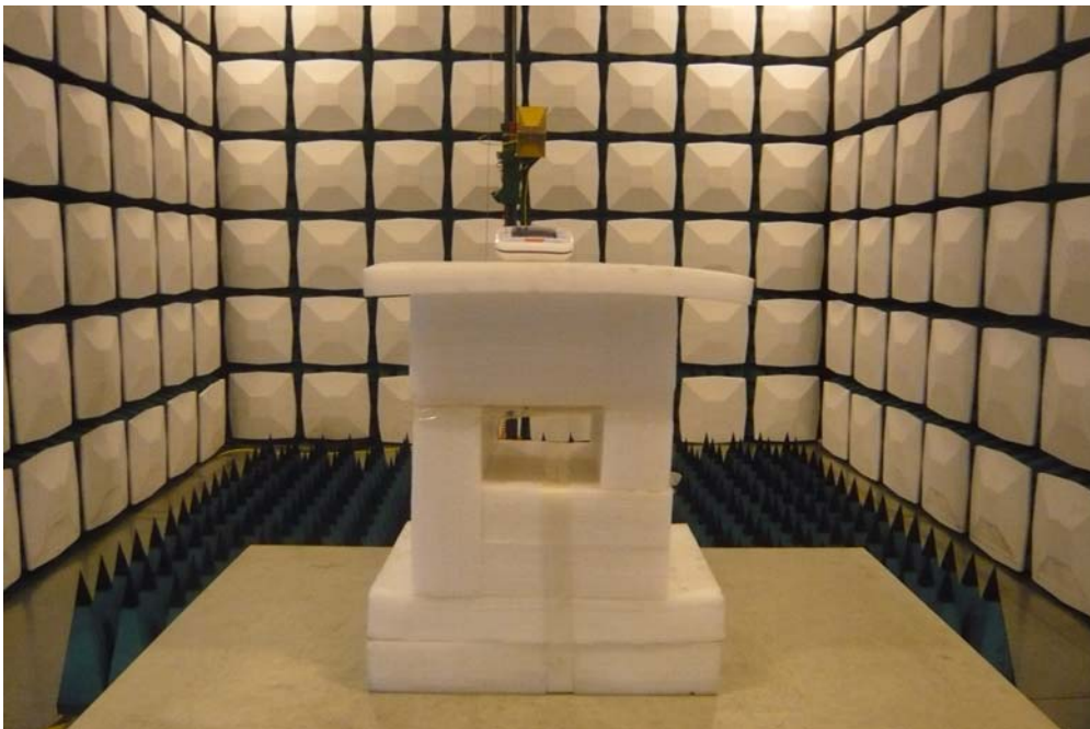
Radiated Emission View (Above 1GHz)
