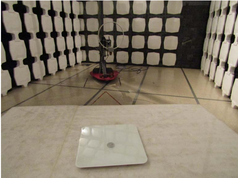
Measurement of Radiated Emission Test Set Up
