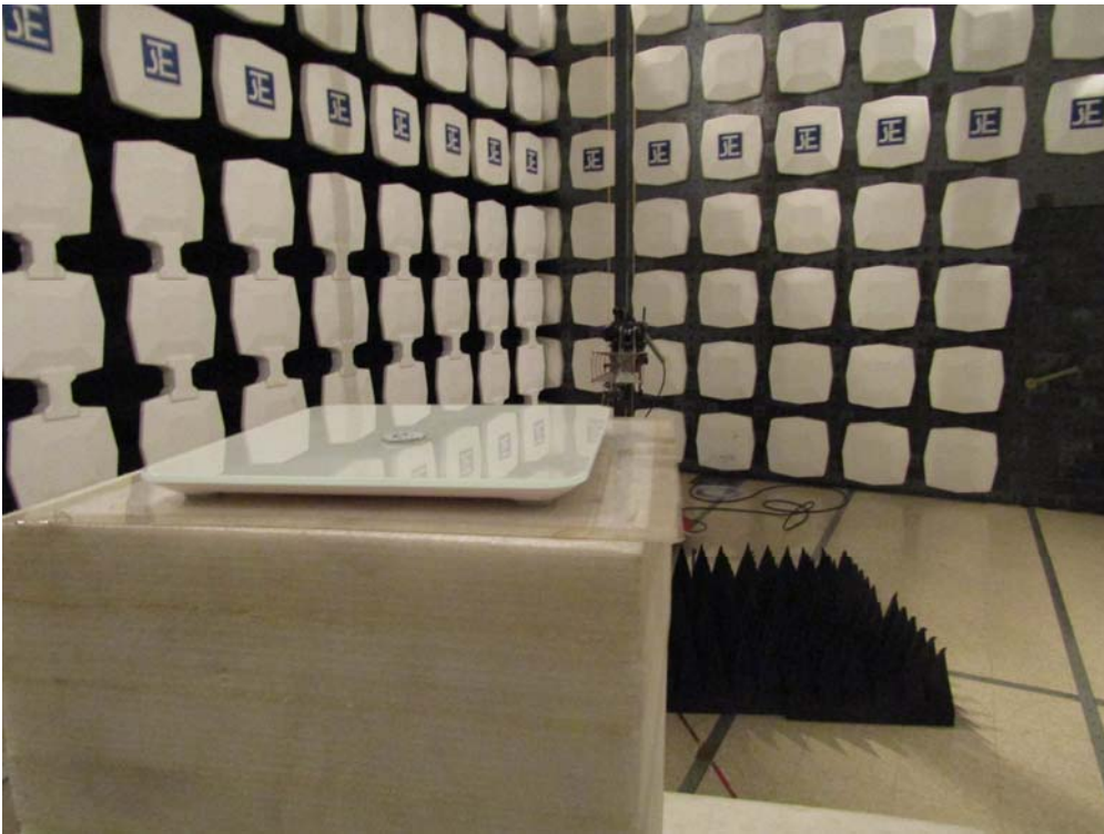
Measurement of Radiated Emission Test Set Up
