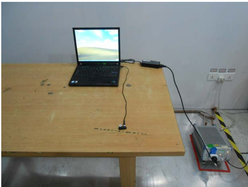
Photo of Setup for Conducted Emission Test
