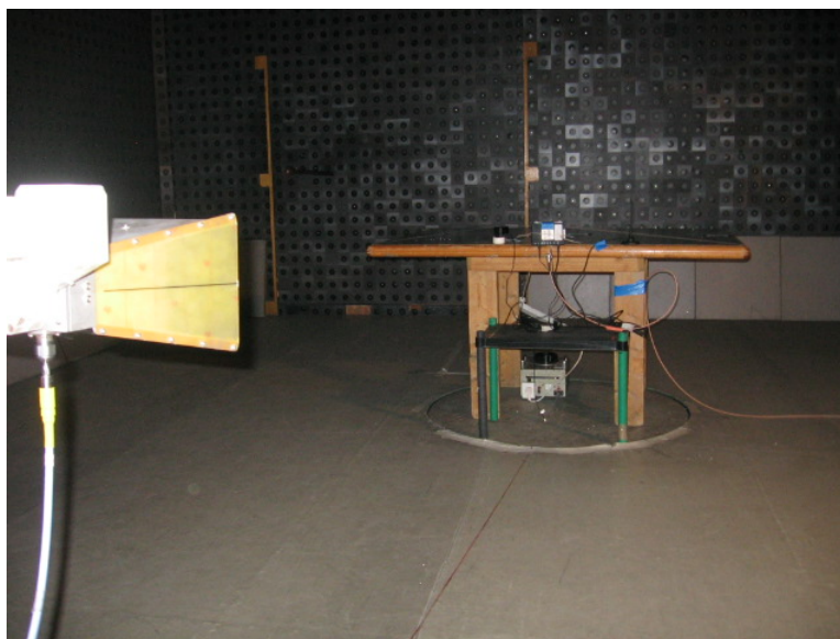
Photograph 8.2.2 Setup for radiated emission measurements
