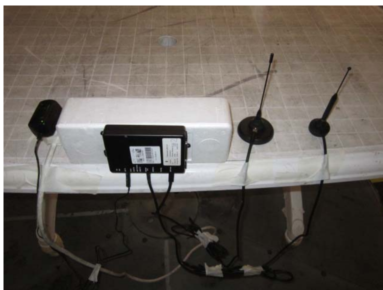
Photograph 8.2.4 Setup for radiated emission measurements, EUT cabling
