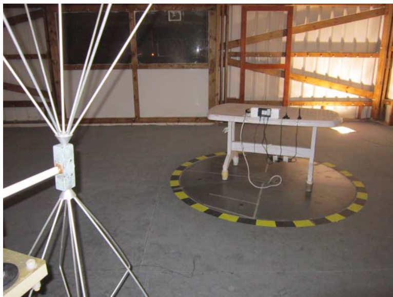
Photograph 8.2.3 Setup for radiated emission measurements, general view
