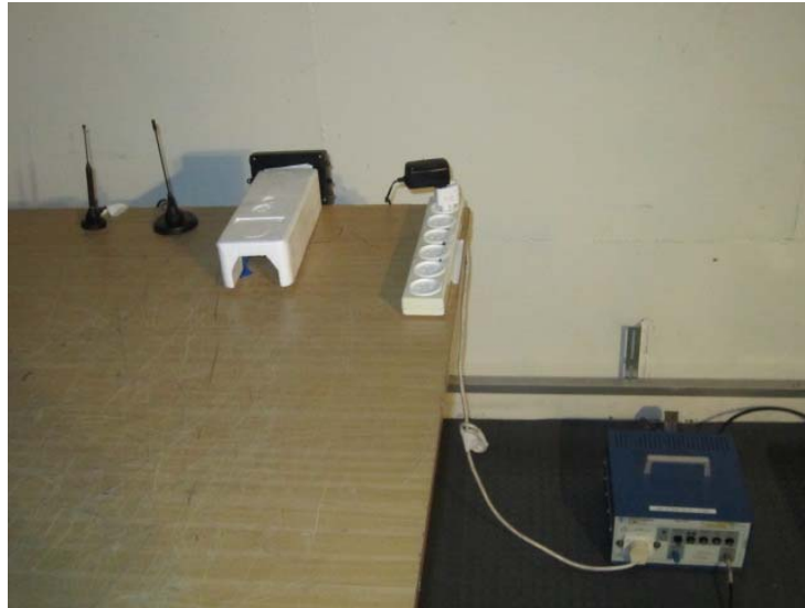
Photograph 8.1.2 Setup for conducted emissions measurements
