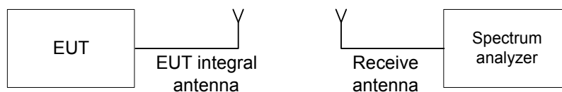
Figure 7.1.1 Setup for transmitter shut down test
