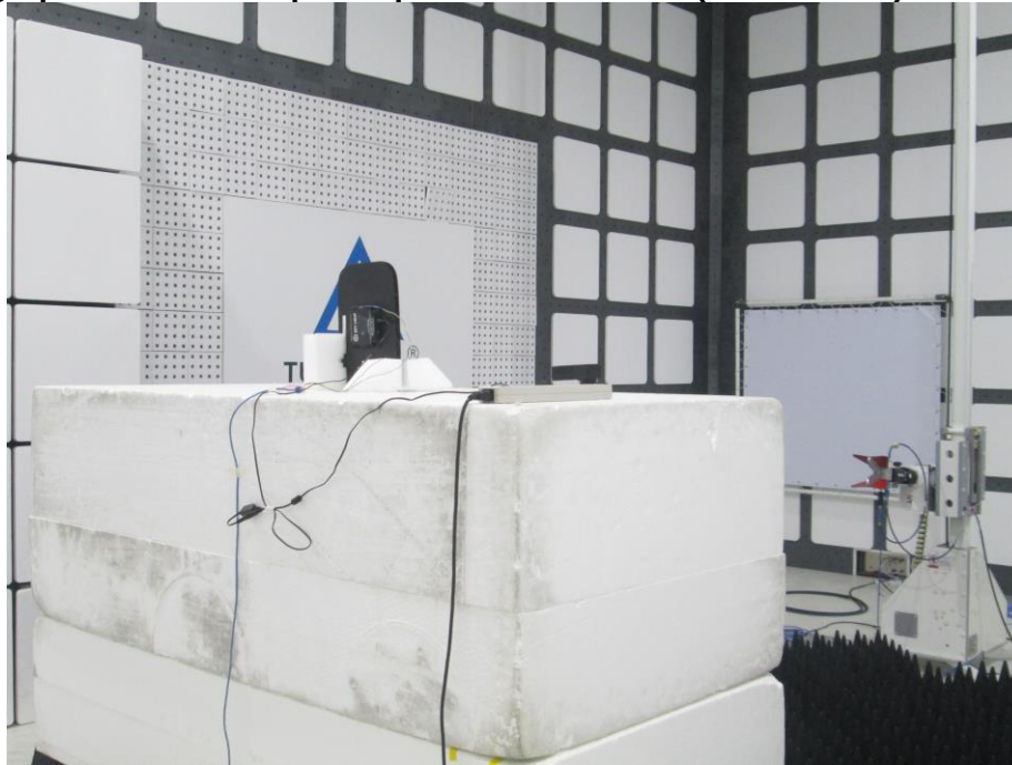
Photograph 14: Test Setup for Spurious Emissions (Back View 4)
