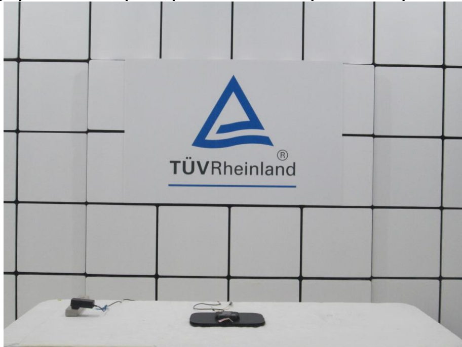
Photograph 1: Test Setup for Spurious Emissions (Front View 1)
