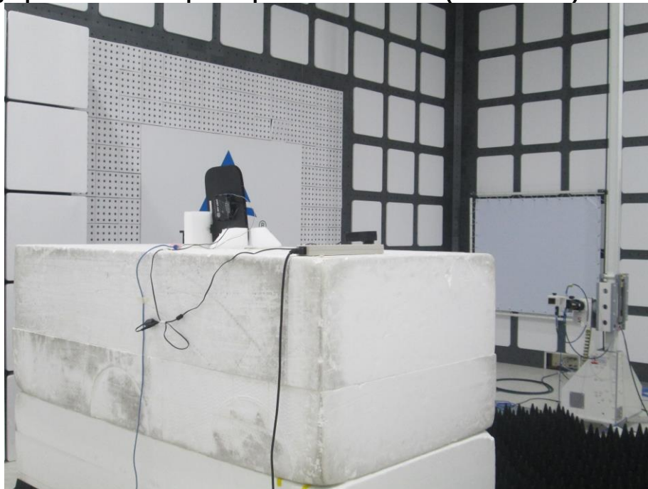
Photograph 14: Test Setup for Spurious Emissions (Back View 4)
