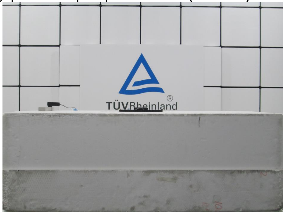
Photograph 2: Test Setup for Spurious Emissions (Front View 2)
