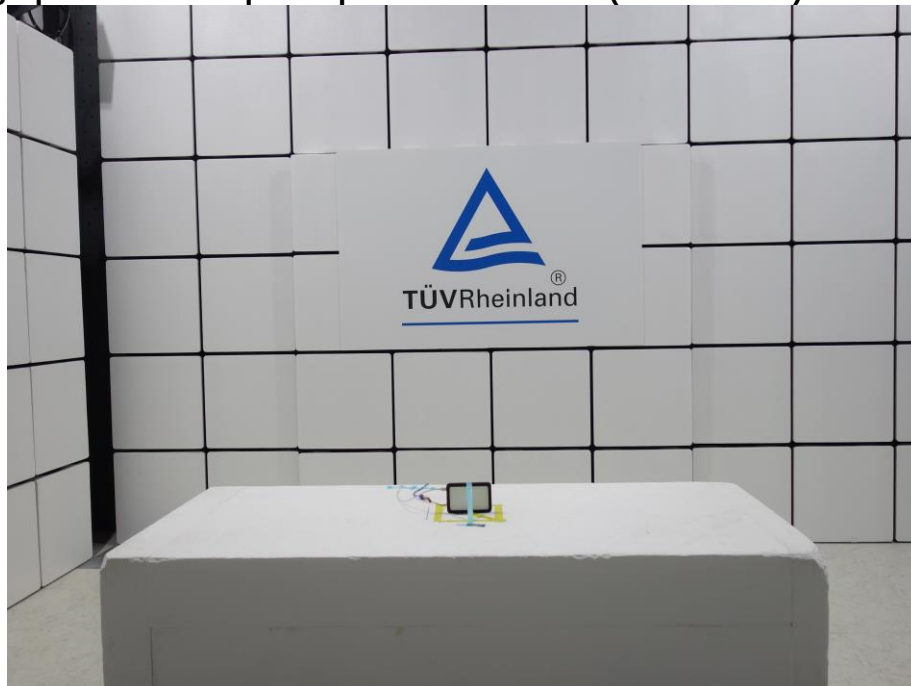
Photograph 2: Test Setup for Spurious Emissions (Front View 2)
