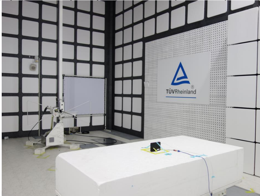
Photograph 5: Test Setup for Spurious Emissions (Back View 3)
