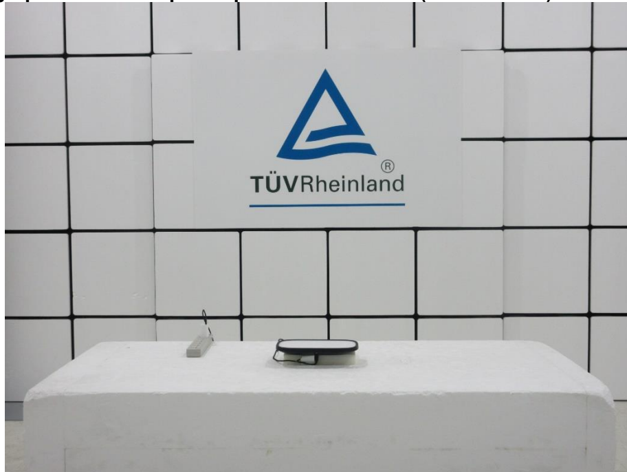
Photograph 1: Test Setup for Spurious Emissions (Front View 1)
