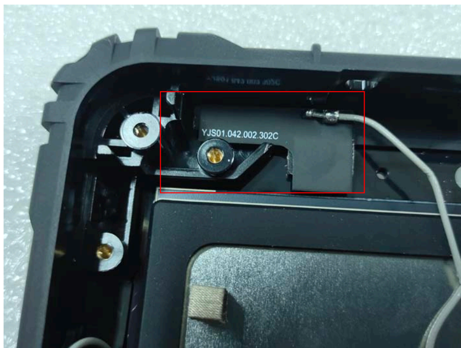
EUT – Main LTE Antenna View
