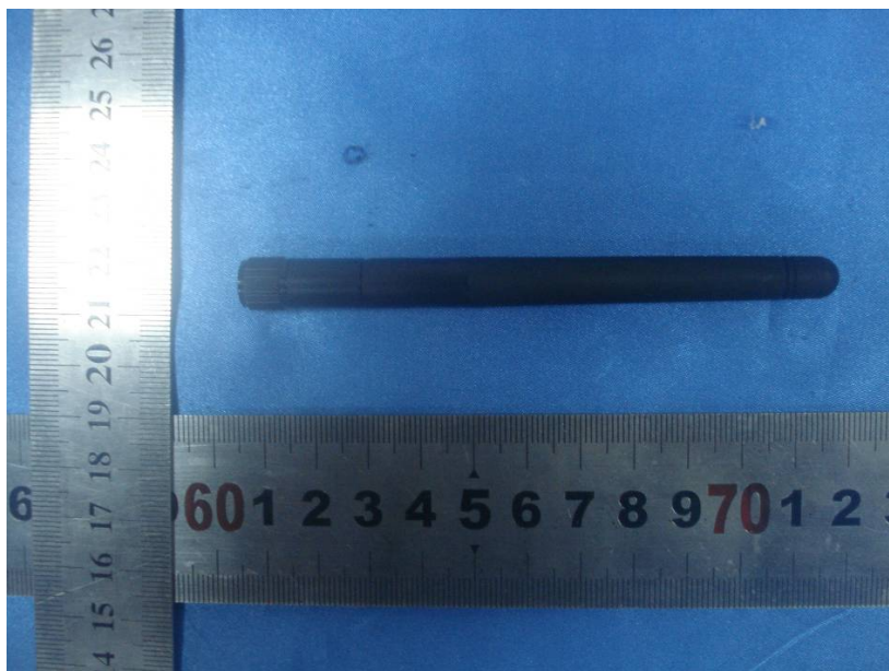
EUT – Zigbee Antenna View
