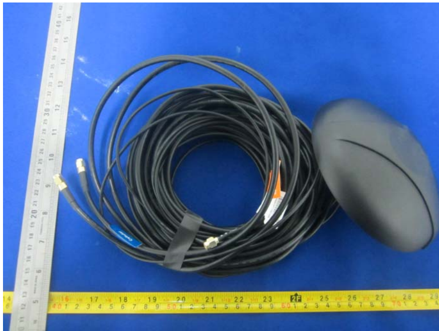
EUT – CDMA&Wifi&GPS Antenna View
