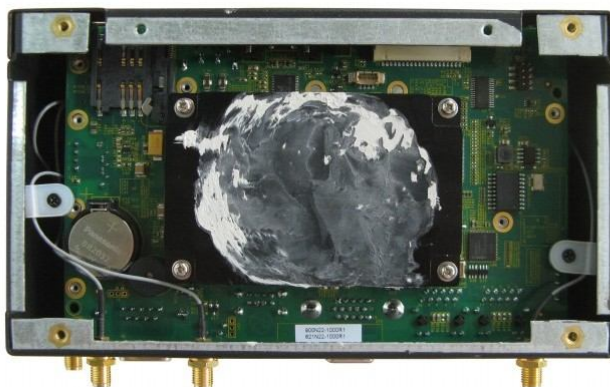
Top View for thermal module
