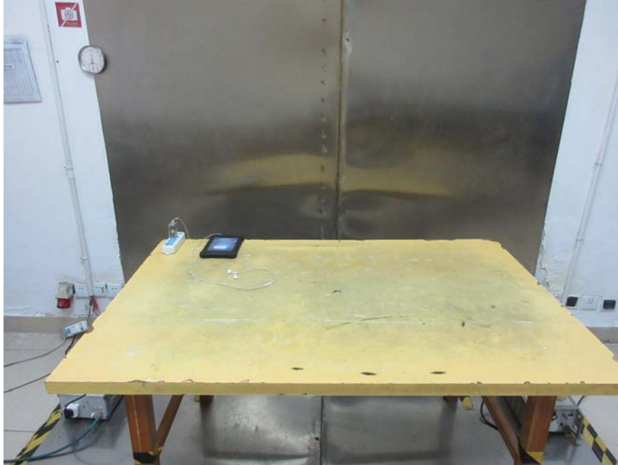
Conducted Emission Front View
