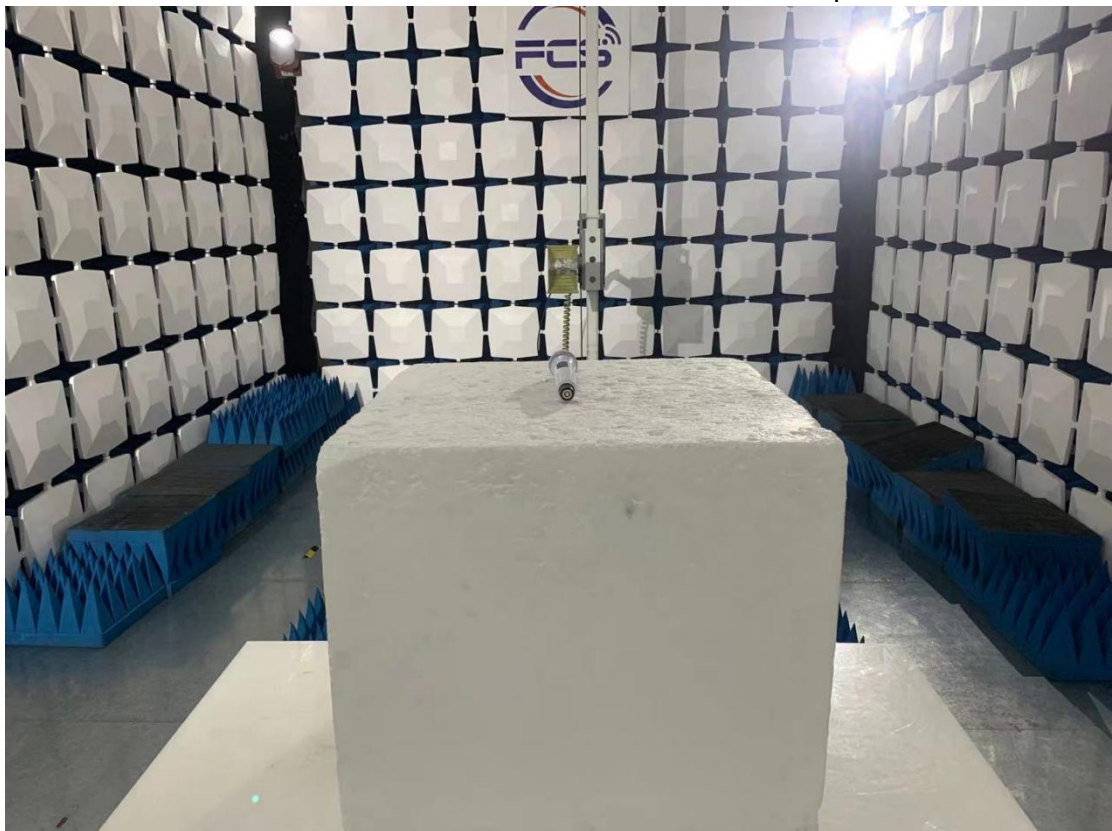
Above 1GHz for radiated emission test setup
