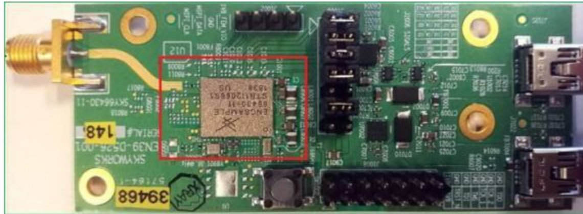
Picture 1. Dev board with SKY module integrated (module with conformal coating)
