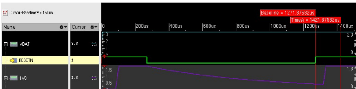
Figure 6. Typical Timing Diagram for Reset Sequence
