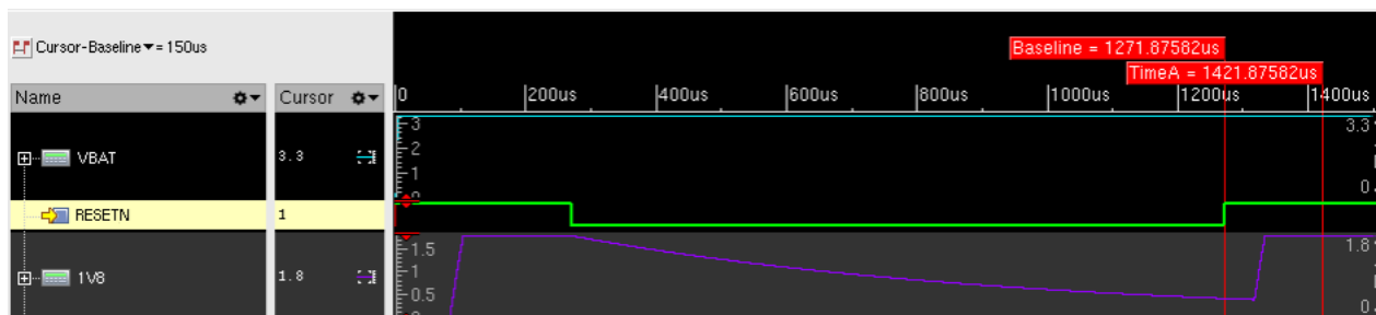
Figure 2-3: Timing Diagram for Reset Sequence
