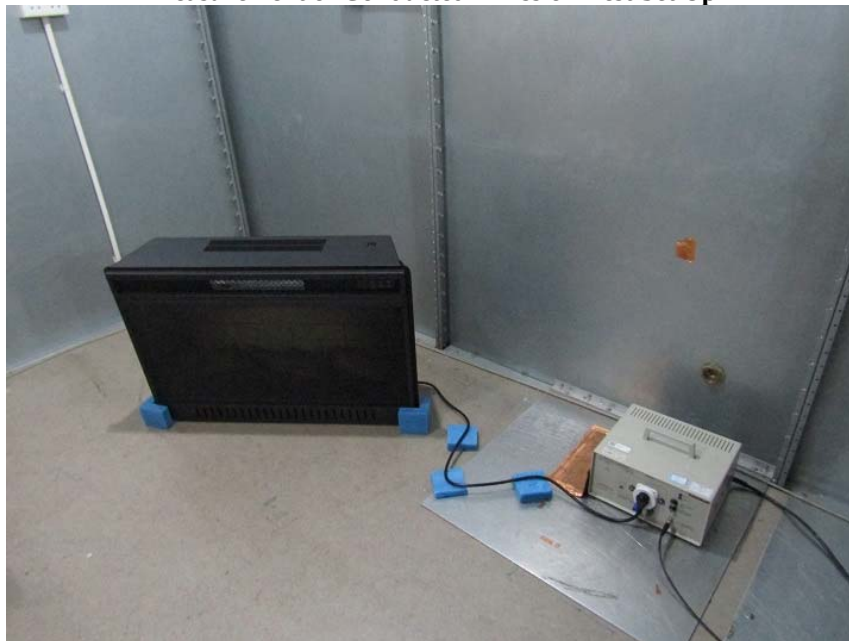
Measurement of Conducted Emission Test Set Up
