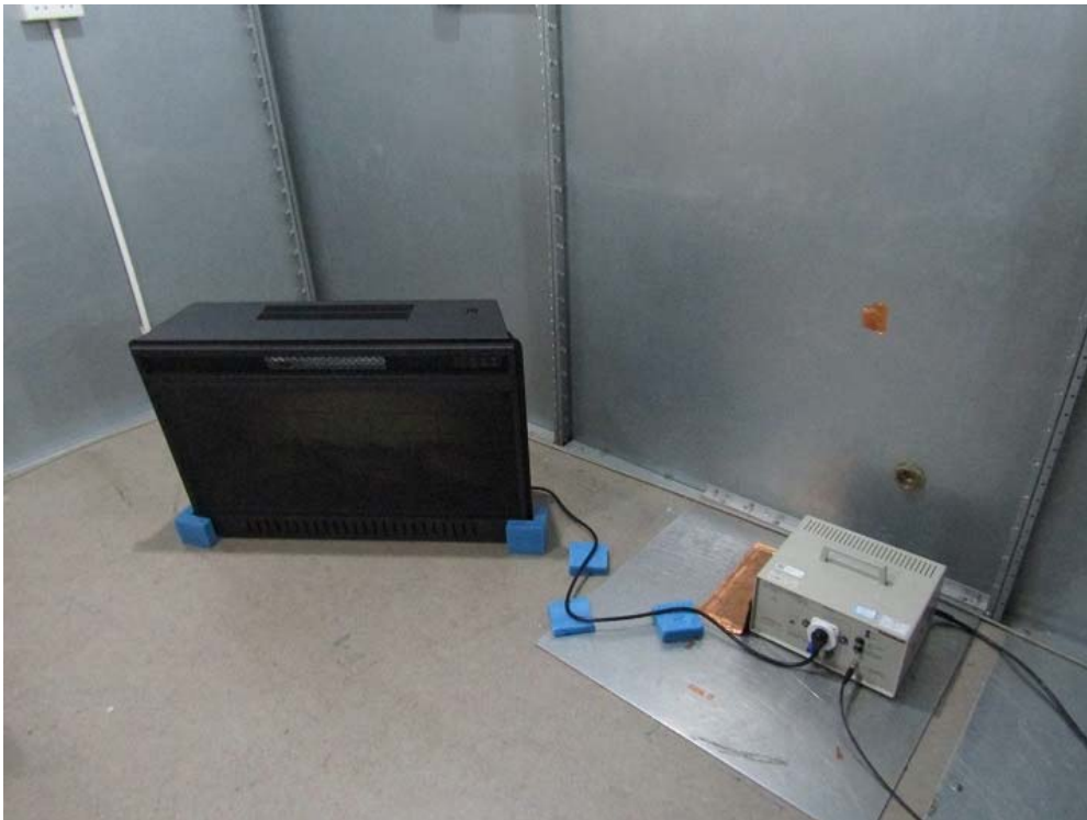
Measurement of Conducted Emission Test Set Up
