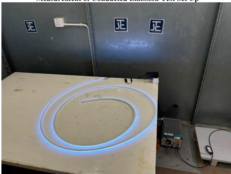
Measurement of Conducted Emission Test Set Up
