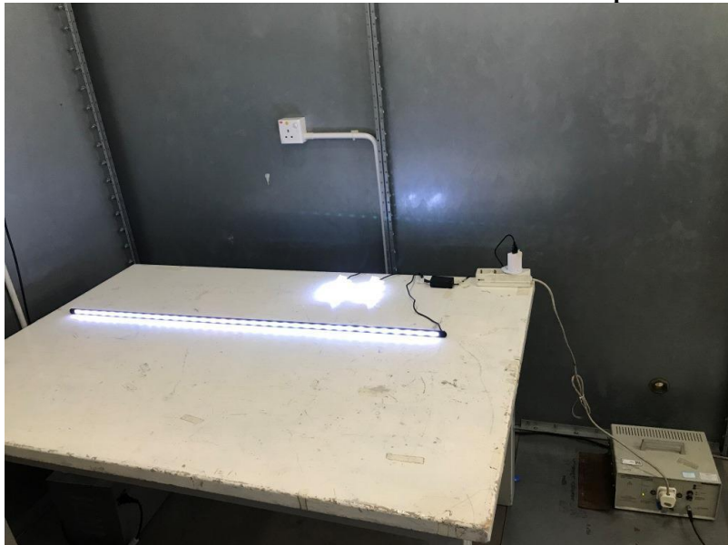
Measurement of Conducted Emission Test Set Up
