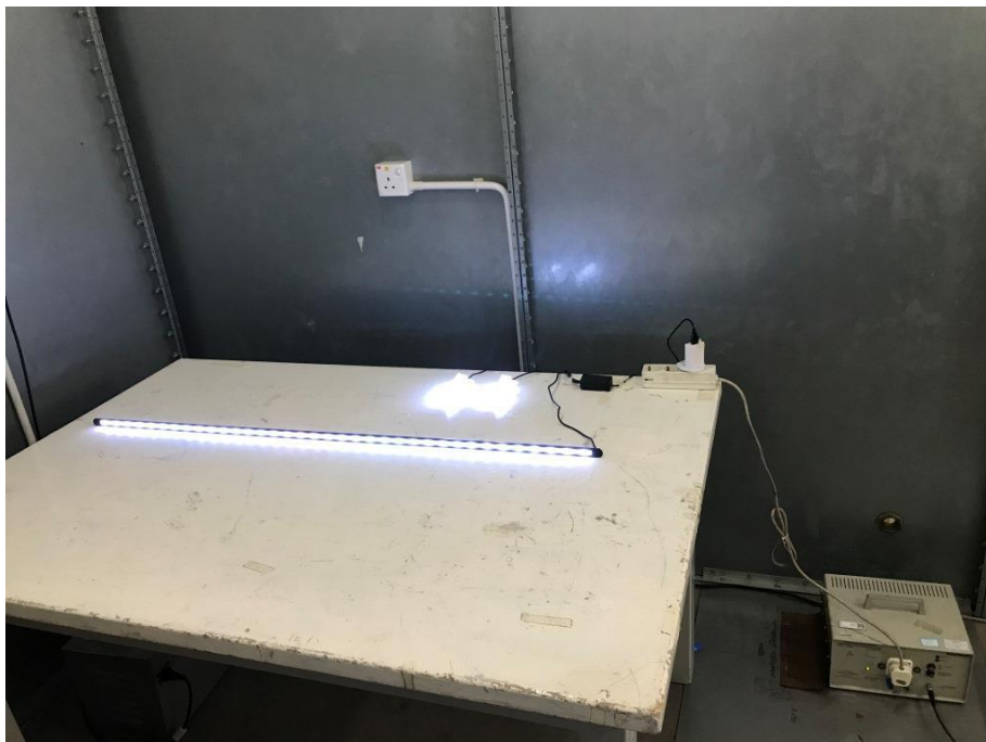
Measurement of Conducted Emission Test Set Up
