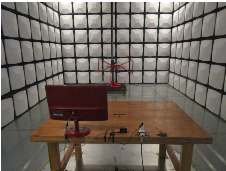
Radiated Emissions Below 1GHz –Rear View (HDMI)
