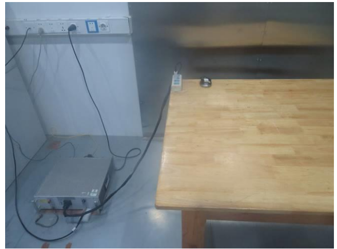
Conducted Emissions Test Setup Side View
