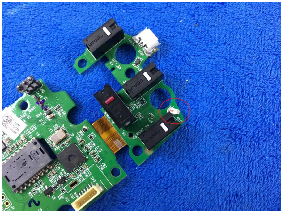
BT - Antenna View
