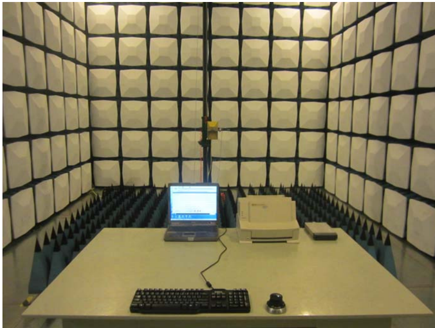
Radiated Emission - Front View (Above 1GHz)
