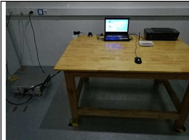
Conducted Emissions Test Setup – Front View
