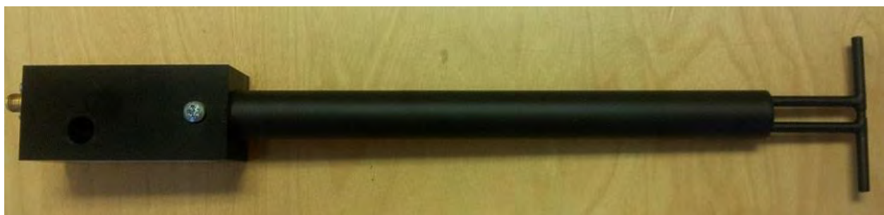
Figure 1 – MVG COMOSAR Validation Dipole
