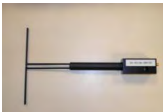
Figure 1 – MVG COMOSAR Validation Dipole
