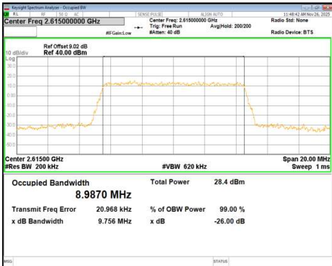
Band38 QPSK BW=15MHz Channel=37825 RB Size=75 Position=#0
