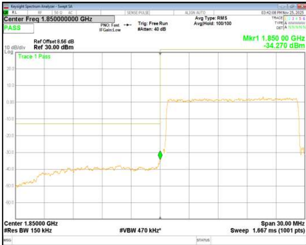
Band2 QPSK BW=15MHz Channel=19125 RB Size=75 Position=#0
