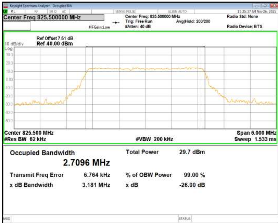
Band26(824-849) 16QAM BW=3MHz Channel=26915 RB Size=15 Position=#0
