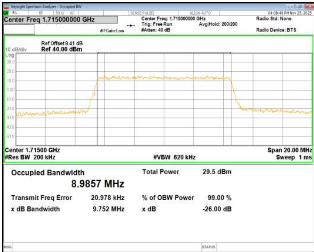
Band4 QPSK BW=10MHz Channel=20175 RB Size=50 Position=#0
