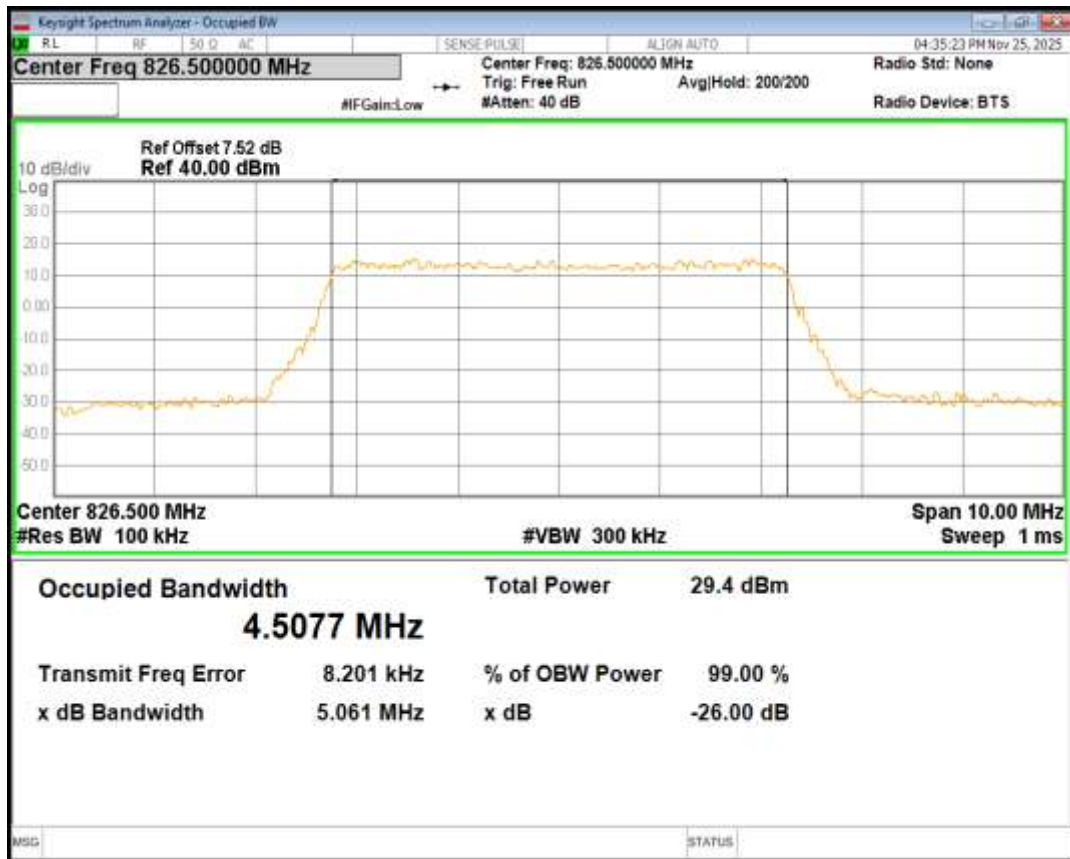
Band5 QPSK BW=5MHz Channel=20625 RB Size=25 Position=#0
