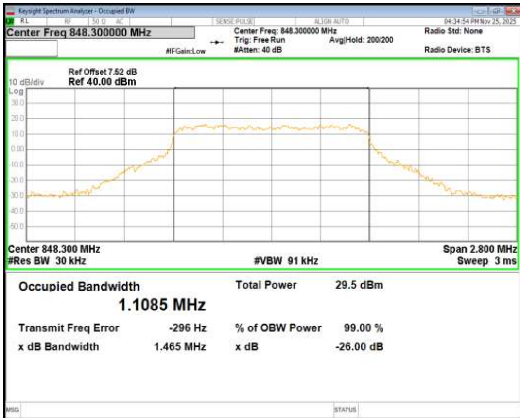
Band5 QPSK BW=1.4MHz Channel=20525 RB Size=6 Position=#0
