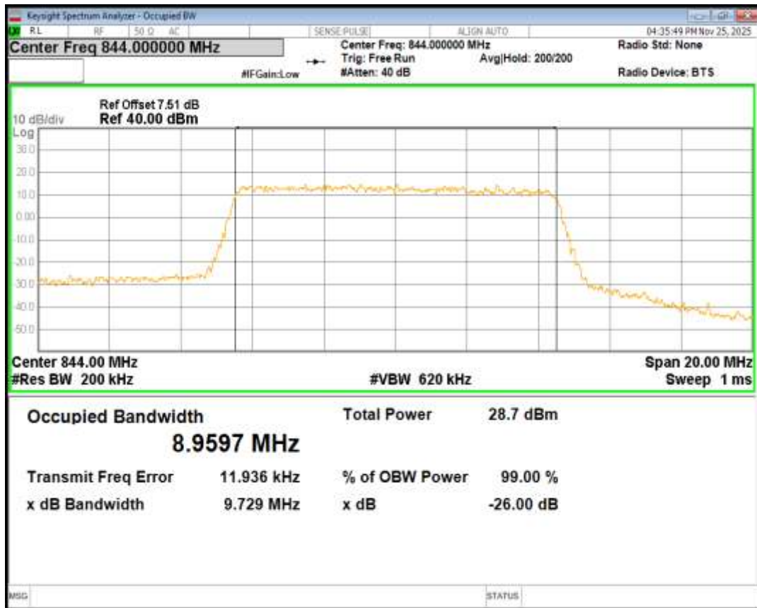
Band7 16QAM BW=5MHz Channel=20775 RB Size=25 Position=#0
