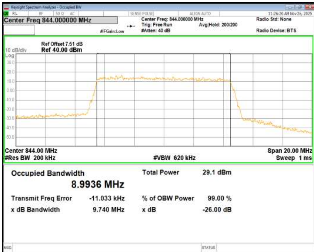
Band26(824-849) QPSK BW=15MHz Channel=26865 RB Size=75 Position=#0
