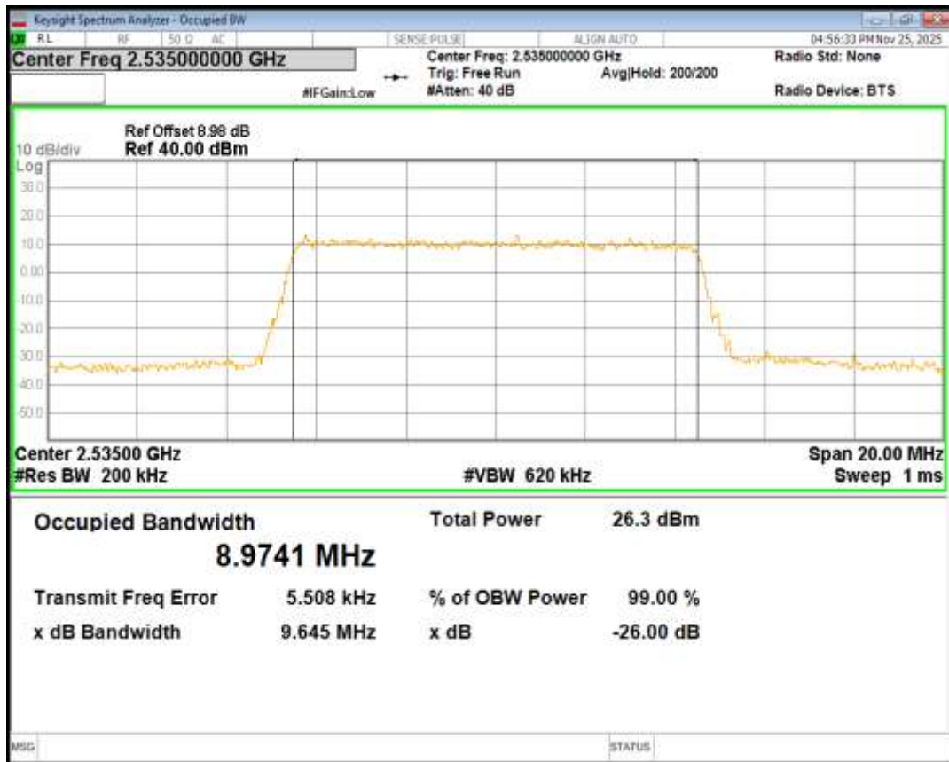
Band7 QPSK BW=10MHz Channel=21400 RB Size=50 Position=#0
