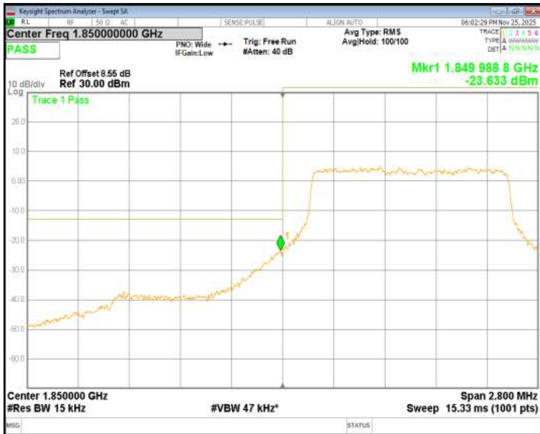
Band25 QPSK BW=1.4MHz Channel=26683 RB Size=6 Position=#0
