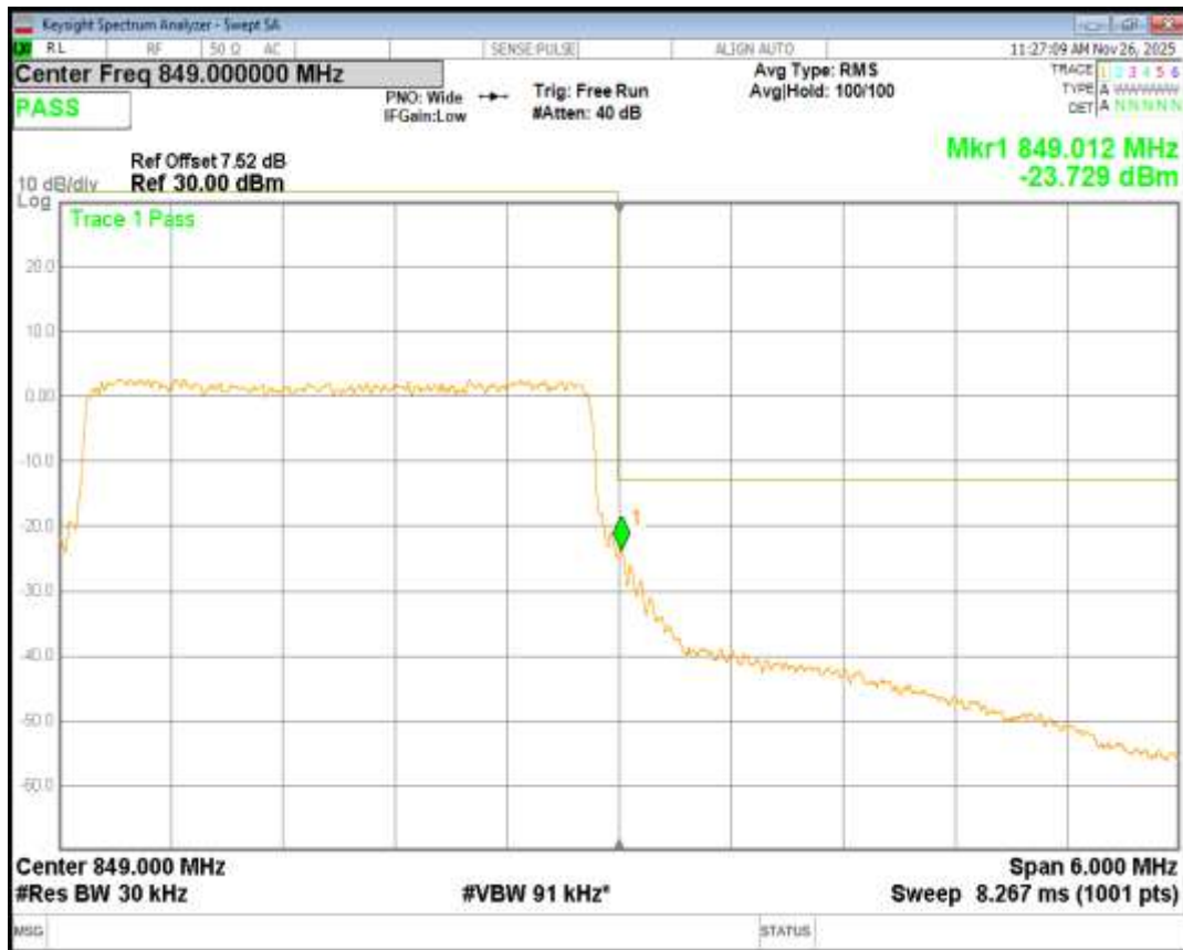
Band26(824-849) 16QAM BW=5MHz Channel=26815 RB Size=25 Position=#0
