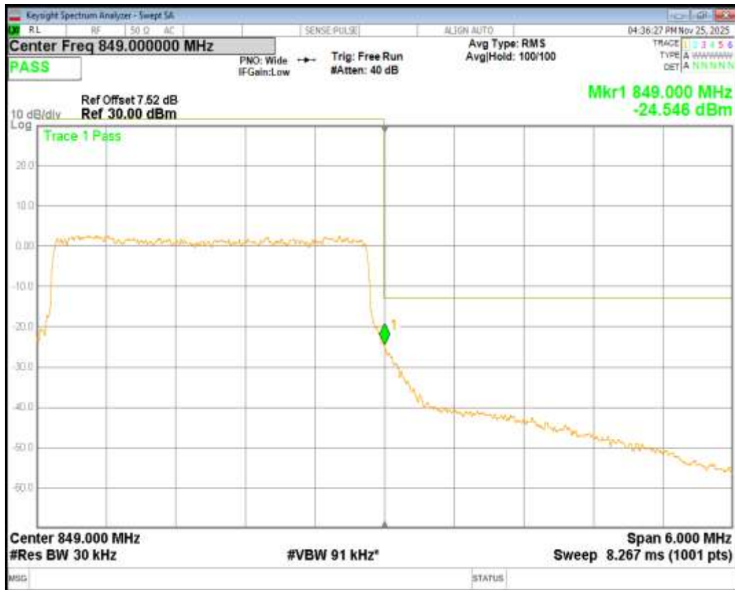
Band5 16QAM BW=5MHz Channel=20425 RB Size=25 Position=#0
