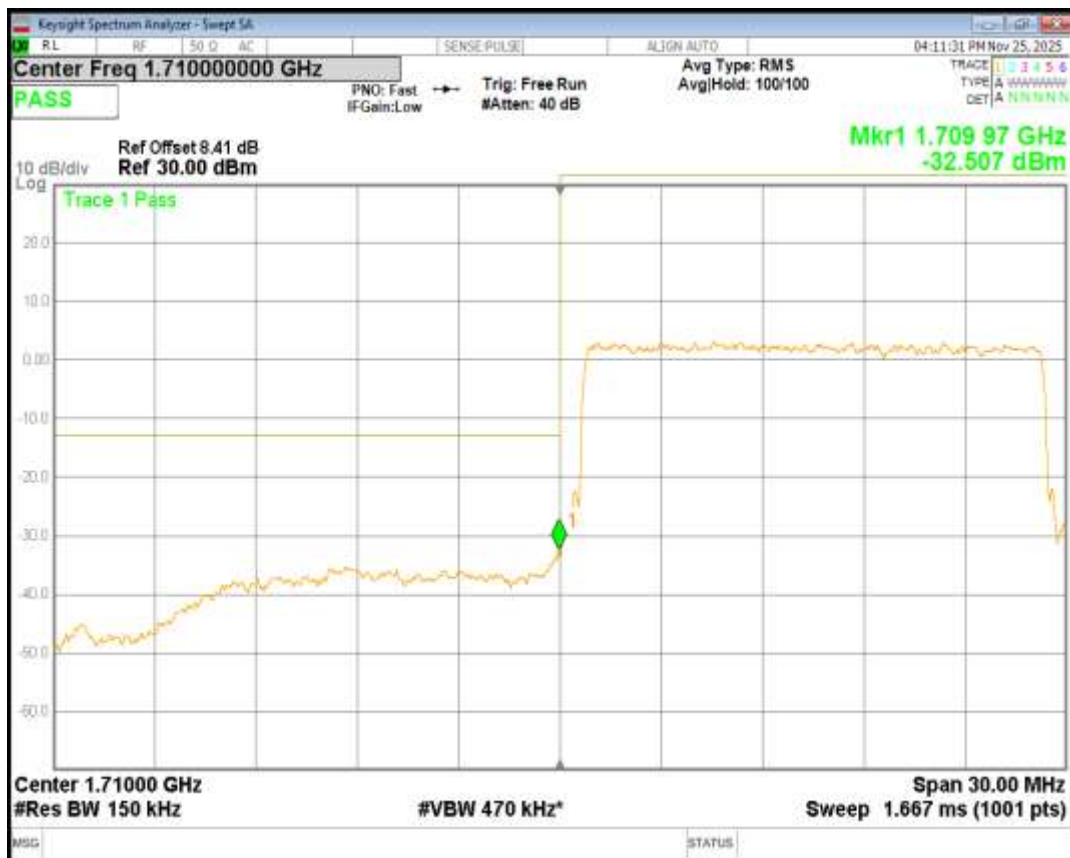
Band4 QPSK BW=15MHz Channel=20325 RB Size=75 Position=#0
