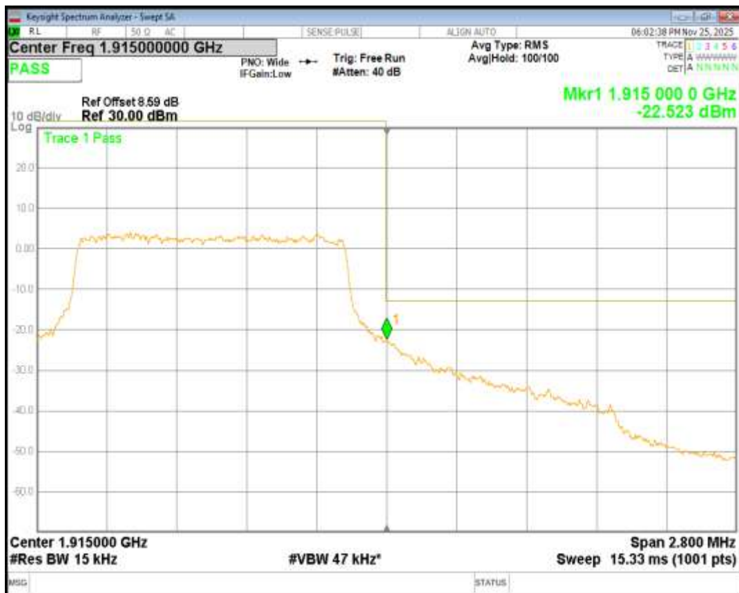
Band25 QPSK BW=3MHz Channel=26055 RB Size=15 Position=#0
