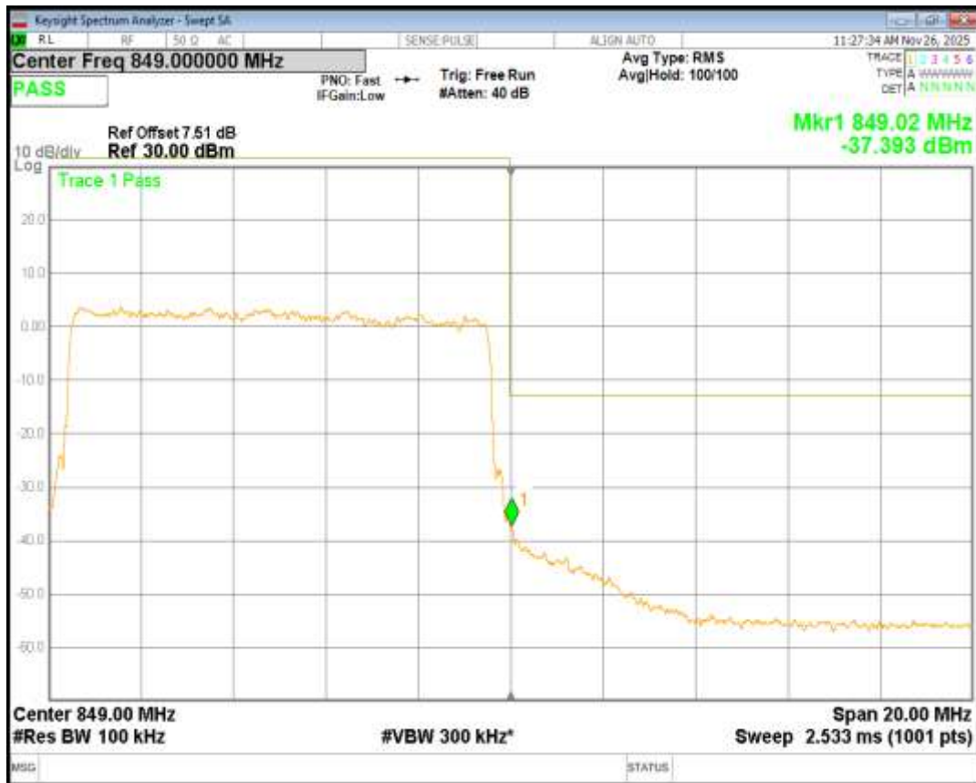
Band26(824-849) QPSK BW=15MHz Channel=26865 RB Size=75 Position=#0
