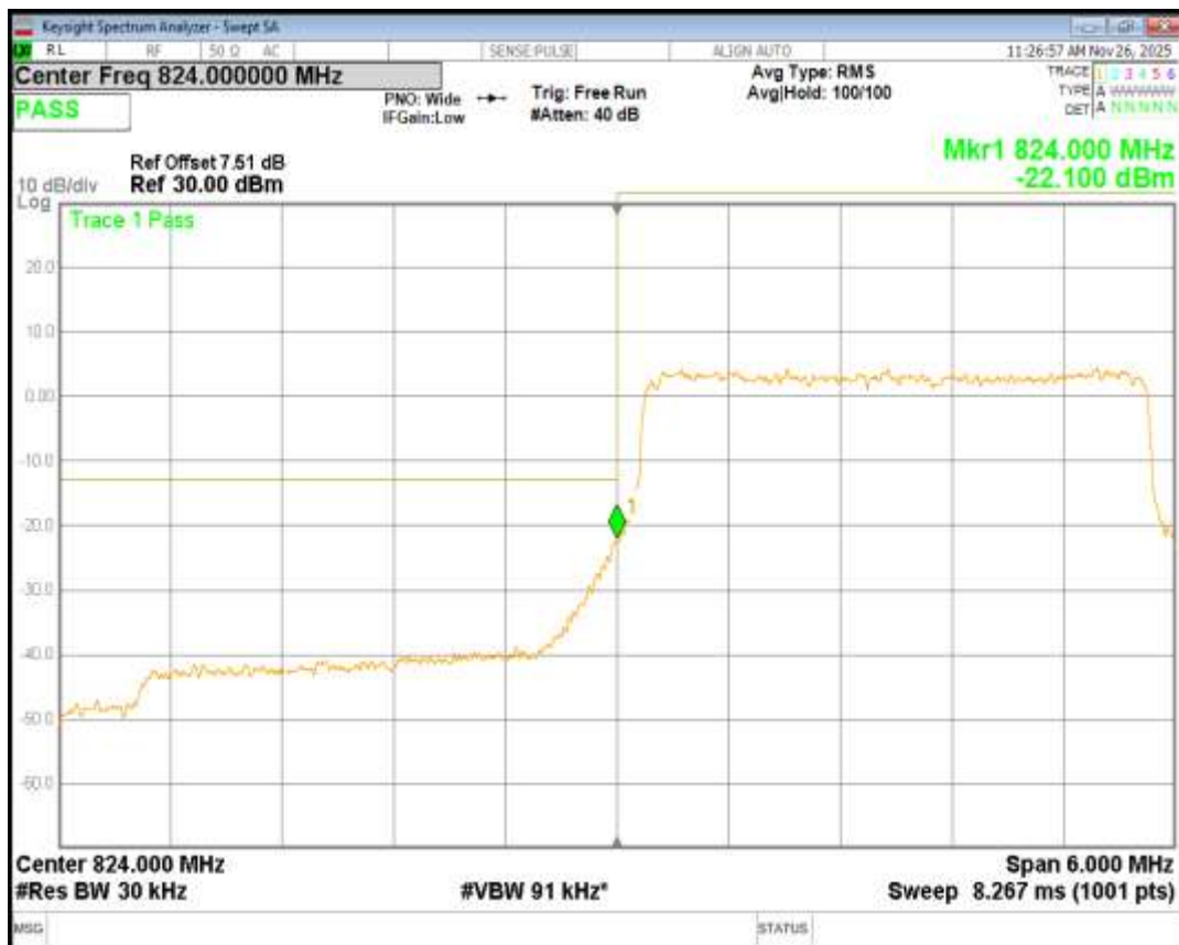
Band26(824-849) QPSK BW=3MHz Channel=27025 RB Size=15 Position=#0
