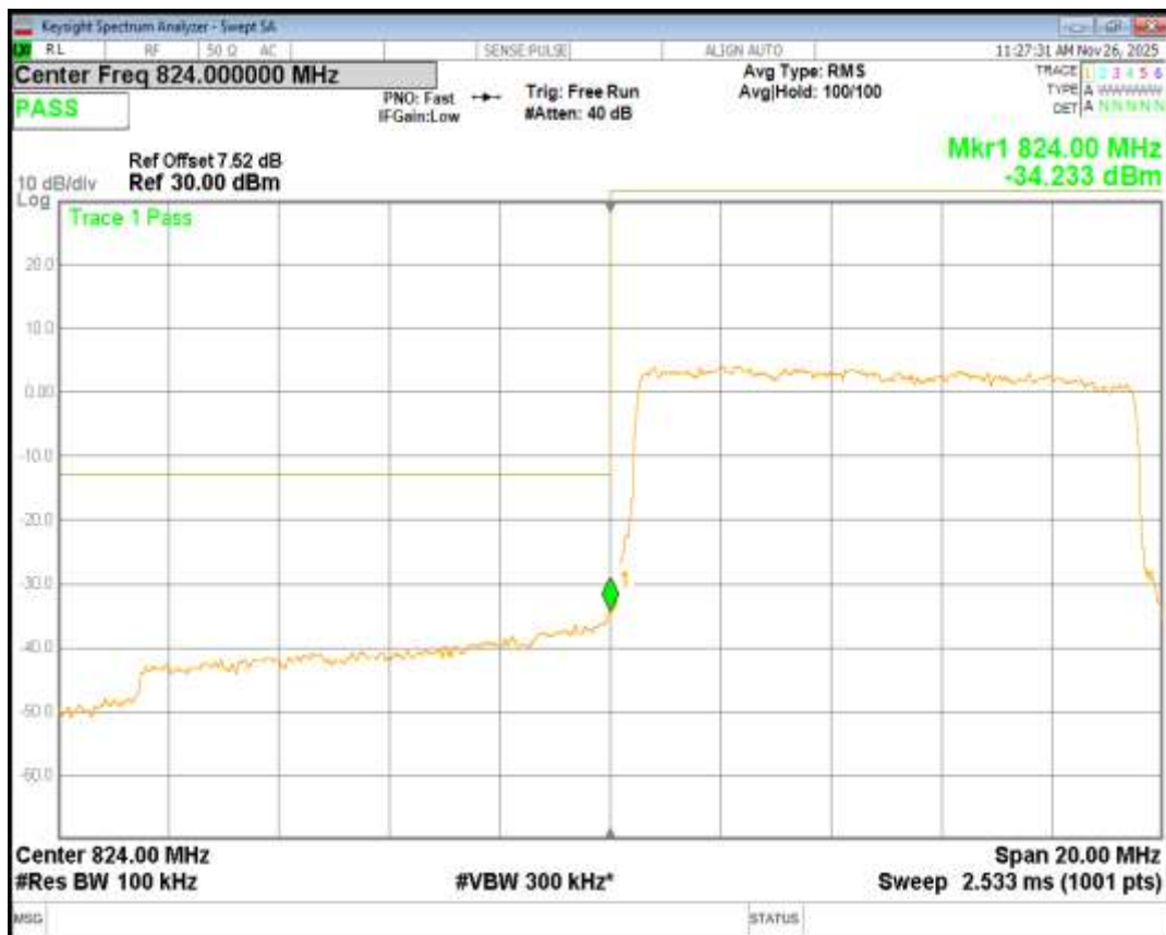
Band26(824-849) QPSK BW=10MHz Channel=26990 RB Size=50 Position=#0
