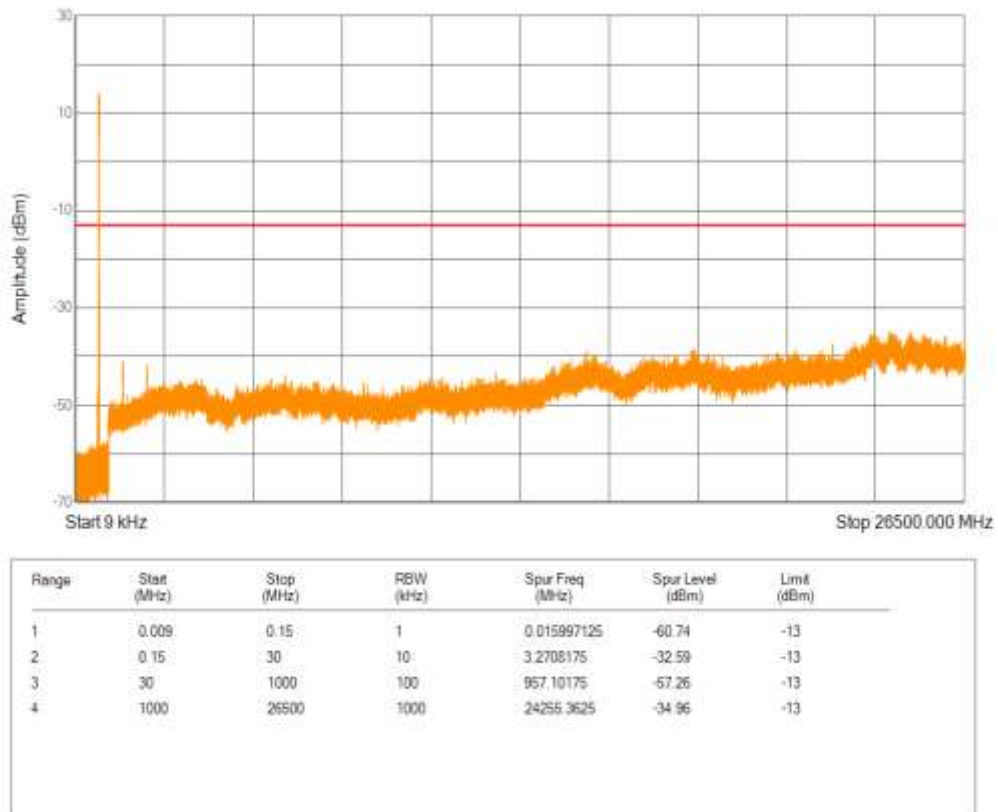
Band12 QPSK BW=10MHz Channel=23060 RB Size=50 Position=#0
