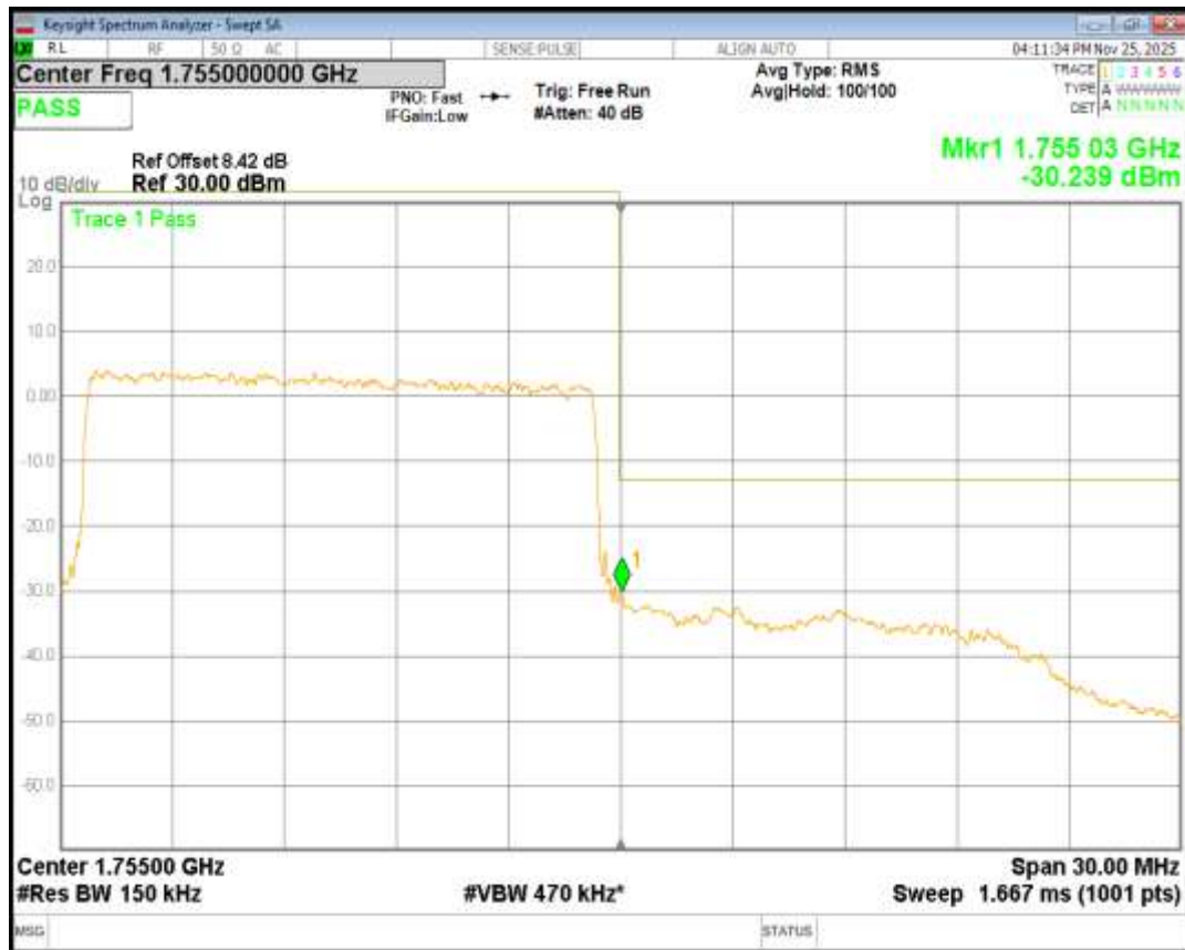
Band4 QPSK BW=20MHz Channel=20050 RB Size=100 Position=#0
