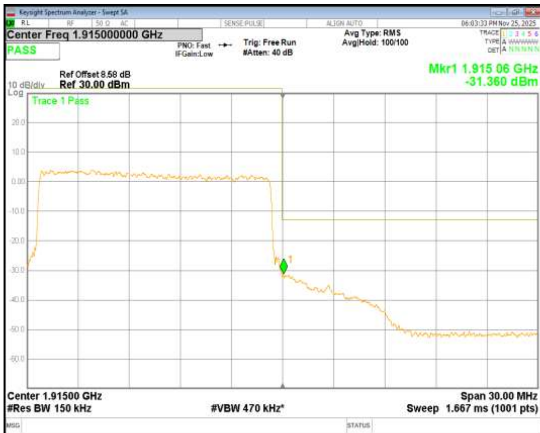
Band25 QPSK BW=20MHz Channel=26140 RB Size=100 Position=#0
