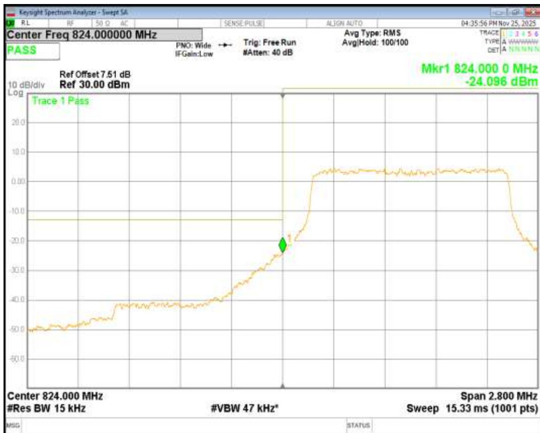
Band5 QPSK BW=1.4MHz Channel=20643 RB Size=6 Position=#0
