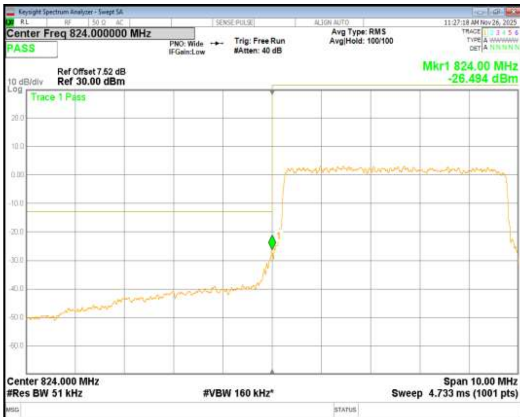
Band26(824-849) 16QAM BW=5MHz Channel=27015 RB Size=25 Position=#0
