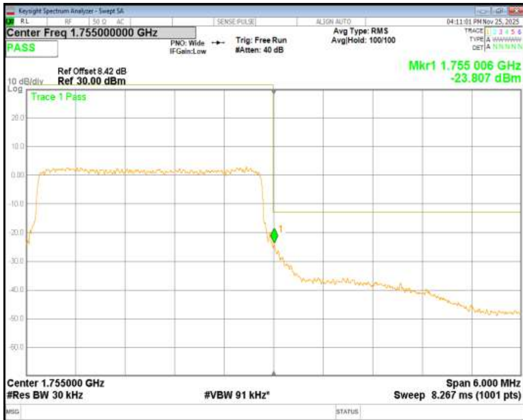
Band4 16QAM BW=5MHz Channel=19975 RB Size=25 Position=#0
