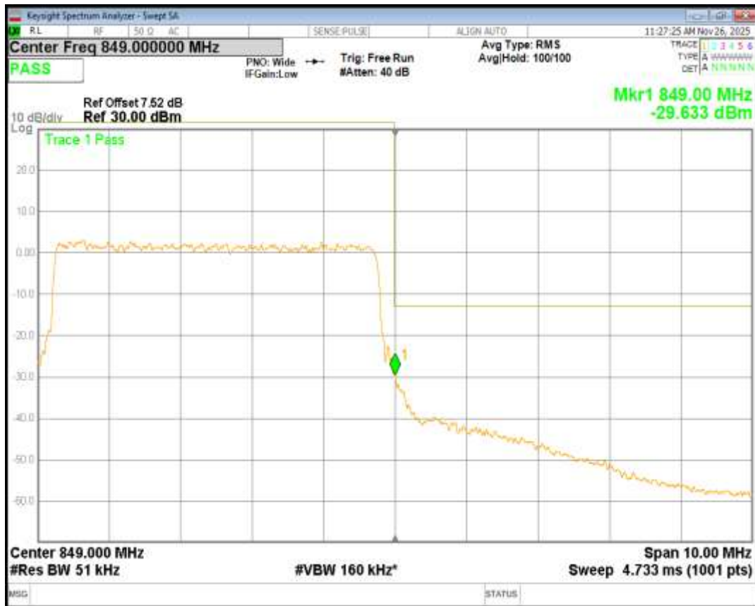
Band26(824-849) QPSK BW=1.4MHz Channel=26797 RB Size=6 Position=#0
