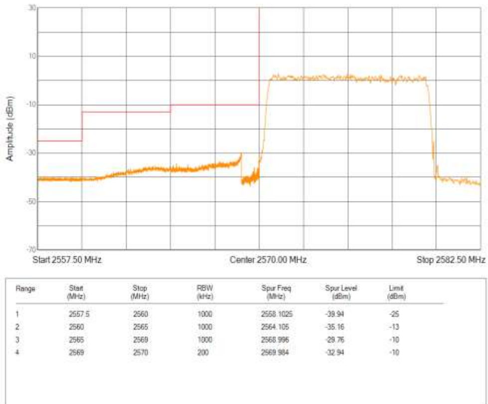
Band38 QPSK BW=10MHz Channel=38200 RB Size=50 Position=#0
