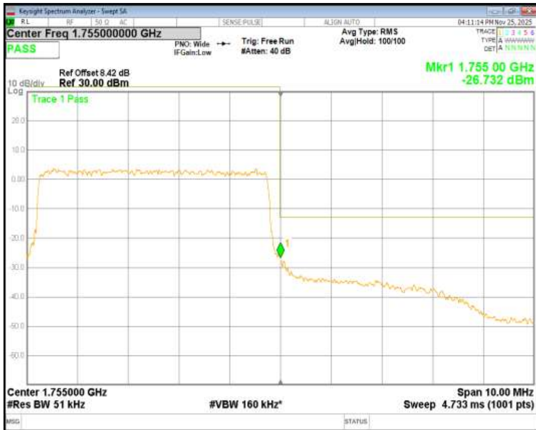
Band4 QPSK BW=10MHz Channel=20000 RB Size=50 Position=#0
