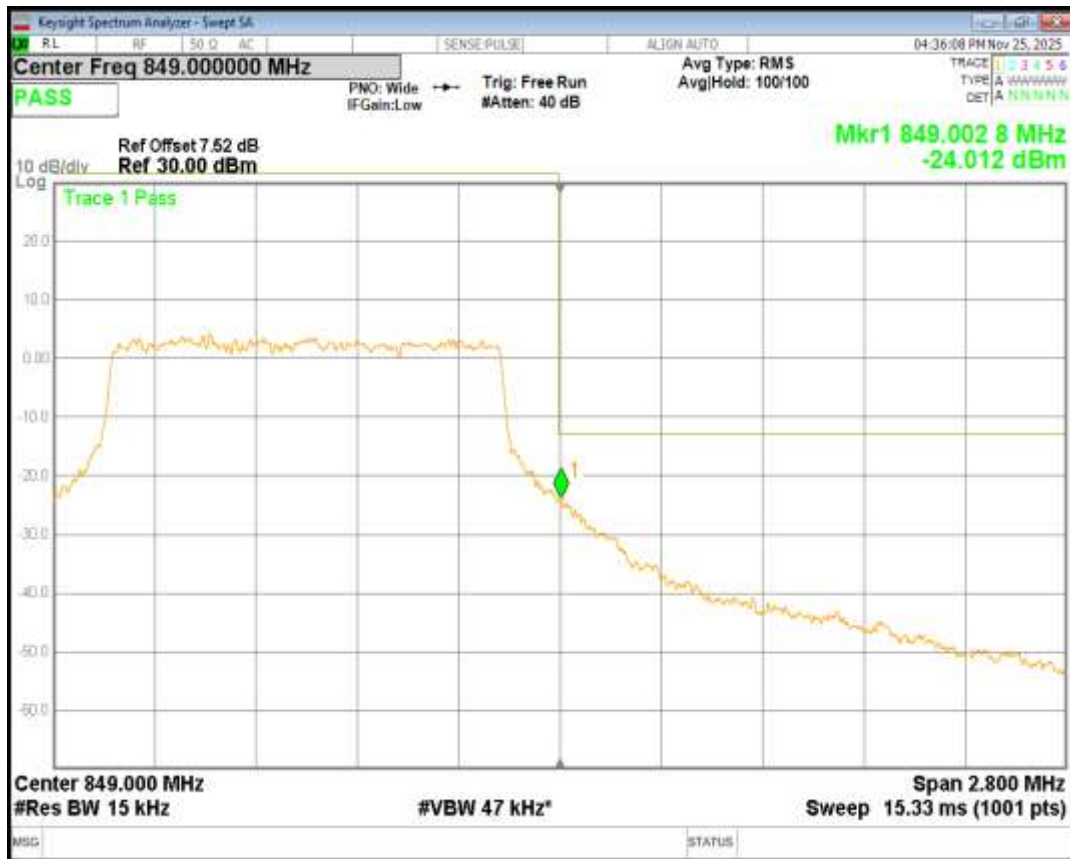
Band5 16QAM BW=3MHz Channel=20415 RB Size=15 Position=#0
