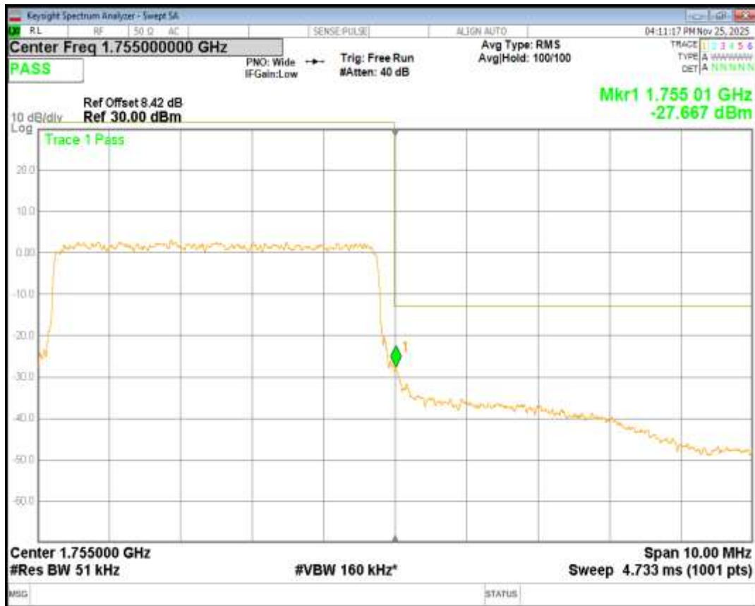
Band4 QPSK BW=1.4MHz Channel=19957 RB Size=6 Position=#0
