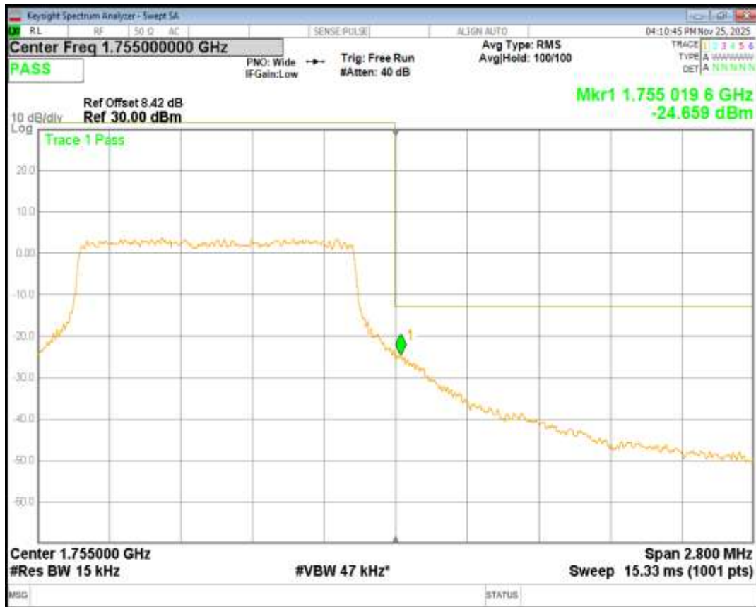
Band4 16QAM BW=3MHz Channel=19965 RB Size=15 Position=#0
