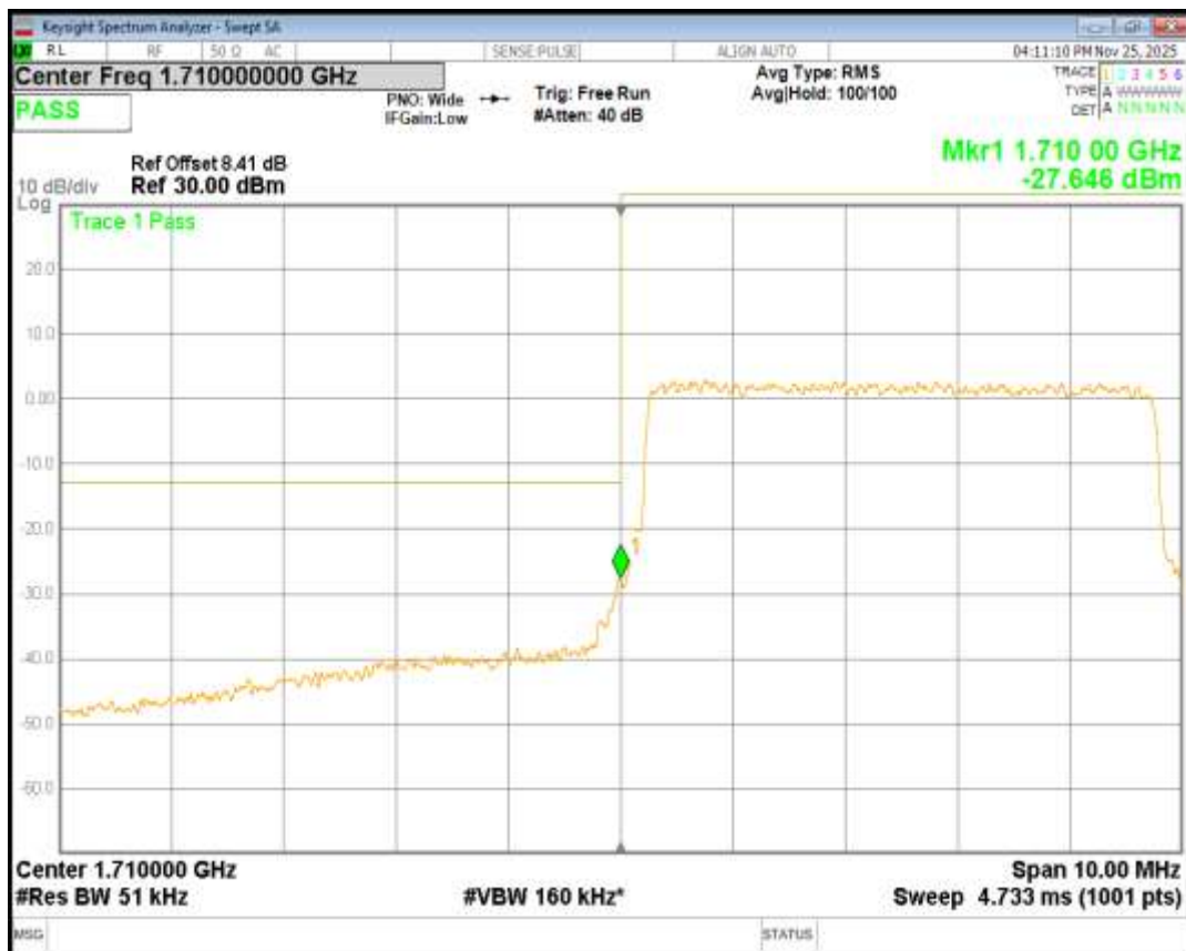
Band4 16QAM BW=5MHz Channel=20375 RB Size=25 Position=#0
