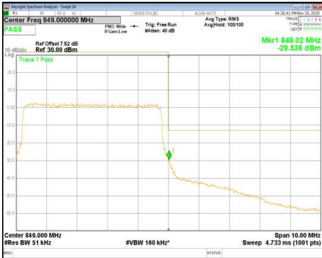
Band5 QPSK BW=1.4MHz Channel=20407 RB Size=6 Position=#0
