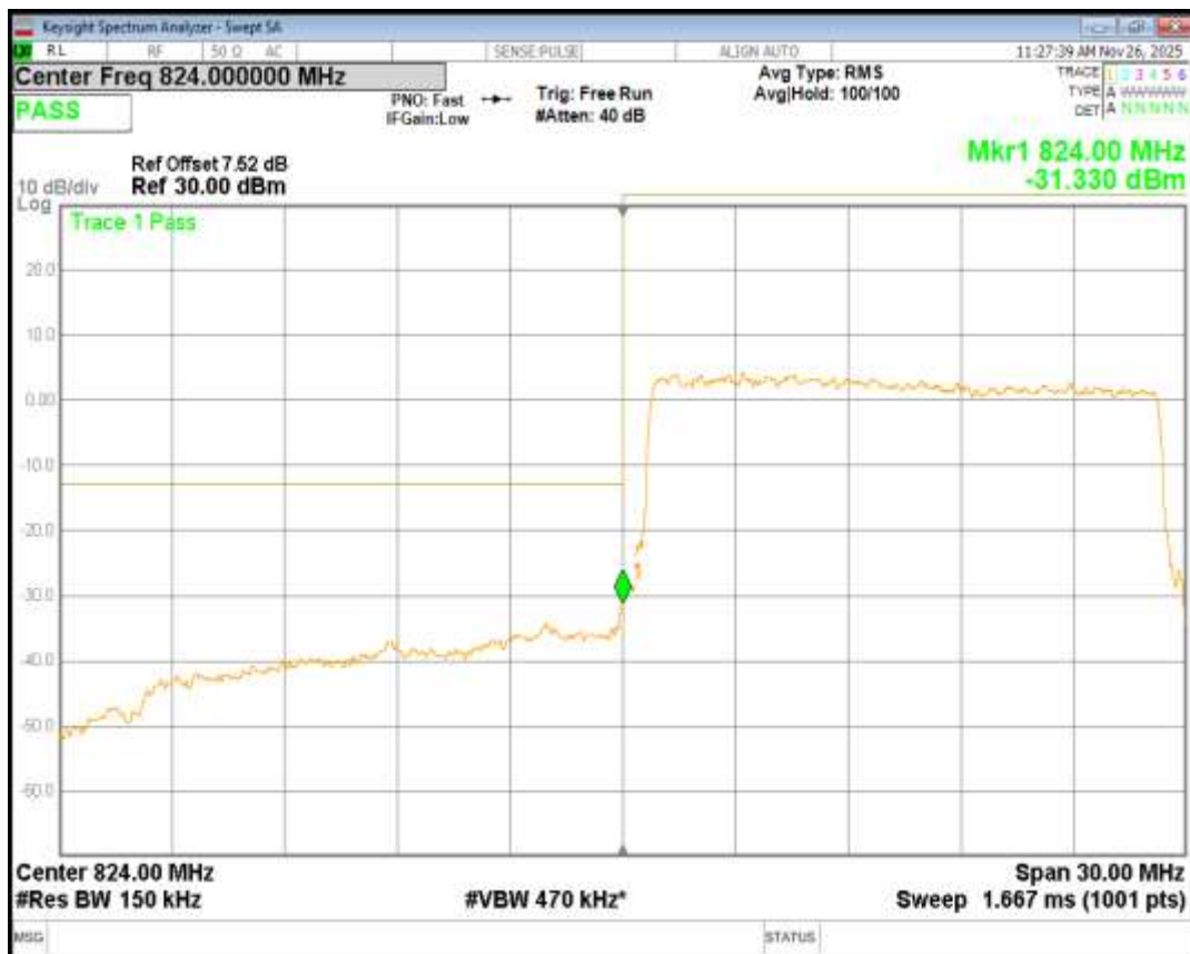
Band26(824-849) QPSK BW=15MHz Channel=26965 RB Size=75 Position=#0
