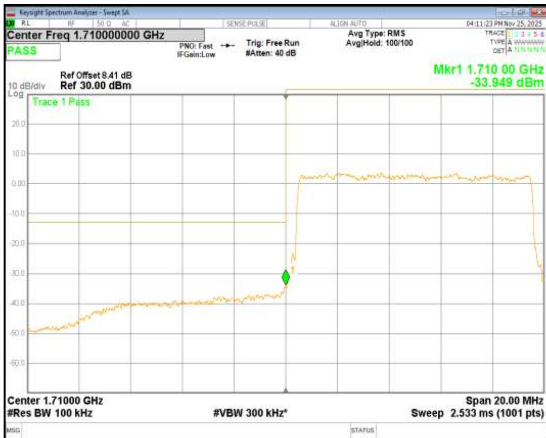
Band4 QPSK BW=10MHz Channel=20350 RB Size=50 Position=#0
