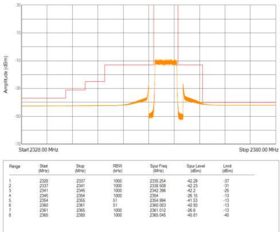
Band40(2350-2360) QPSK BW=5MHz Channel=39175 RB Size=25 Position=#0
