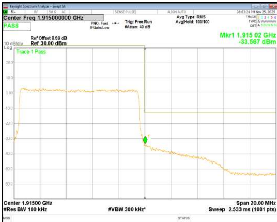
Band25 QPSK BW=15MHz Channel=26115 RB Size=75 Position=#0
