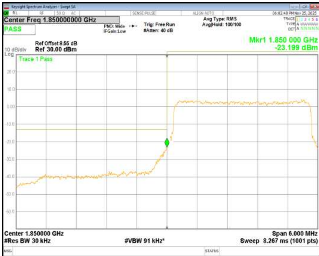
Band25 QPSK BW=3MHz Channel=26675 RB Size=15 Position=#0
