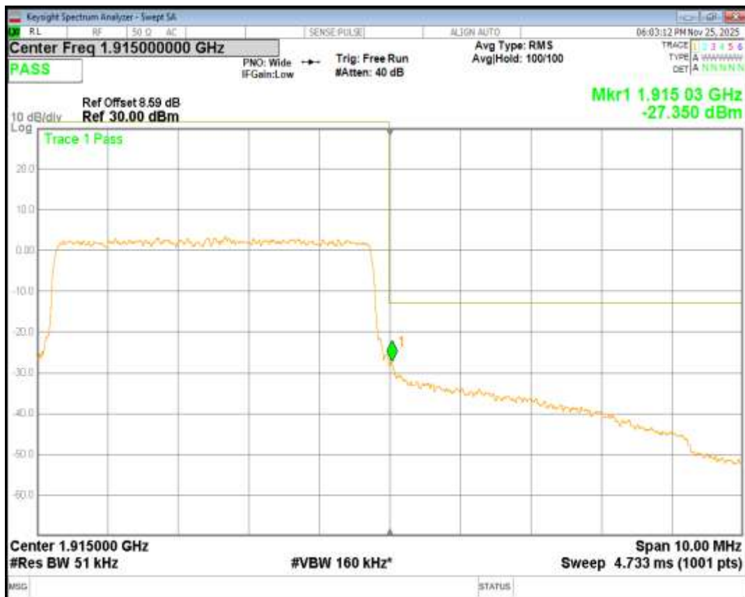
Band25 QPSK BW=10MHz Channel=26090 RB Size=50 Position=#0
