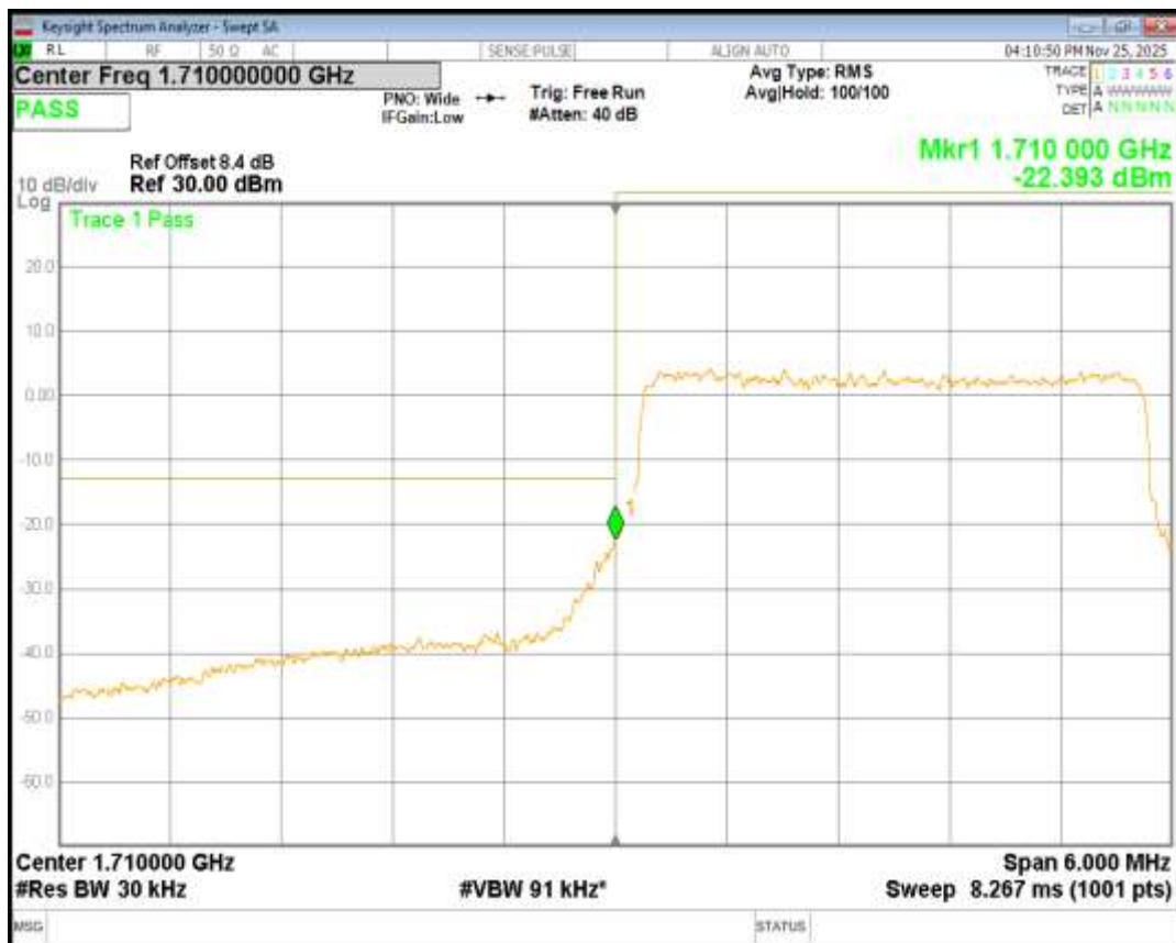
Band4 QPSK BW=3MHz Channel=20385 RB Size=15 Position=#0
