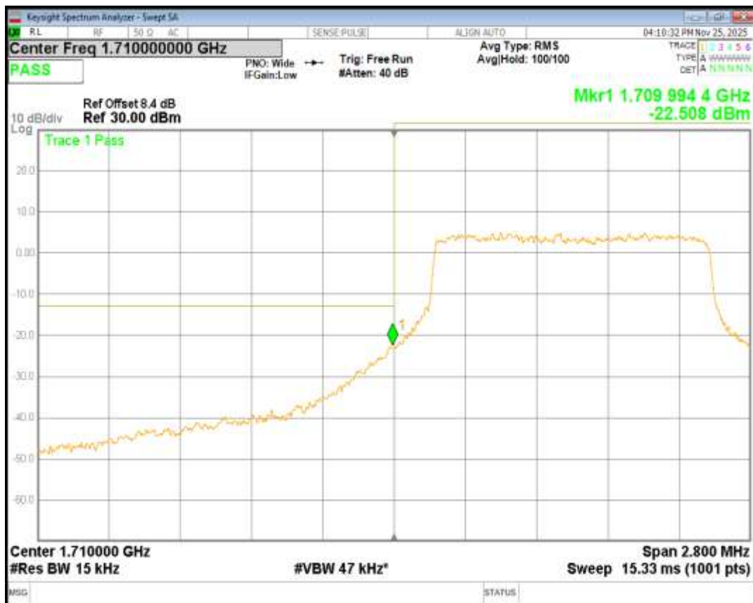
Band4 QPSK BW=1.4MHz Channel=20393 RB Size=6 Position=#0
