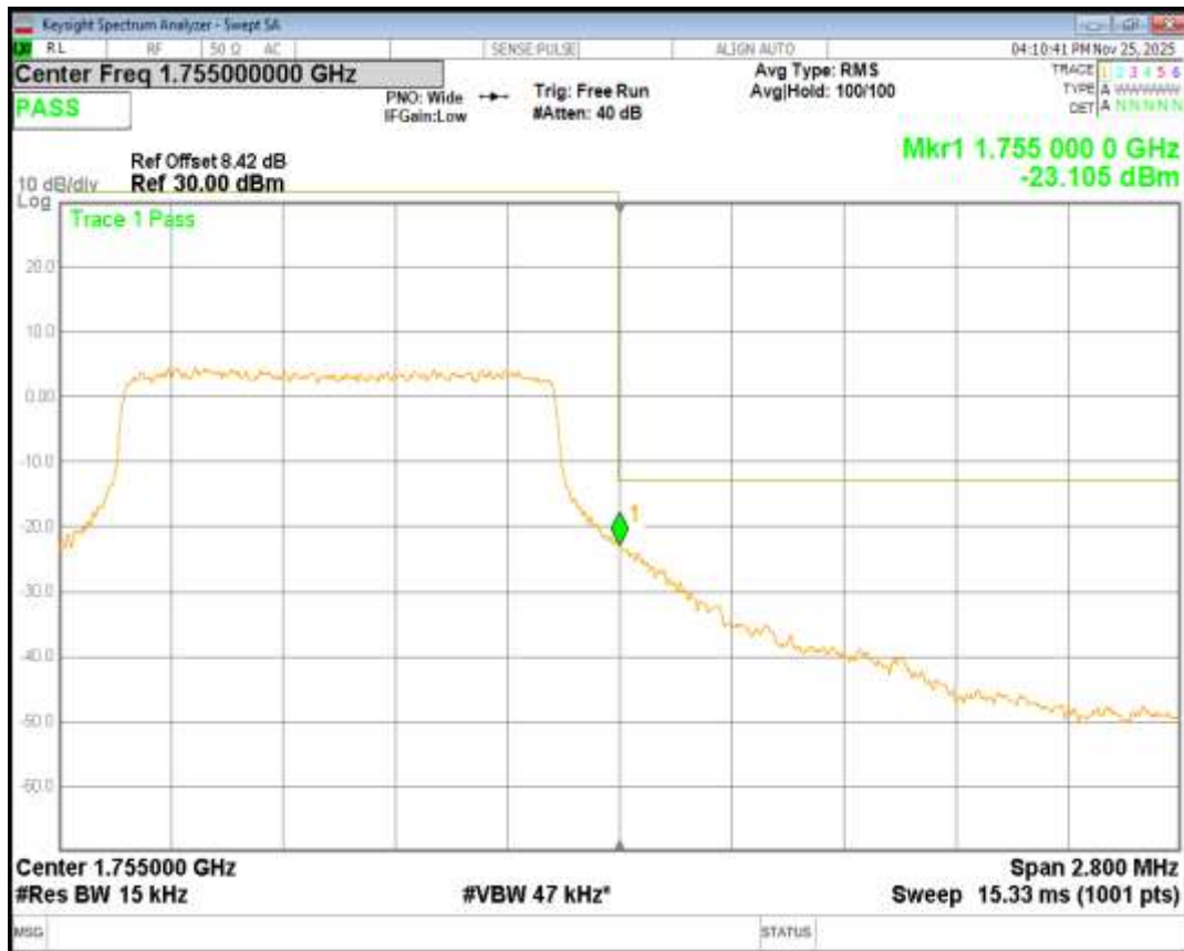
Band4 QPSK BW=3MHz Channel=19965 RB Size=15 Position=#0
