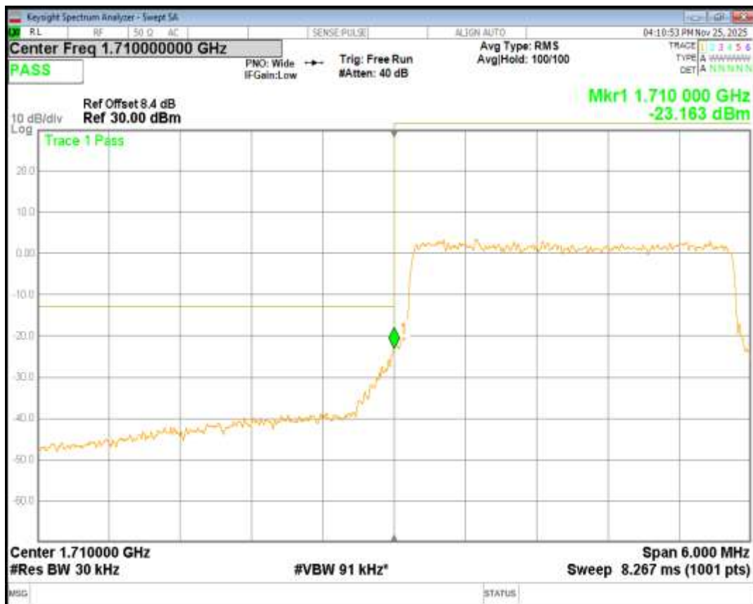
Band4 16QAM BW=3MHz Channel=20385 RB Size=15 Position=#0
