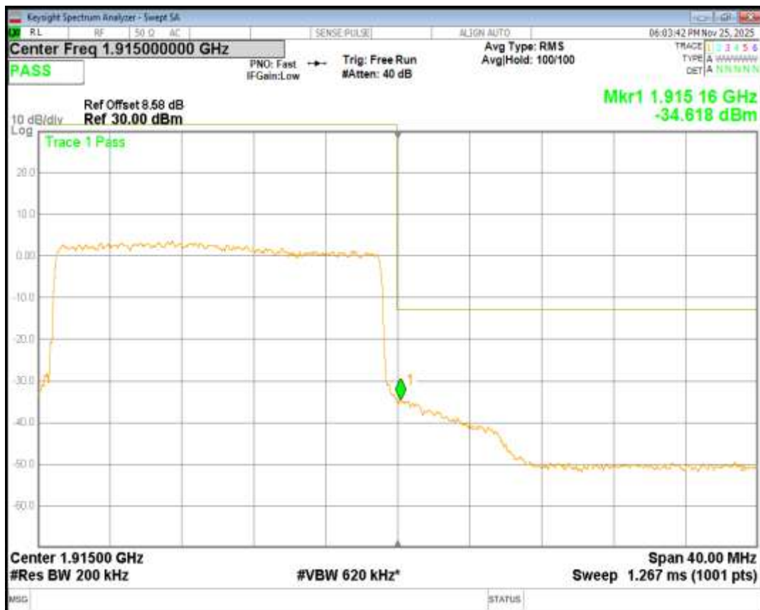
Band26(814-824) 16QAM BW=1.4MHz Channel=26697 RB Size=6 Position=#0
