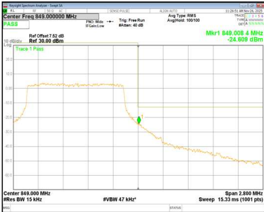
Band26(824-849) 16QAM BW=3MHz Channel=26805 RB Size=15 Position=#0
