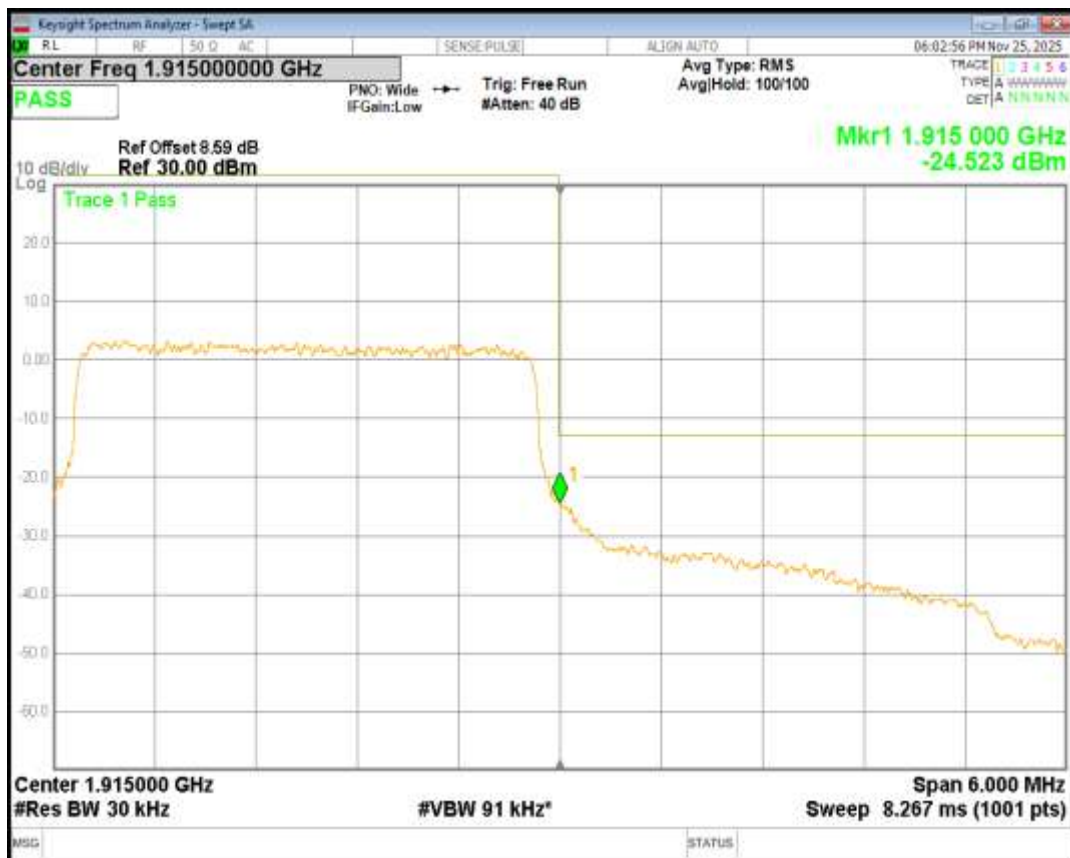
Band25 QPSK BW=5MHz Channel=26065 RB Size=25 Position=#0
