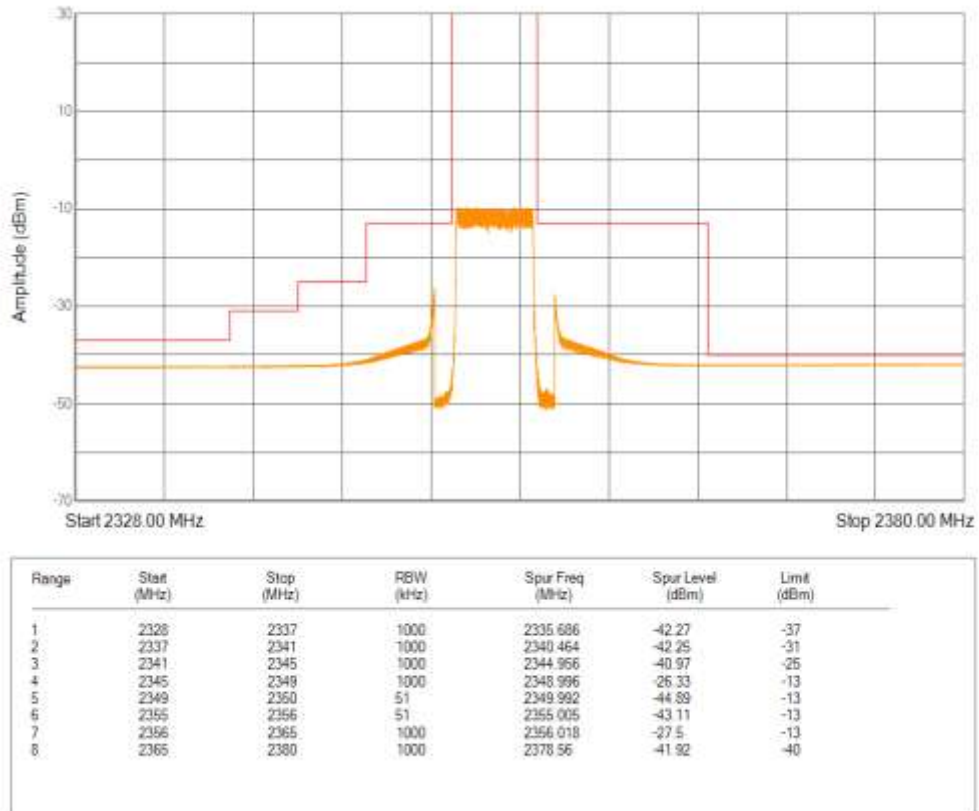
Band40(2350-2360) 16QAM BW=5MHz Channel=39225 RB Size=25 Position=#0
