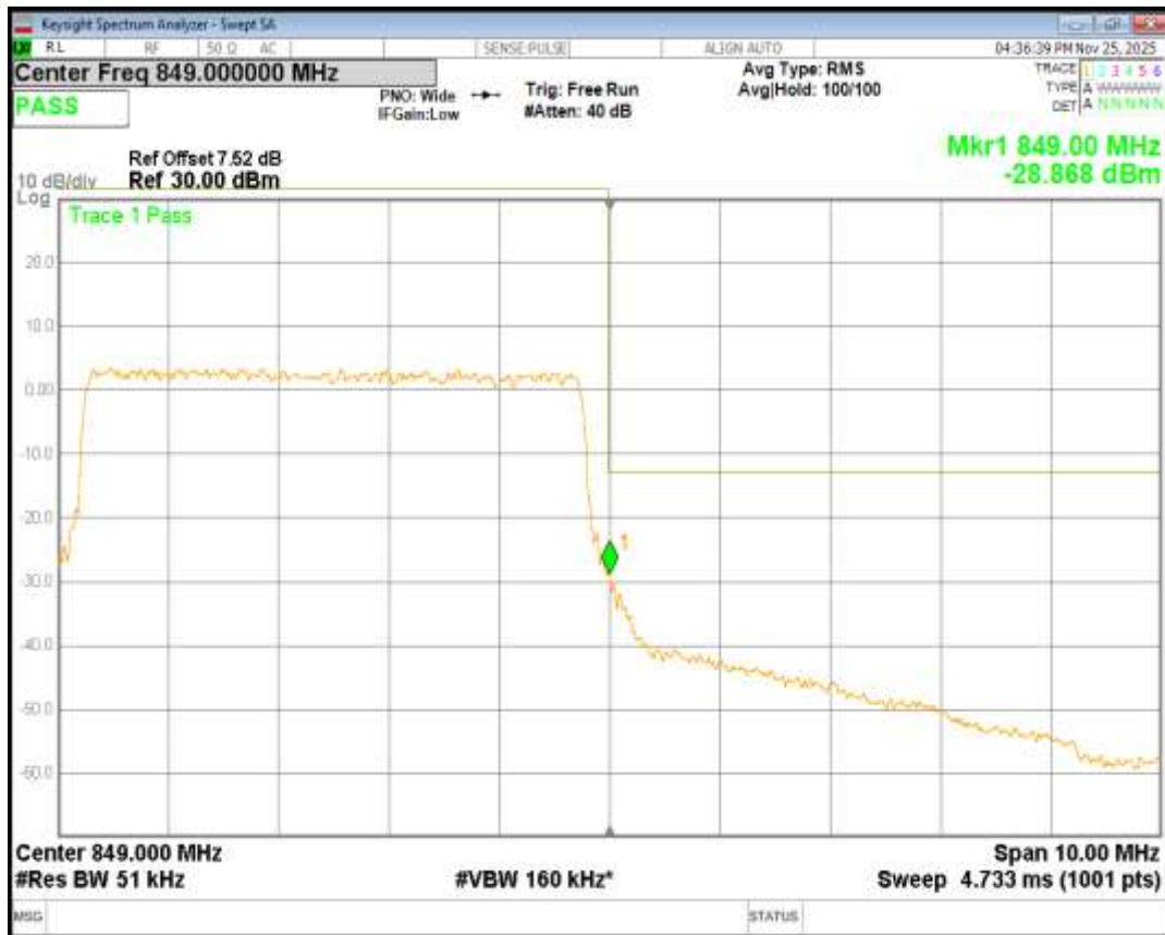
Band5 QPSK BW=10MHz Channel=20450 RB Size=50 Position=#0
