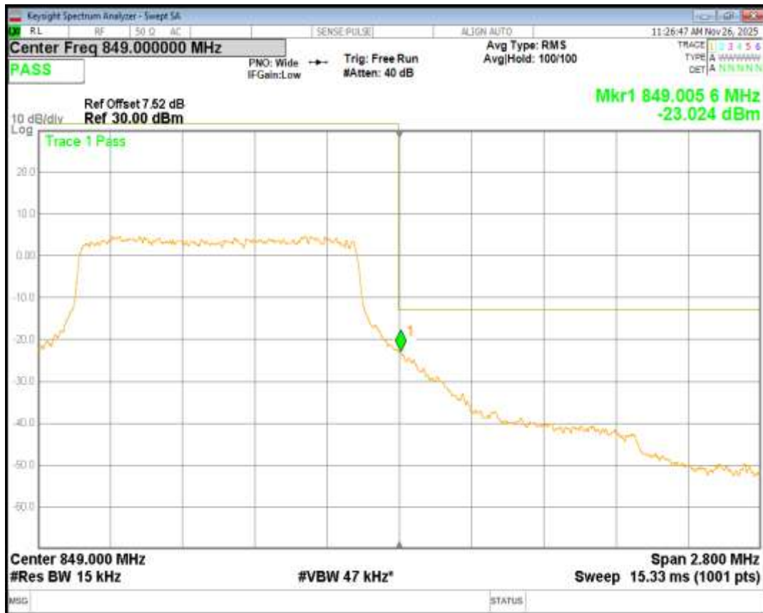
Band26(824-849) QPSK BW=3MHz Channel=26805 RB Size=15 Position=#0
