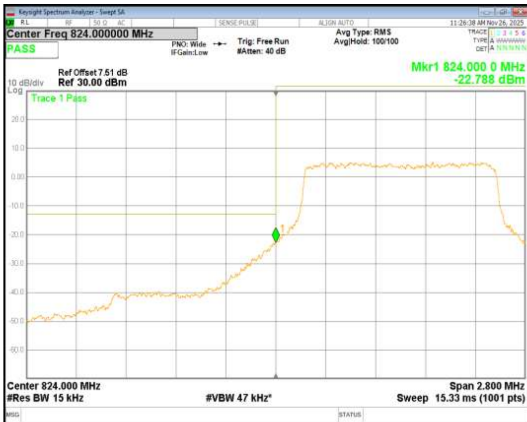
Band26(824-849) QPSK BW=1.4MHz Channel=27033 RB Size=6 Position=#0
