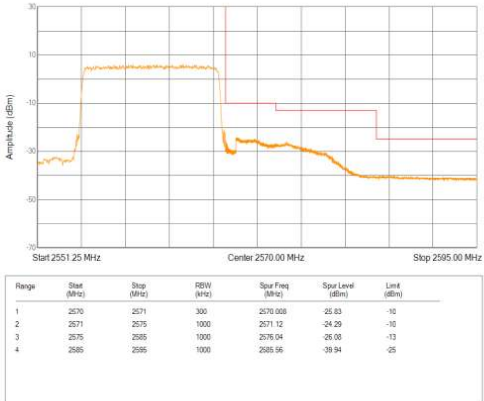
Band7 QPSK BW=20MHz Channel=20850 RB Size=100 Position=#0
