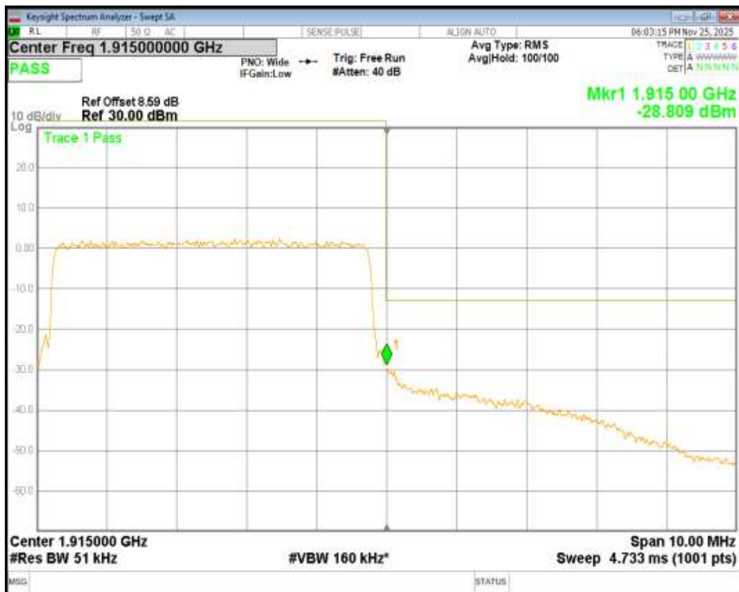
Band25 QPSK BW=1.4MHz Channel=26047 RB Size=6 Position=#0
