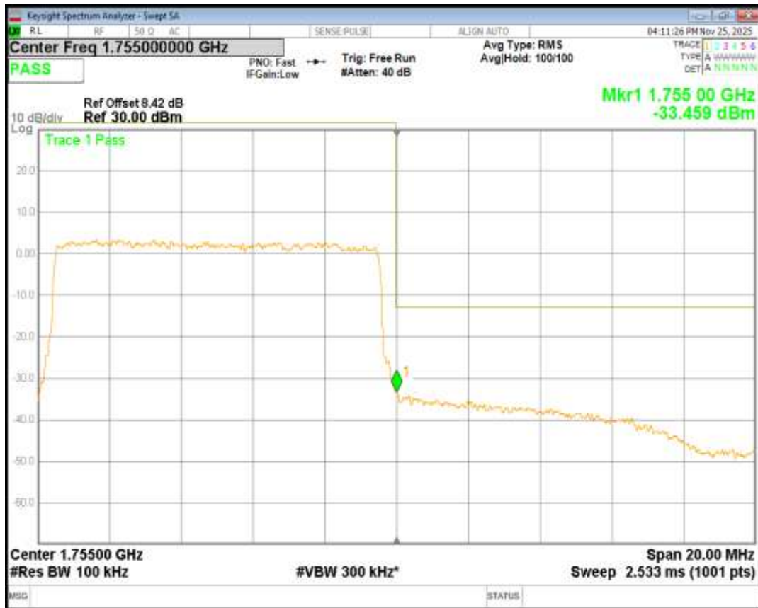
Band4 QPSK BW=15MHz Channel=20025 RB Size=75 Position=#0
