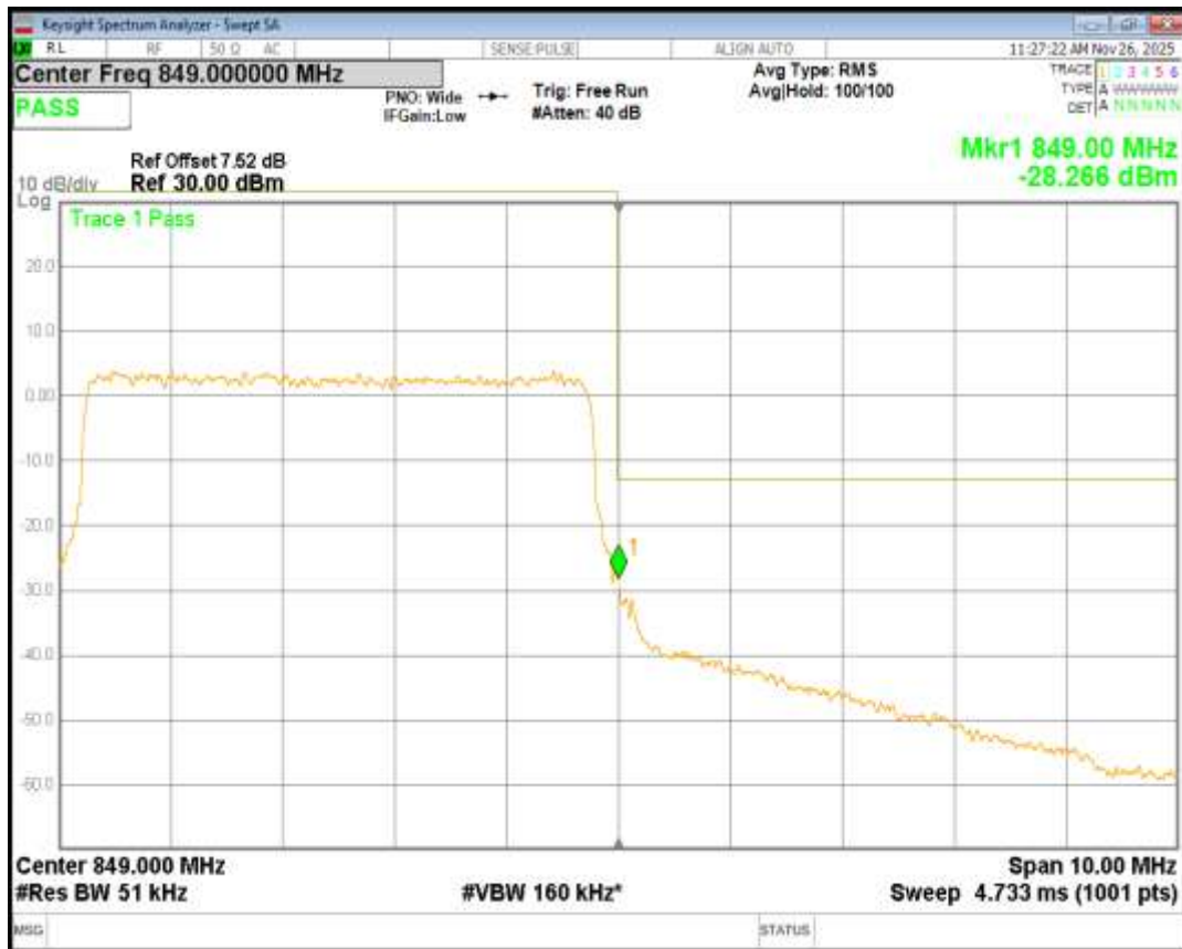
Band26(824-849) QPSK BW=10MHz Channel=26840 RB Size=50 Position=#0
