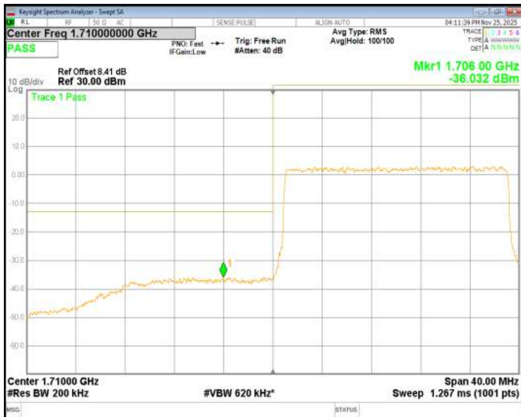
Band4 QPSK BW=20MHz Channel=20300 RB Size=100 Position=#0
