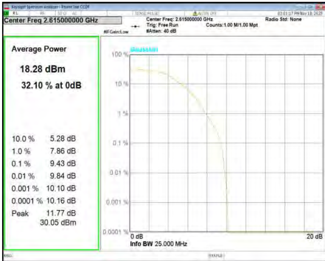
Band38 QPSK BW=15MHz Channel=37825 RB Size=1 Position=#0
