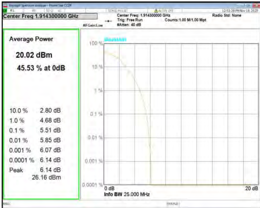
Band25 16QAM BW=3MHz Channel=26055 RB Size=1 Position=#0
