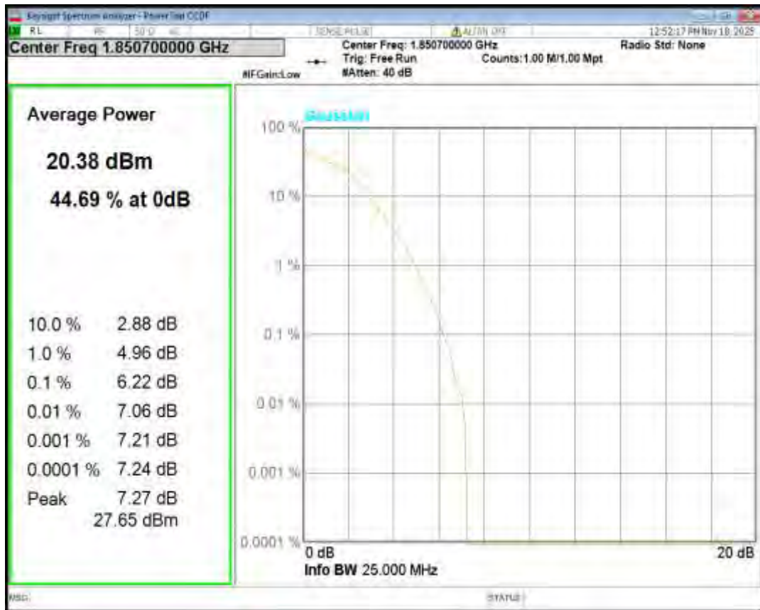
Band25 16QAM BW=1.4MHz Channel=26365 RB Size=1 Position=#0
