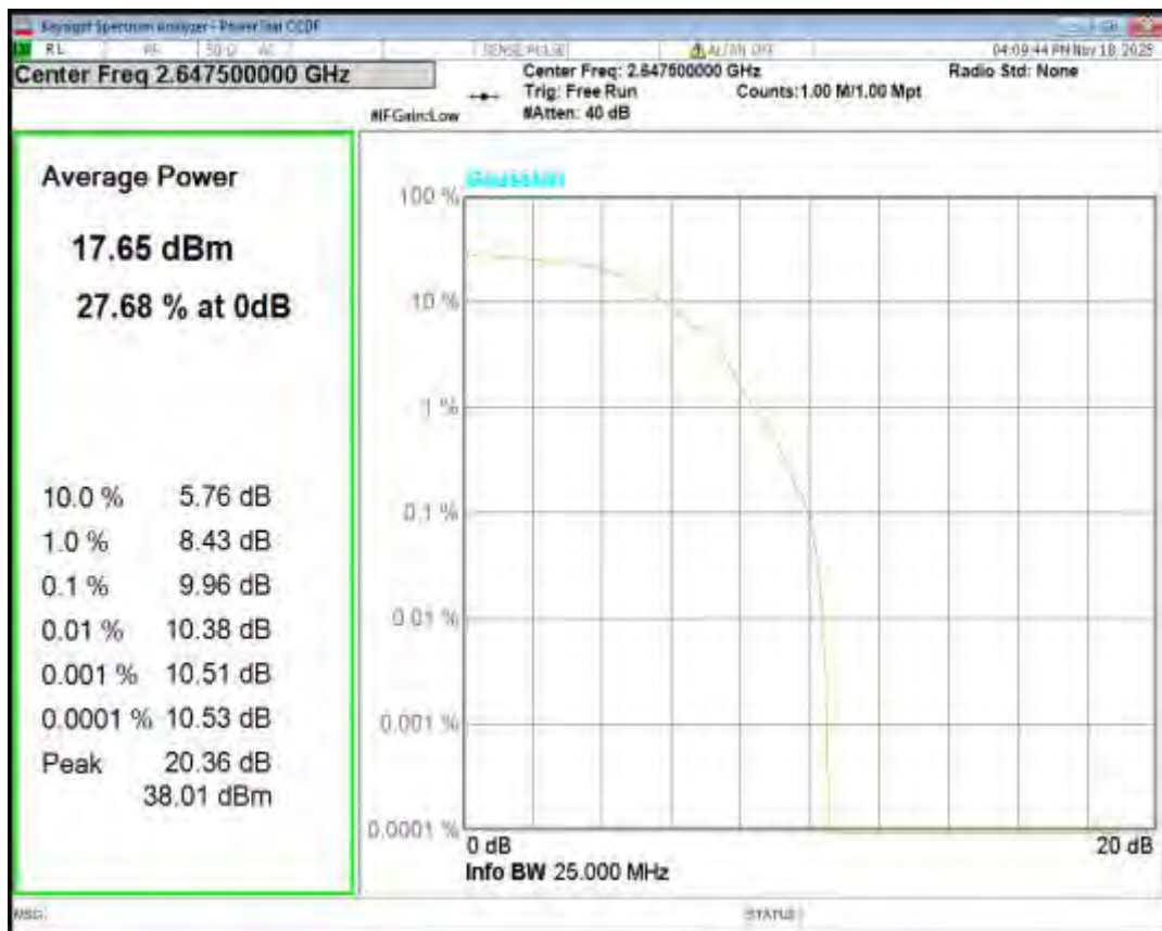
Band41(2555-2655) QPSK BW=20MHz Channel=40340 RB Size=1 Position=#0
