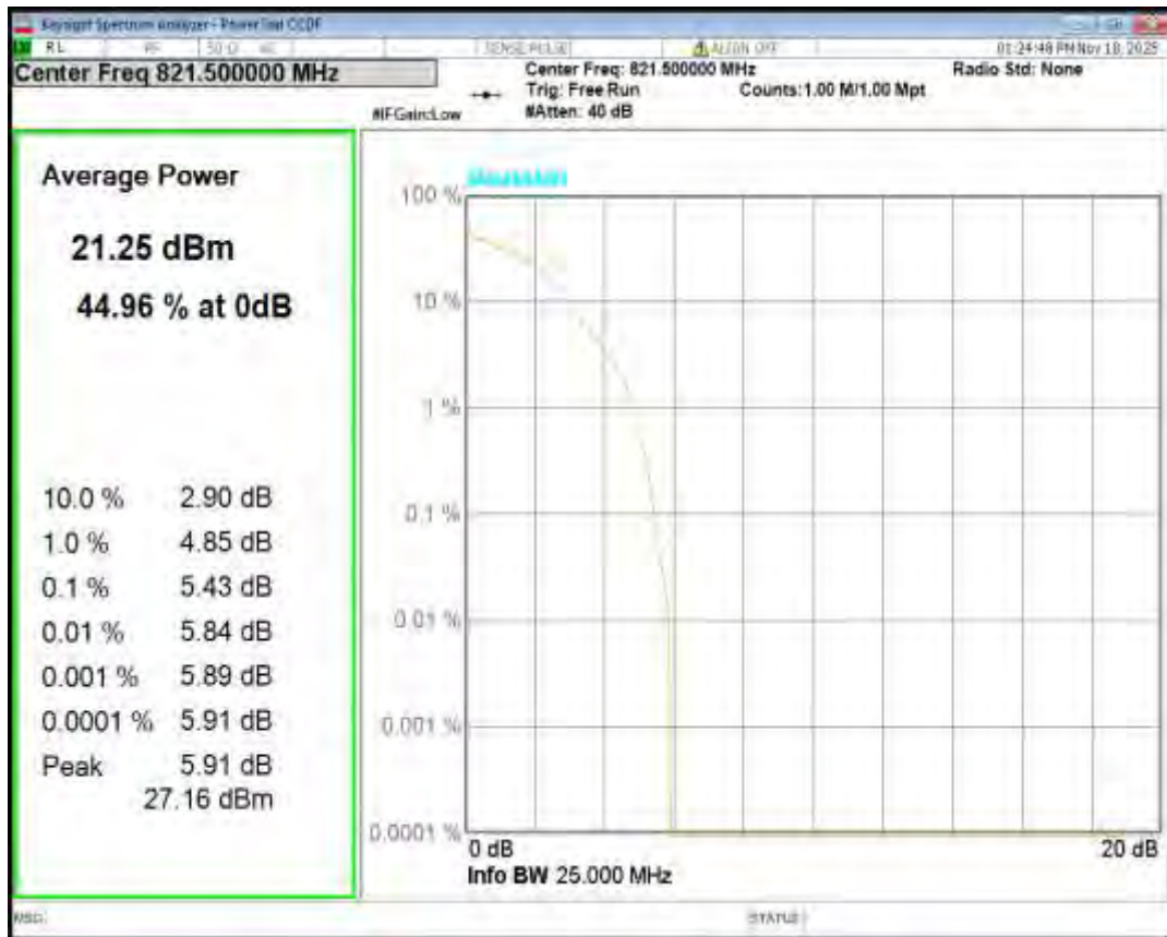
Band26(814-824) 16QAM BW=5MHz Channel=26715 RB Size=1 Position=#0
