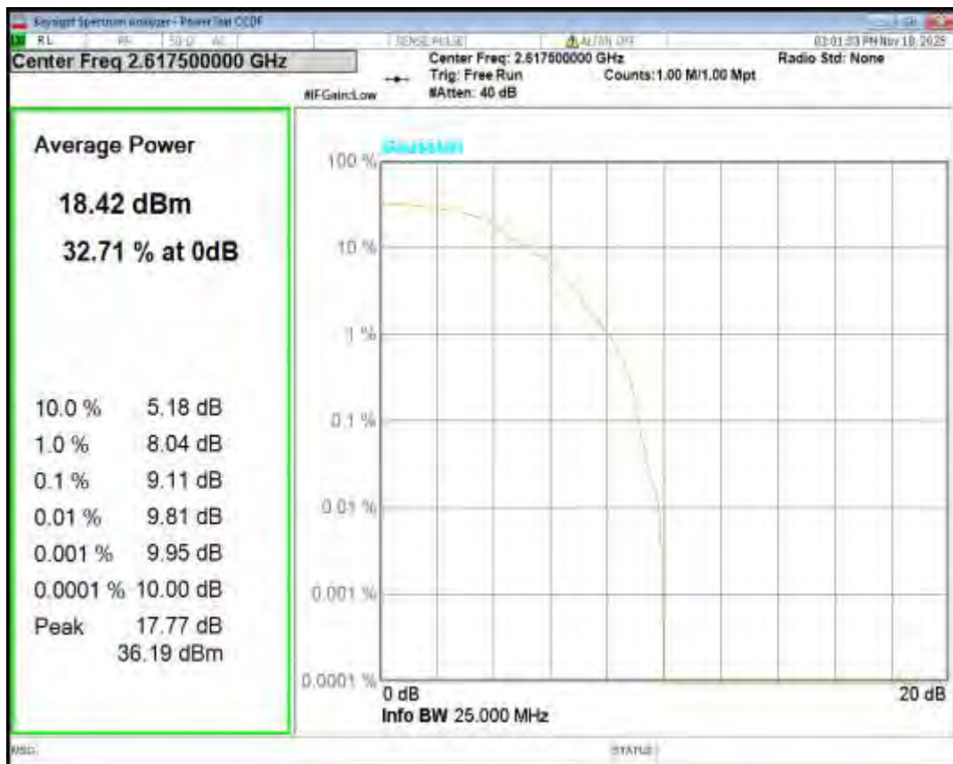
Band38 QPSK BW=10MHz Channel=37800 RB Size=1 Position=#0
