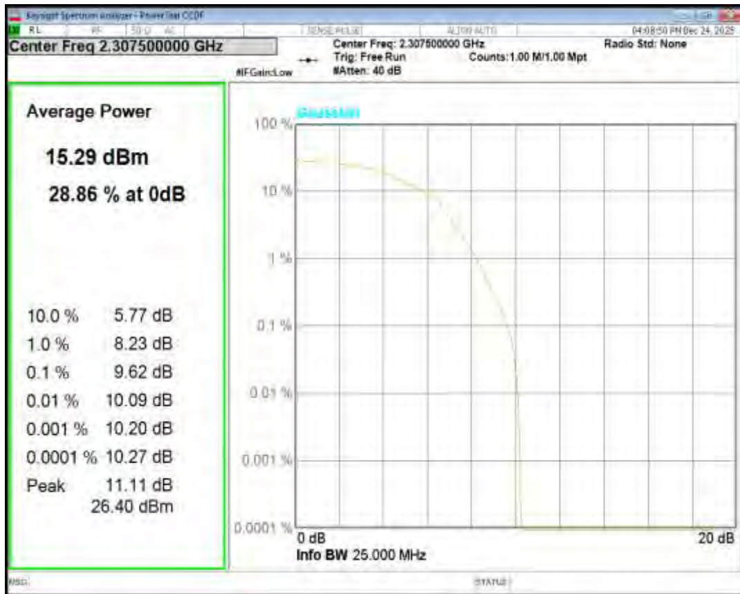
Band40(2305-2315) 16QAM BW=5MHz Channel=38750 RB Size=1 Position=#0
