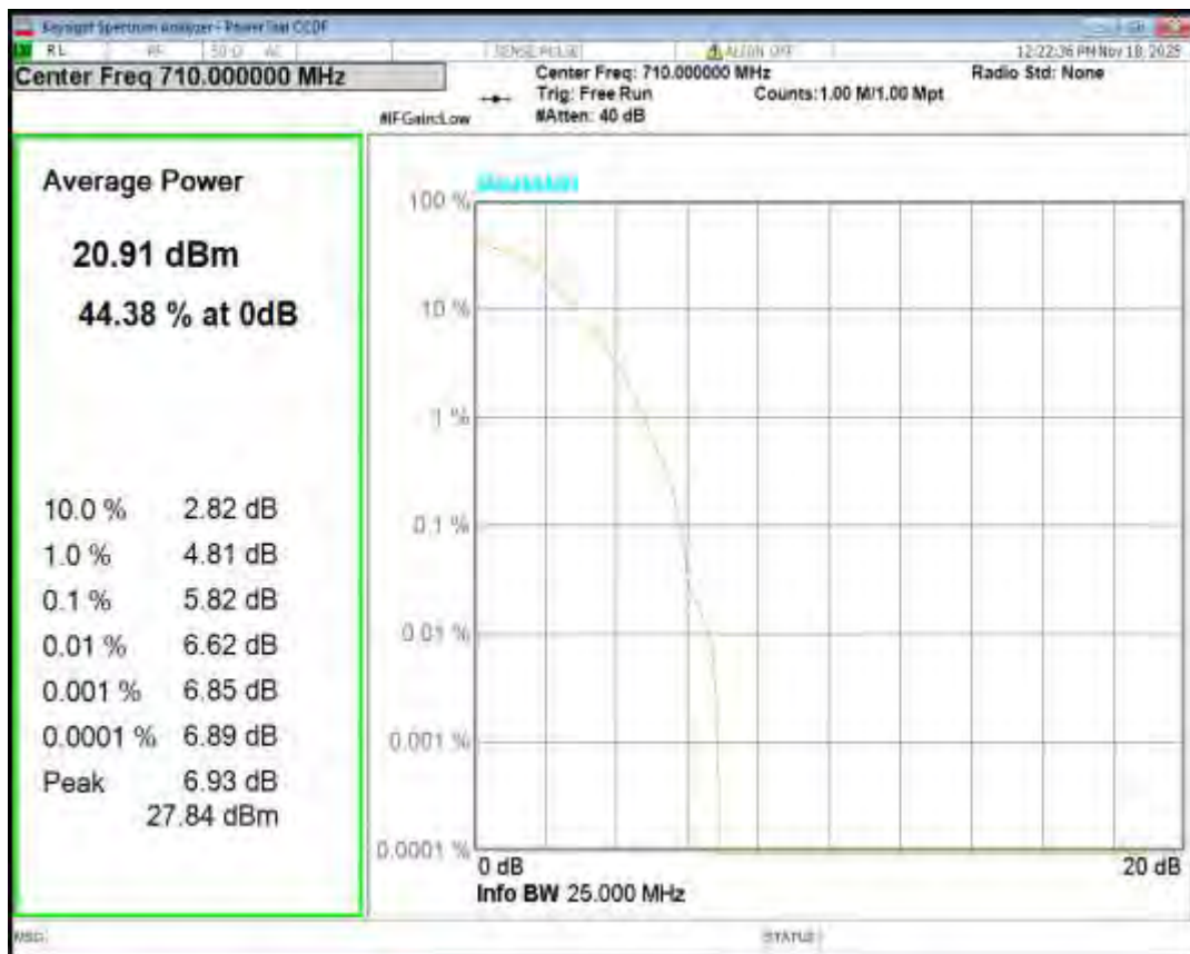
Band17 16QAM BW=5MHz Channel=23825 RB Size=1 Position=#0
