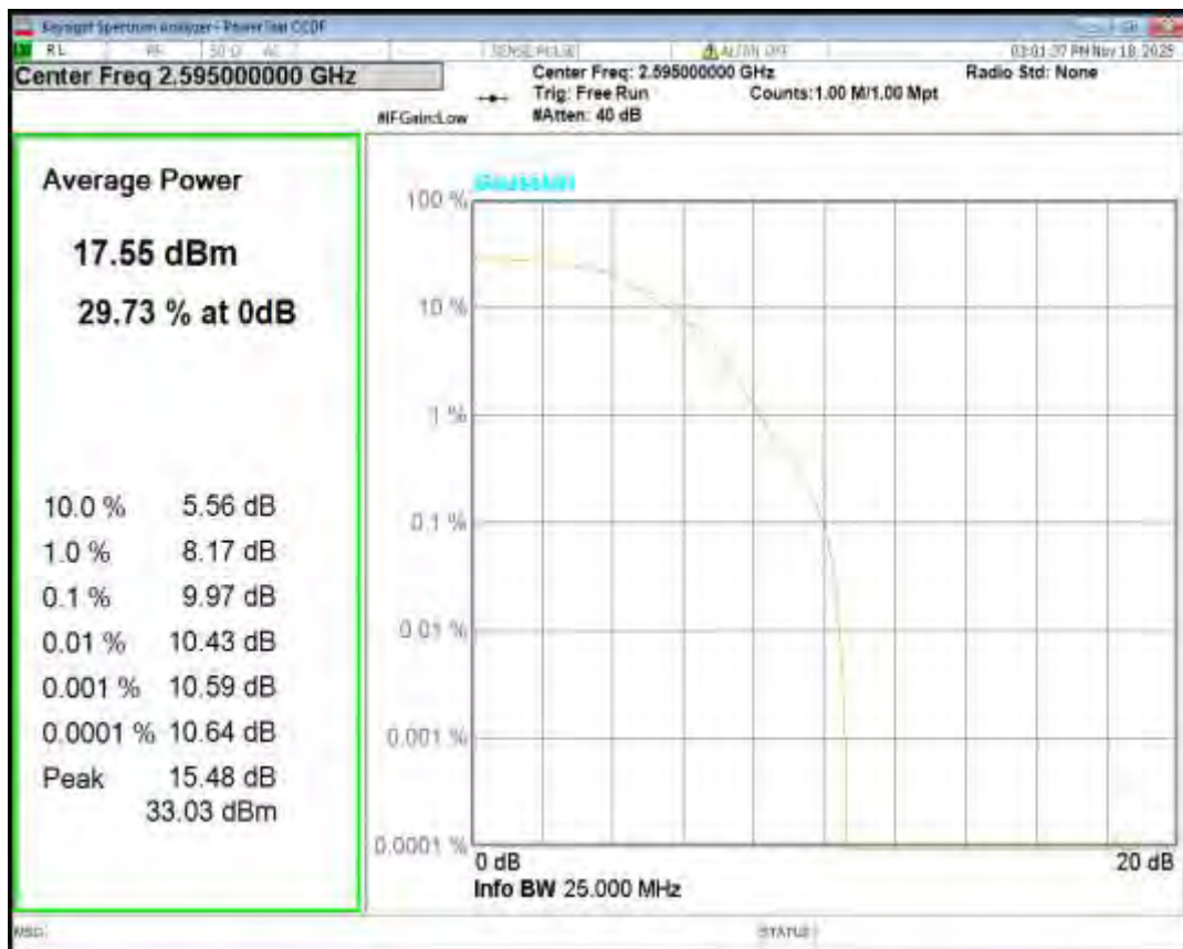
Band38 QPSK BW=20MHz Channel=38150 RB Size=1 Position=#0
