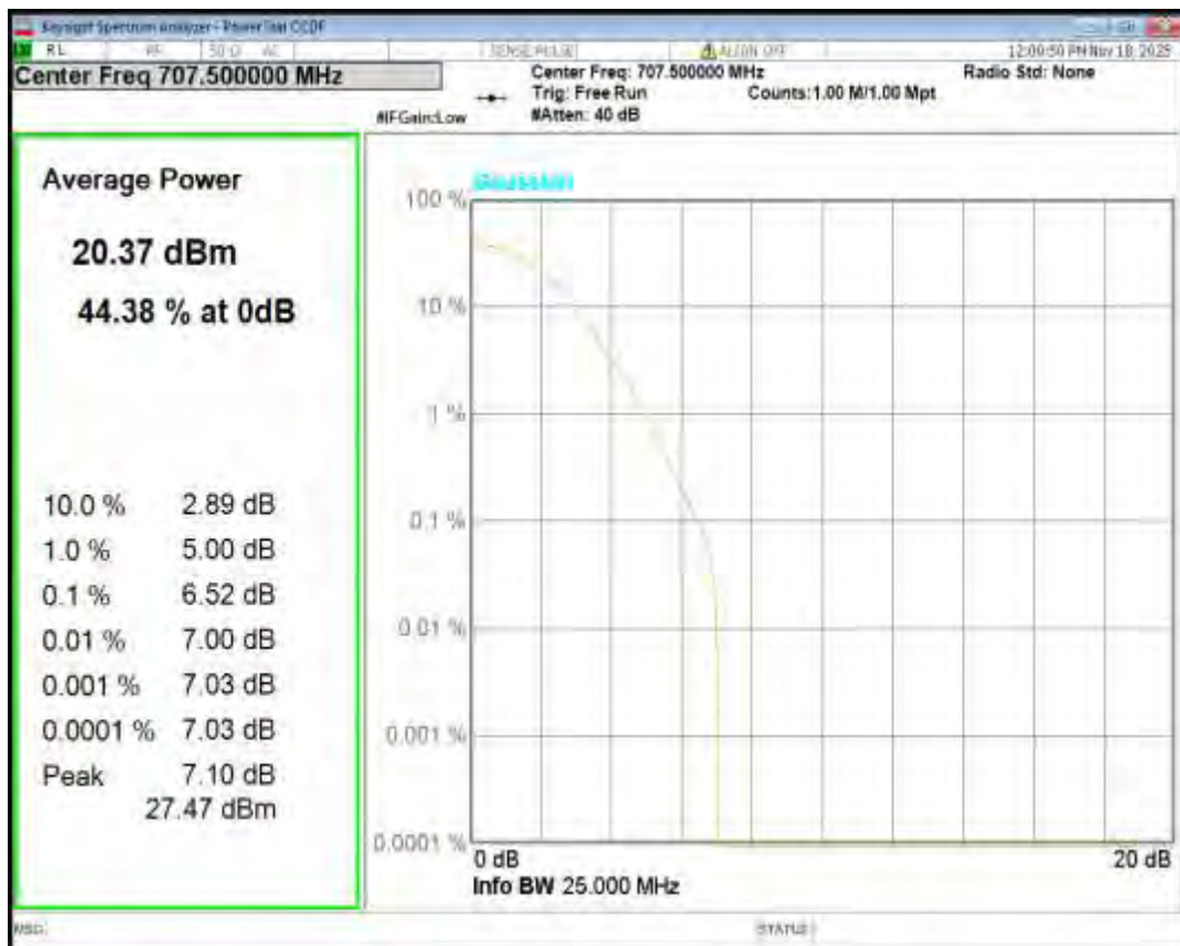
Band12 16QAM BW=3MHz Channel=23165 RB Size=1 Position=#0
