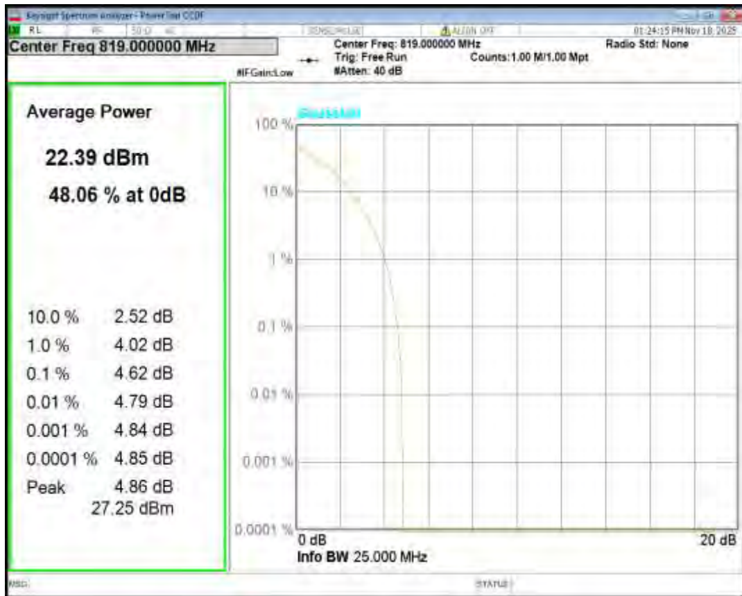
Band26(814-824) QPSK BW=3MHz Channel=26775 RB Size=1 Position=#0
