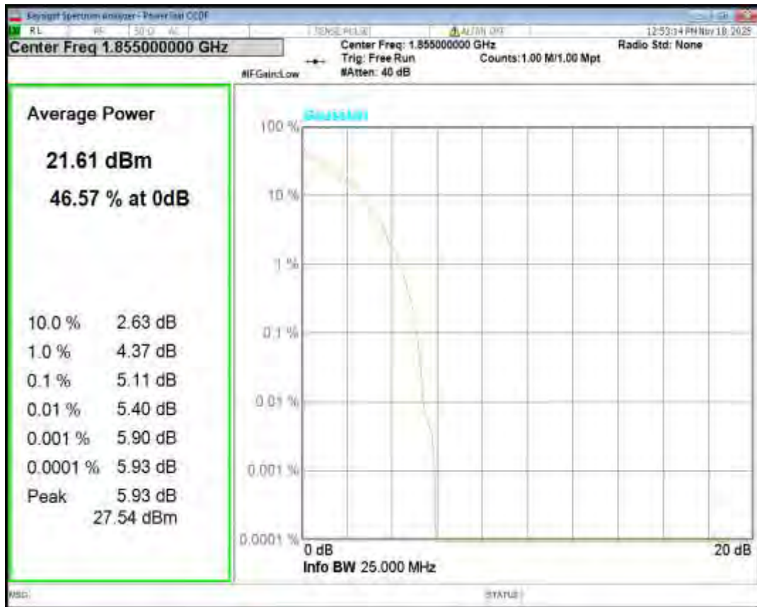
Band25 QPSK BW=10MHz Channel=26365 RB Size=1 Position=#0
