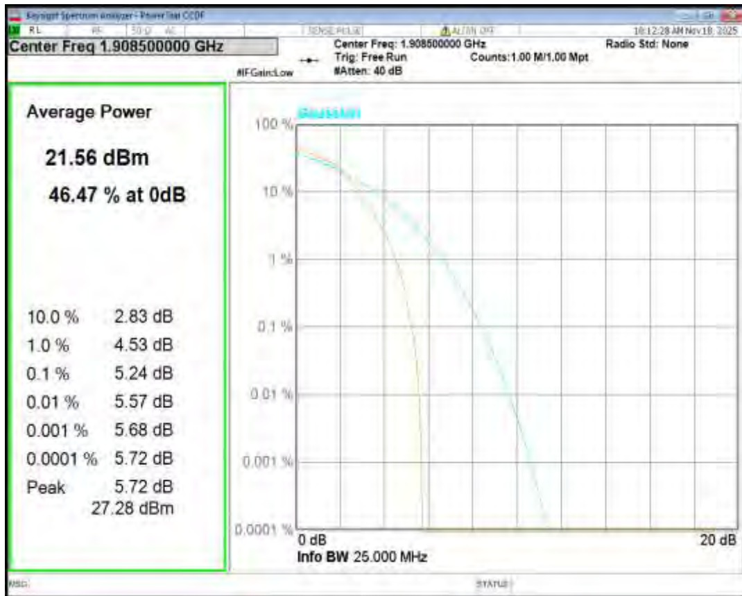
Band2 16QAM BW=5MHz Channel=18625 RB Size=1 Position=#0
