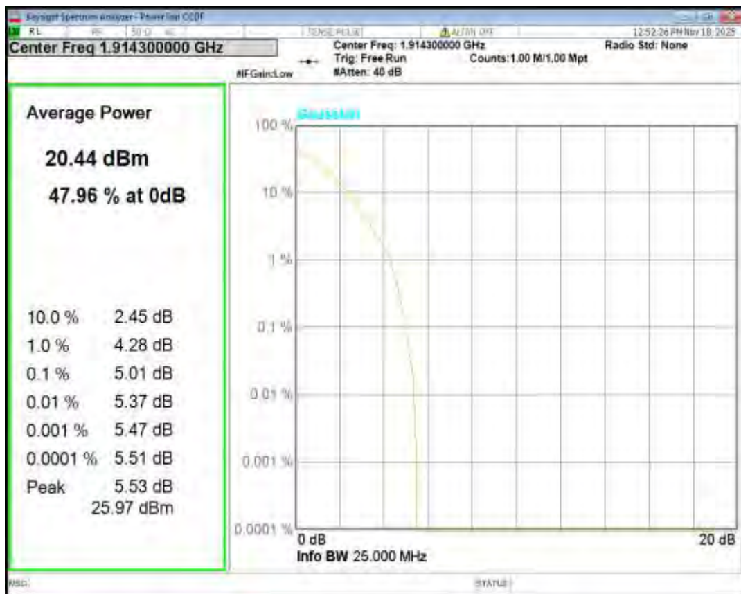
Band25 QPSK BW=3MHz Channel=26055 RB Size=1 Position=#0
