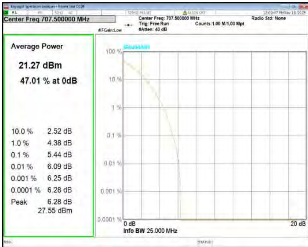
Band12 QPSK BW=3MHz Channel=23165 RB Size=1 Position=#0
