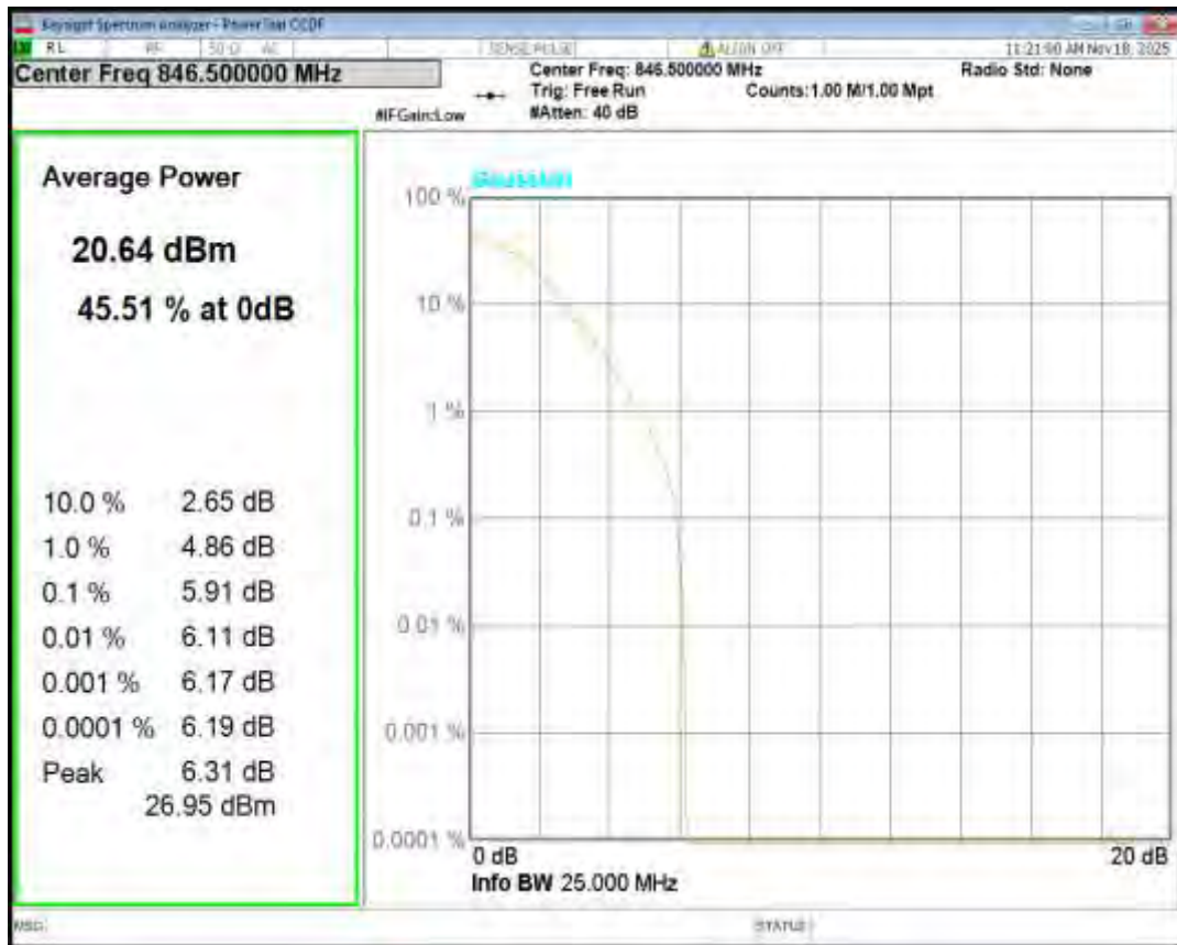
Band5 QPSK BW=1.4MHz Channel=20525 RB Size=1 Position=#0
