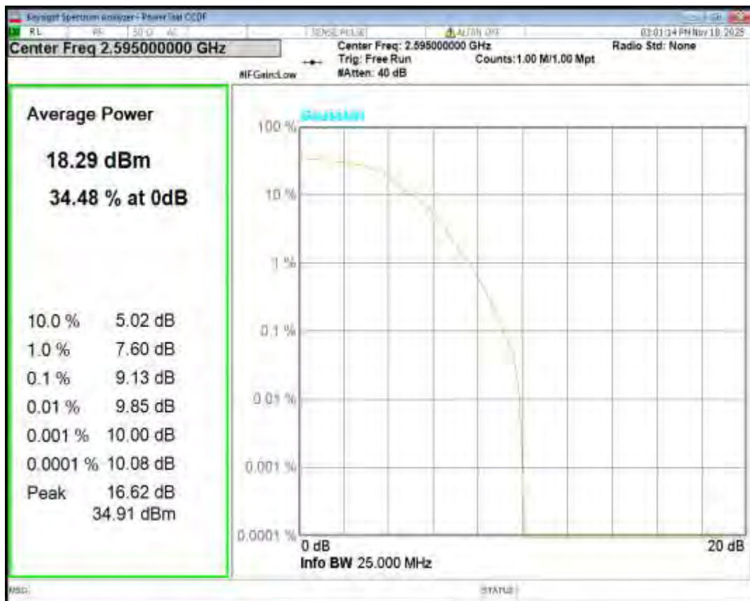
Band38 QPSK BW=10MHz Channel=38200 RB Size=1 Position=#0
