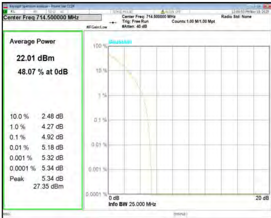
Band12 QPSK BW=5MHz Channel=23095 RB Size=1 Position=#0
