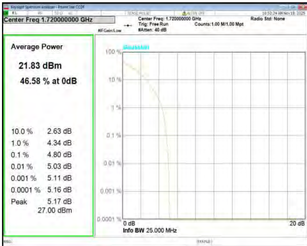
Band4 QPSK BW=20MHz Channel=20175 RB Size=1 Position=#0
