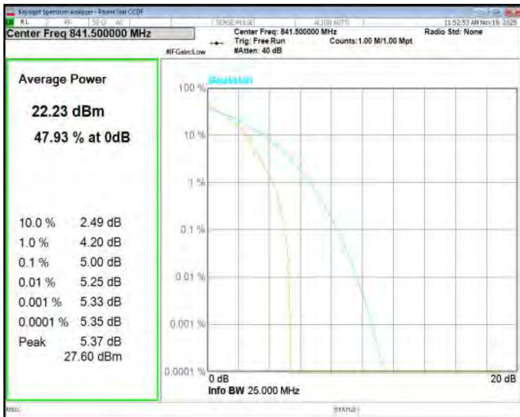
Band38 16QAM BW=5MHz Channel=37775 RB Size=1 Position=#0
