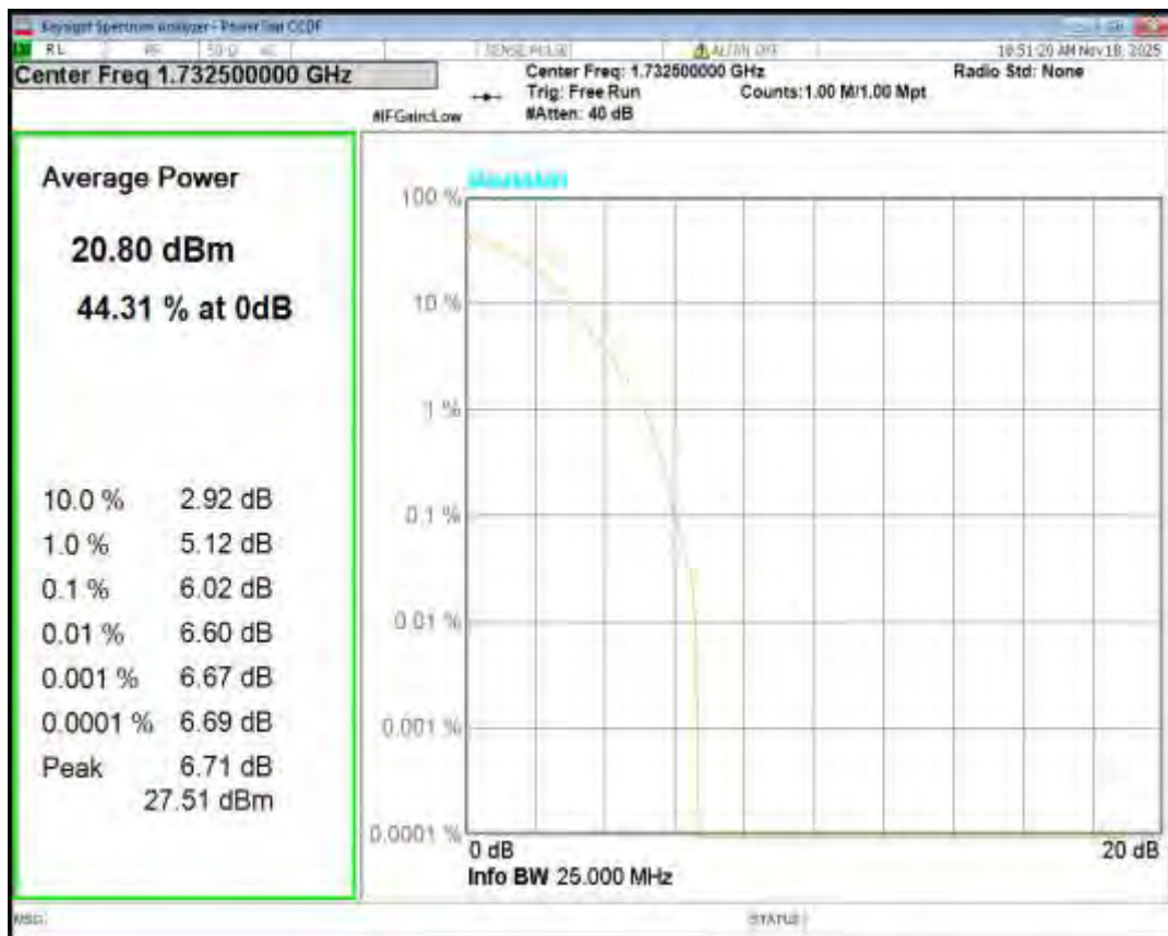
Band4 16QAM BW=3MHz Channel=20385 RB Size=1 Position=#0
