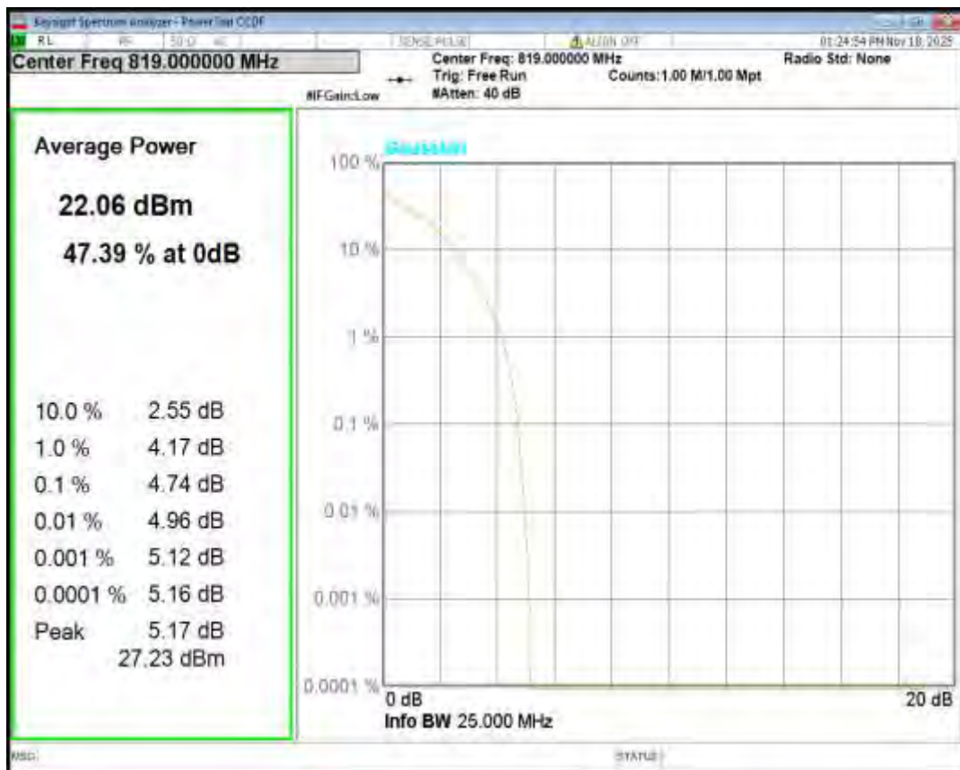
Band26(824-849) 16QAM BW=1.4MHz Channel=26797 RB Size=1 Position=#0
