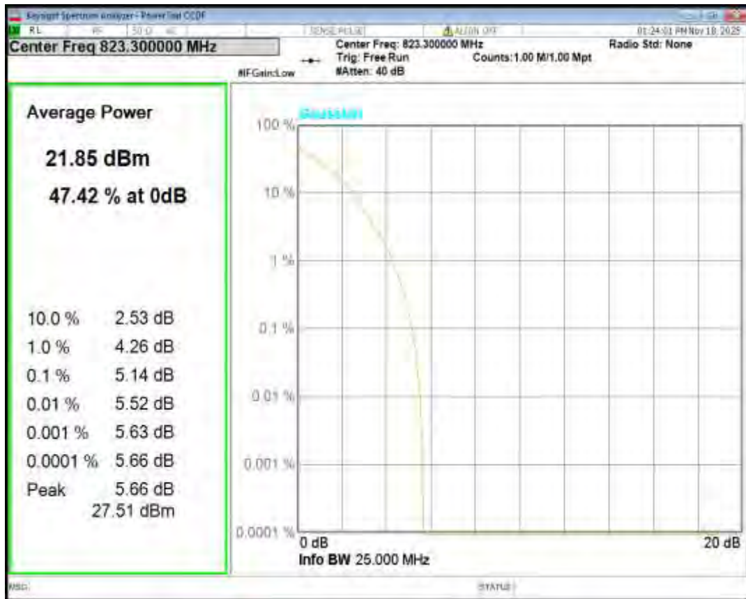
Band26(814-824) QPSK BW=3MHz Channel=26705 RB Size=1 Position=#0
