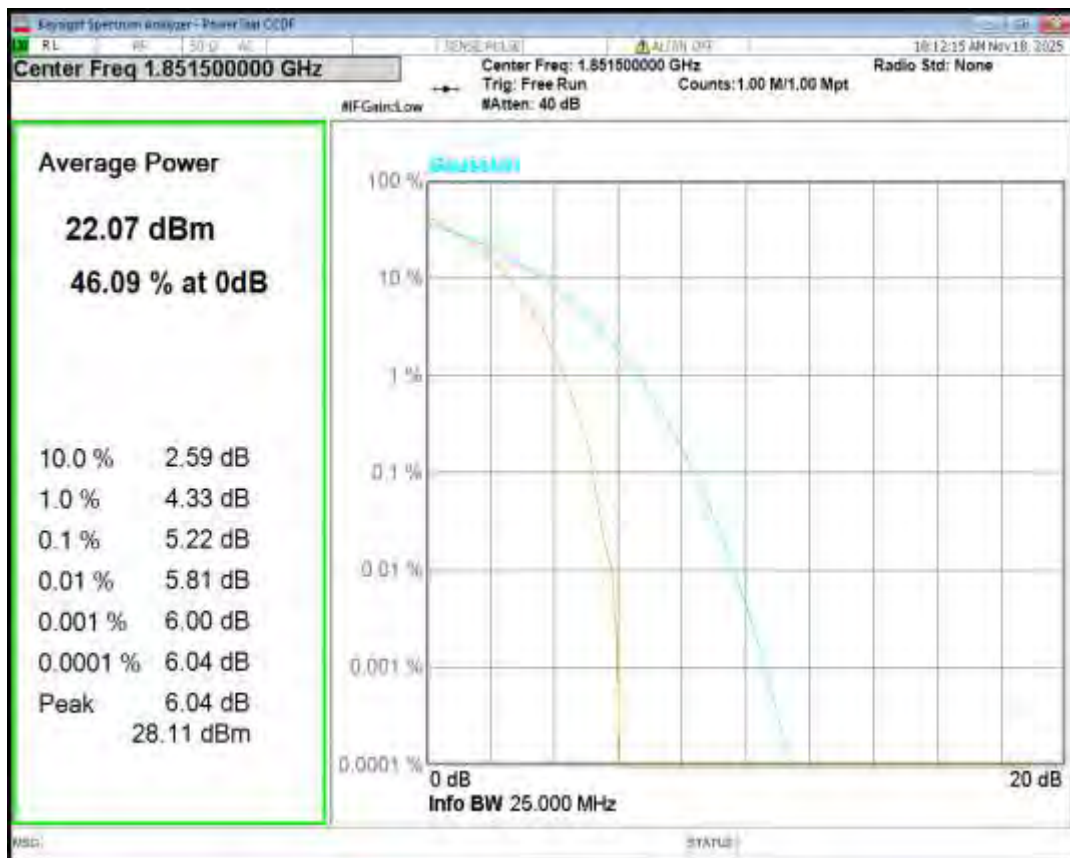
Band2 QPSK BW=3MHz Channel=18900 RB Size=1 Position=#0
