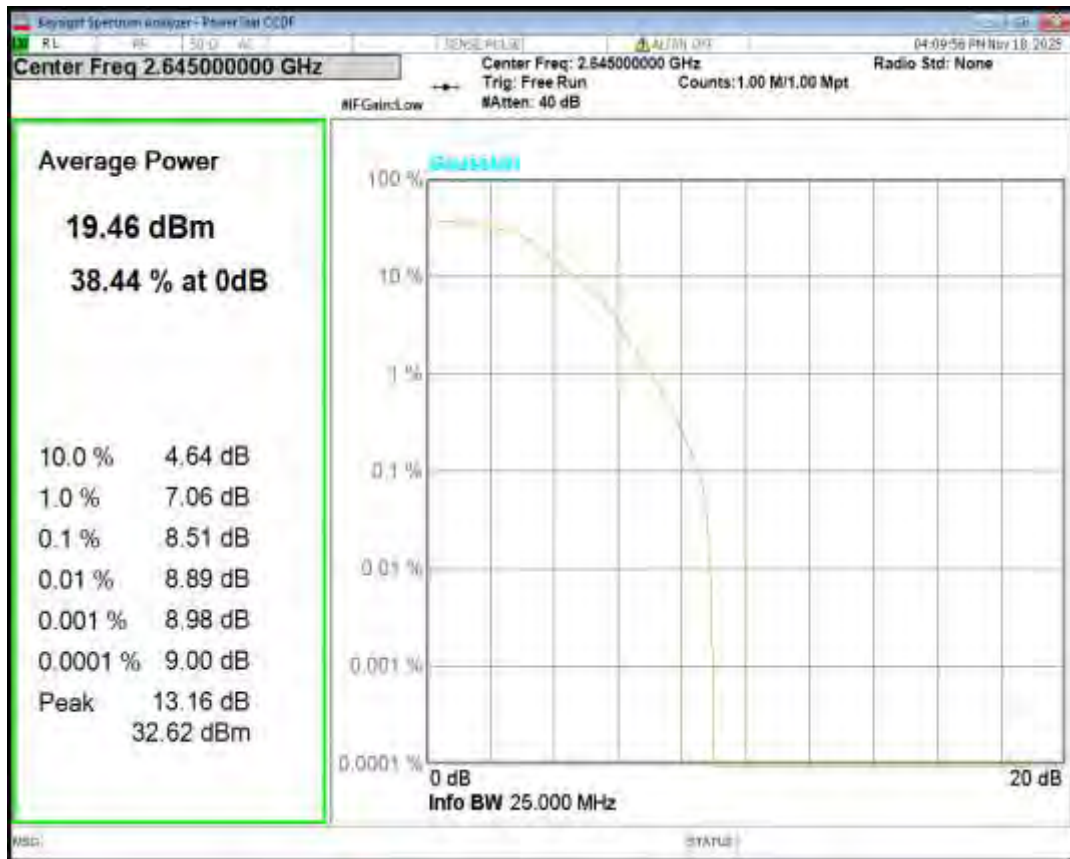
Band5 16QAM BW=1.4MHz Channel=20407 RB Size=1 Position=#0
