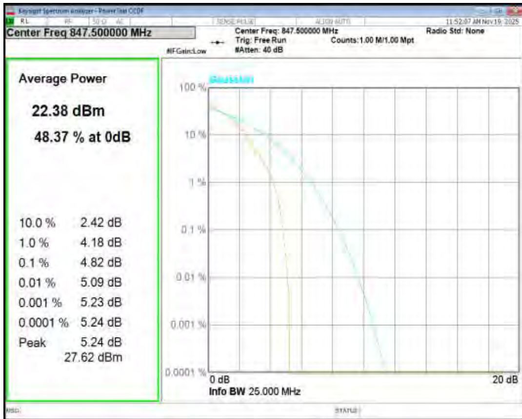
Band26(824-849) QPSK BW=5MHz Channel=26815 RB Size=1 Position=#0
