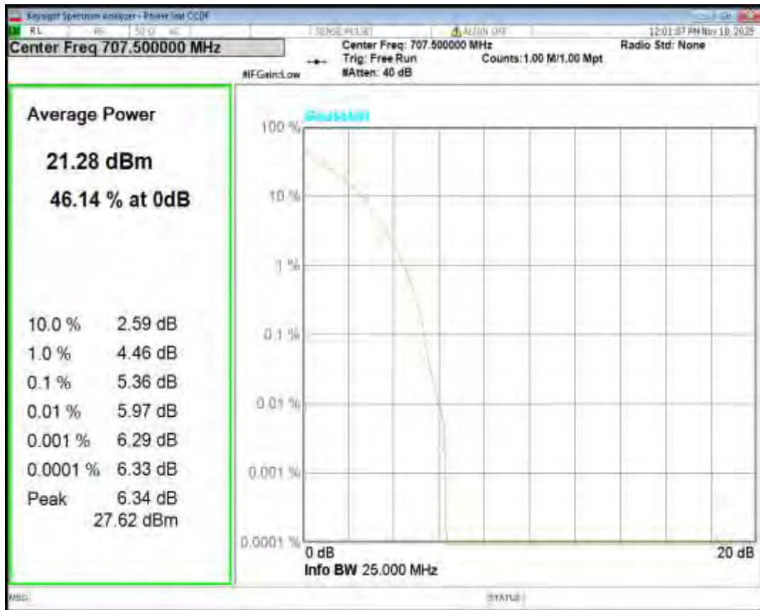
Band12 QPSK BW=5MHz Channel=23035 RB Size=1 Position=#0
