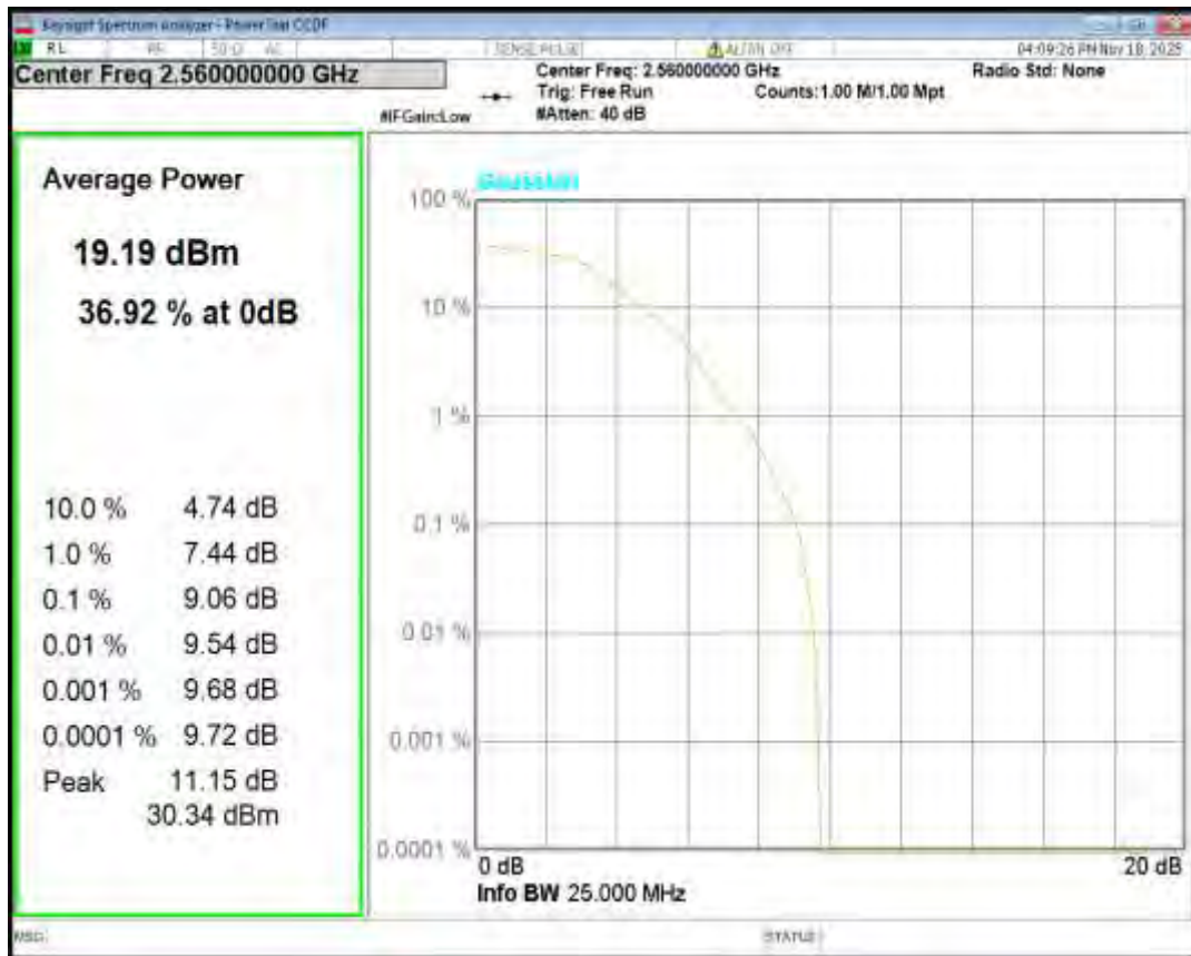
Band41(2555-2655) QPSK BW=10MHz Channel=40740 RB Size=1 Position=#0
