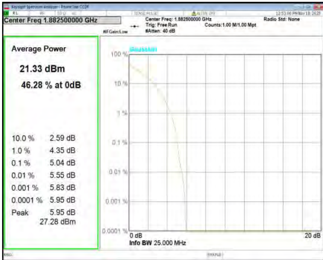
Band25 QPSK BW=5MHz Channel=26665 RB Size=1 Position=#0
