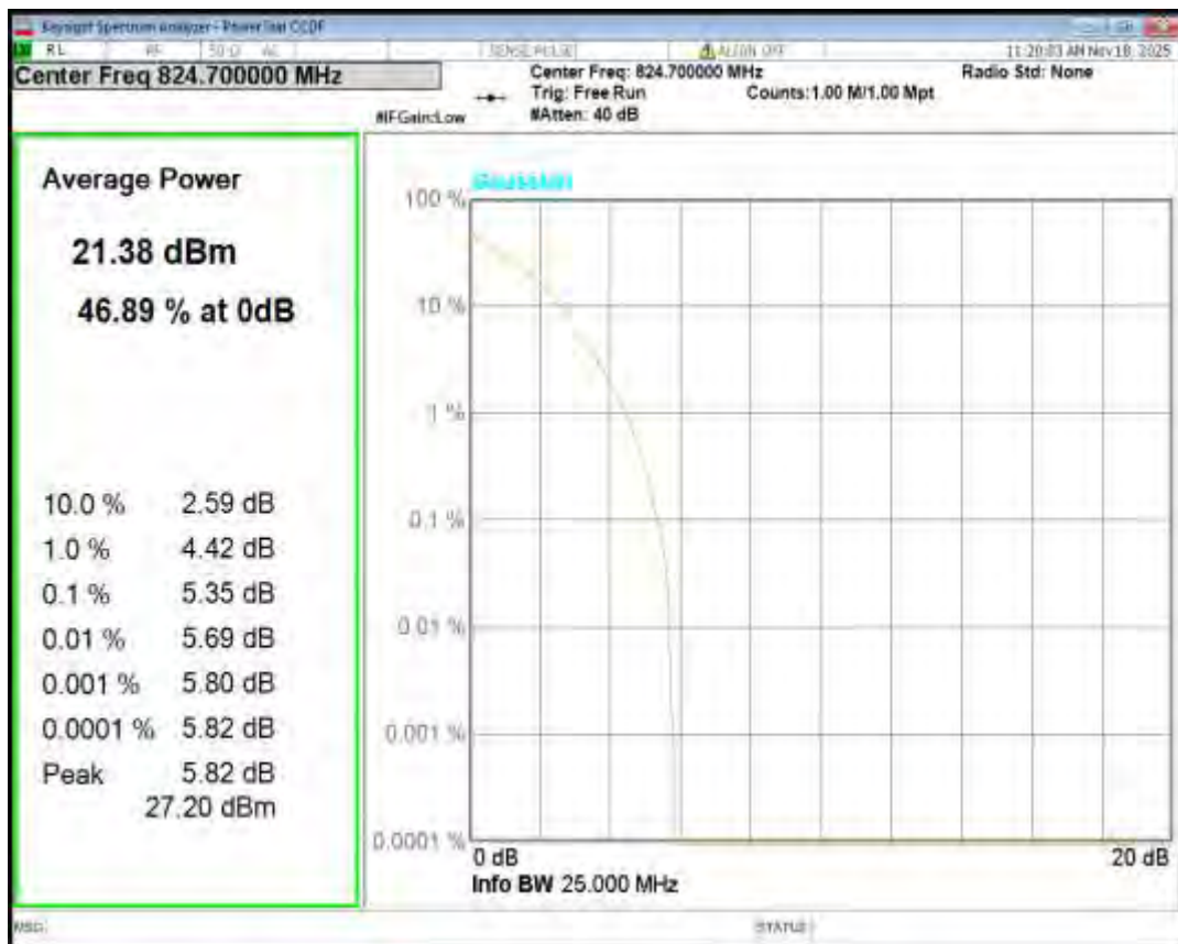
Band5 16QAM BW=5MHz Channel=20625 RB Size=1 Position=#0
