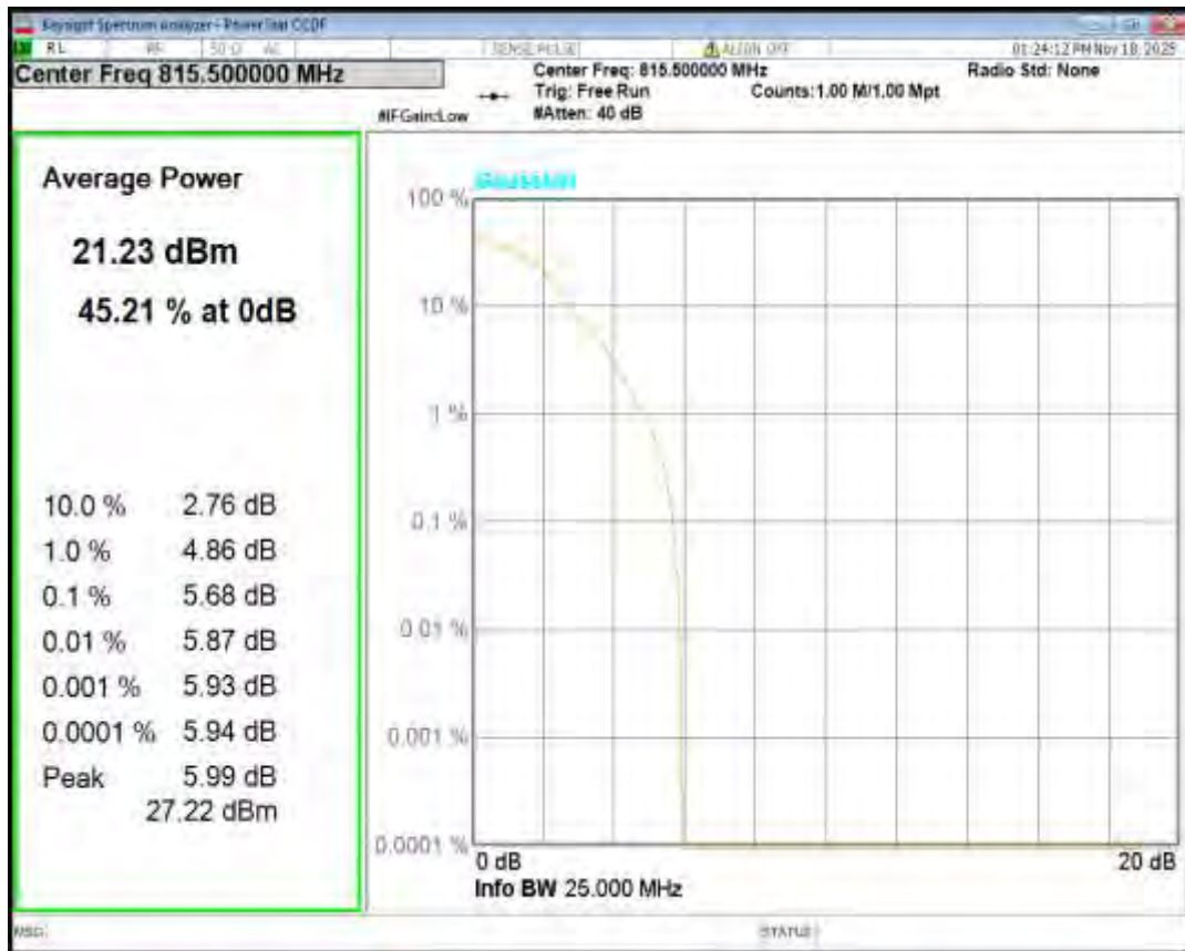
Band26(814-824) 16QAM BW=3MHz Channel=26740 RB Size=1 Position=#0
