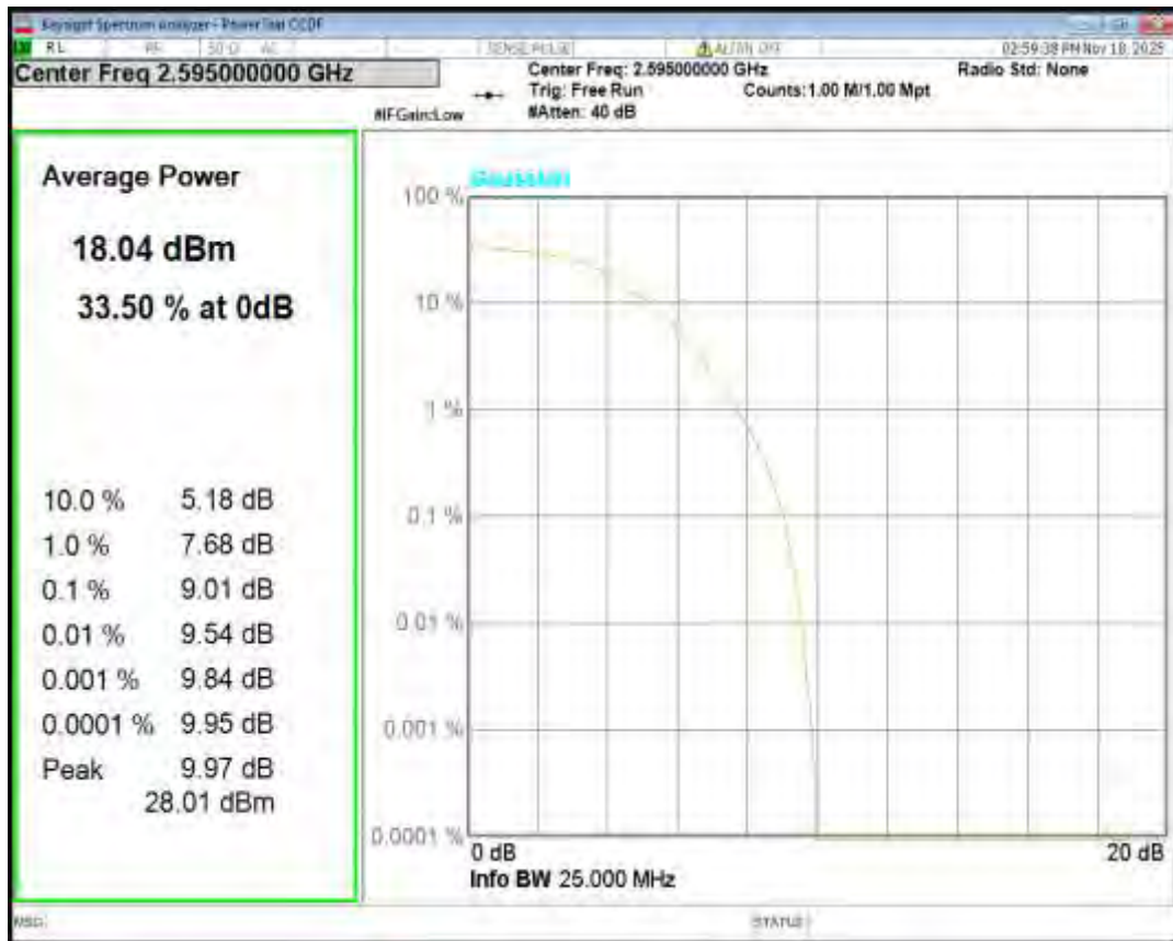
Band38 QPSK BW=5MHz Channel=38225 RB Size=1 Position=#0
