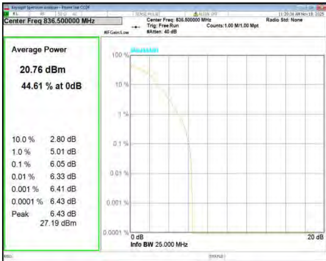
Band5 16QAM BW=3MHz Channel=20635 RB Size=1 Position=#0
