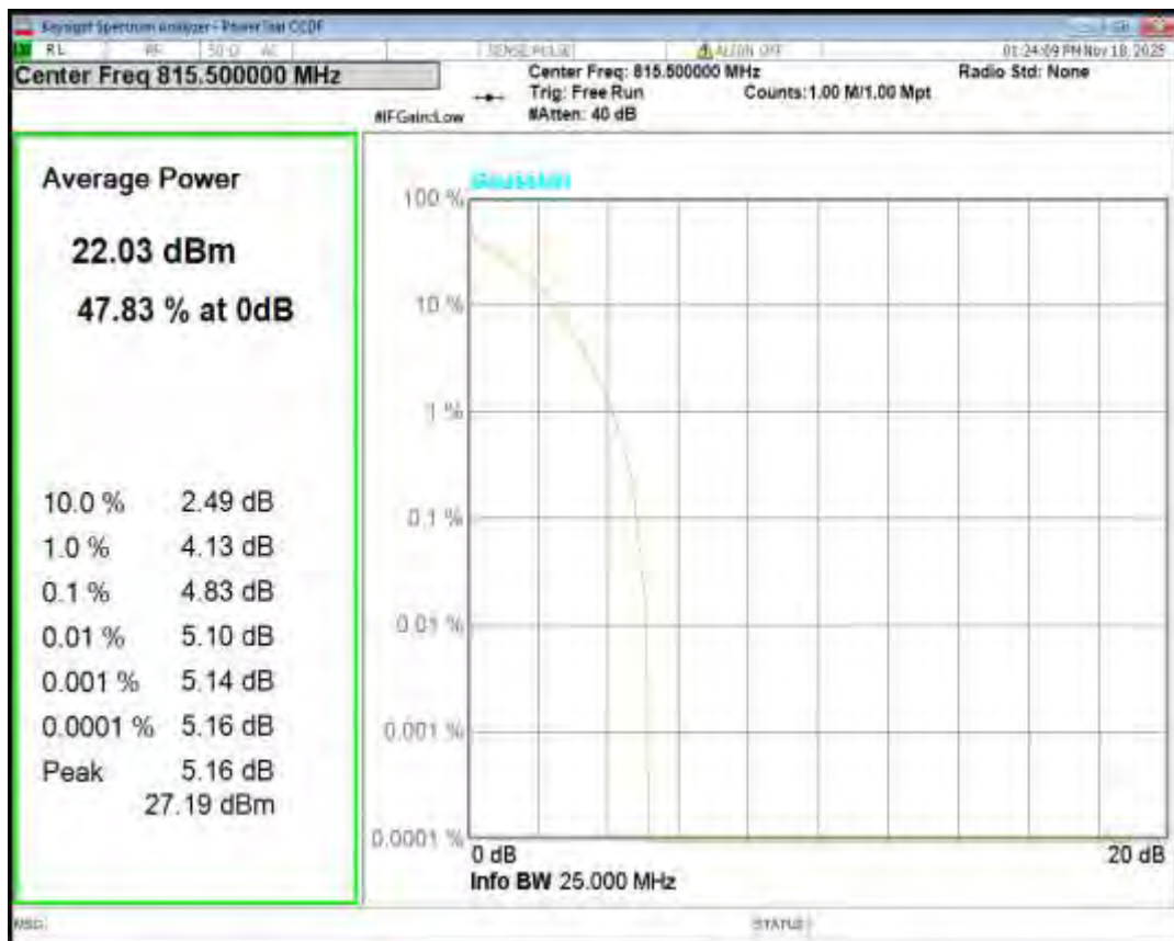
Band26(814-824) QPSK BW=3MHz Channel=26740 RB Size=1 Position=#0
