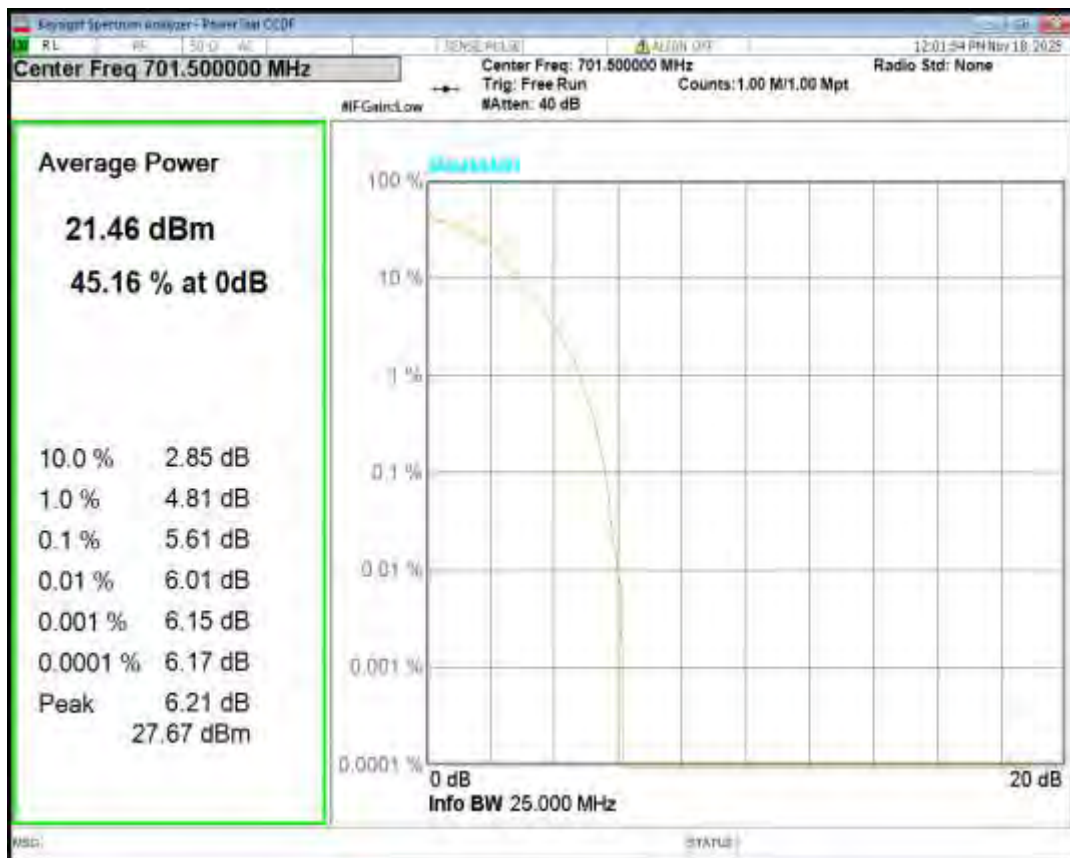
Band12 16QAM BW=5MHz Channel=23155 RB Size=1 Position=#0
