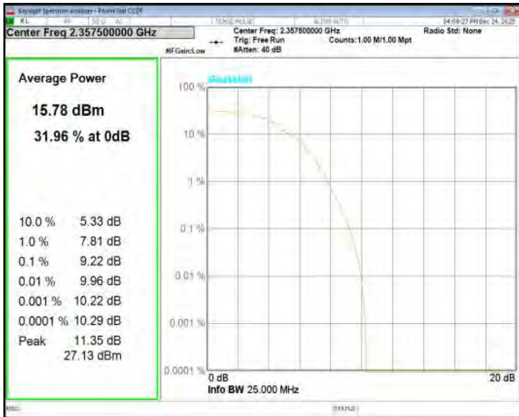
Band40(2350-2360) QPSK BW=10MHz Channel=39200 RB Size=1 Position=#0
