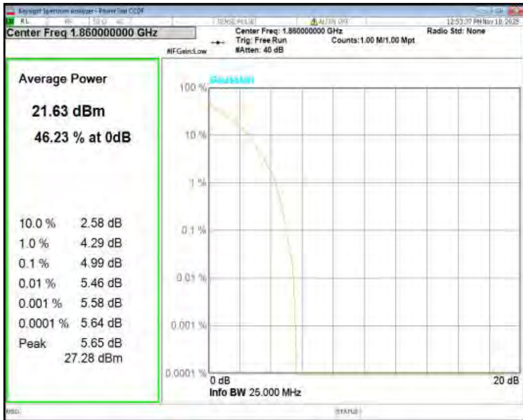
Band25 QPSK BW=20MHz Channel=26365 RB Size=1 Position=#0
