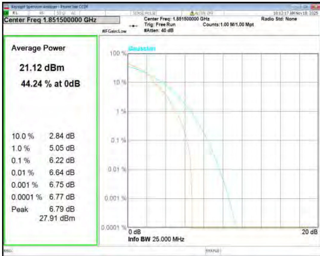
Band2 16QAM BW=3MHz Channel=18900 RB Size=1 Position=#0
