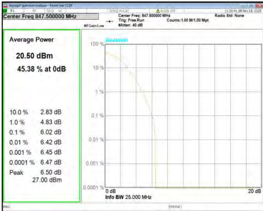
Band5 16QAM BW=5MHz Channel=20425 RB Size=1 Position=#0
