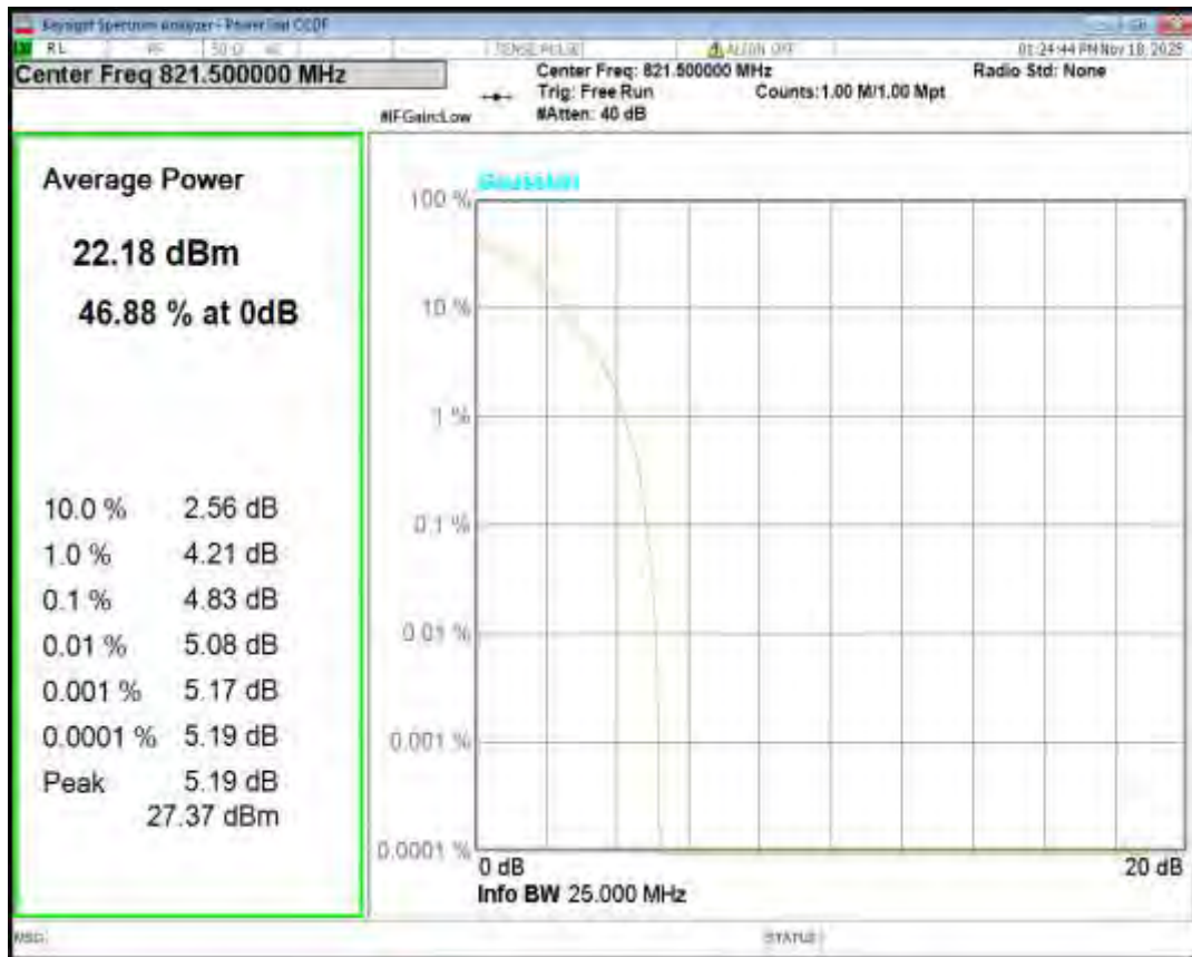
Band26(814-824) QPSK BW=10MHz Channel=26740 RB Size=1 Position=#0
