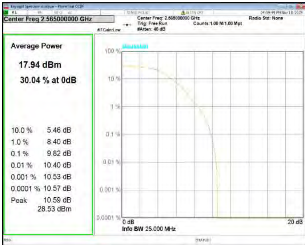
Band41(2555-2655) QPSK BW=20MHz Channel=40740 RB Size=1 Position=#0
