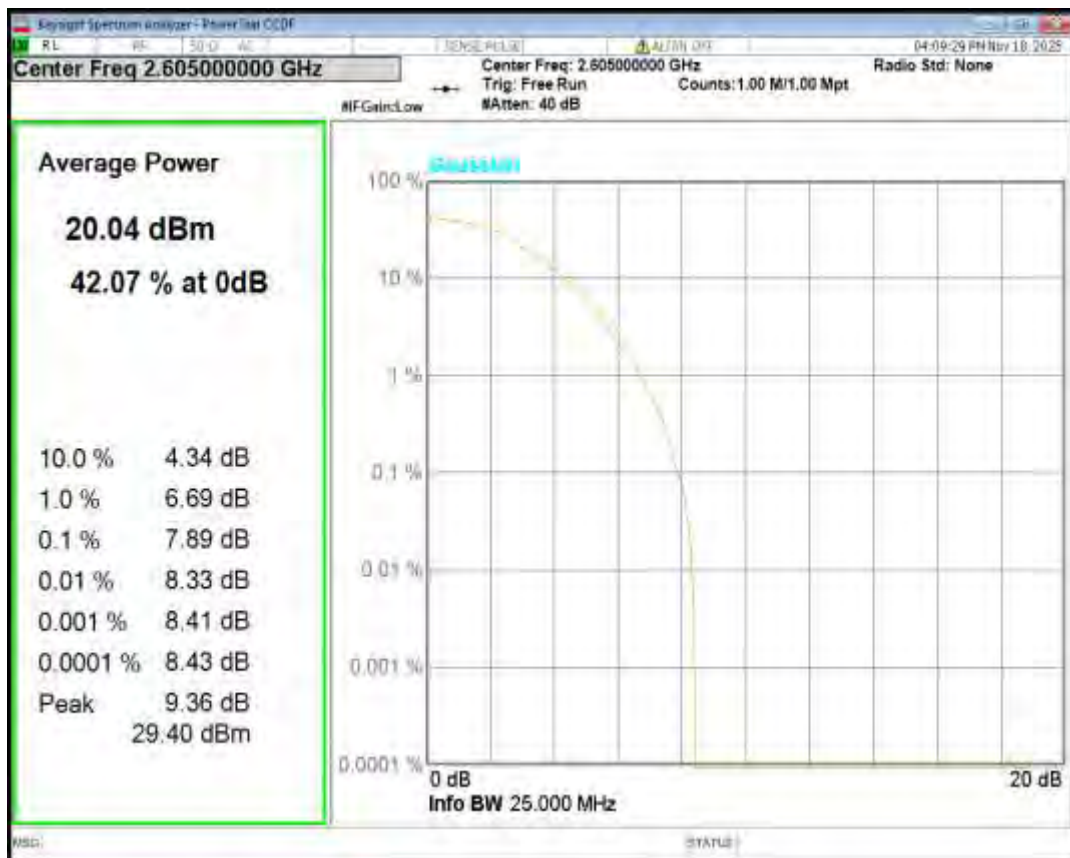
Band41(2555-2655) QPSK BW=10MHz Channel=41190 RB Size=1 Position=#0
