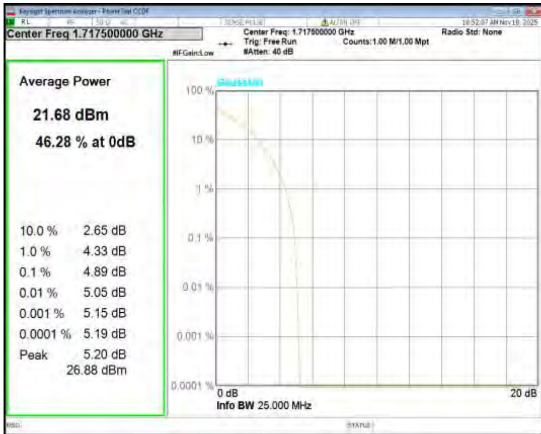
Band4 QPSK BW=15MHz Channel=20175 RB Size=1 Position=#0
