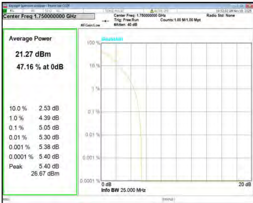
Band4 QPSK BW=15MHz Channel=20025 RB Size=1 Position=#0
