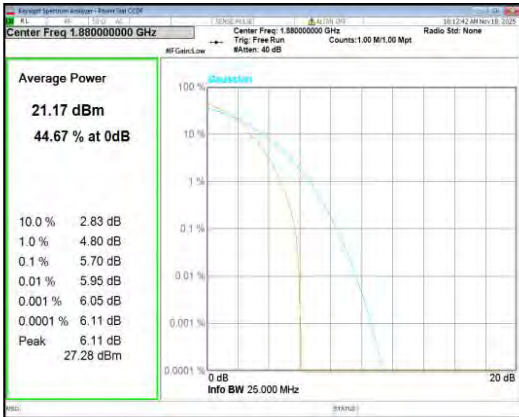
Band2 QPSK BW=1.4MHz Channel=18900 RB Size=1 Position=#0
