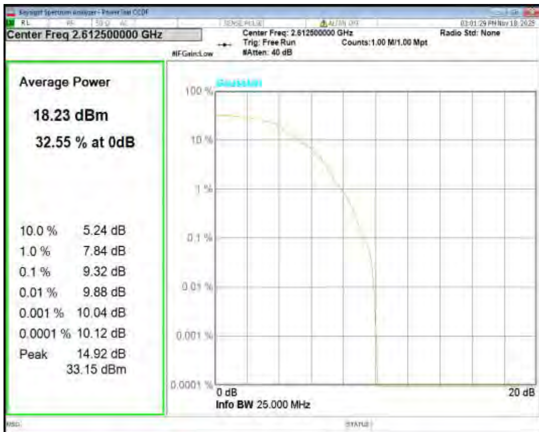
Band38 QPSK BW=20MHz Channel=37850 RB Size=1 Position=#0
