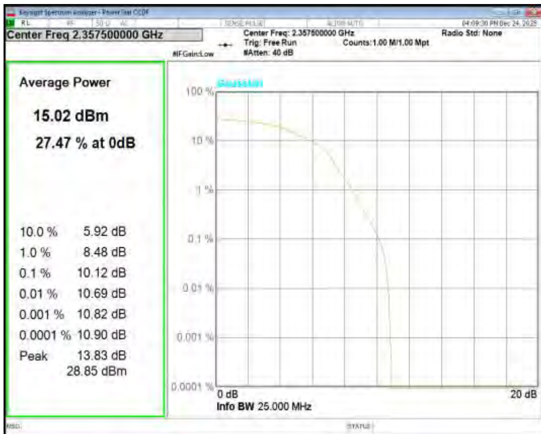
Band40(2350-2360) QPSK BW=5MHz Channel=39175 RB Size=1 Position=#0
