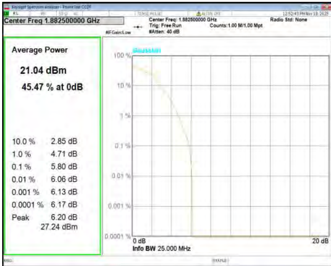
Band25 16QAM BW=3MHz Channel=26675 RB Size=1 Position=#0
