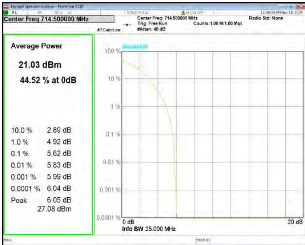
Band12 16QAM BW=5MHz Channel=23035 RB Size=1 Position=#0
