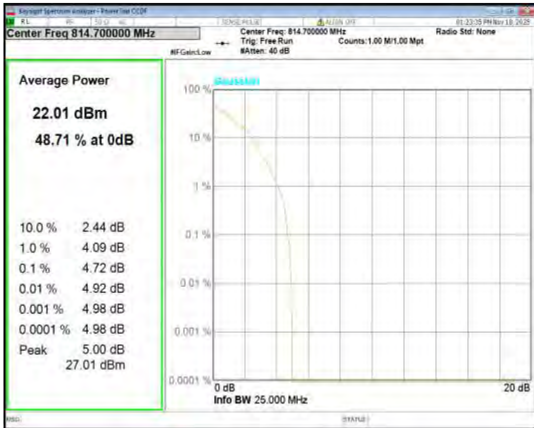
Band26(814-824) QPSK BW=1.4MHz Channel=26740 RB Size=1 Position=#0
