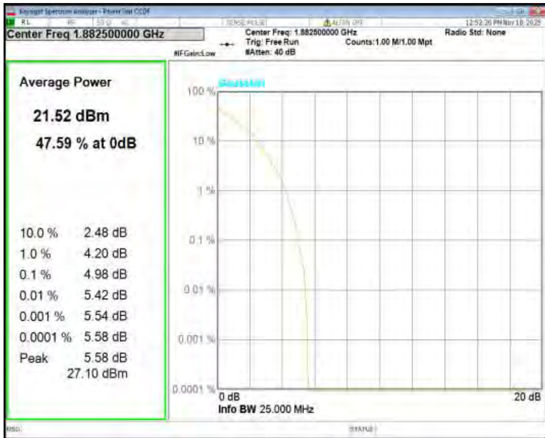
Band25 16QAM BW=5MHz Channel=26665 RB Size=1 Position=#0
