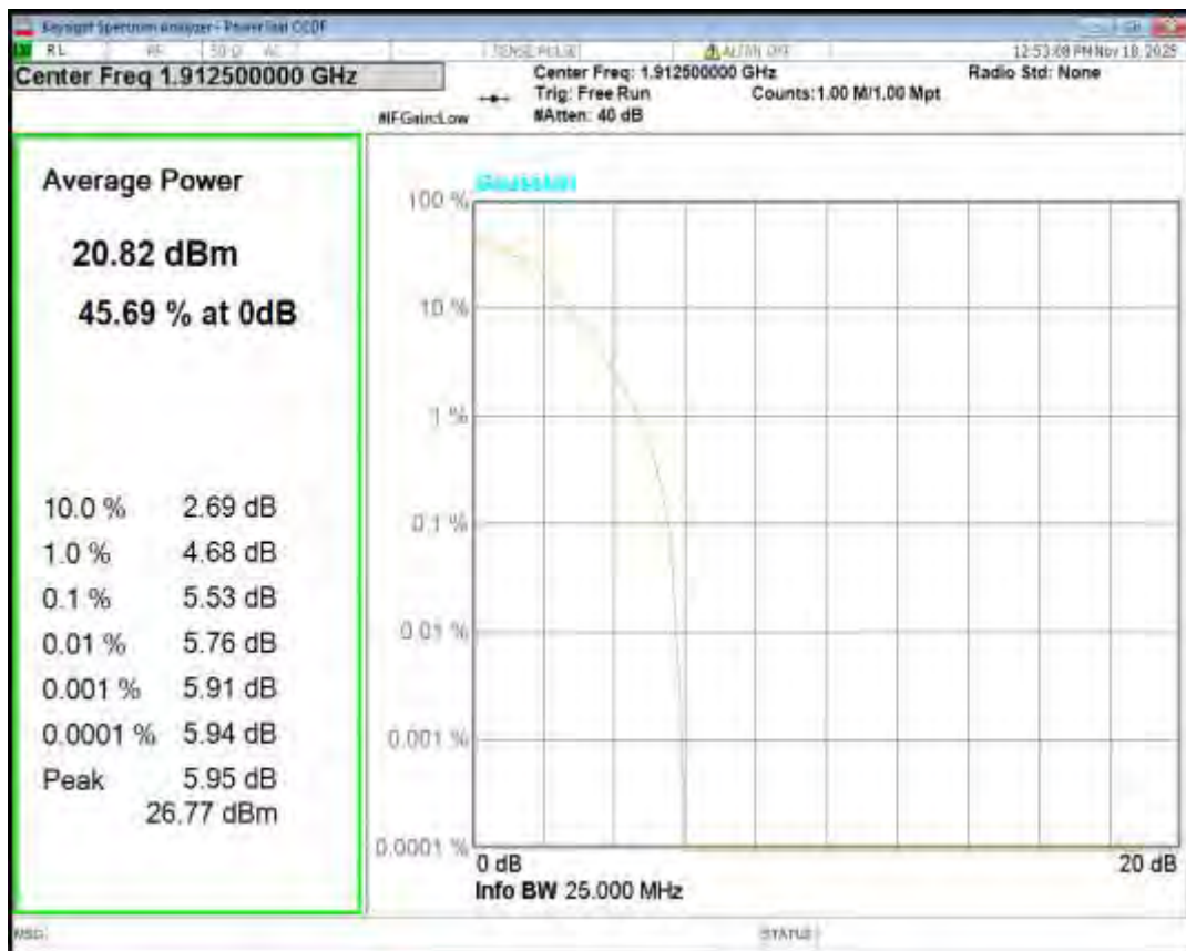
Band25 QPSK BW=1.4MHz Channel=26047 RB Size=1 Position=#0
