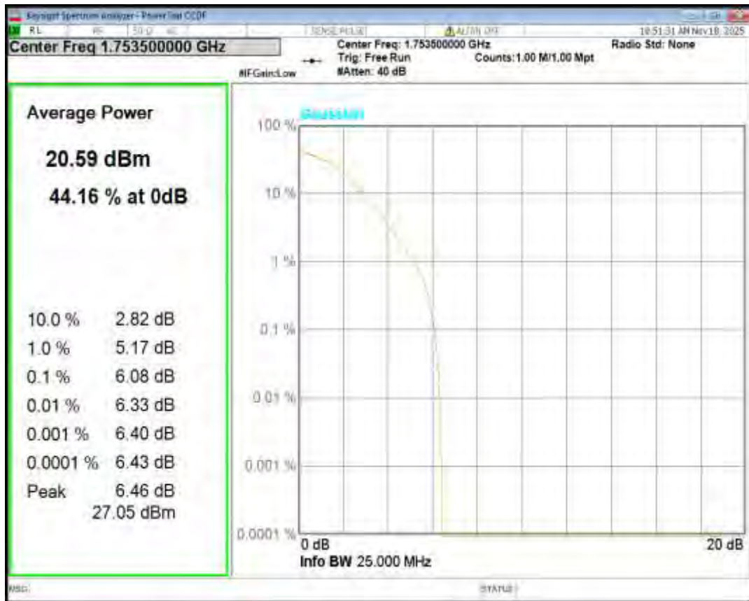
Band4 16QAM BW=5MHz Channel=19975 RB Size=1 Position=#0
