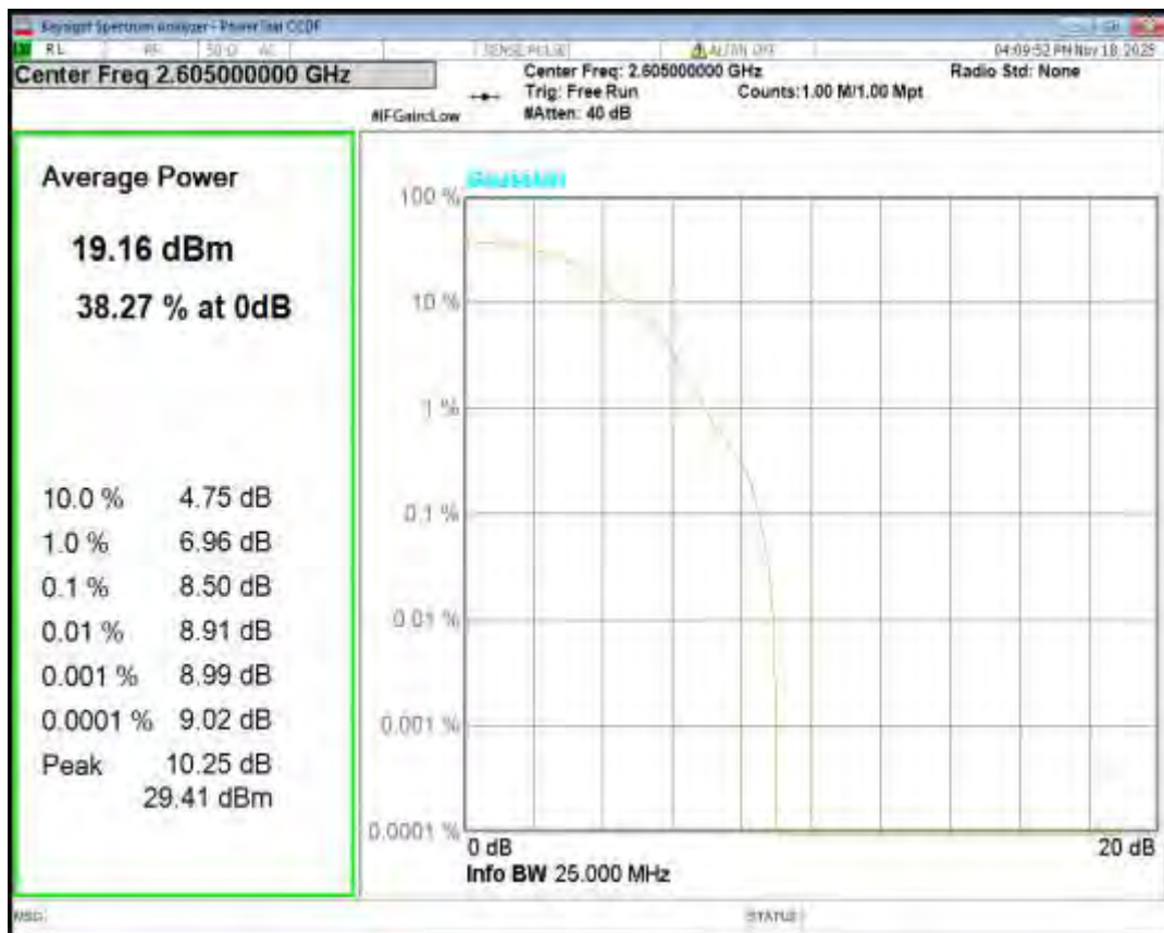
Band41(2555-2655) QPSK BW=20MHz Channel=41140 RB Size=1 Position=#0
