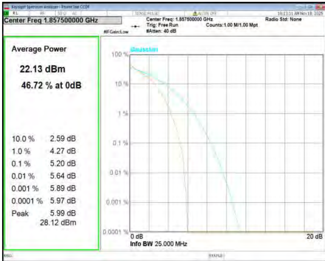
Band2 QPSK BW=15MHz Channel=18900 RB Size=1 Position=#0
