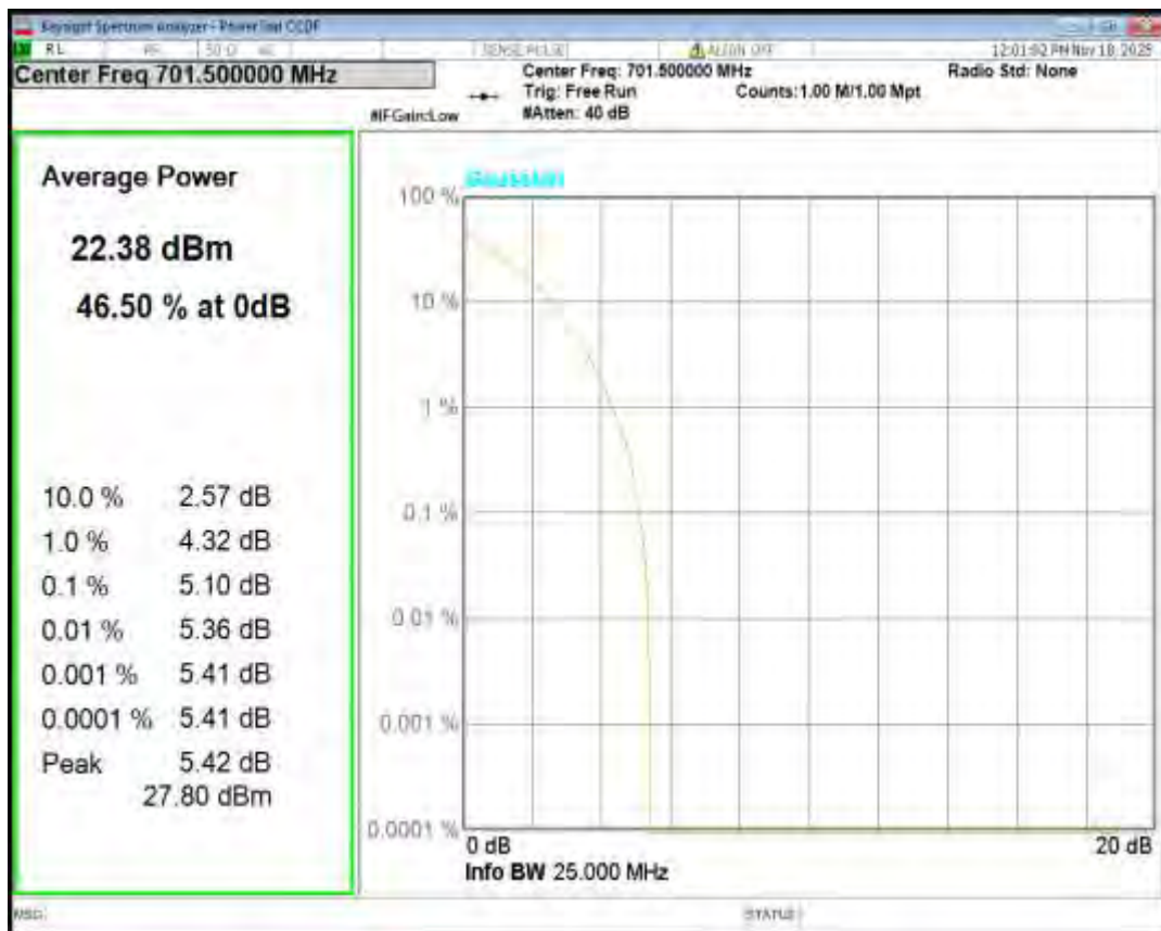
Band12 QPSK BW=5MHz Channel=23155 RB Size=1 Position=#0
