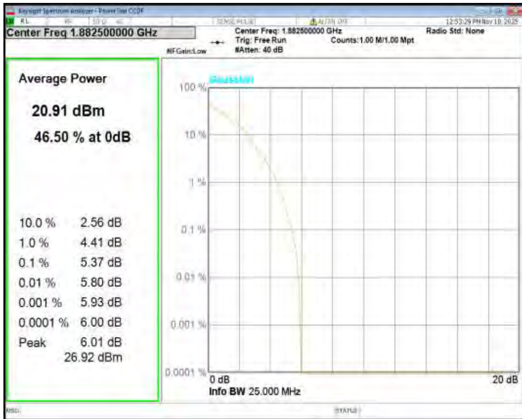
Band25 QPSK BW=15MHz Channel=26615 RB Size=1 Position=#0
