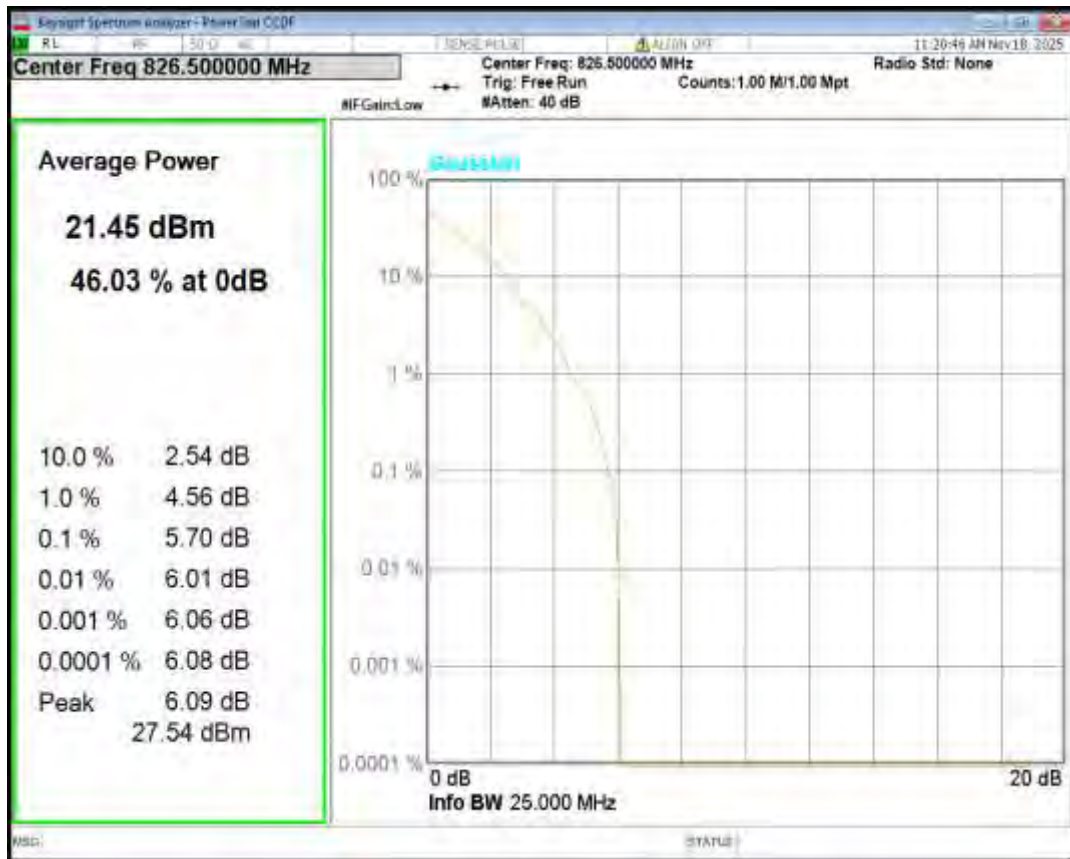
Band5 QPSK BW=5MHz Channel=20525 RB Size=1 Position=#0
