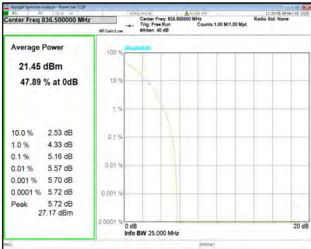
Band5 QPSK BW=1.4MHz Channel=20643 RB Size=1 Position=#0
