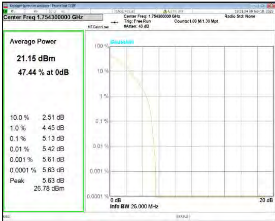
Band4 QPSK BW=3MHz Channel=19965 RB Size=1 Position=#0
