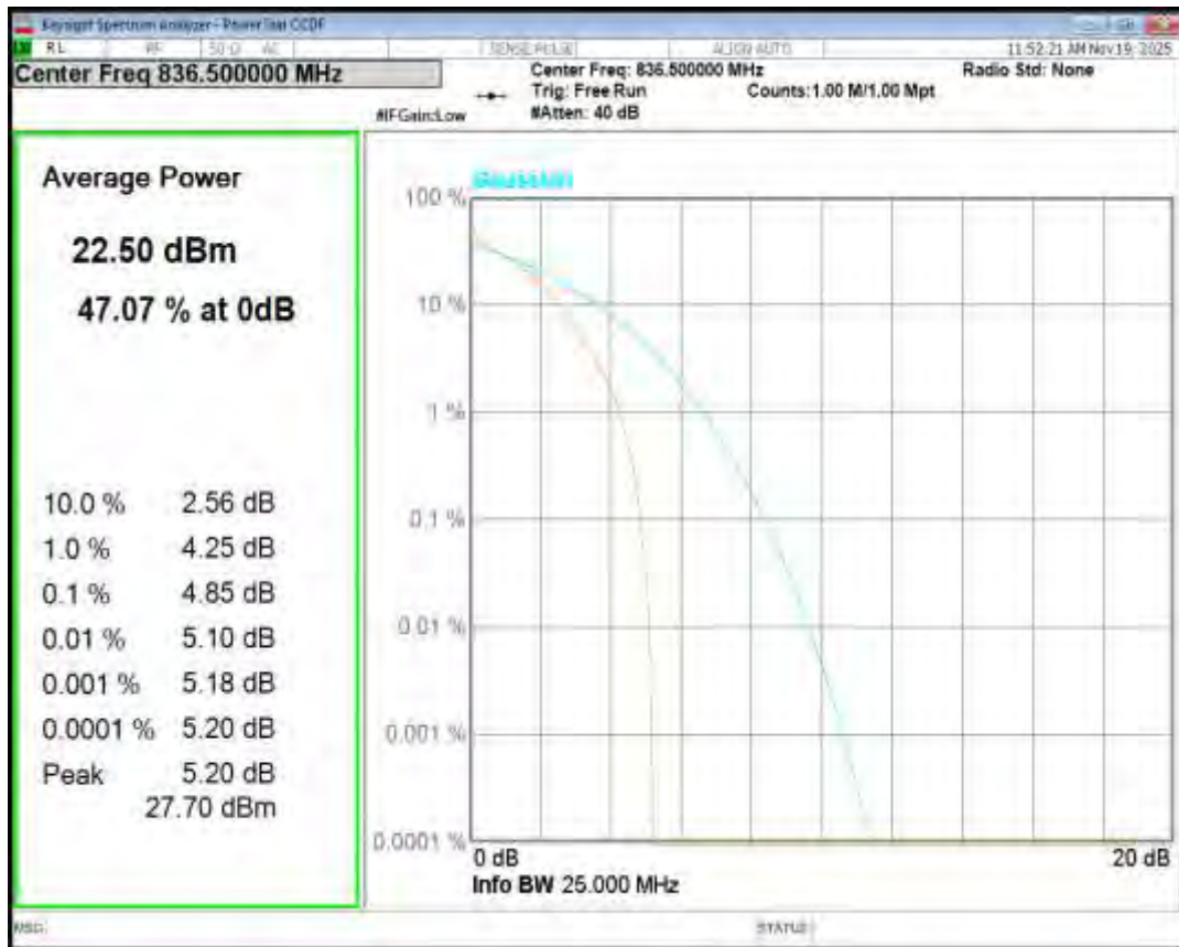
Band26(824-849) QPSK BW=5MHz Channel=27015 RB Size=1 Position=#0
