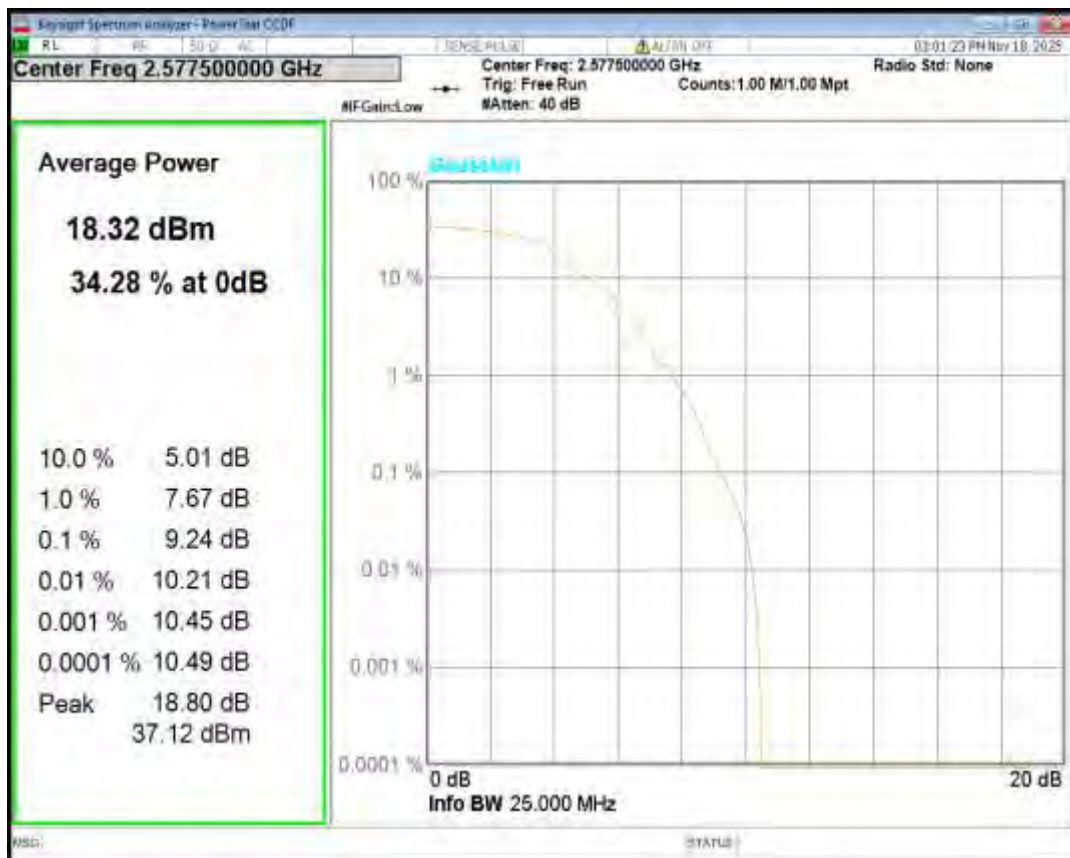
Band38 QPSK BW=15MHz Channel=38000 RB Size=1 Position=#0
