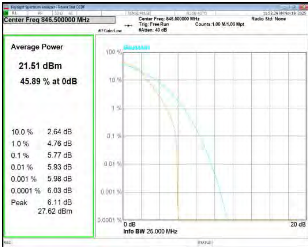
Band26(824-849) QPSK BW=1.4MHz Channel=26915 RB Size=1 Position=#0
