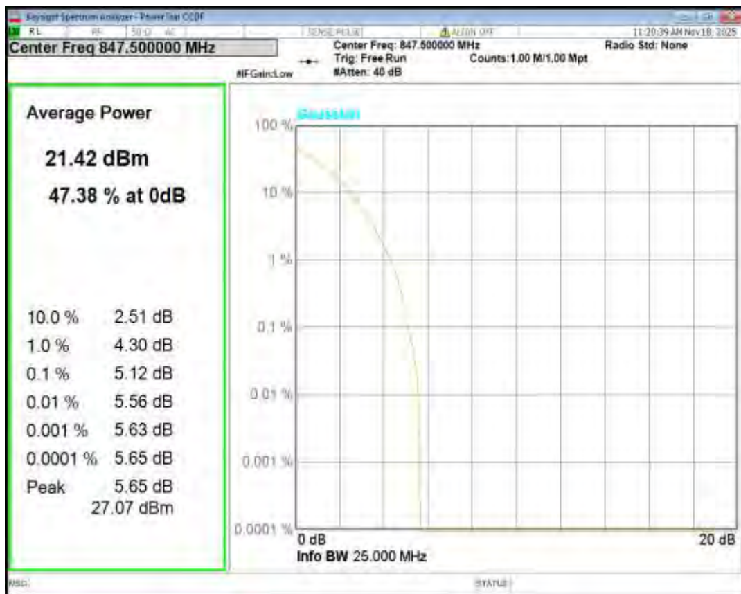
Band5 QPSK BW=5MHz Channel=20425 RB Size=1 Position=#0
