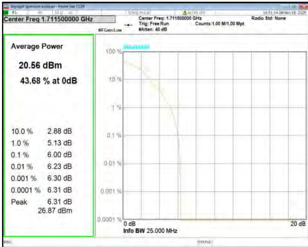
Band4 16QAM BW=3MHz Channel=20175 RB Size=1 Position=#0
