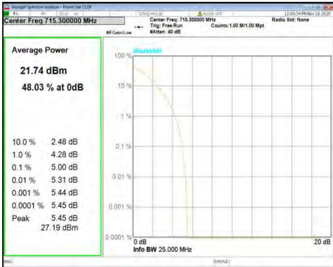
Band12 QPSK BW=3MHz Channel=23025 RB Size=1 Position=#0
