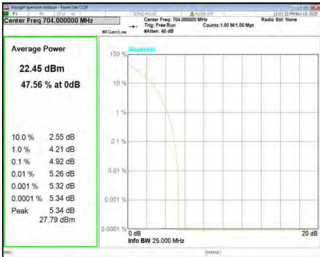
Band12 QPSK BW=10MHz Channel=23095 RB Size=1 Position=#0
