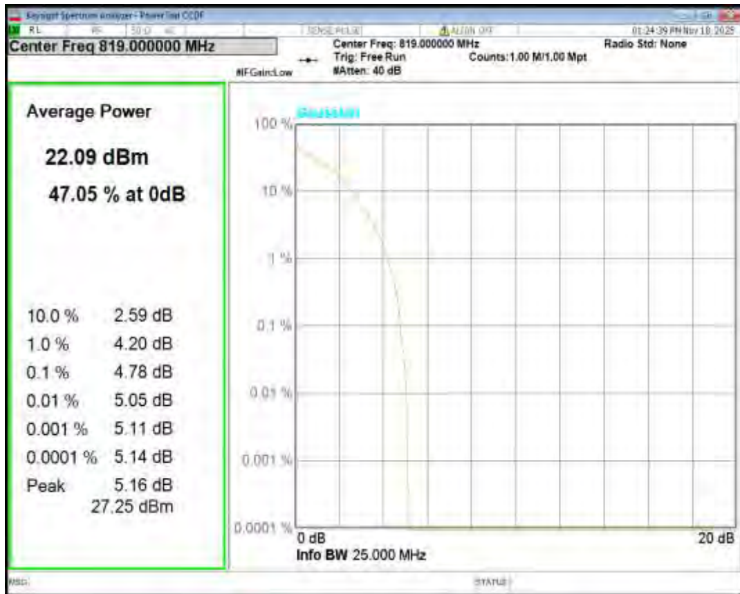
Band26(814-824) QPSK BW=5MHz Channel=26715 RB Size=1 Position=#0
