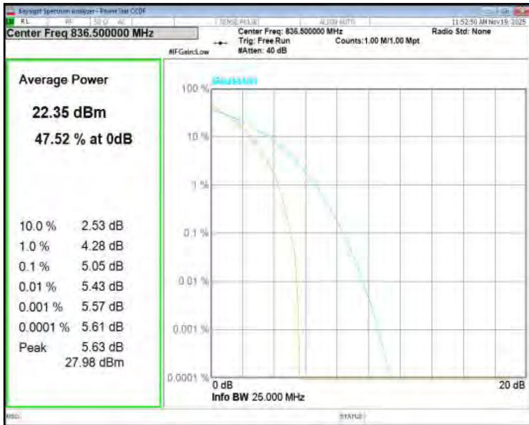
Band26(824-849) QPSK BW=15MHz Channel=26965 RB Size=1 Position=#0
