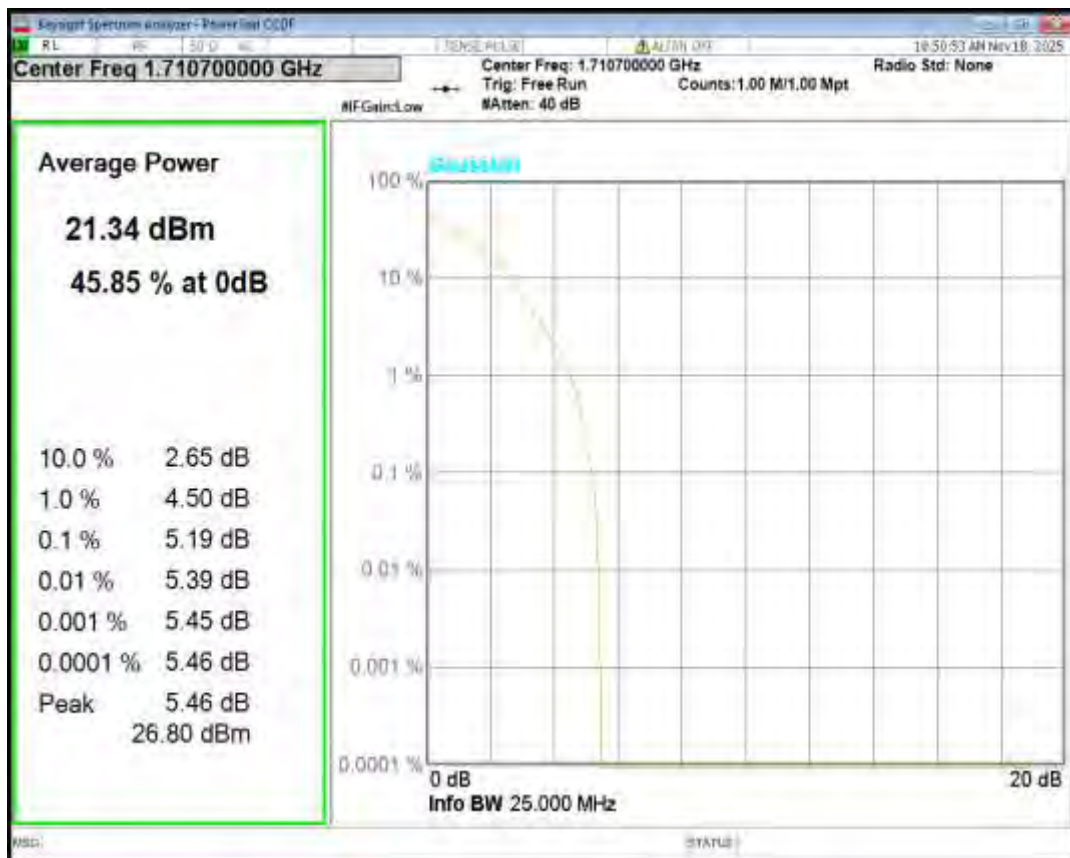
Band4 QPSK BW=1.4MHz Channel=20393 RB Size=1 Position=#0
