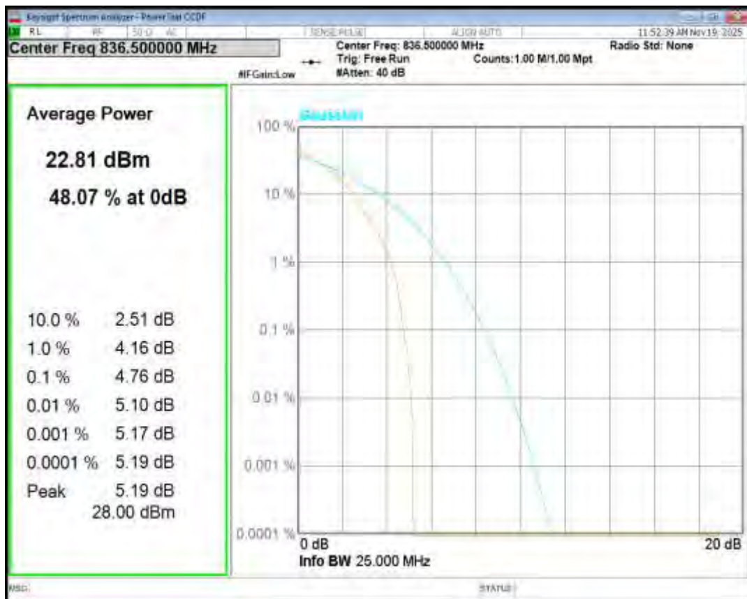
Band26(824-849) QPSK BW=10MHz Channel=26990 RB Size=1 Position=#0
