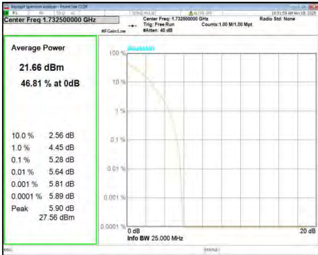
Band4 QPSK BW=10MHz Channel=20350 RB Size=1 Position=#0
