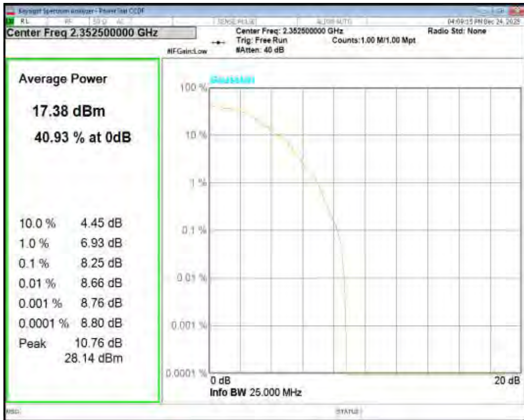
Band40(2350-2360) QPSK BW=5MHz Channel=39200 RB Size=1 Position=#0
