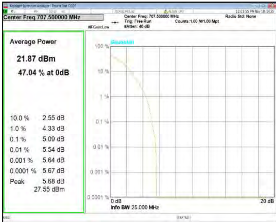
Band12 QPSK BW=10MHz Channel=23130 RB Size=1 Position=#0
