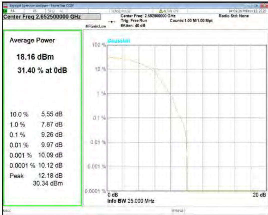
Band41(2555-2655) QPSK BW=5MHz Channel=40265 RB Size=1 Position=#0
