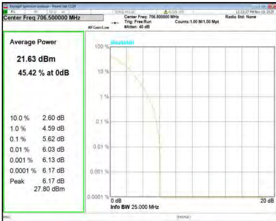
Band17 QPSK BW=5MHz Channel=23790 RB Size=1 Position=#0
