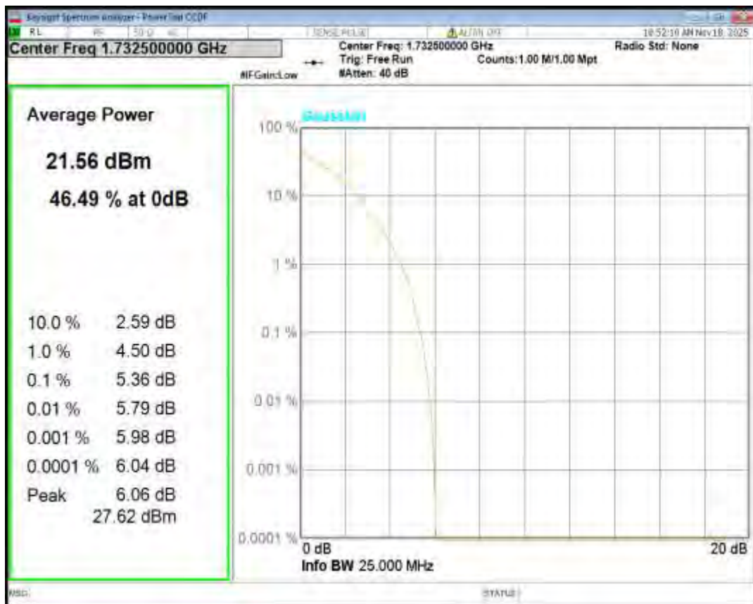
Band4 QPSK BW=15MHz Channel=20325 RB Size=1 Position=#0
