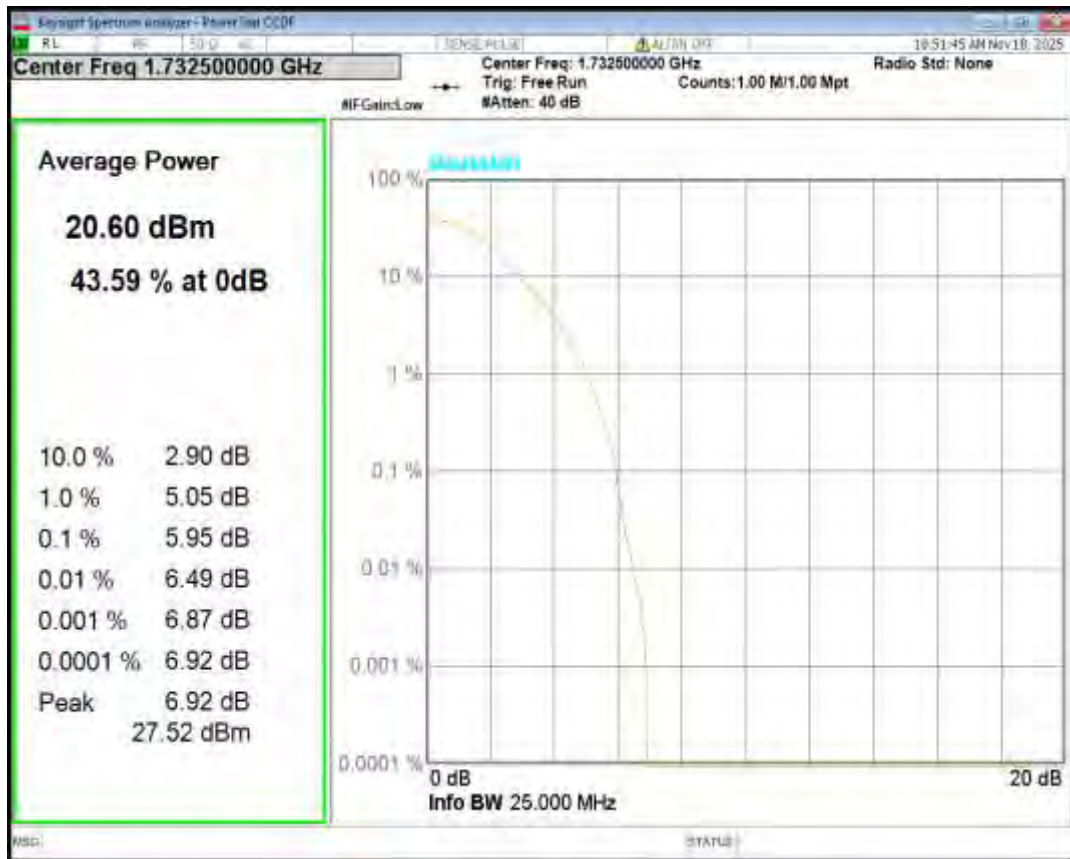
Band4 QPSK BW=1.4MHz Channel=20175 RB Size=1 Position=#0
