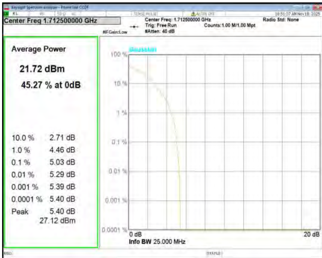
Band4 QPSK BW=5MHz Channel=20375 RB Size=1 Position=#0
