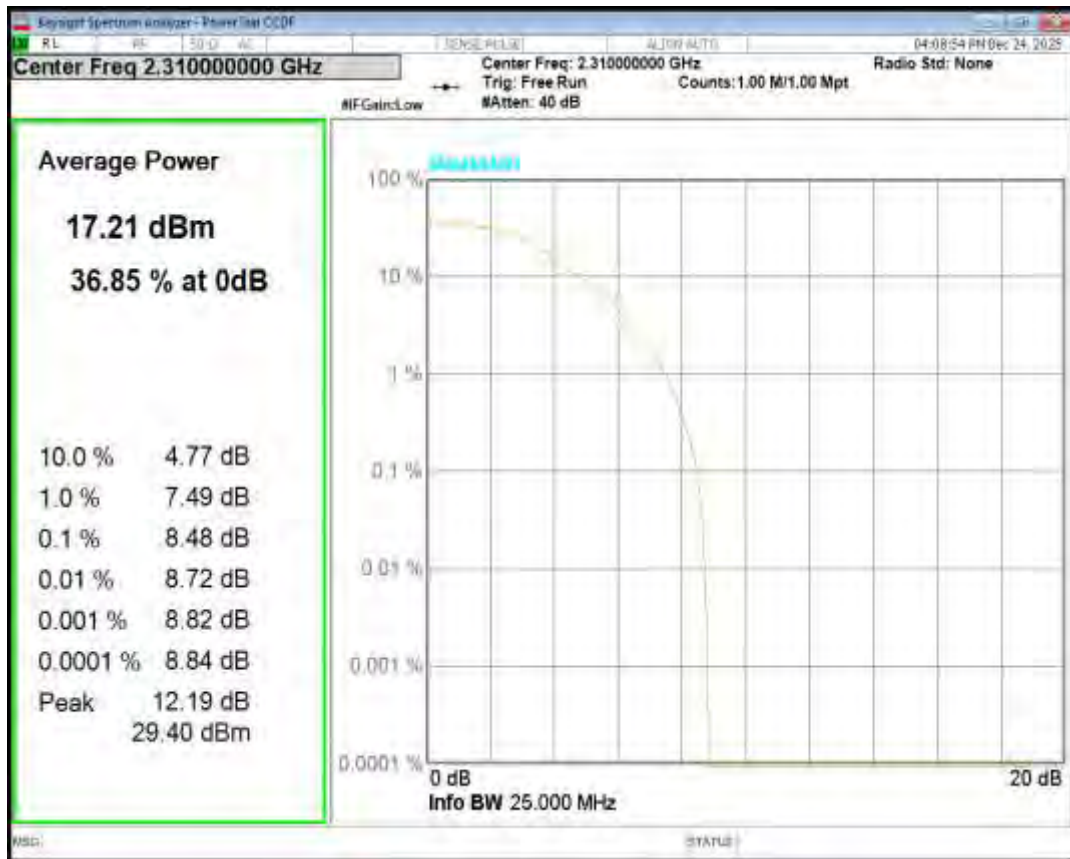
Band40(2305-2315) QPSK BW=5MHz Channel=38775 RB Size=1 Position=#0
