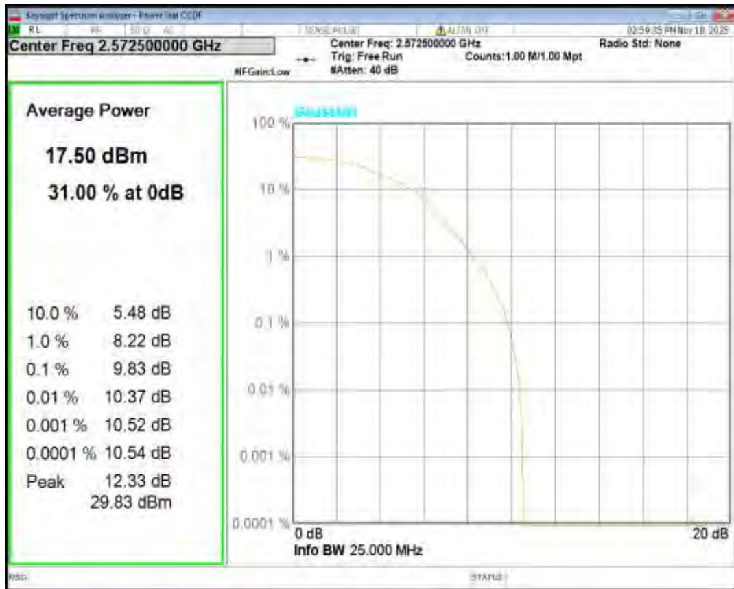
Band38 16QAM BW=5MHz Channel=38000 RB Size=1 Position=#0
