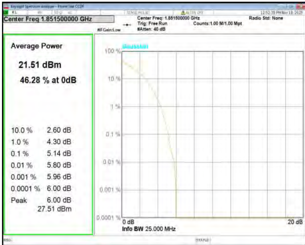
Band25 QPSK BW=3MHz Channel=26365 RB Size=1 Position=#0
