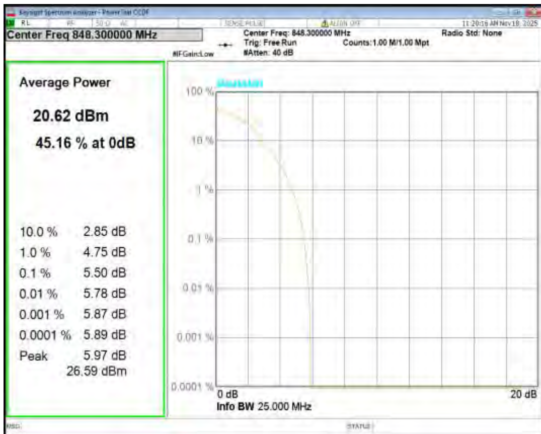
Band5 16QAM BW=3MHz Channel=20415 RB Size=1 Position=#0
