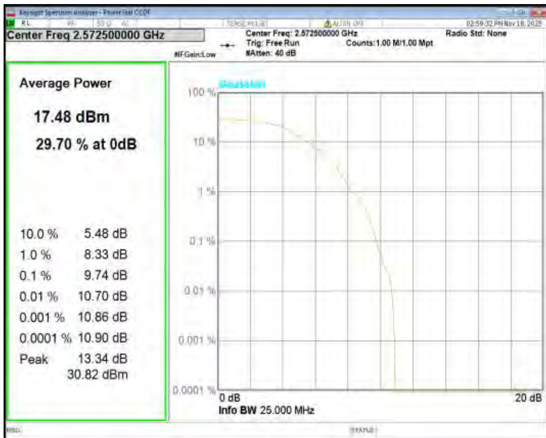
Band38 QPSK BW=5MHz Channel=38000 RB Size=1 Position=#0
