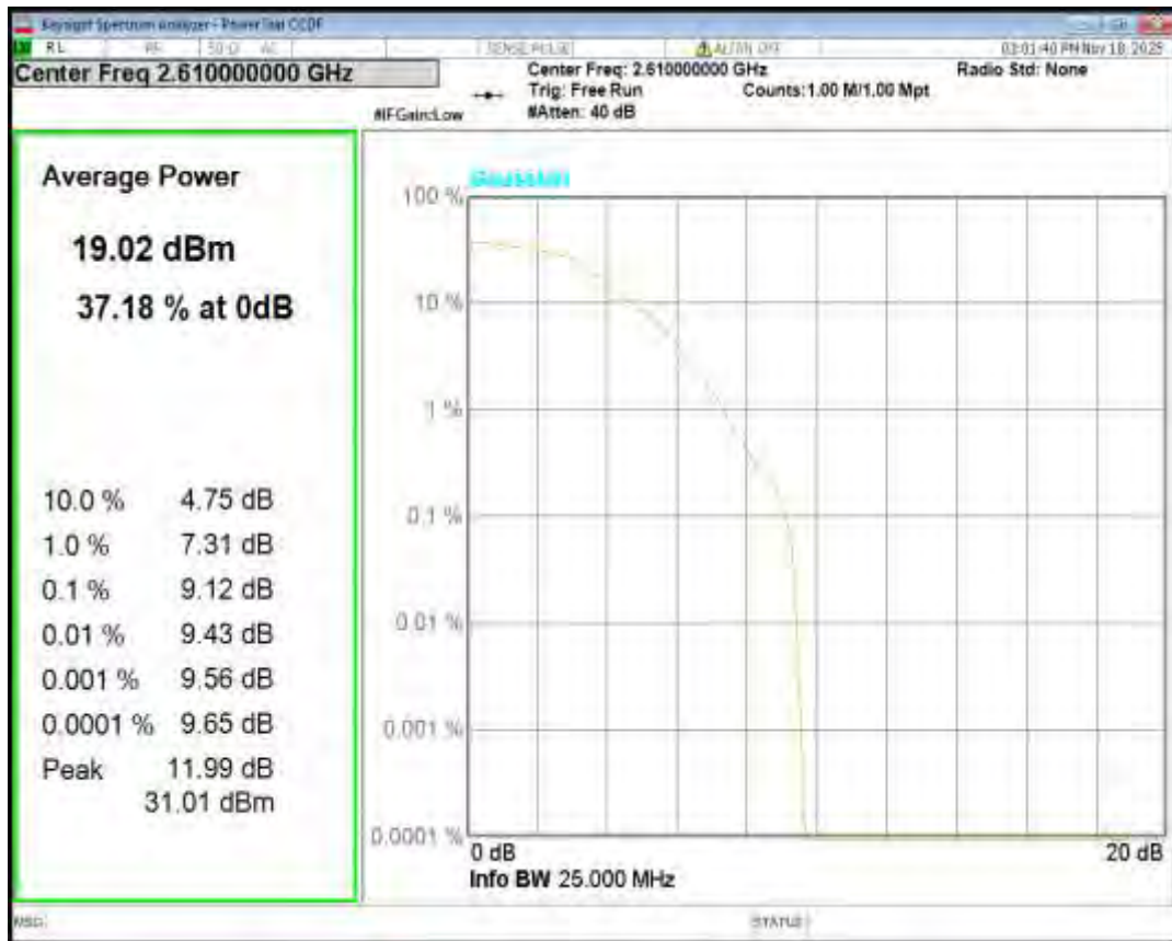
Band4 16QAM BW=1.4MHz Channel=19957 RB Size=1 Position=#0
