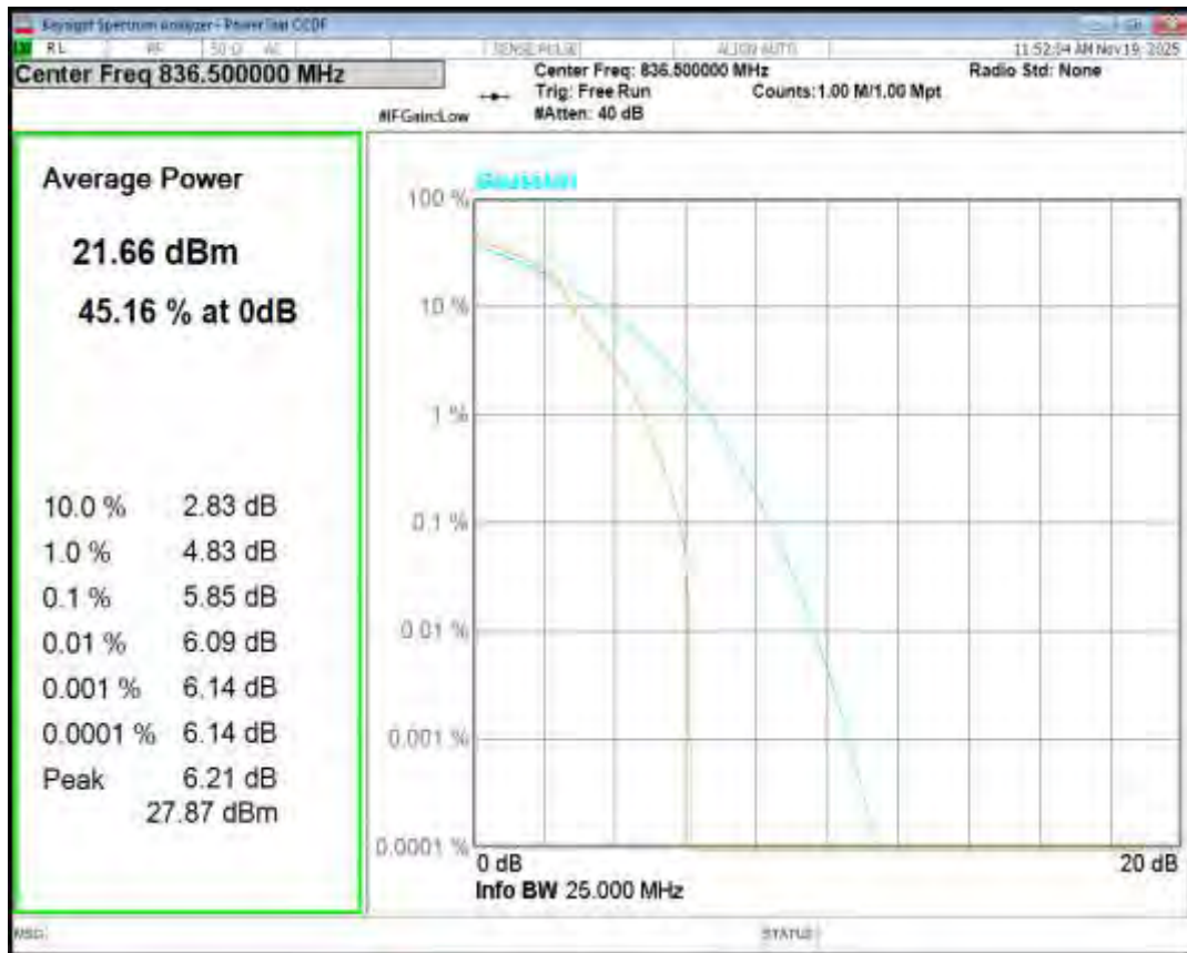
Band26(824-849) 16QAM BW=3MHz Channel=27025 RB Size=1 Position=#0
