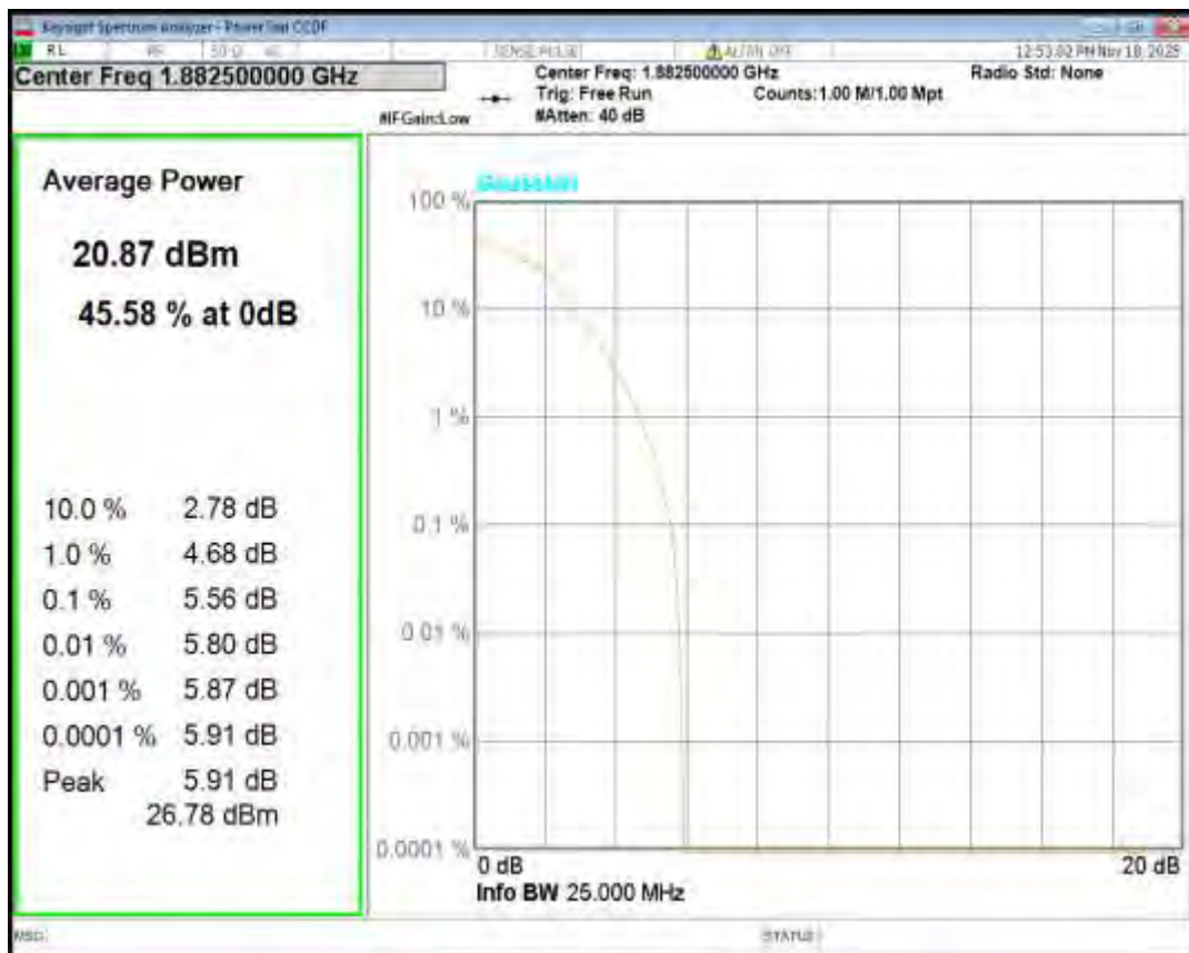
Band25 QPSK BW=1.4MHz Channel=26365 RB Size=1 Position=#0
