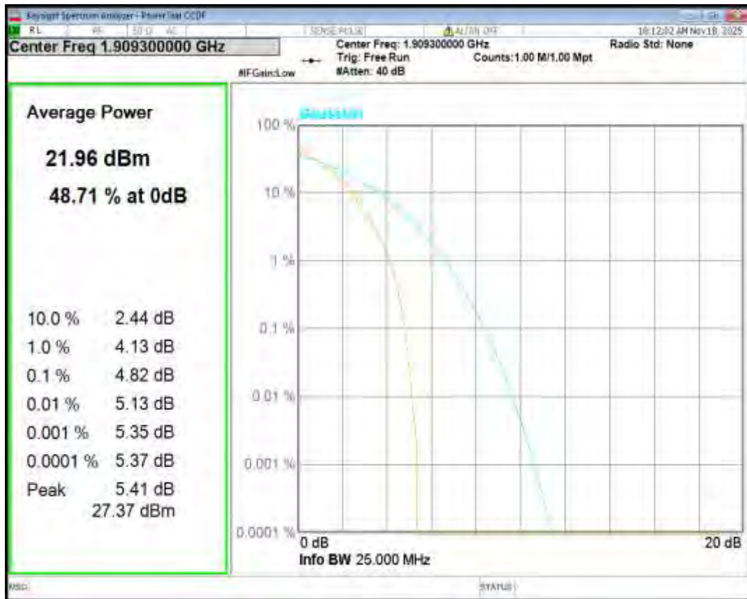
Band2 QPSK BW=3MHz Channel=18615 RB Size=1 Position=#0
