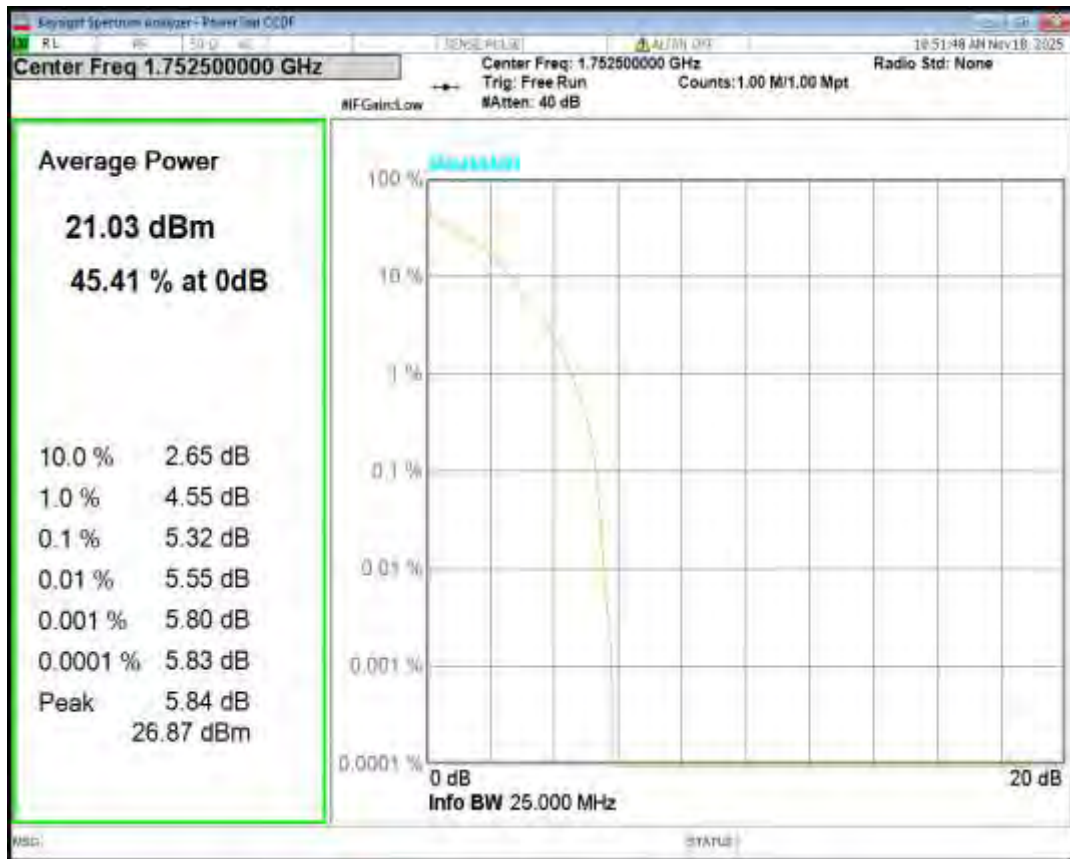
Band4 QPSK BW=10MHz Channel=20000 RB Size=1 Position=#0
