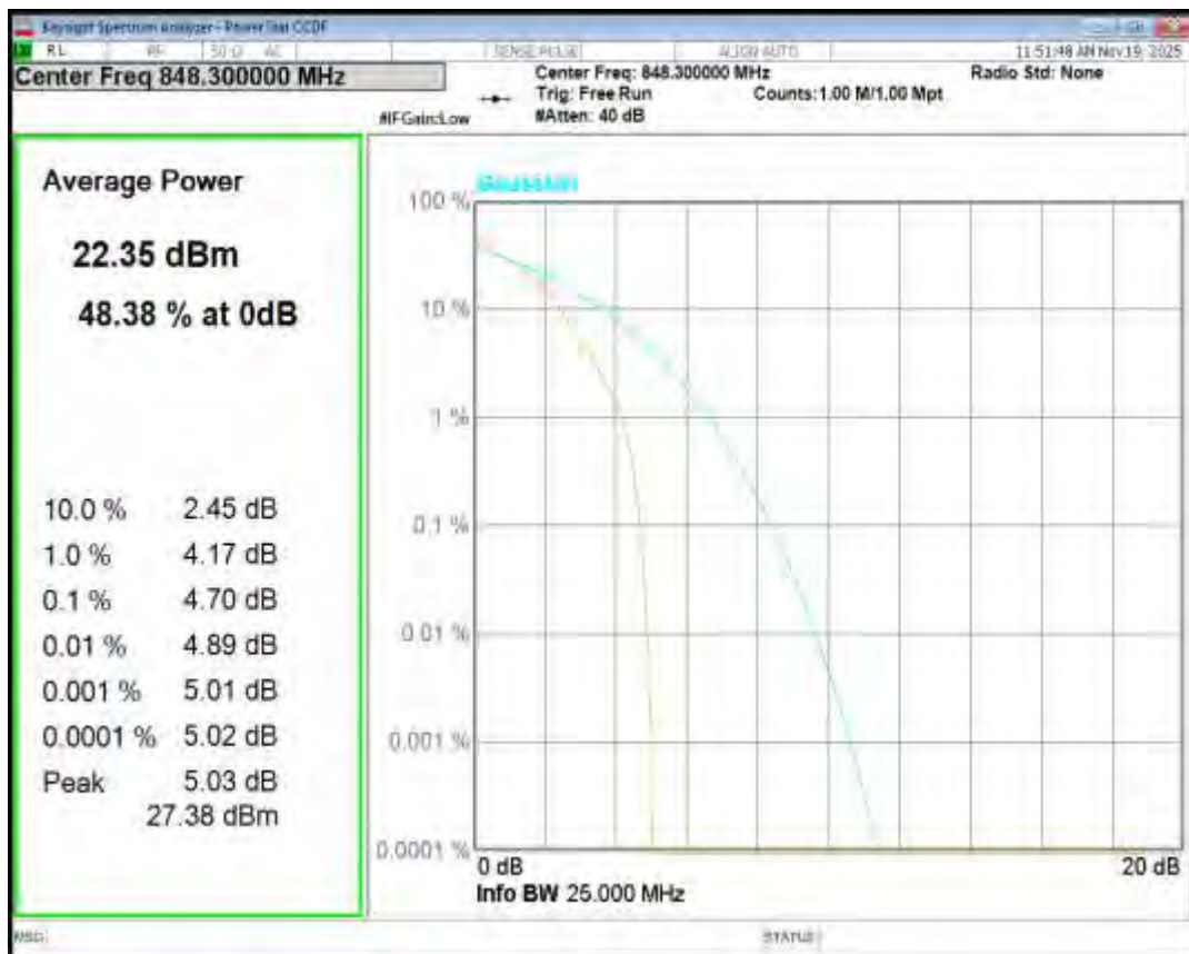
Band26(824-849) QPSK BW=3MHz Channel=26805 RB Size=1 Position=#0
