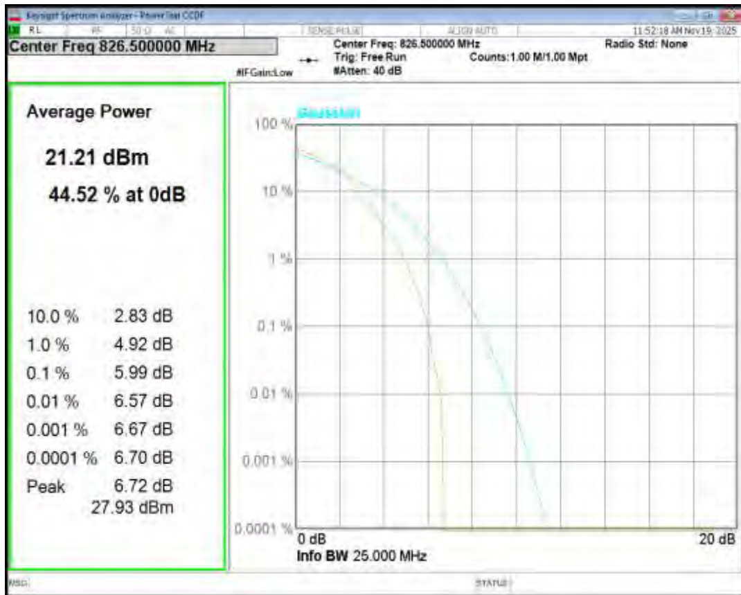
Band26(824-849) 16QAM BW=5MHz Channel=26915 RB Size=1 Position=#0
