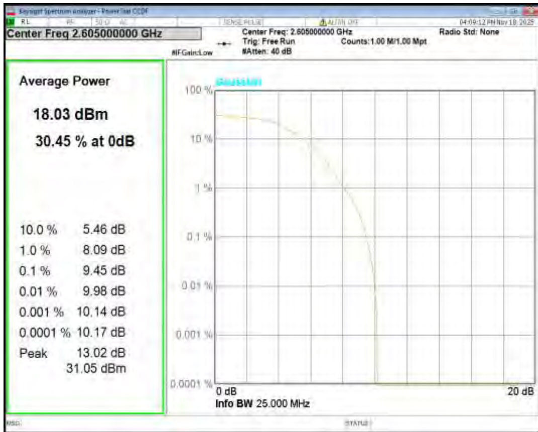
Band41(2555-2655) QPSK BW=5MHz Channel=41215 RB Size=1 Position=#0
