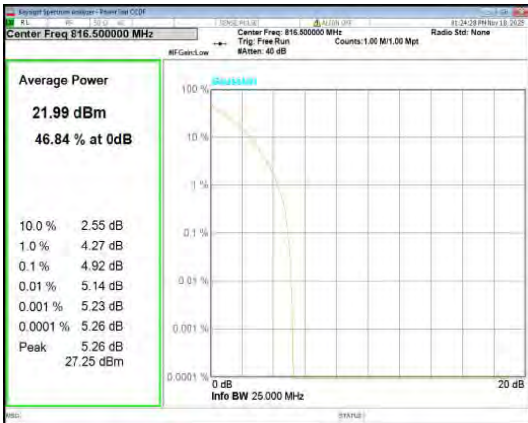
Band26(814-824) QPSK BW=5MHz Channel=26765 RB Size=1 Position=#0
