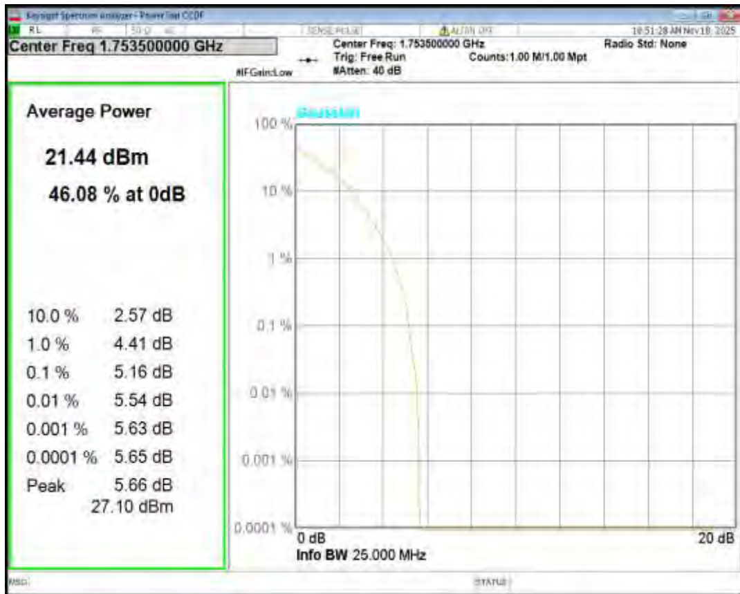
Band4 QPSK BW=5MHz Channel=19975 RB Size=1 Position=#0
