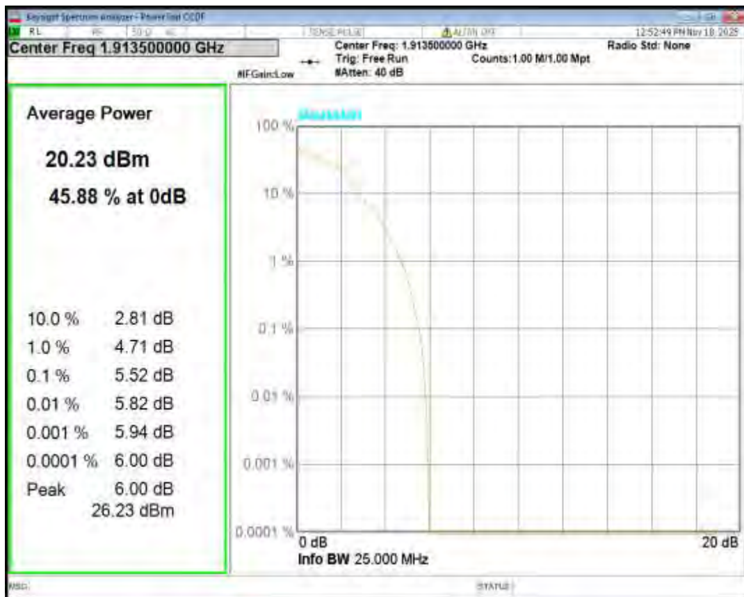
Band25 16QAM BW=5MHz Channel=26065 RB Size=1 Position=#0
