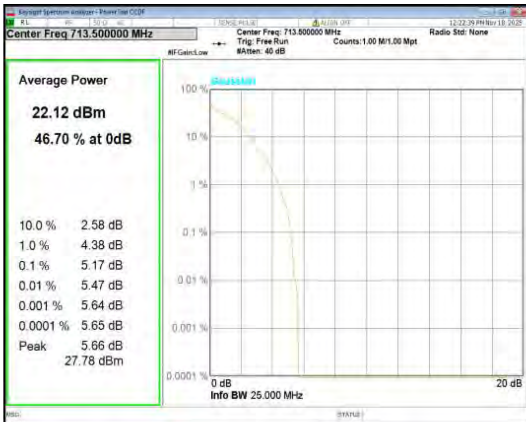
Band17 QPSK BW=10MHz Channel=23780 RB Size=1 Position=#0
