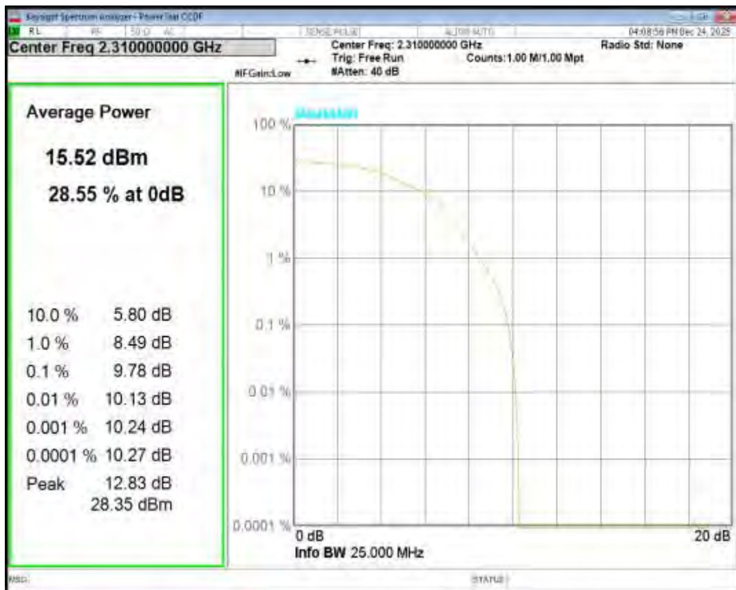
Band40(2305-2315) 16QAM BW=5MHz Channel=38775 RB Size=1 Position=#0
