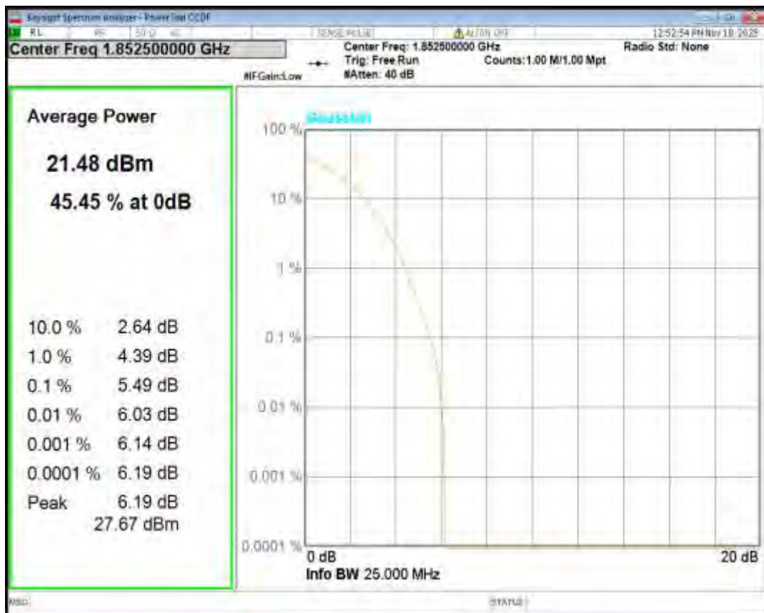
Band25 QPSK BW=5MHz Channel=26365 RB Size=1 Position=#0
