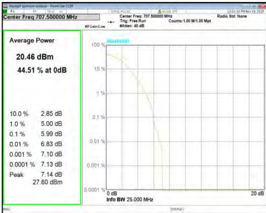
Band12 QPSK BW=1.4MHz Channel=23017 RB Size=1 Position=#0
