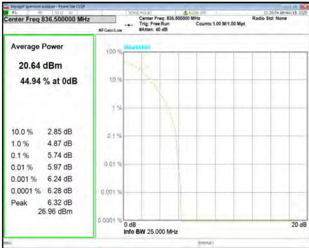
Band5 QPSK BW=1.4MHz Channel=20407 RB Size=1 Position=#0
