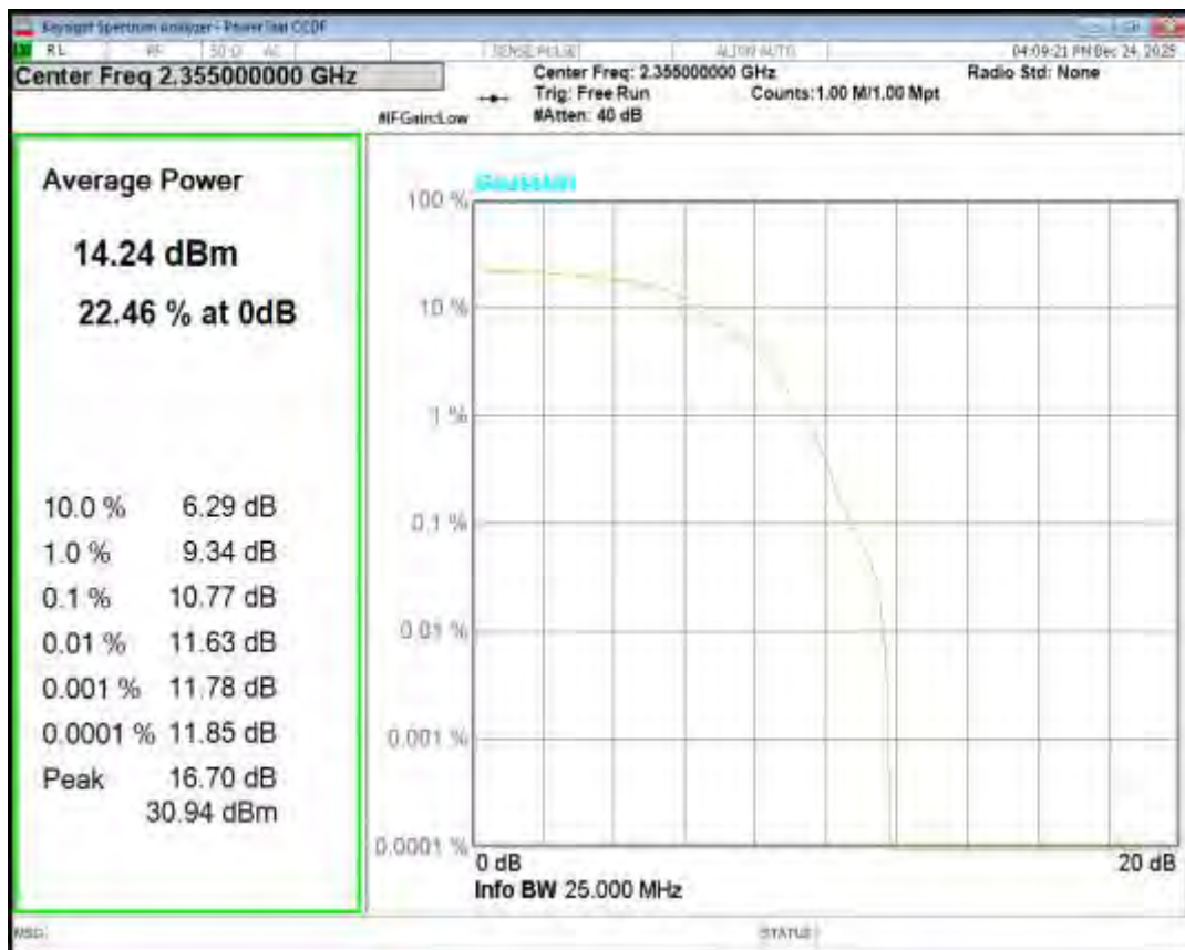
Band40(2350-2360) QPSK BW=5MHz Channel=39225 RB Size=1 Position=#0
