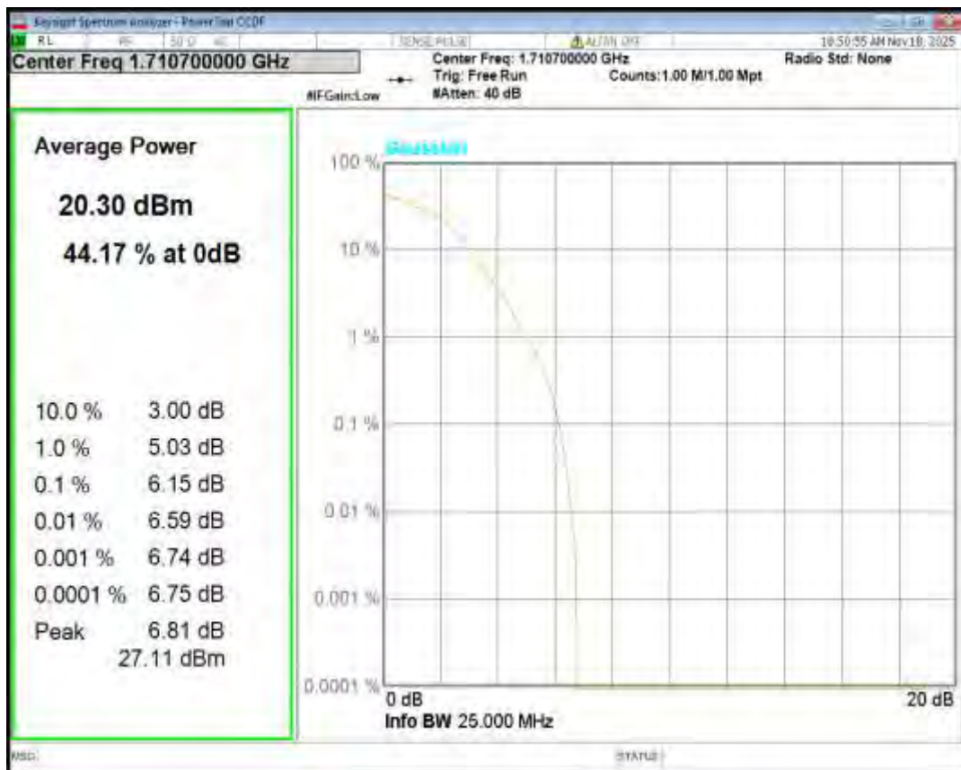
Band4 16QAM BW=1.4MHz Channel=20175 RB Size=1 Position=#0
