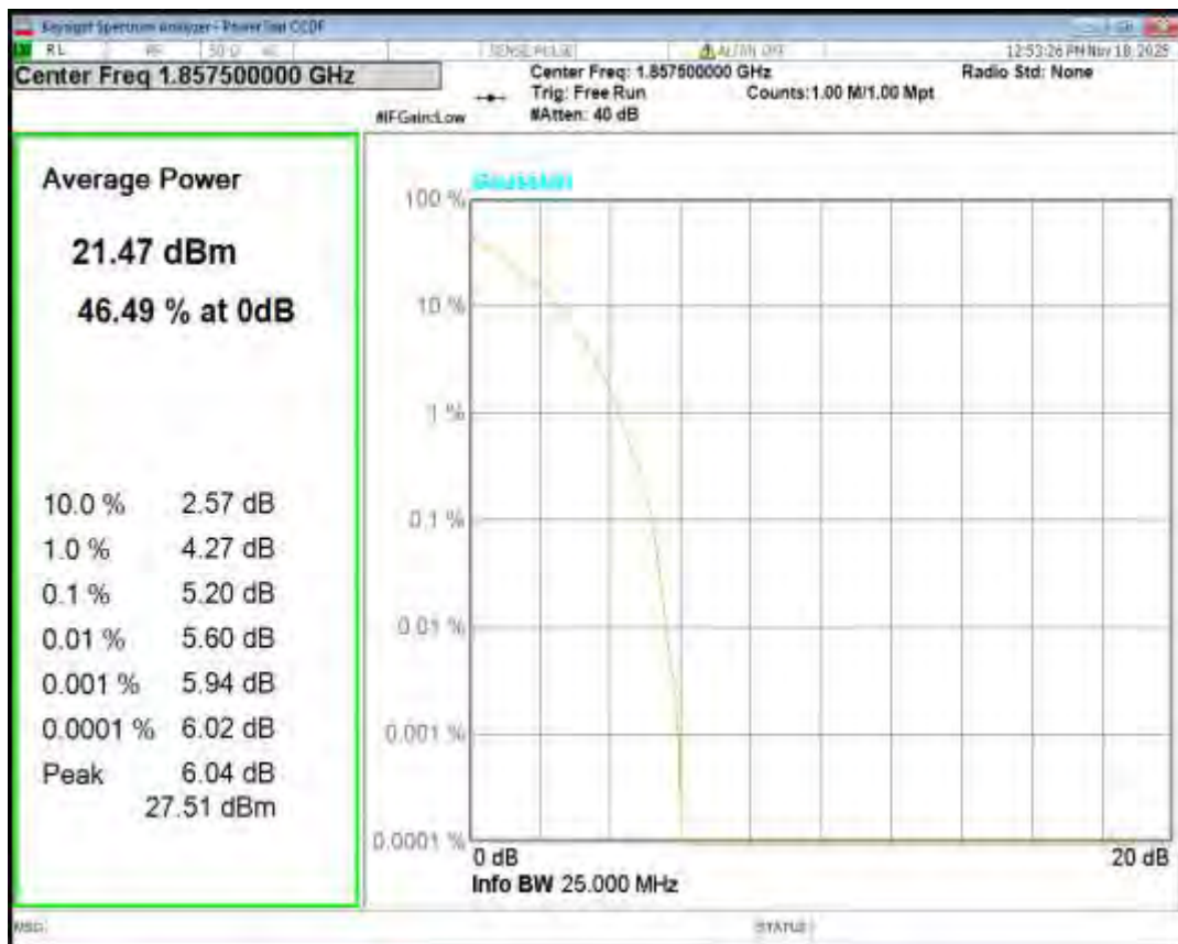
Band25 QPSK BW=15MHz Channel=26365 RB Size=1 Position=#0
