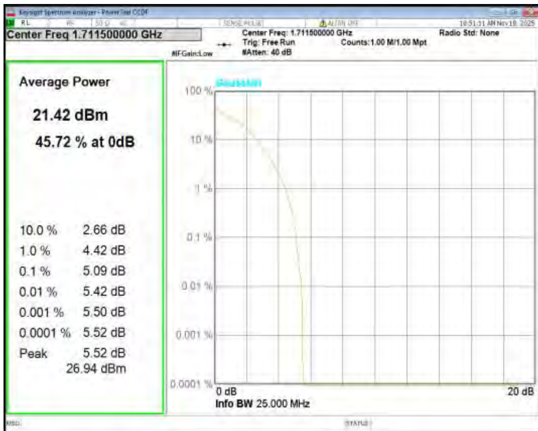
Band4 QPSK BW=3MHz Channel=20175 RB Size=1 Position=#0
