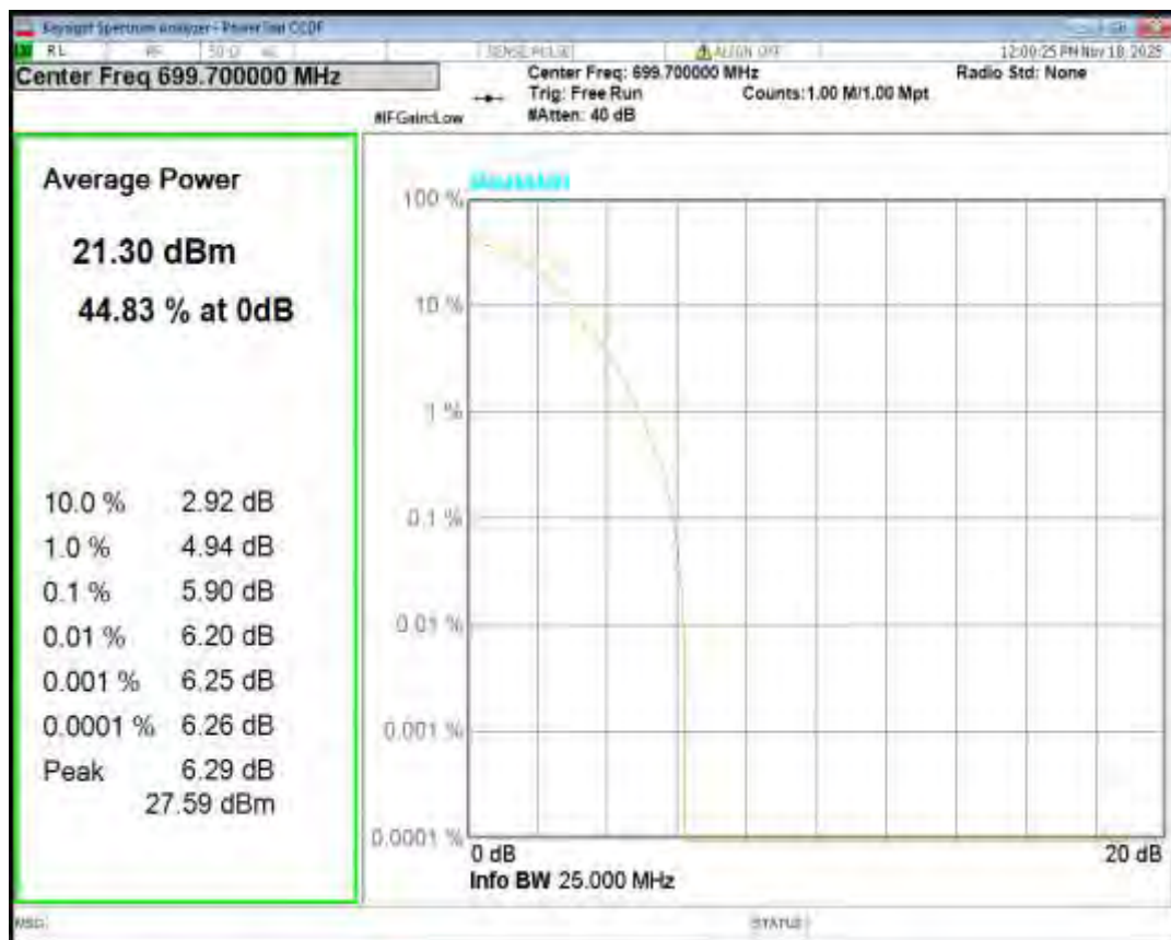
Band12 16QAM BW=1.4MHz Channel=23095 RB Size=1 Position=#0
