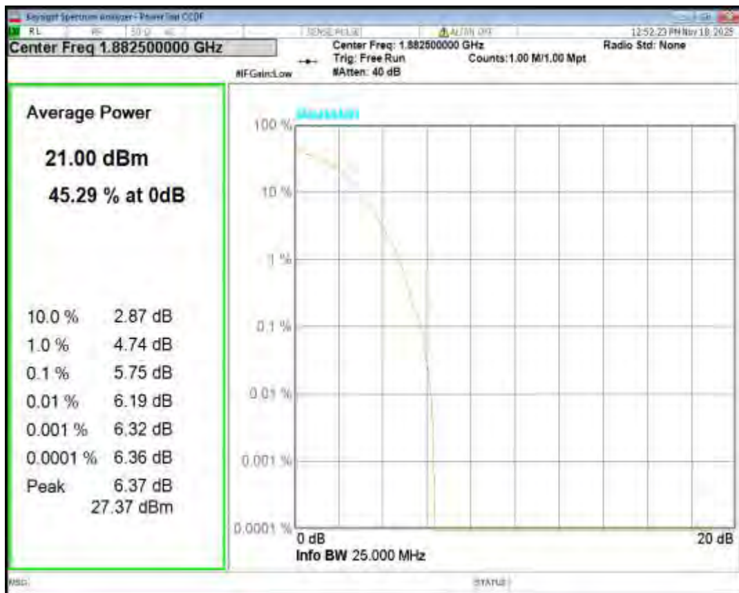
Band25 16QAM BW=1.4MHz Channel=26683 RB Size=1 Position=#0
