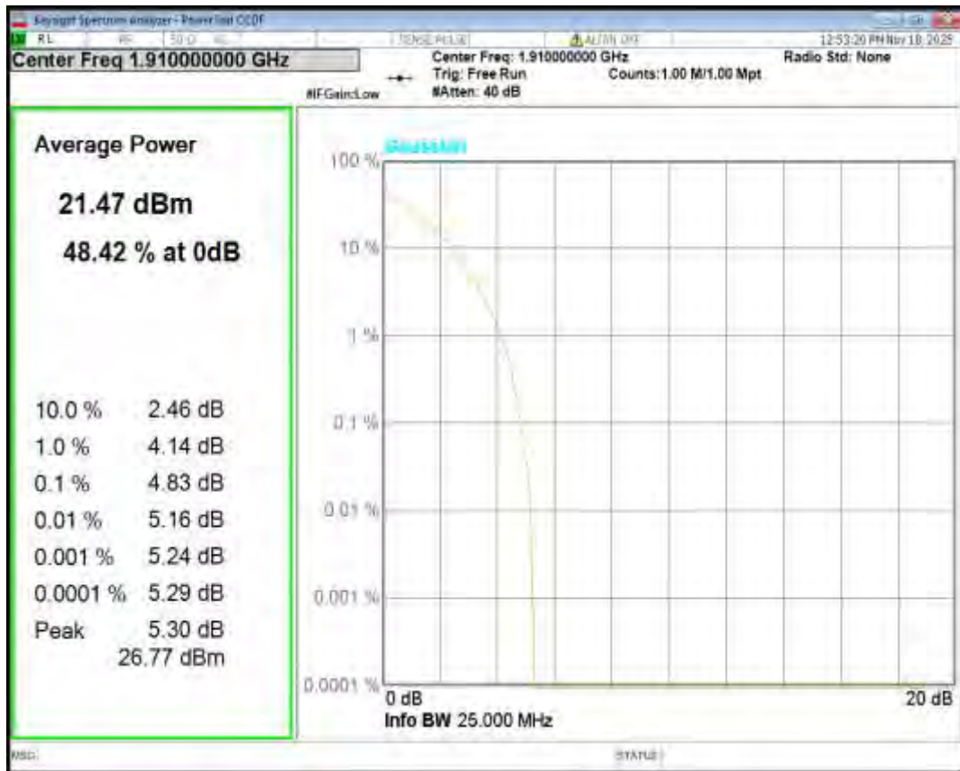
Band25 QPSK BW=15MHz Channel=26115 RB Size=1 Position=#0
