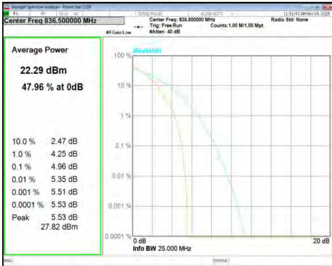
Band26(824-849) QPSK BW=1.4MHz Channel=27033 RB Size=1 Position=#0
