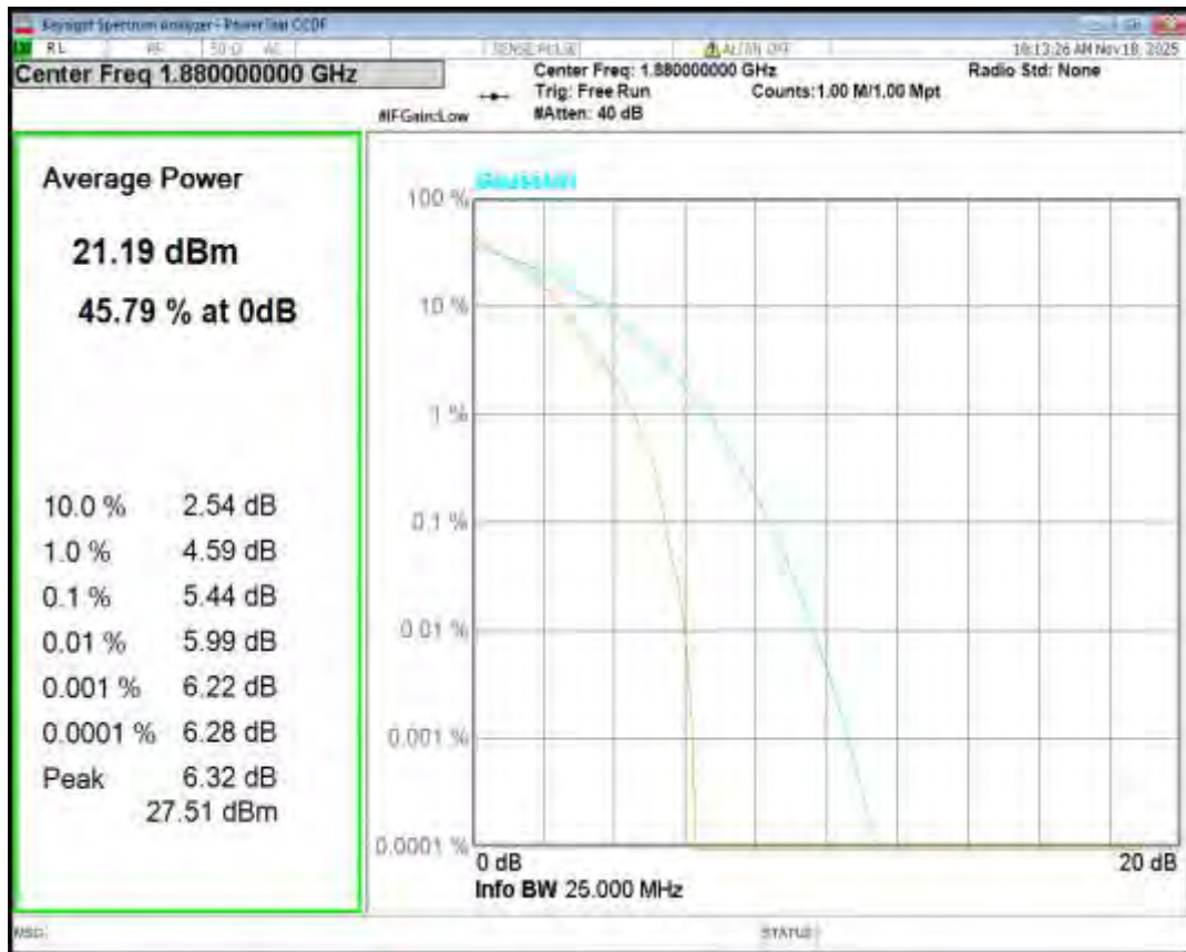
Band2 QPSK BW=20MHz Channel=19100 RB Size=1 Position=#0
