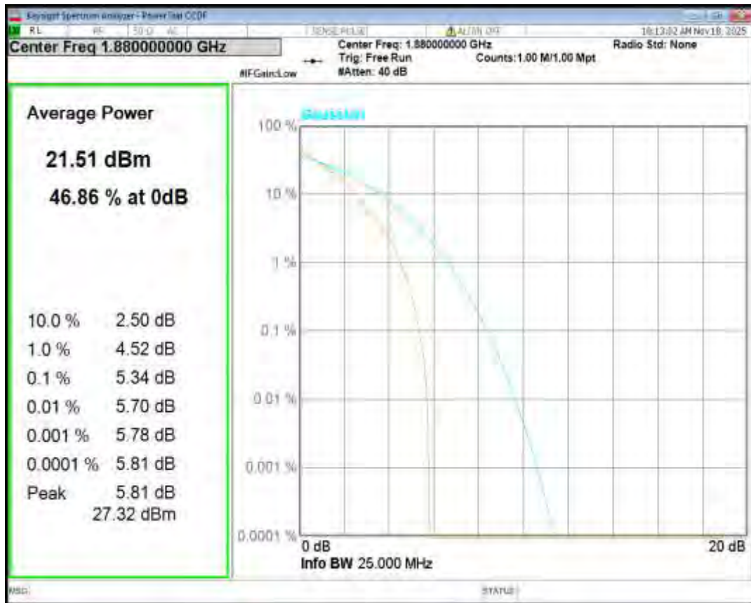
Band2 QPSK BW=10MHz Channel=19150 RB Size=1 Position=#0
