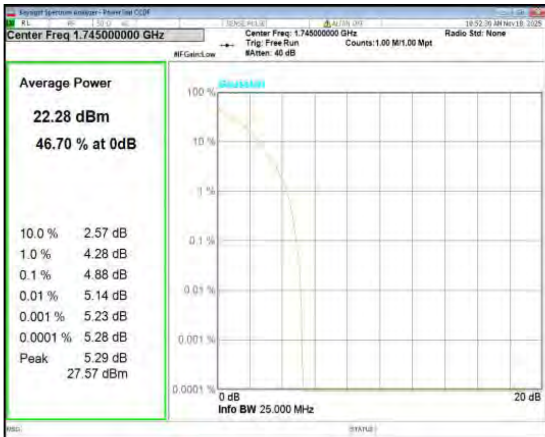
Band40(2305-2315) 16QAM BW=5MHz Channel=38725 RB Size=1 Position=#0
