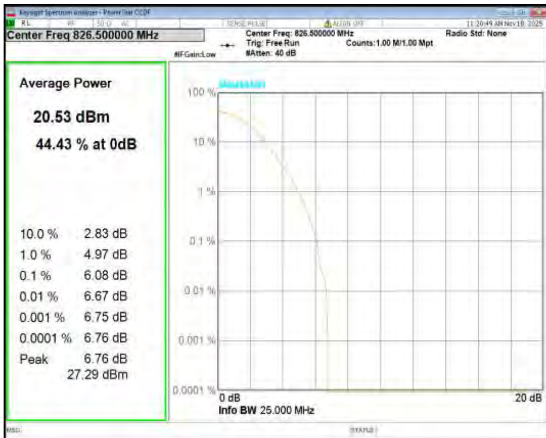
Band5 16QAM BW=5MHz Channel=20525 RB Size=1 Position=#0
