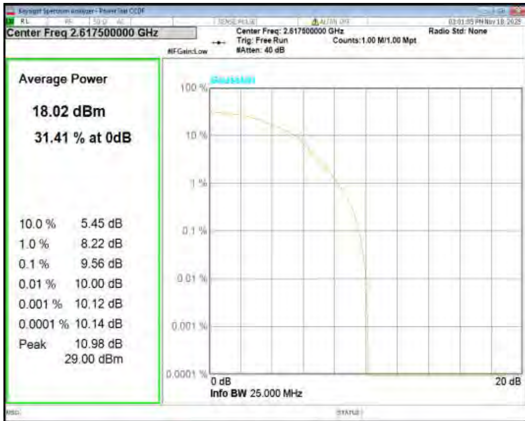
Band38 QPSK BW=5MHz Channel=37775 RB Size=1 Position=#0
