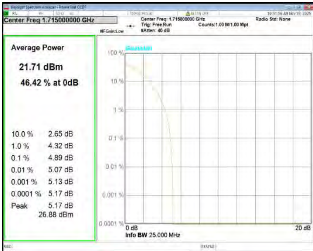
Band4 QPSK BW=10MHz Channel=20175 RB Size=1 Position=#0
