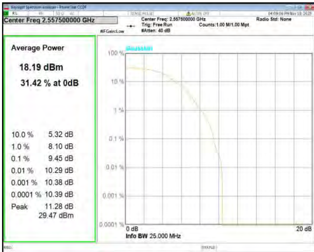
Band41(2555-2655) QPSK BW=5MHz Channel=40740 RB Size=1 Position=#0
