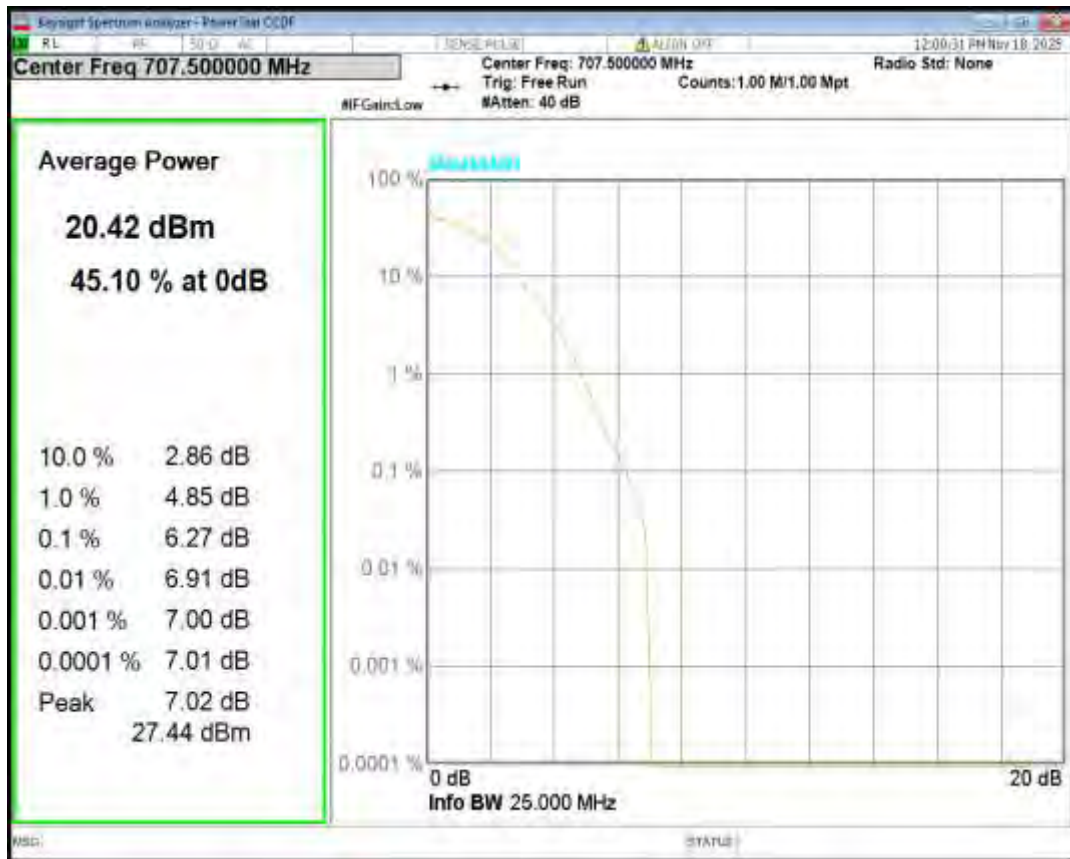
Band12 16QAM BW=1.4MHz Channel=23173 RB Size=1 Position=#0
