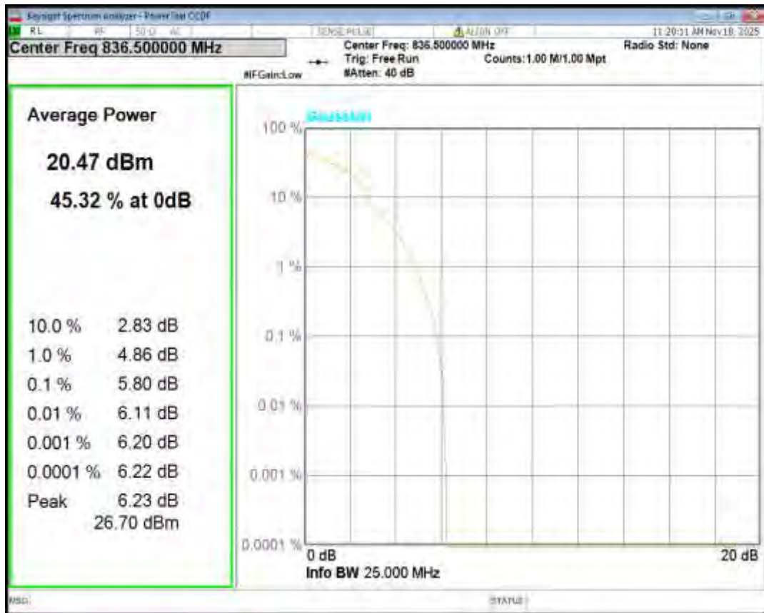
Band5 16QAM BW=1.4MHz Channel=20643 RB Size=1 Position=#0
