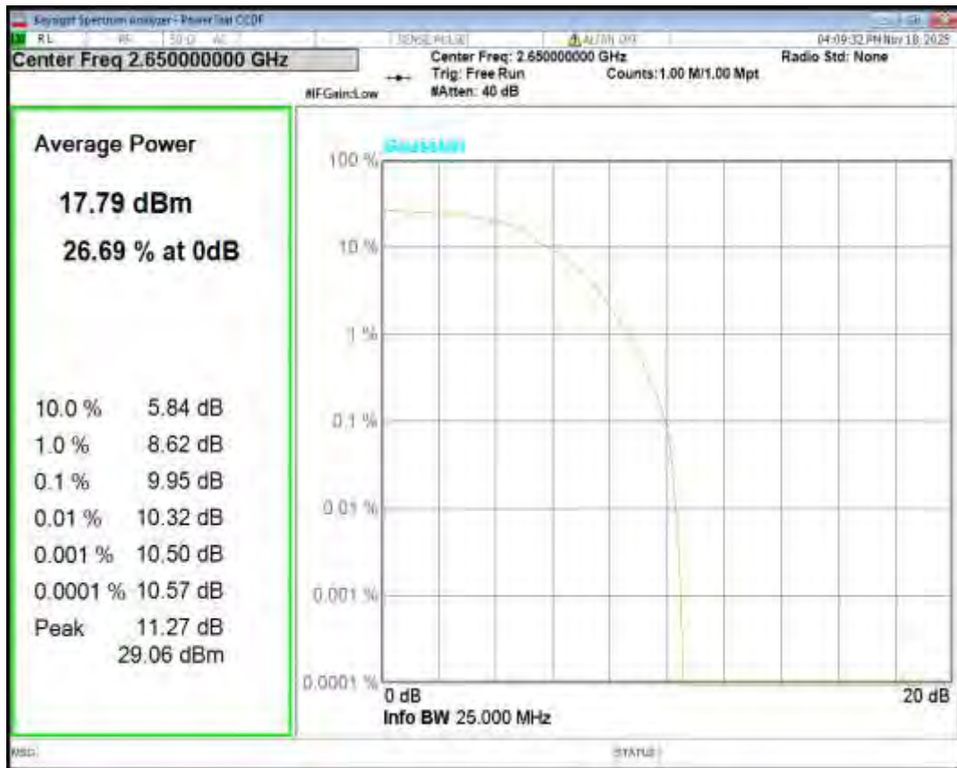
Band41(2555-2655) QPSK BW=15MHz Channel=40315 RB Size=1 Position=#0
