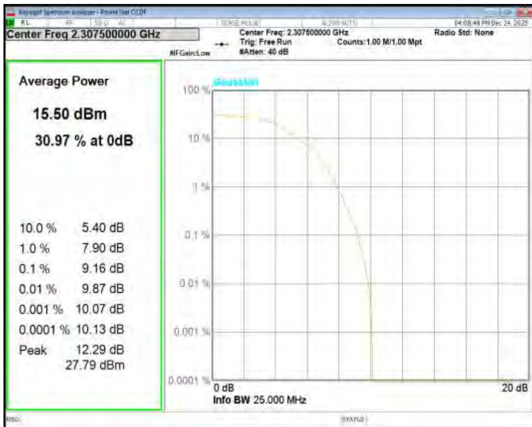
Band40(2305-2315) QPSK BW=5MHz Channel=38750 RB Size=1 Position=#0
