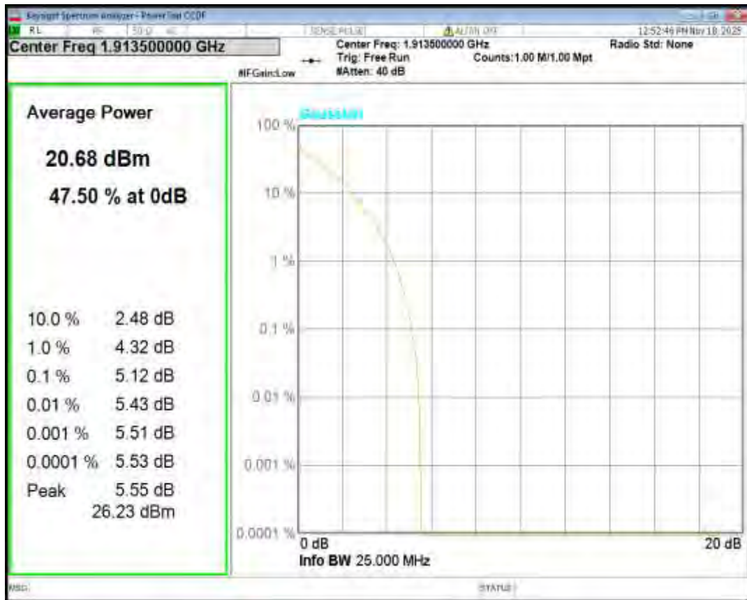
Band25 QPSK BW=5MHz Channel=26065 RB Size=1 Position=#0
