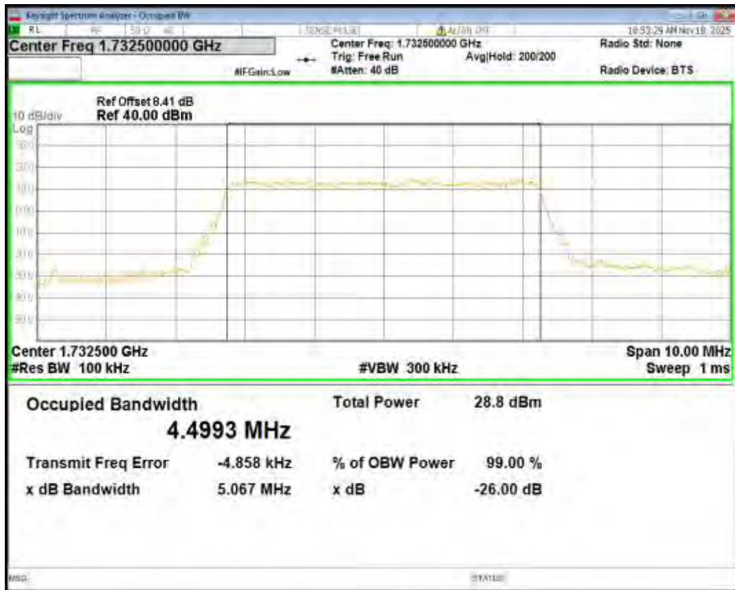
Band4 QPSK BW=5MHz Channel=20375 RB Size=25 Position=#0
