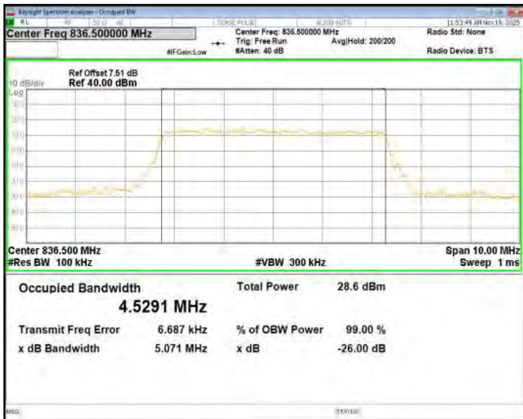
Band26(824-849) 16QAM BW=5MHz Channel=27015 RB Size=25 Position=#0
