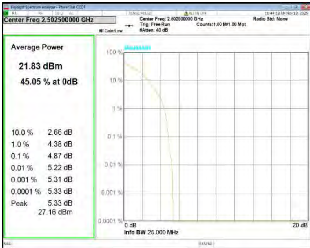
Band7 QPSK BW=5MHz Channel=21100 RB Size=1 Position=#0
