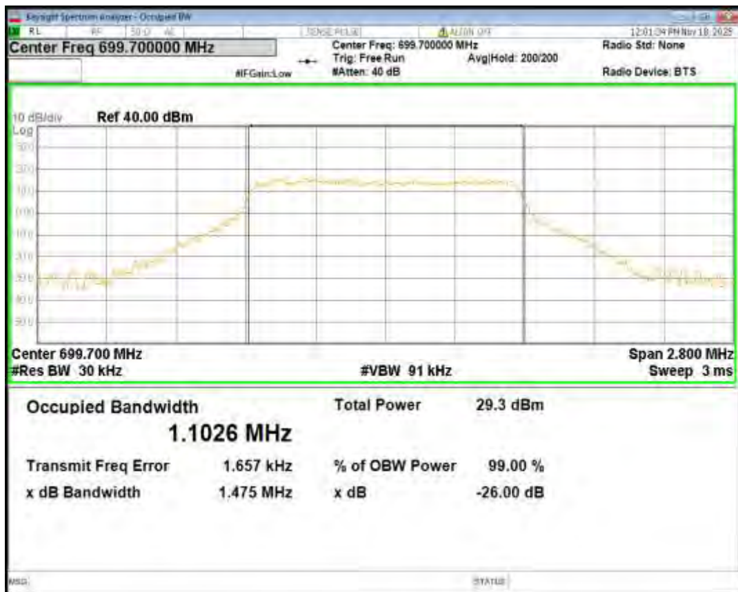
Band12 QPSK BW=1.4MHz Channel=23095 RB Size=6 Position=#0
