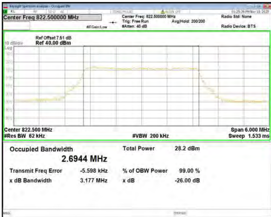
Band26(814-824) 16QAM BW=5MHz Channel=26715 RB Size=25 Position=#0
