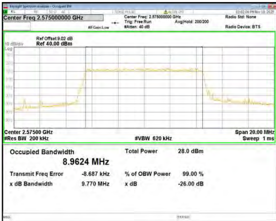
Band38 QPSK BW=10MHz Channel=38000 RB Size=50 Position=#0
