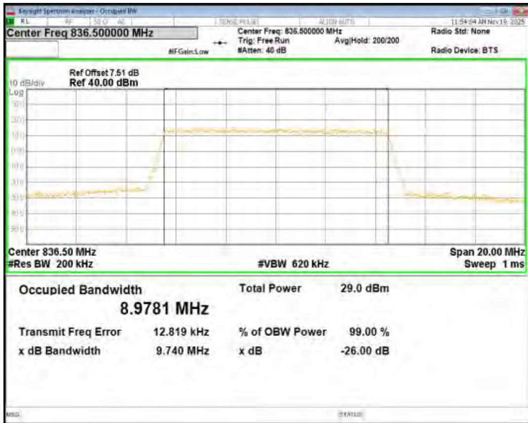
Band26(824-849) QPSK BW=10MHz Channel=26990 RB Size=50 Position=#0
