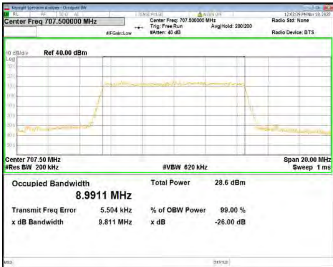
Band12 QPSK BW=10MHz Channel=23130 RB Size=50 Position=#0
