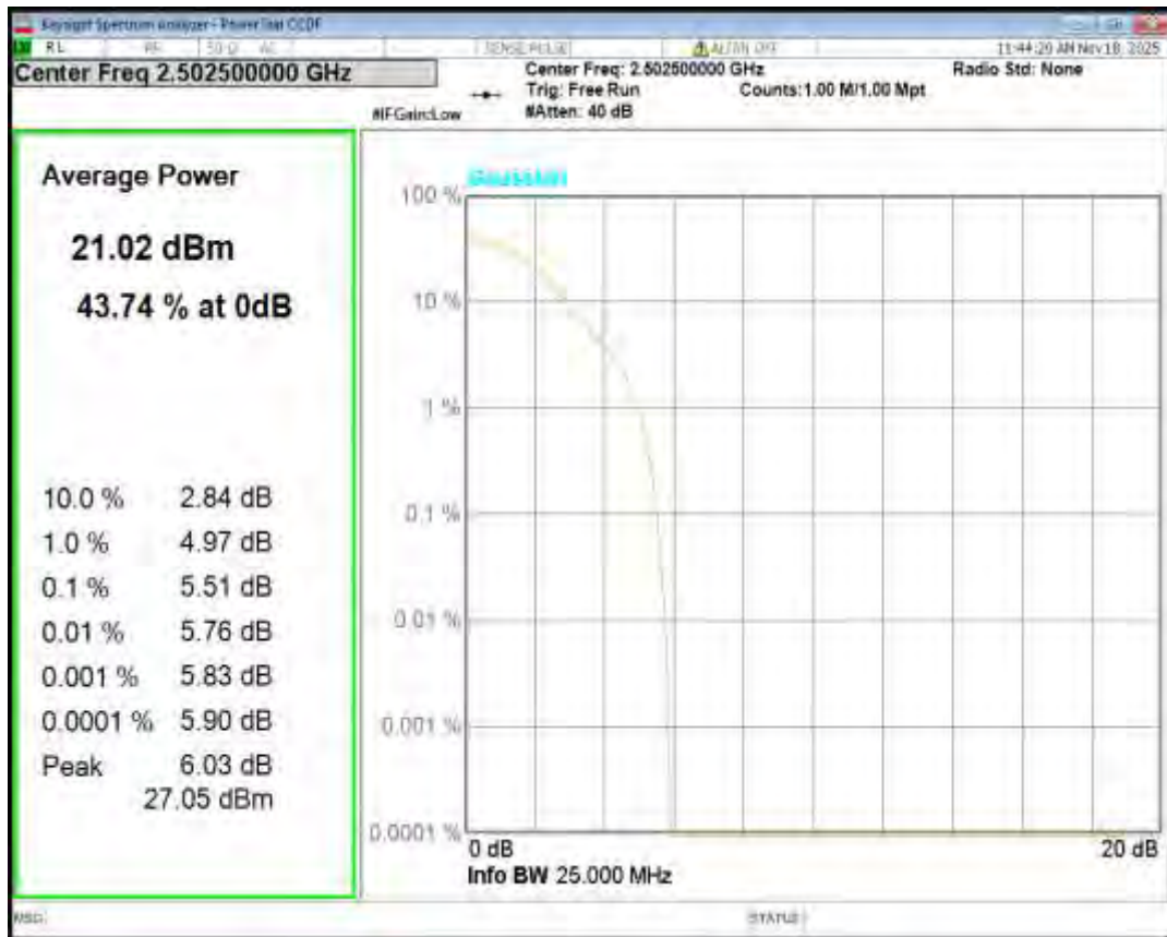
Band7 16QAM BW=5MHz Channel=21100 RB Size=1 Position=#0
