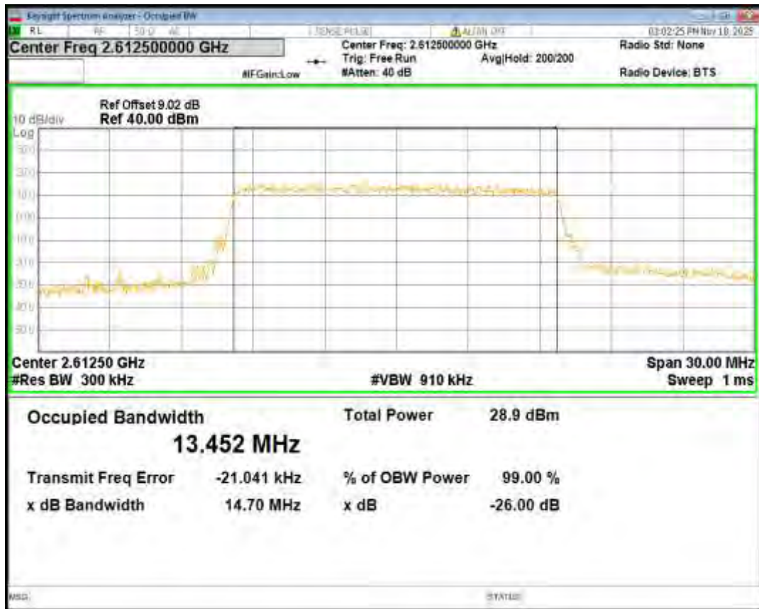
Band38 QPSK BW=20MHz Channel=37850 RB Size=100 Position=#0
