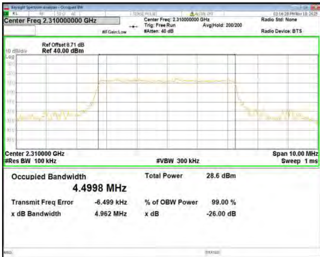
Band40(2305-2315) QPSK BW=5MHz Channel=38775 RB Size=25 Position=#0
