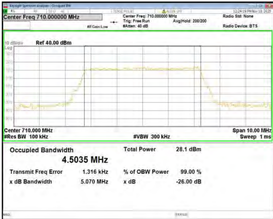
Band17 16QAM BW=5MHz Channel=23825 RB Size=25 Position=#0
