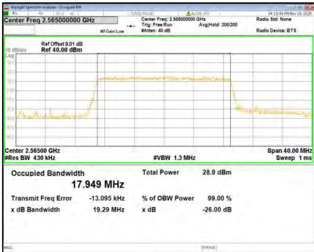
Band41(2555-2655) QPSK BW=20MHz Channel=40740 RB Size=100 Position=#0
