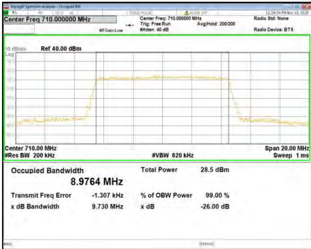
Band17 QPSK BW=10MHz Channel=23800 RB Size=50 Position=#0
