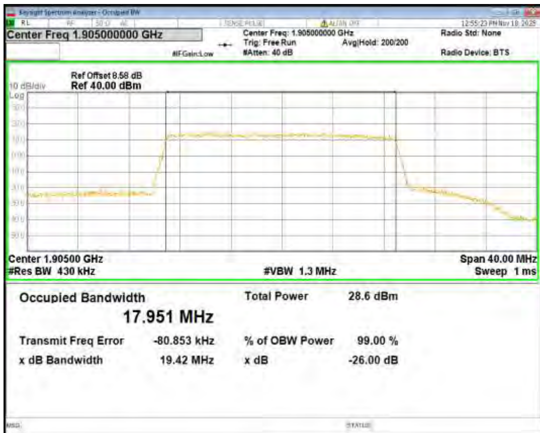
Band26(814-824) 16QAM BW=1.4MHz Channel=26697 RB Size=6 Position=#0
