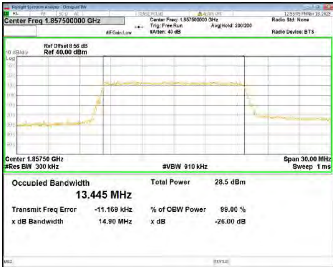
Band25 QPSK BW=15MHz Channel=26365 RB Size=75 Position=#0
