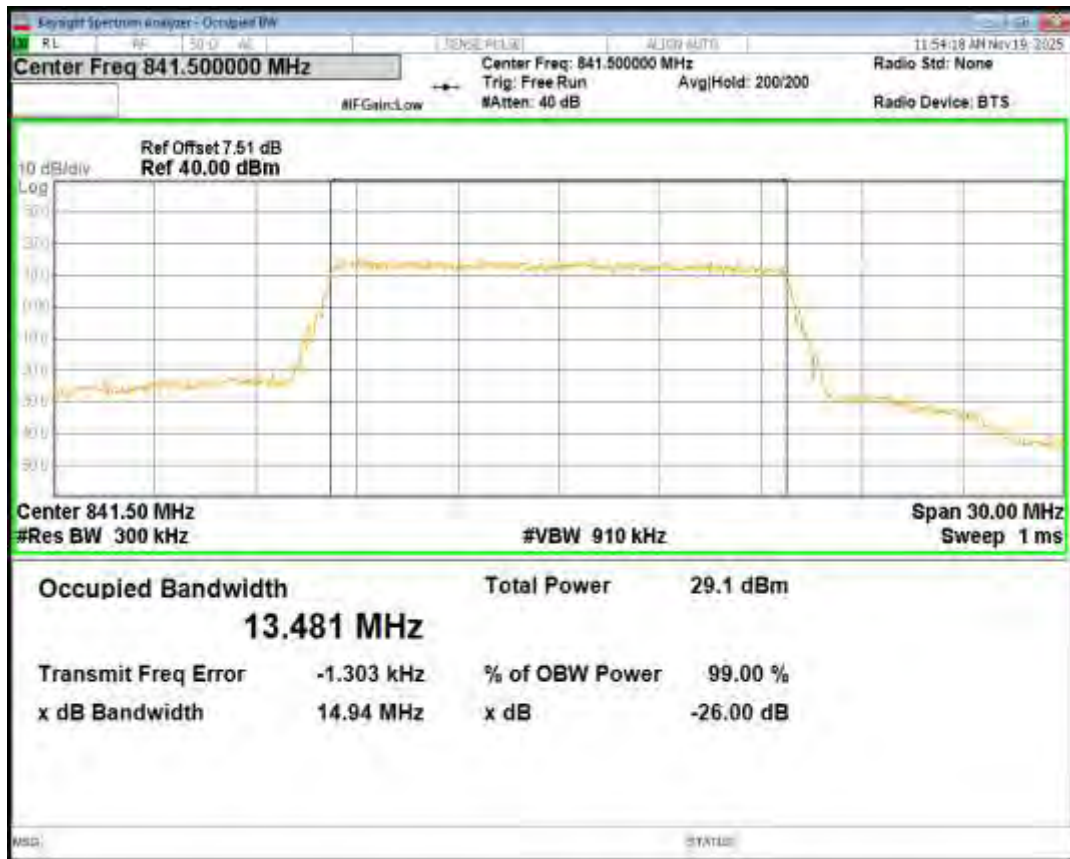
Band38 16QAM BW=5MHz Channel=37775 RB Size=25 Position=#0
