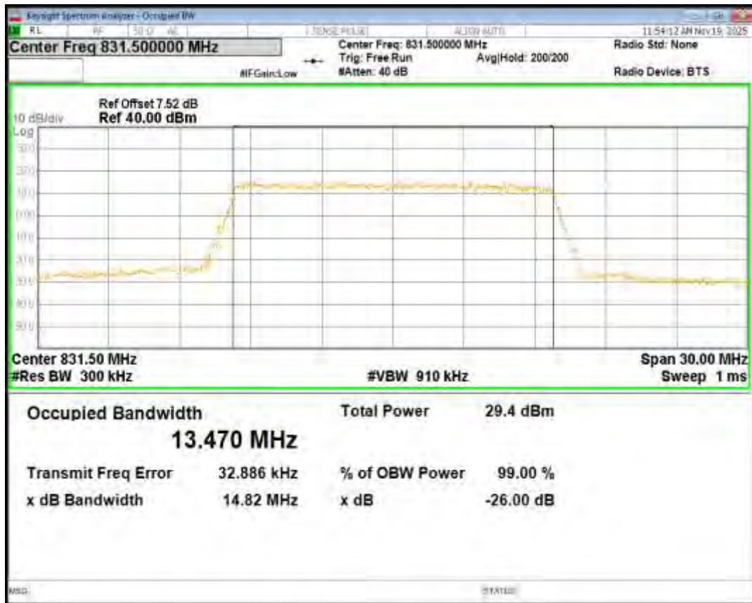
Band26(824-849) QPSK BW=15MHz Channel=26915 RB Size=75 Position=#0
