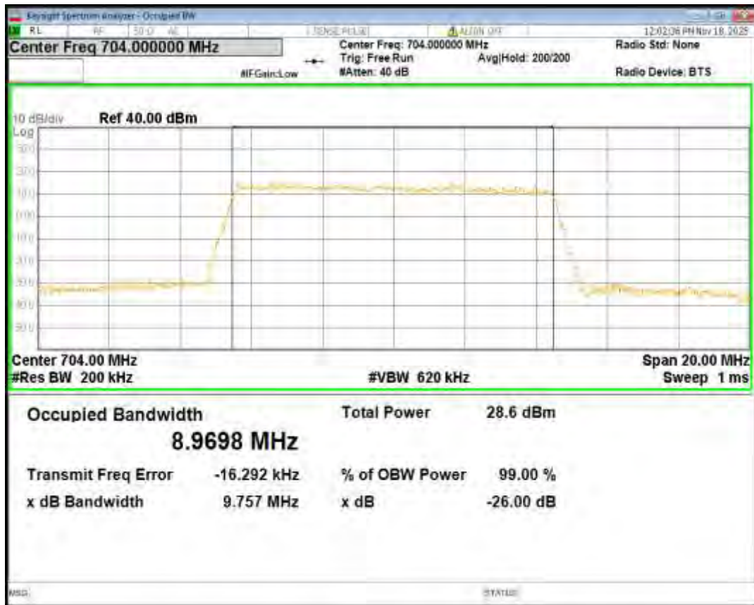
Band12 QPSK BW=10MHz Channel=23095 RB Size=50 Position=#0
