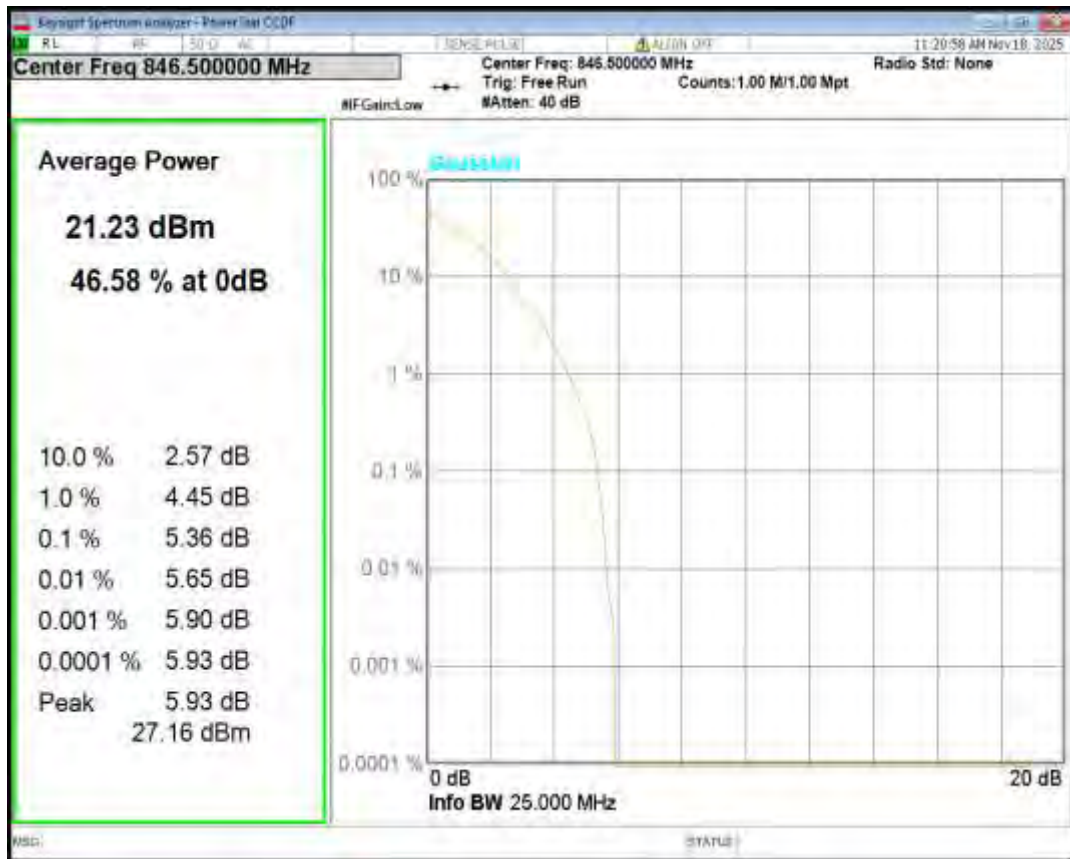
Band5 QPSK BW=10MHz Channel=20450 RB Size=1 Position=#0
