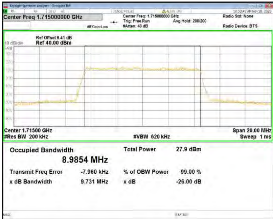
Band4 QPSK BW=10MHz Channel=20175 RB Size=50 Position=#0
