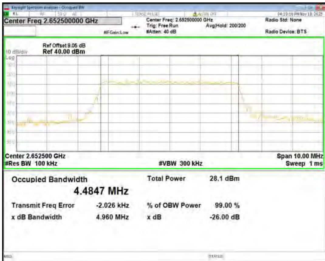
Band41(2555-2655) QPSK BW=5MHz Channel=40265 RB Size=25 Position=#0
