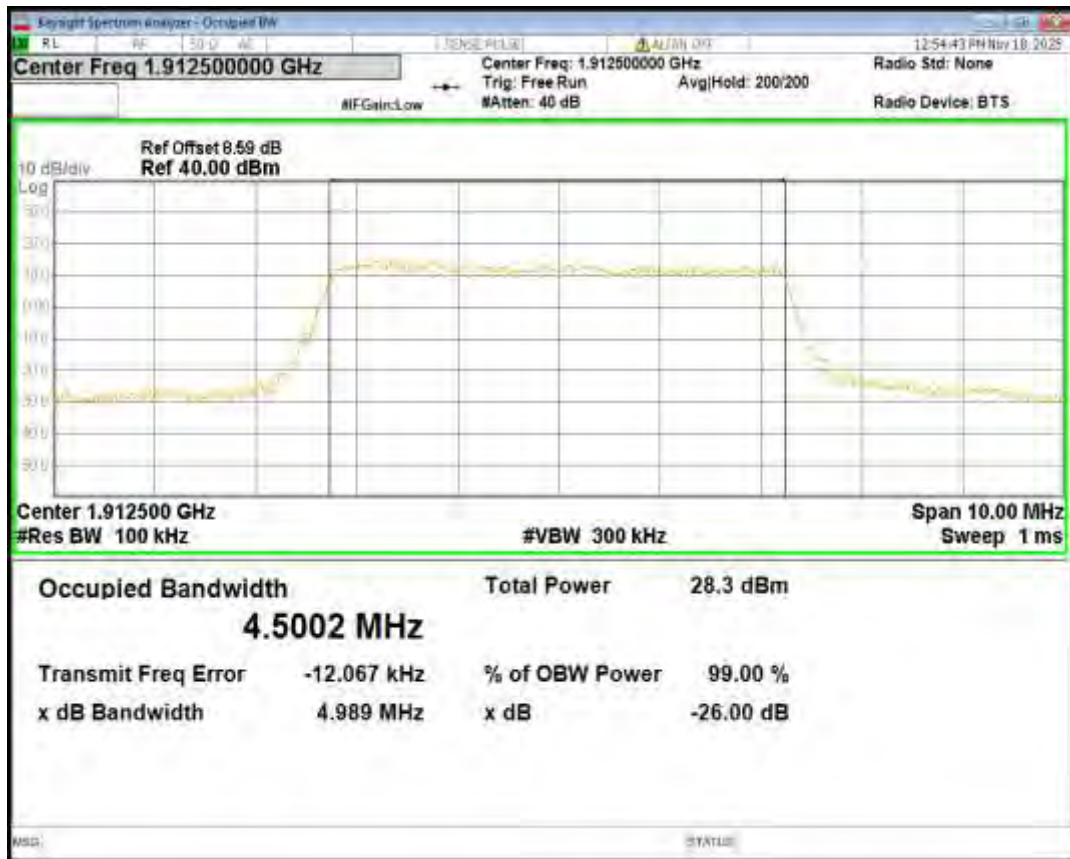
Band25 QPSK BW=10MHz Channel=26090 RB Size=50 Position=#0
