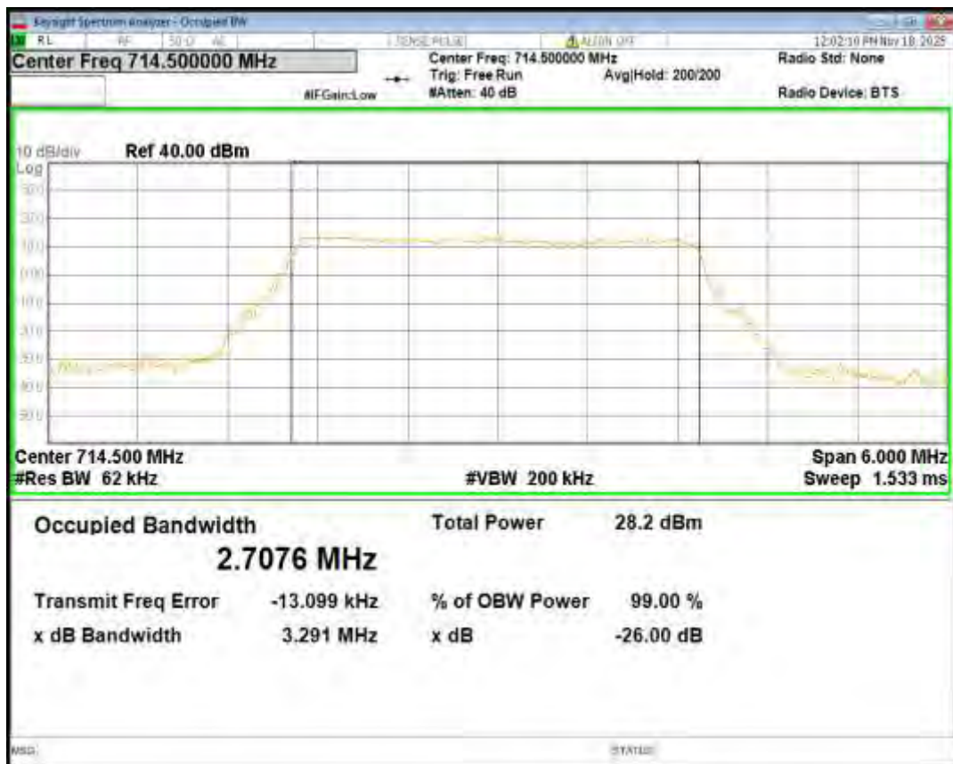
Band12 16QAM BW=5MHz Channel=23035 RB Size=25 Position=#0
