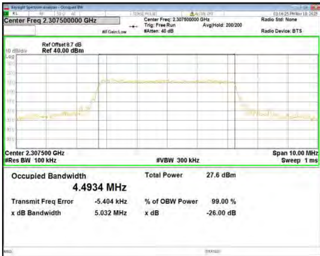
Band40(2305-2315) 16QAM BW=5MHz Channel=38750 RB Size=25 Position=#0
