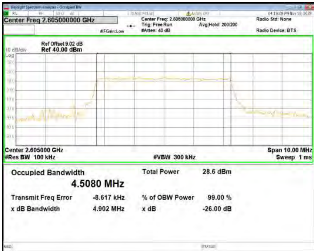
Band41(2555-2655) QPSK BW=5MHz Channel=41215 RB Size=25 Position=#0
