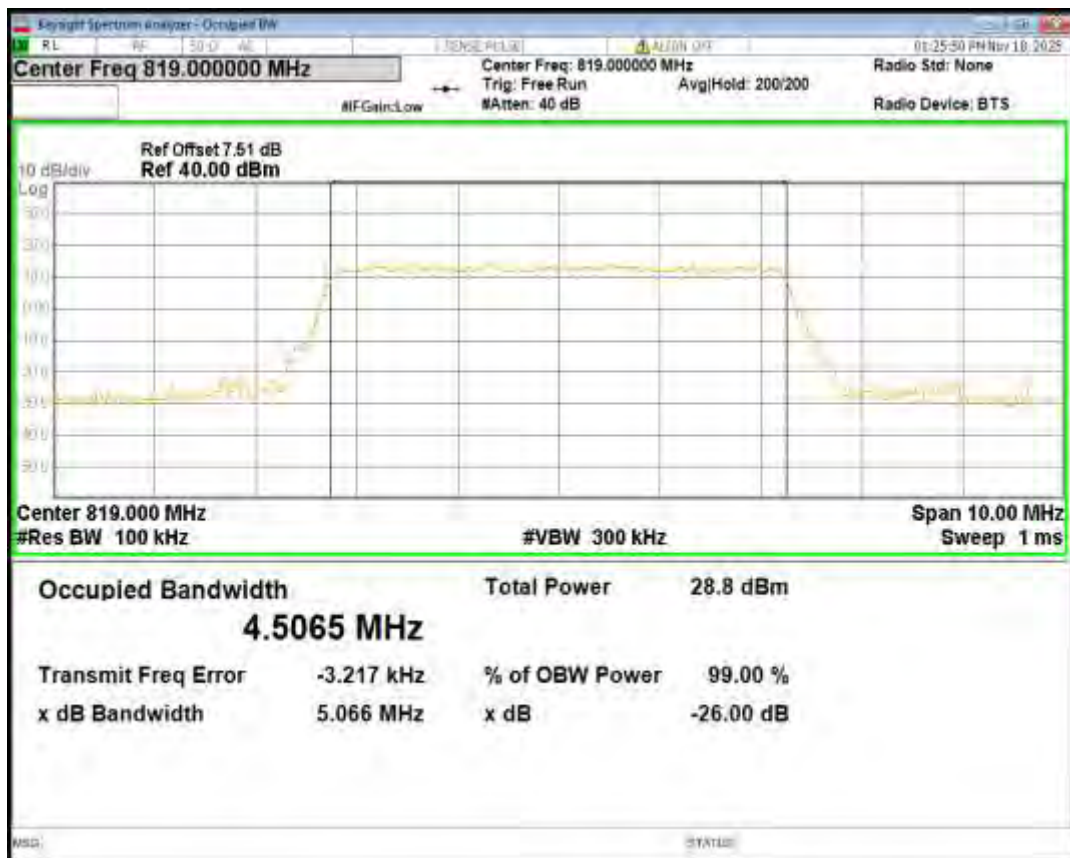
Band26(814-824) QPSK BW=5MHz Channel=26715 RB Size=25 Position=#0
