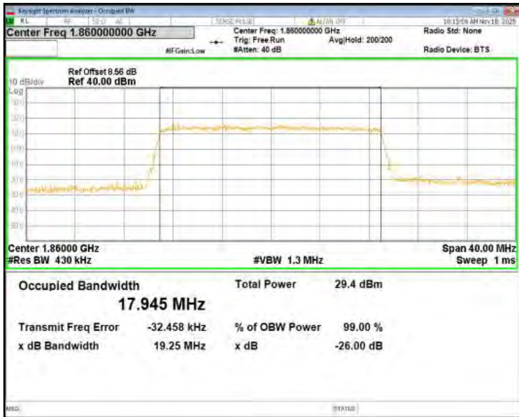
Band2 QPSK BW=20MHz Channel=18900 RB Size=100 Position=#0
