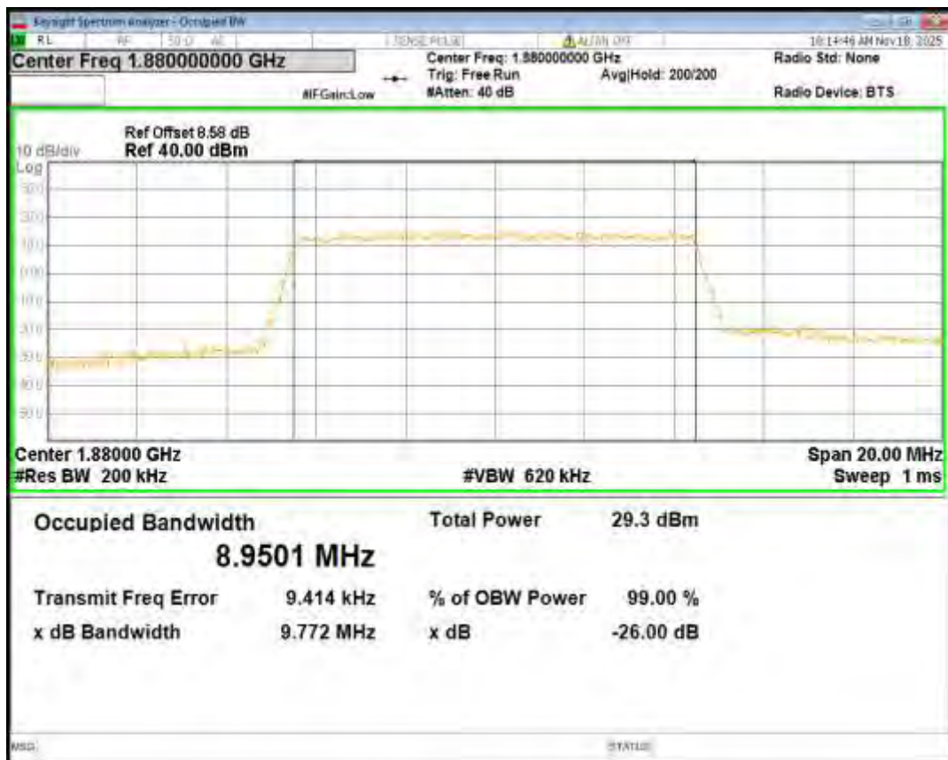
Band2 QPSK BW=10MHz Channel=19150 RB Size=50 Position=#0
