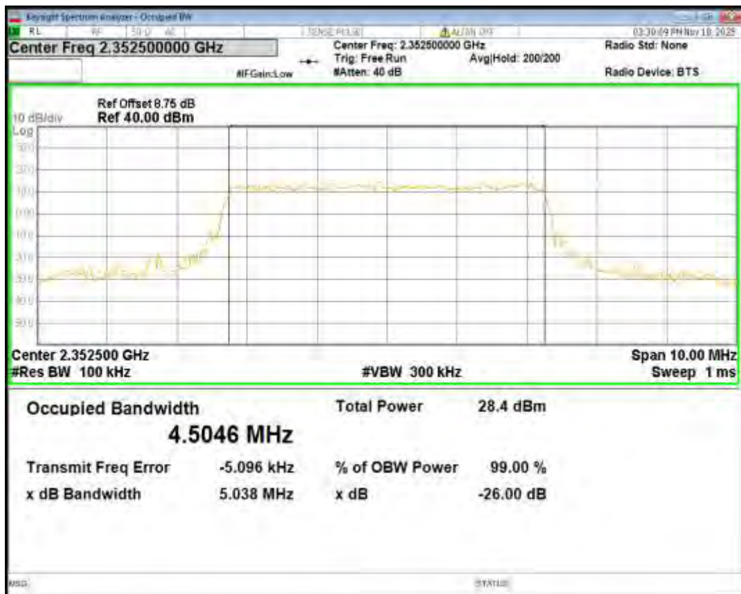
Band40(2350-2360) QPSK BW=5MHz Channel=39200 RB Size=25 Position=#0
