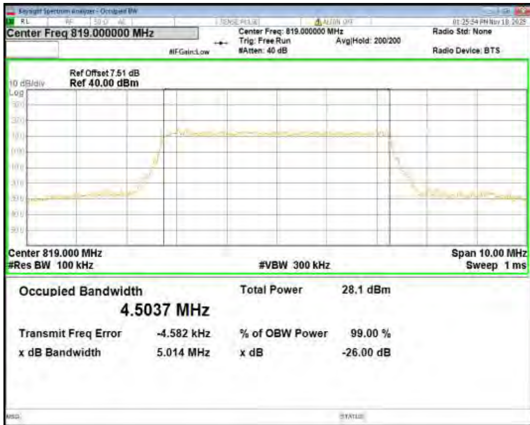
Band26(814-824) QPSK BW=1.4MHz Channel=26697 RB Size=6 Position=#0
