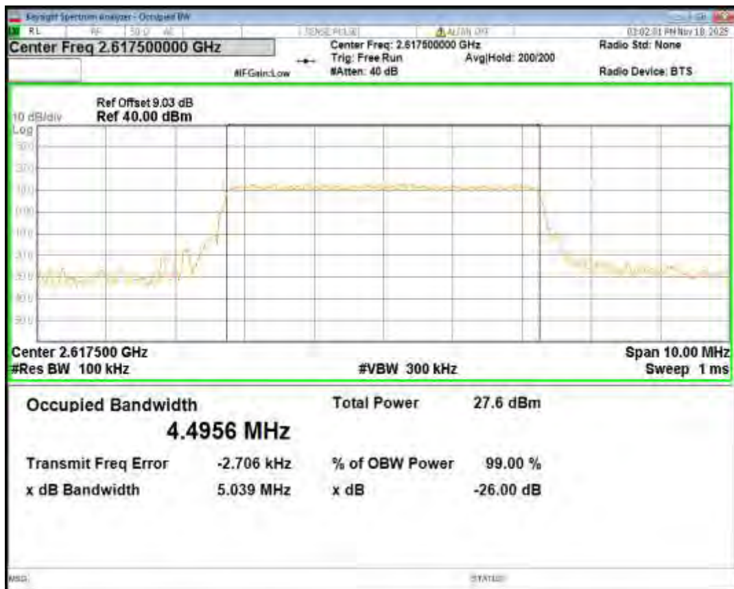
Band38 QPSK BW=5MHz Channel=37775 RB Size=25 Position=#0
