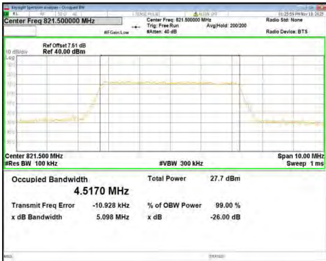
Band26(814-824) 16QAM BW=5MHz Channel=26740 RB Size=25 Position=#0
