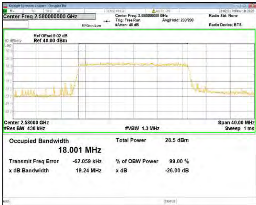
Band38 QPSK BW=20MHz Channel=38000 RB Size=100 Position=#0
