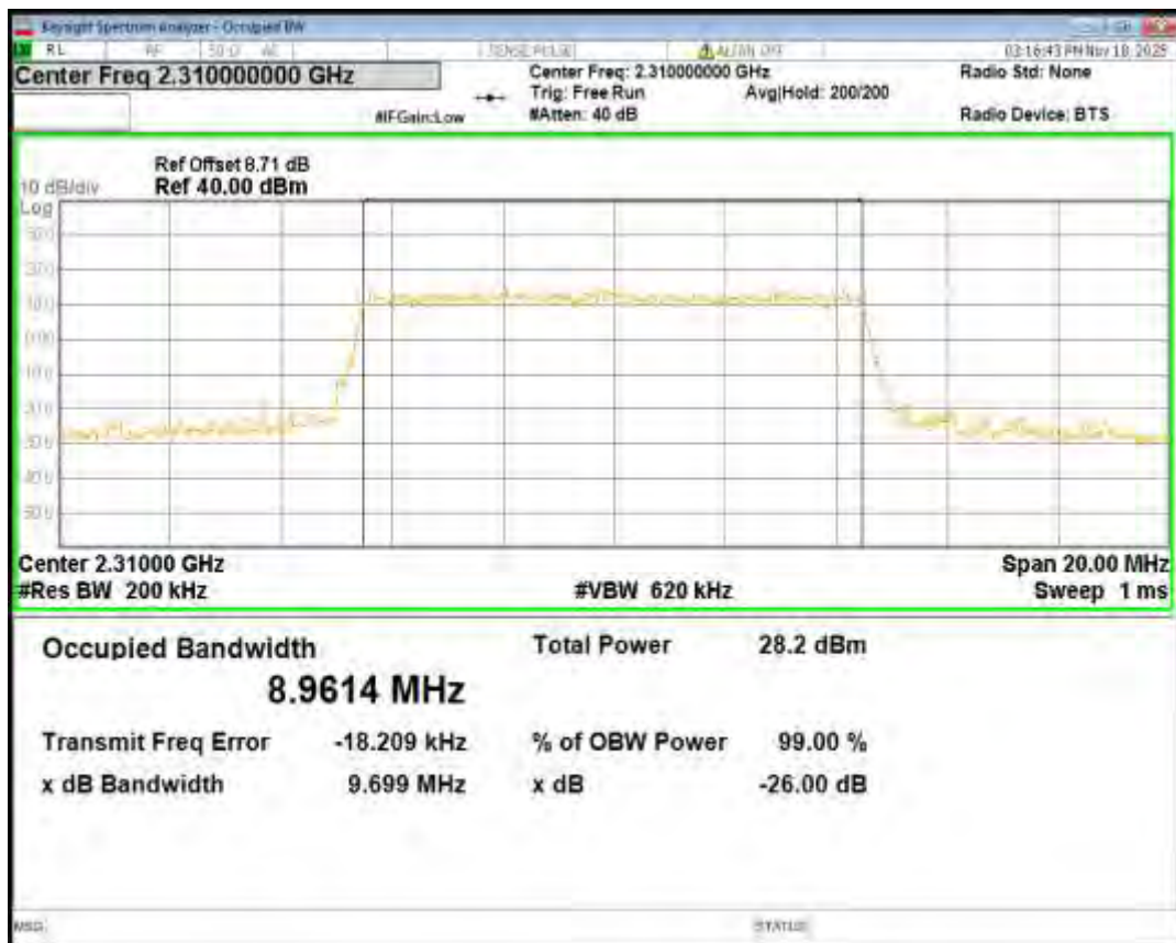
Band40(2350-2360) 16QAM BW=5MHz Channel=39175 RB Size=25 Position=#0
