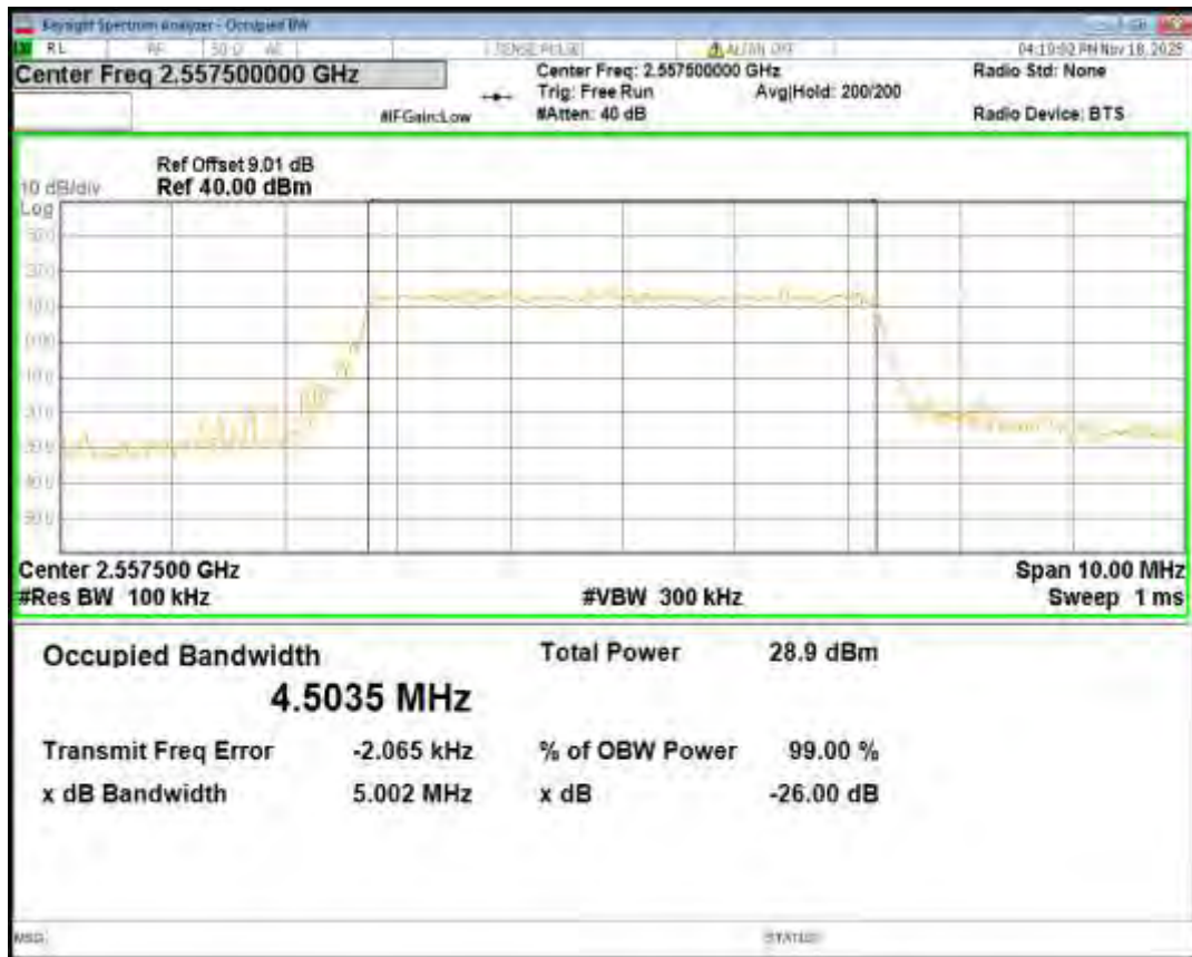
Band41(2555-2655) QPSK BW=5MHz Channel=40740 RB Size=25 Position=#0
