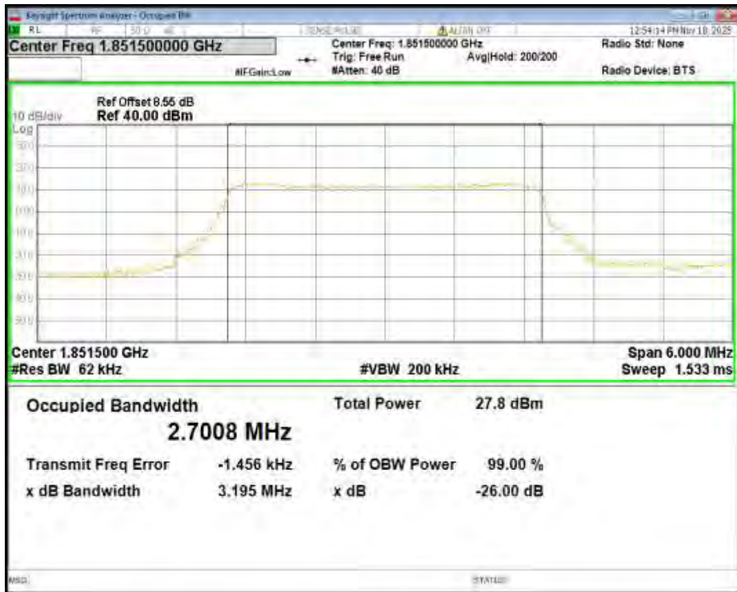
Band25 16QAM BW=3MHz Channel=26365 RB Size=15 Position=#0
