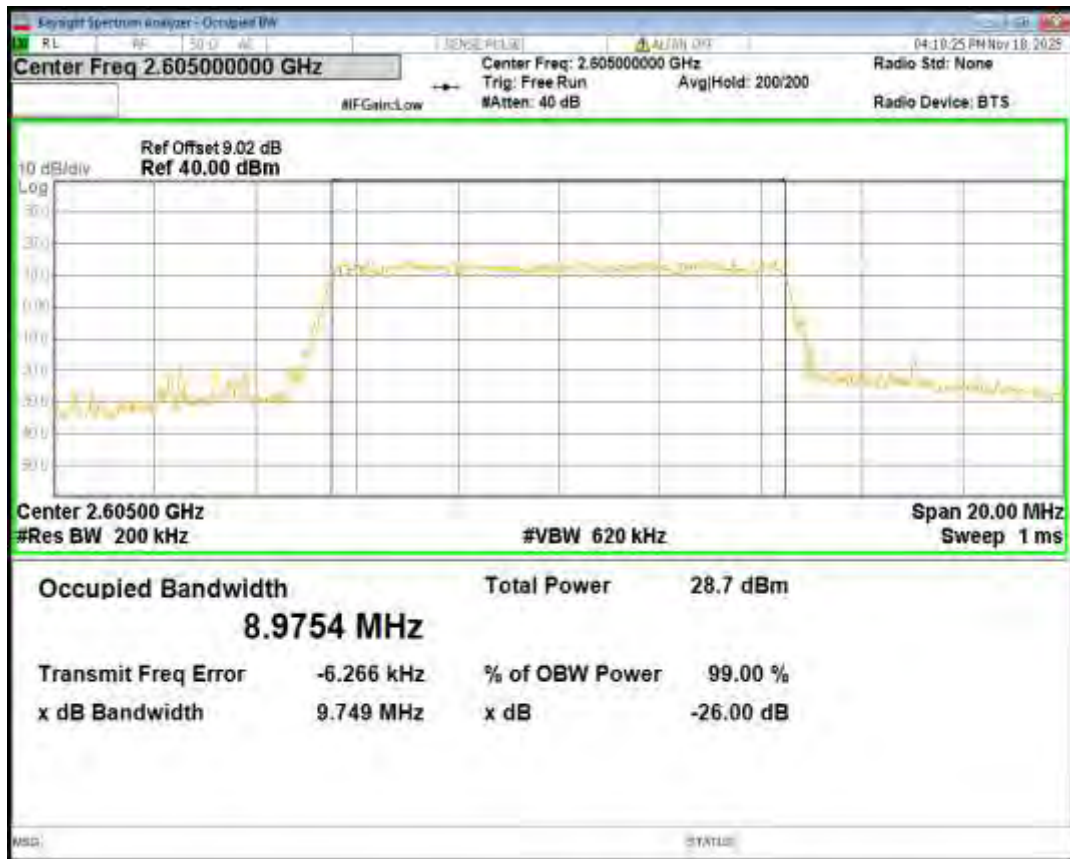
Band41(2555-2655) QPSK BW=10MHz Channel=41190 RB Size=50 Position=#0
