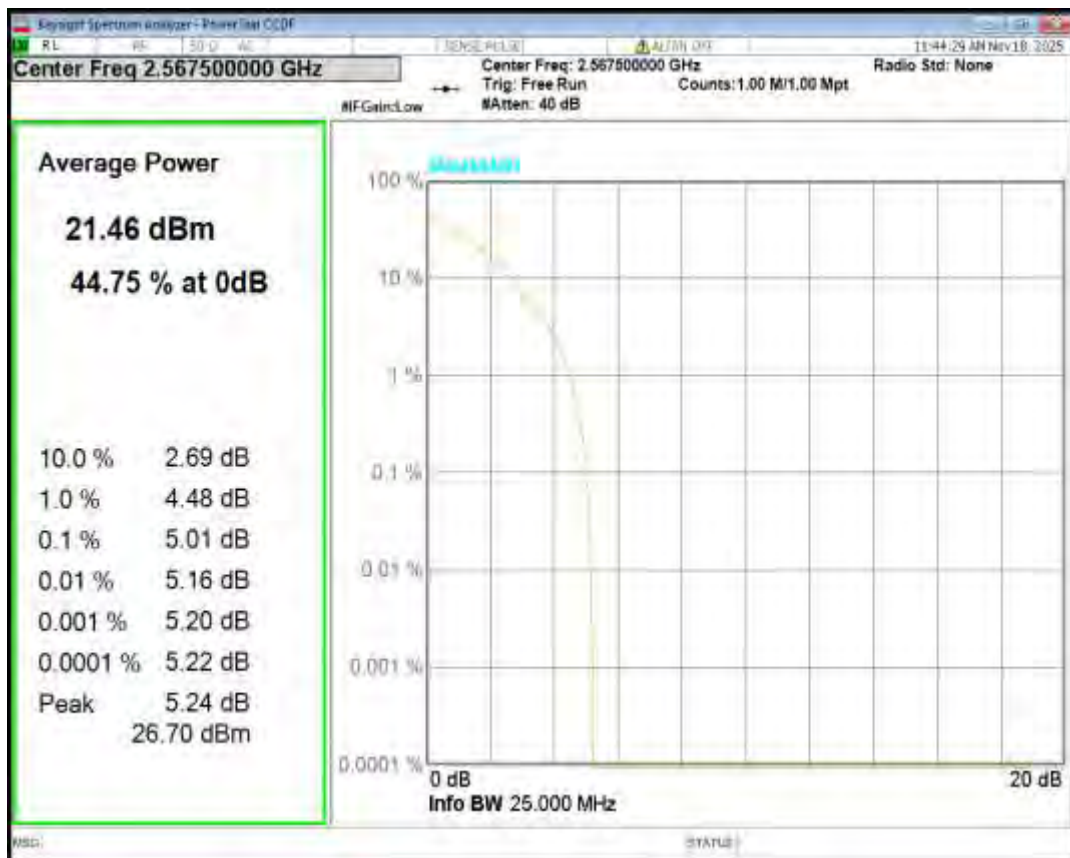
Band7 QPSK BW=10MHz Channel=20800 RB Size=1 Position=#0
