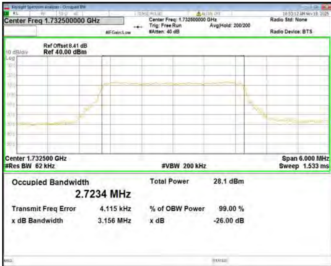
Band4 16QAM BW=3MHz Channel=20385 RB Size=15 Position=#0
