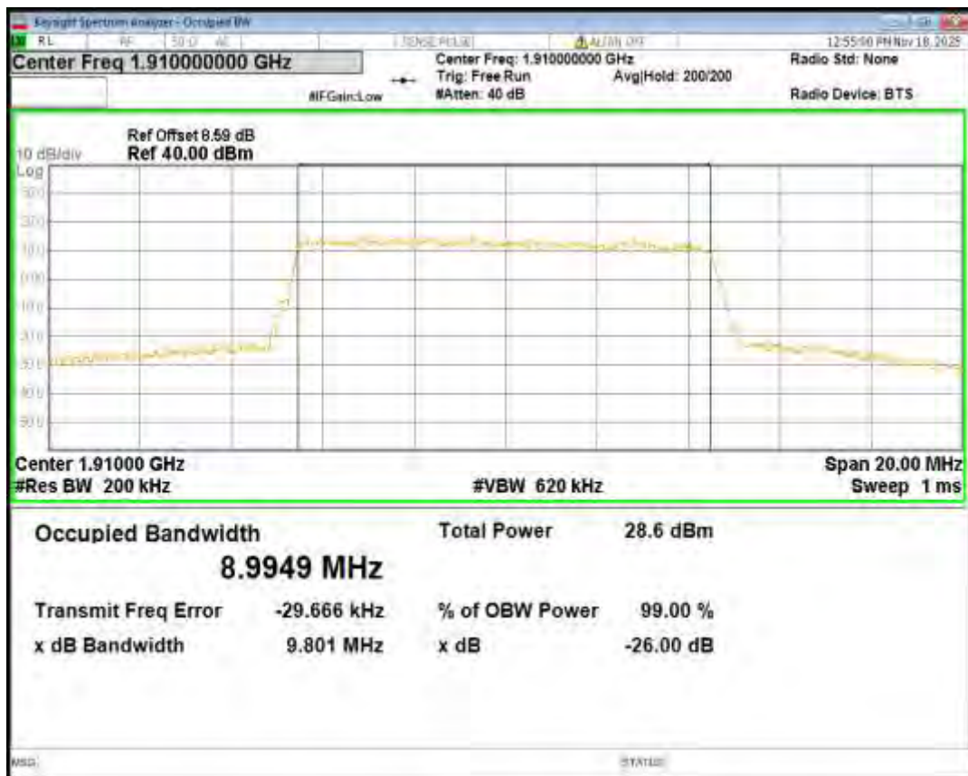
Band25 QPSK BW=15MHz Channel=26115 RB Size=75 Position=#0
