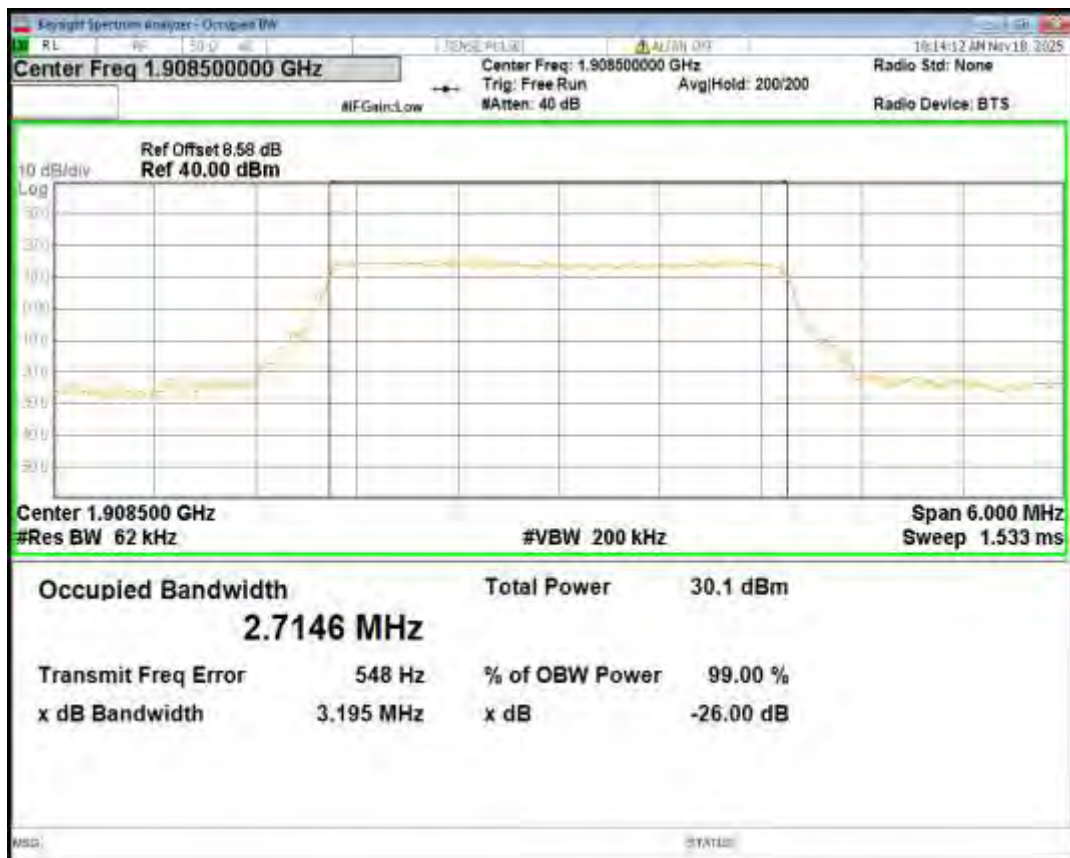
Band2 QPSK BW=5MHz Channel=18625 RB Size=25 Position=#0
