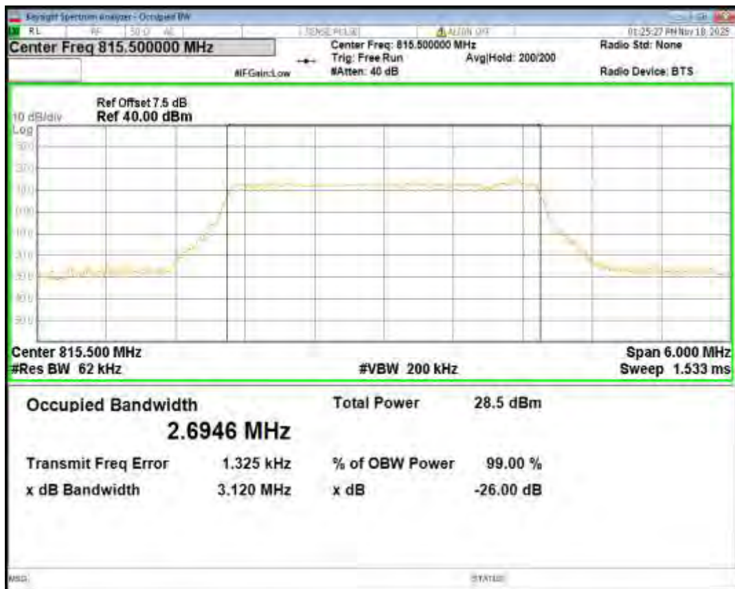
Band26(814-824) 16QAM BW=3MHz Channel=26740 RB Size=15 Position=#0
