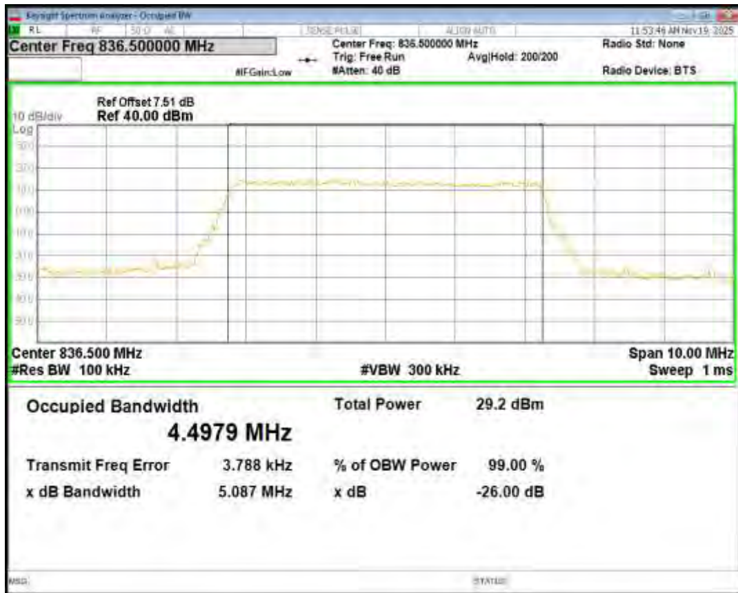
Band26(824-849) QPSK BW=5MHz Channel=26815 RB Size=25 Position=#0
