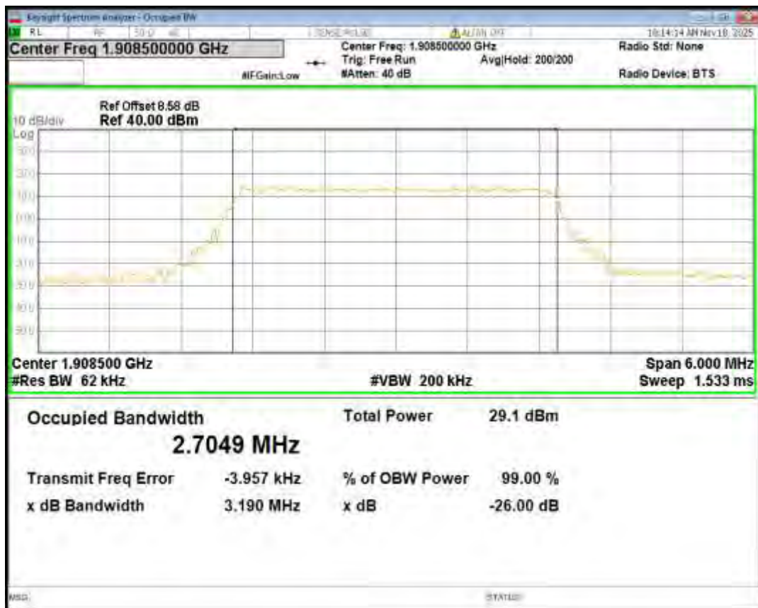
Band2 16QAM BW=5MHz Channel=18625 RB Size=25 Position=#0
