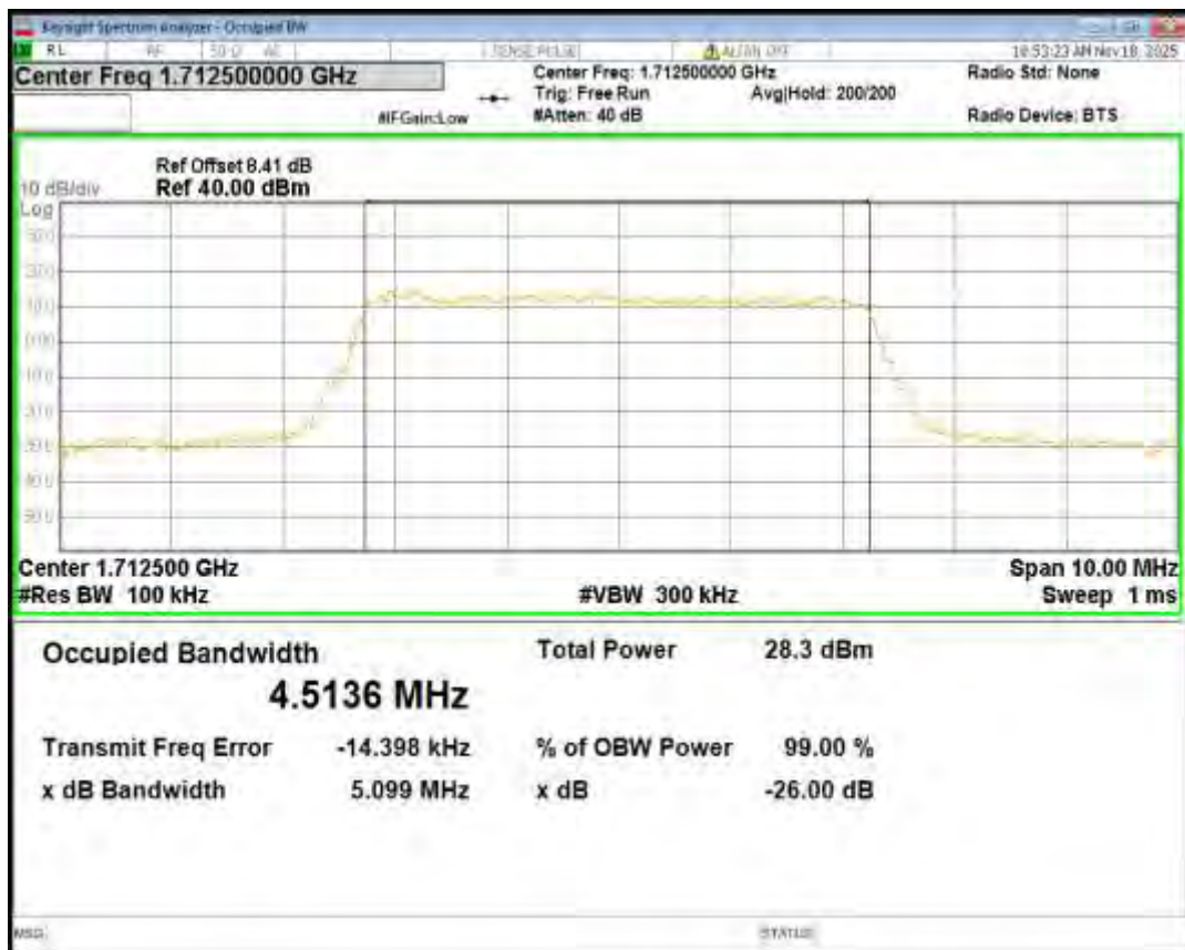
Band4 QPSK BW=5MHz Channel=20175 RB Size=25 Position=#0
