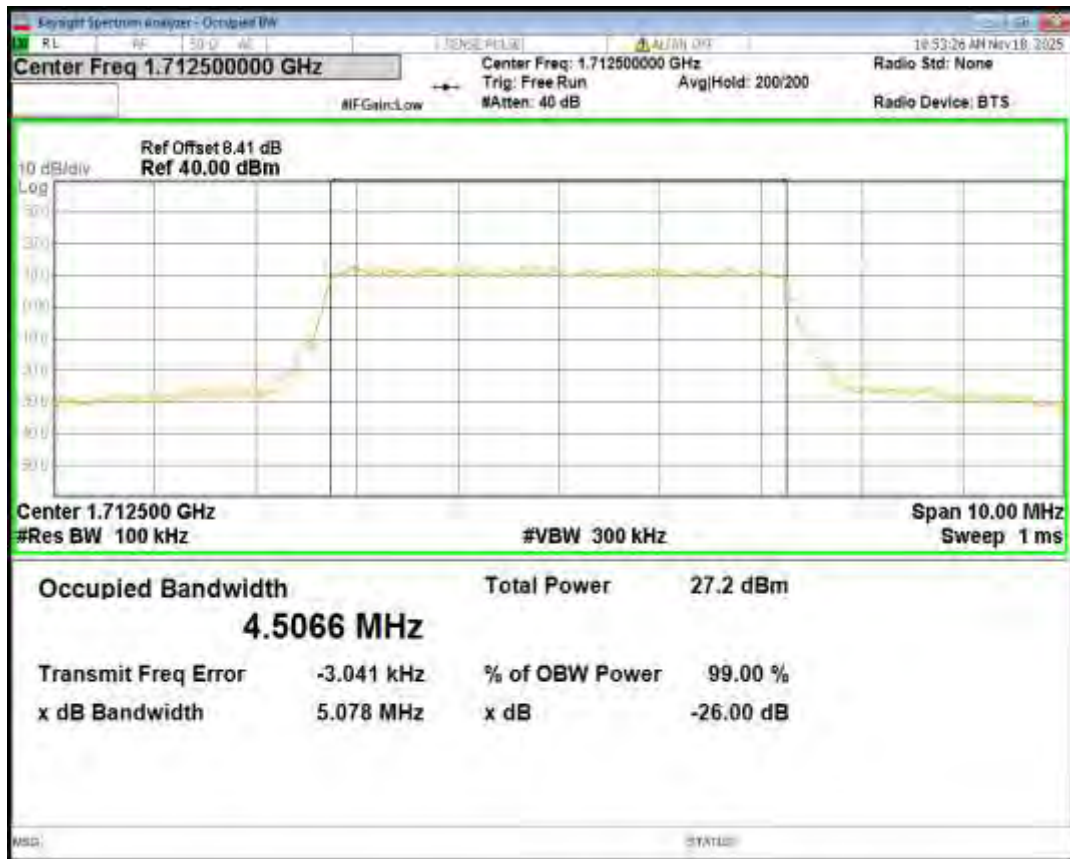
Band4 16QAM BW=5MHz Channel=20175 RB Size=25 Position=#0
