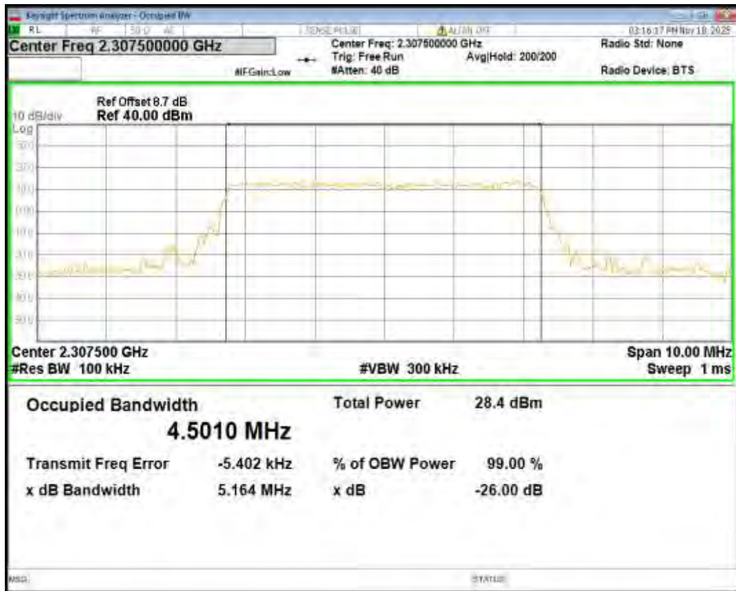
Band40(2305-2315) QPSK BW=5MHz Channel=38750 RB Size=25 Position=#0
