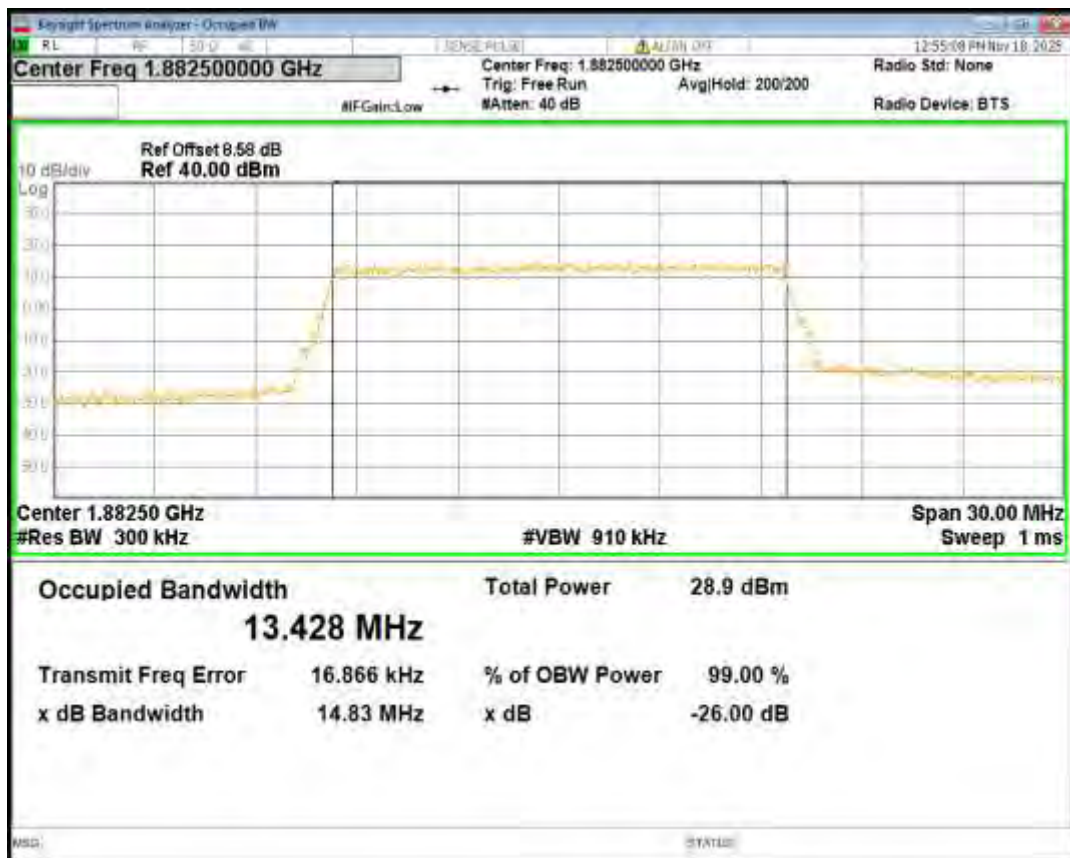
Band25 QPSK BW=15MHz Channel=26615 RB Size=75 Position=#0
