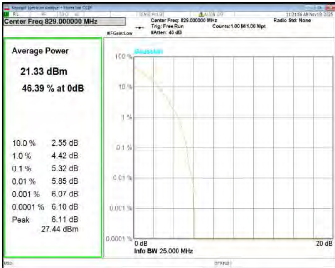
Band5 QPSK BW=10MHz Channel=20525 RB Size=1 Position=#0
