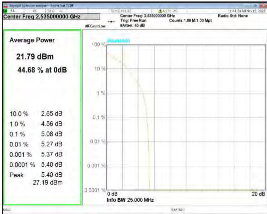
Band7 QPSK BW=5MHz Channel=21425 RB Size=1 Position=#0
