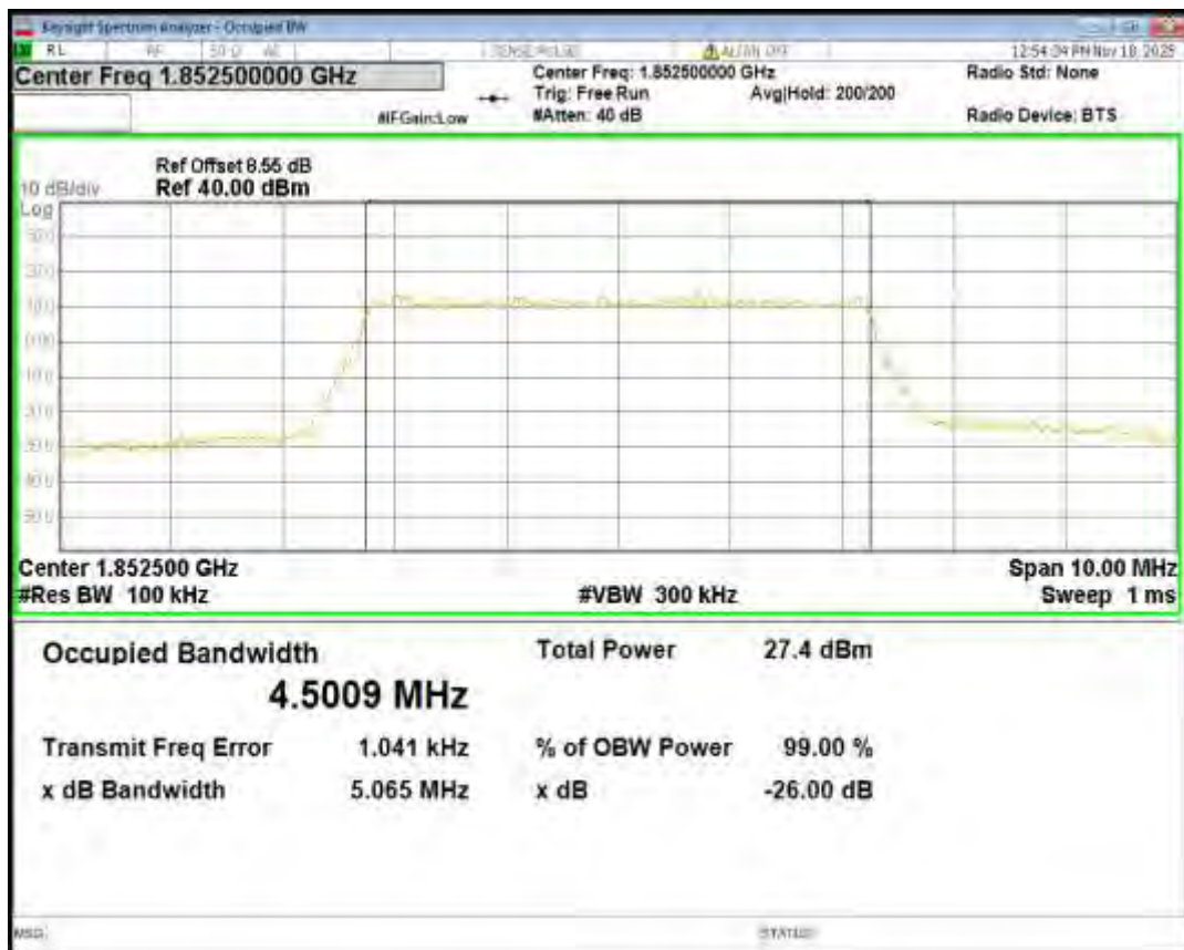
Band25 16QAM BW=5MHz Channel=26665 RB Size=25 Position=#0
