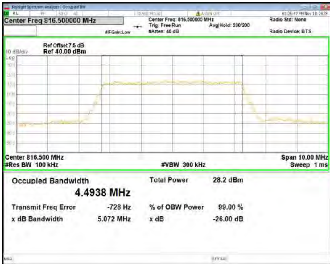
Band26(814-824) 16QAM BW=5MHz Channel=26765 RB Size=25 Position=#0
