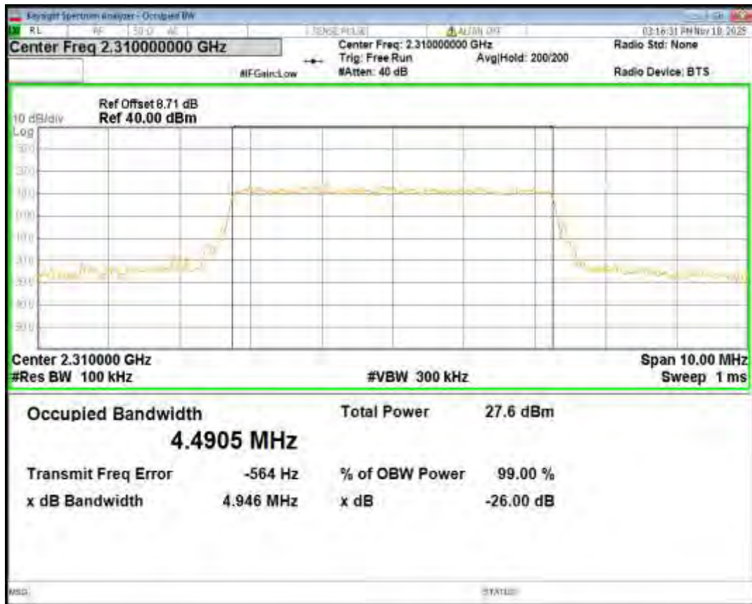
Band40(2305-2315) 16QAM BW=5MHz Channel=38775 RB Size=25 Position=#0
