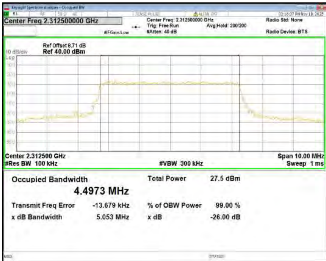
Band40(2305-2315) QPSK BW=5MHz Channel=38725 RB Size=25 Position=#0
