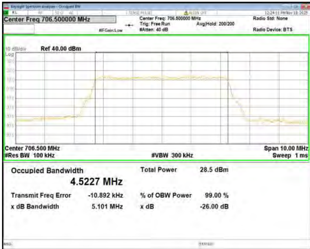
Band17 QPSK BW=5MHz Channel=23790 RB Size=25 Position=#0
