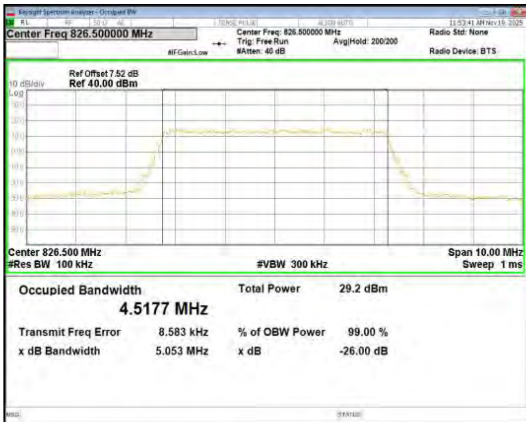
Band26(824-849) QPSK BW=5MHz Channel=27015 RB Size=25 Position=#0
