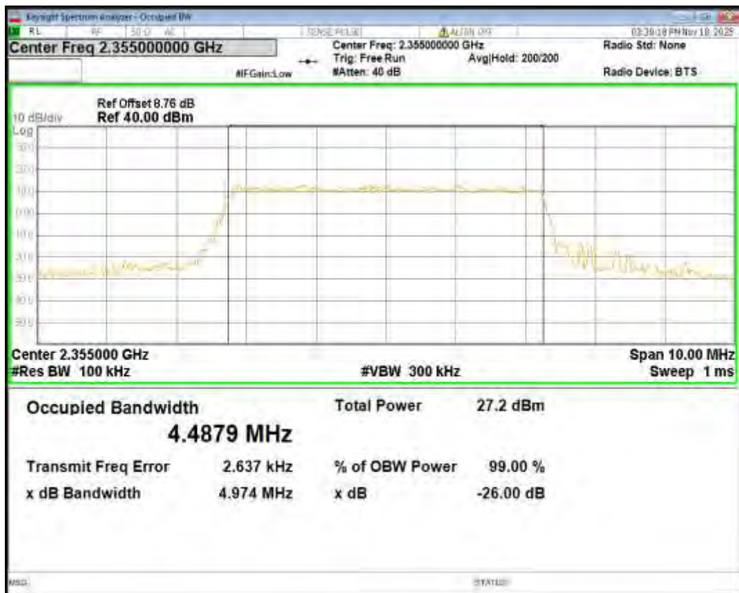
Band40(2350-2360) 16QAM BW=5MHz Channel=39225 RB Size=25 Position=#0
