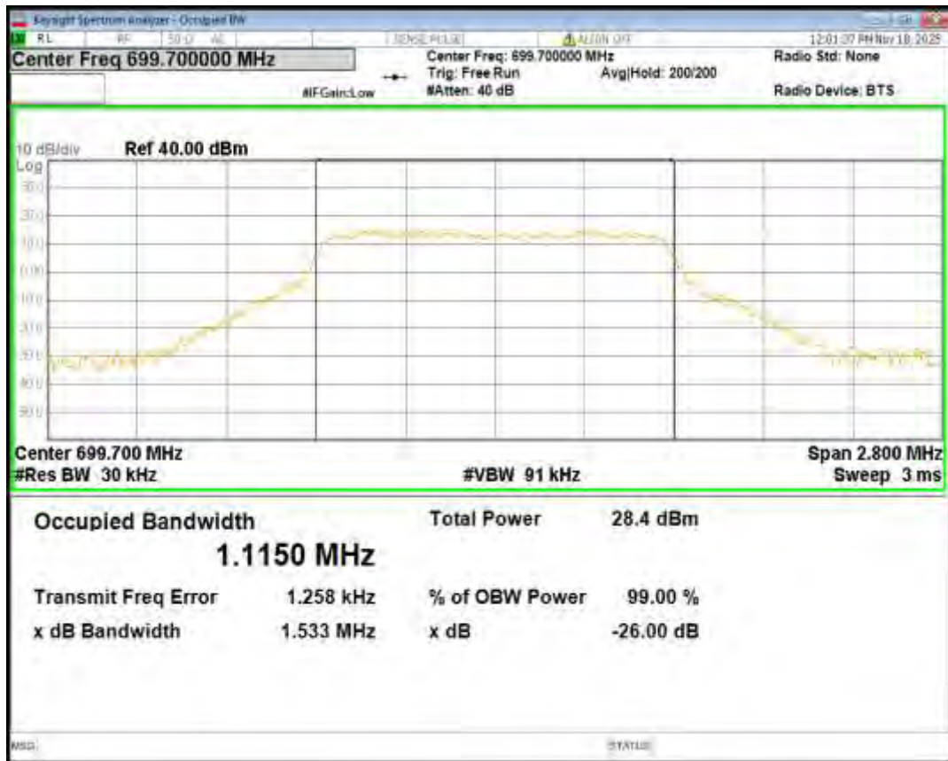
Band12 16QAM BW=1.4MHz Channel=23095 RB Size=6 Position=#0
