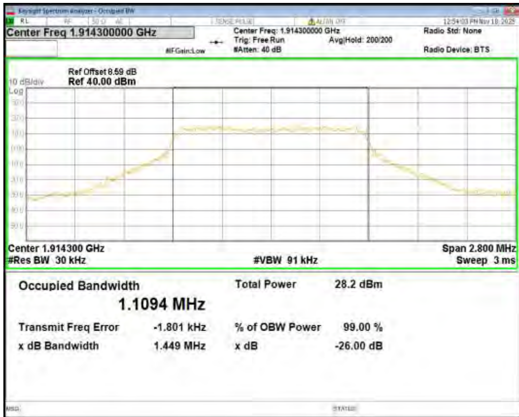
Band25 QPSK BW=3MHz Channel=26055 RB Size=15 Position=#0
