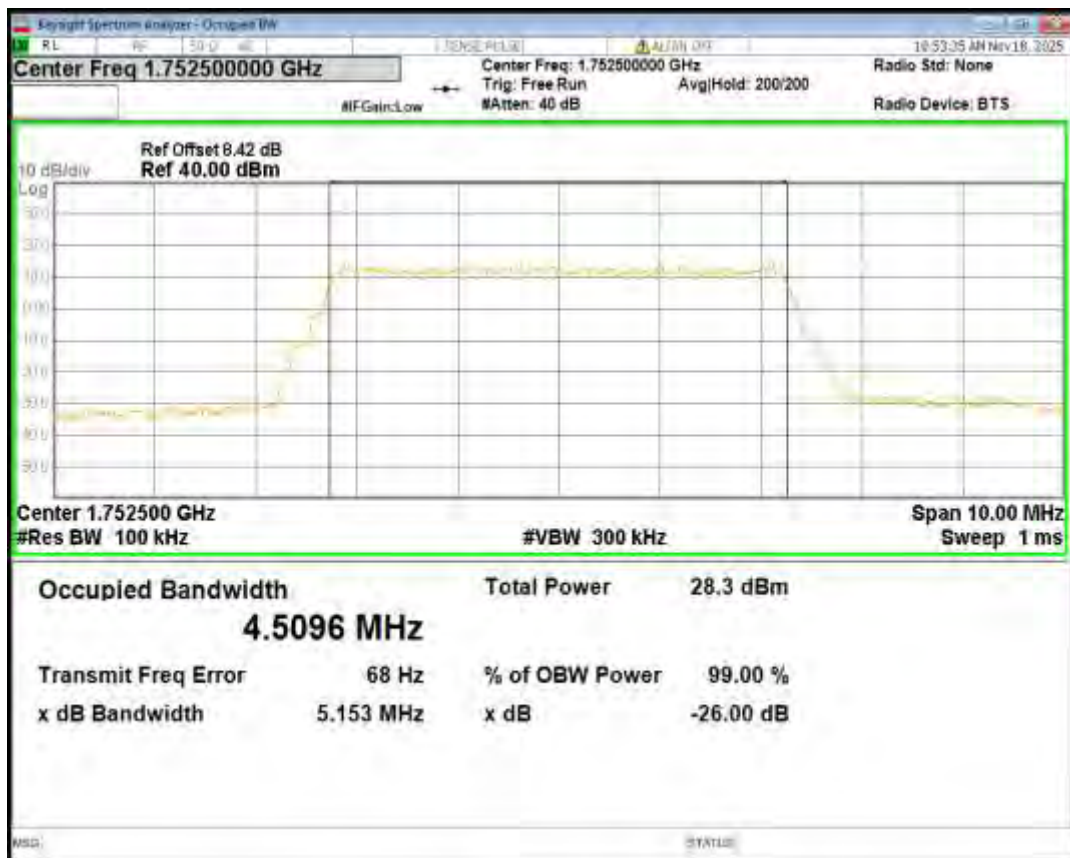
Band4 QPSK BW=10MHz Channel=20000 RB Size=50 Position=#0
