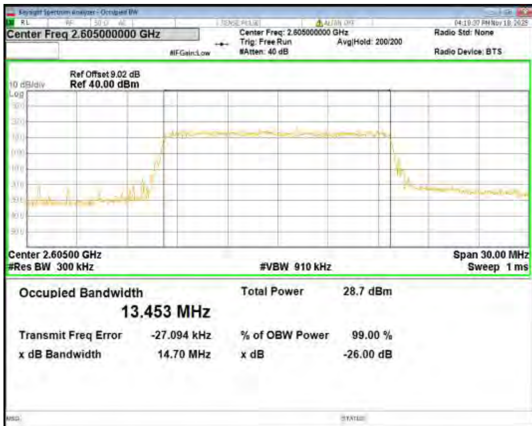
Band41(2555-2655) QPSK BW=15MHz Channel=41165 RB Size=75 Position=#0
