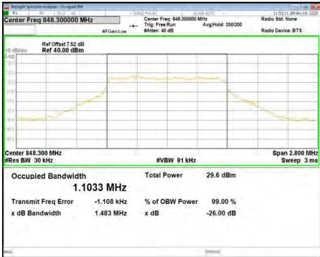
Band26(824-849) QPSK BW=3MHz Channel=26805 RB Size=15 Position=#0
