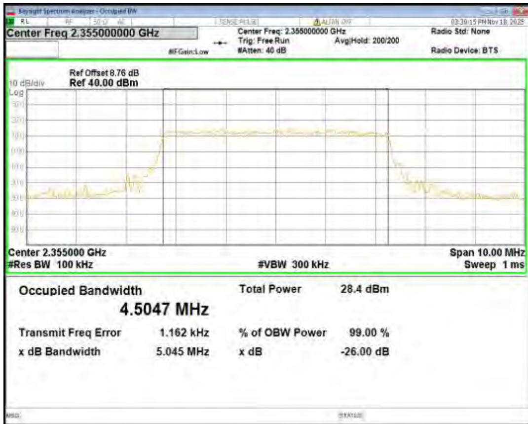
Band40(2350-2360) QPSK BW=5MHz Channel=39225 RB Size=25 Position=#0
