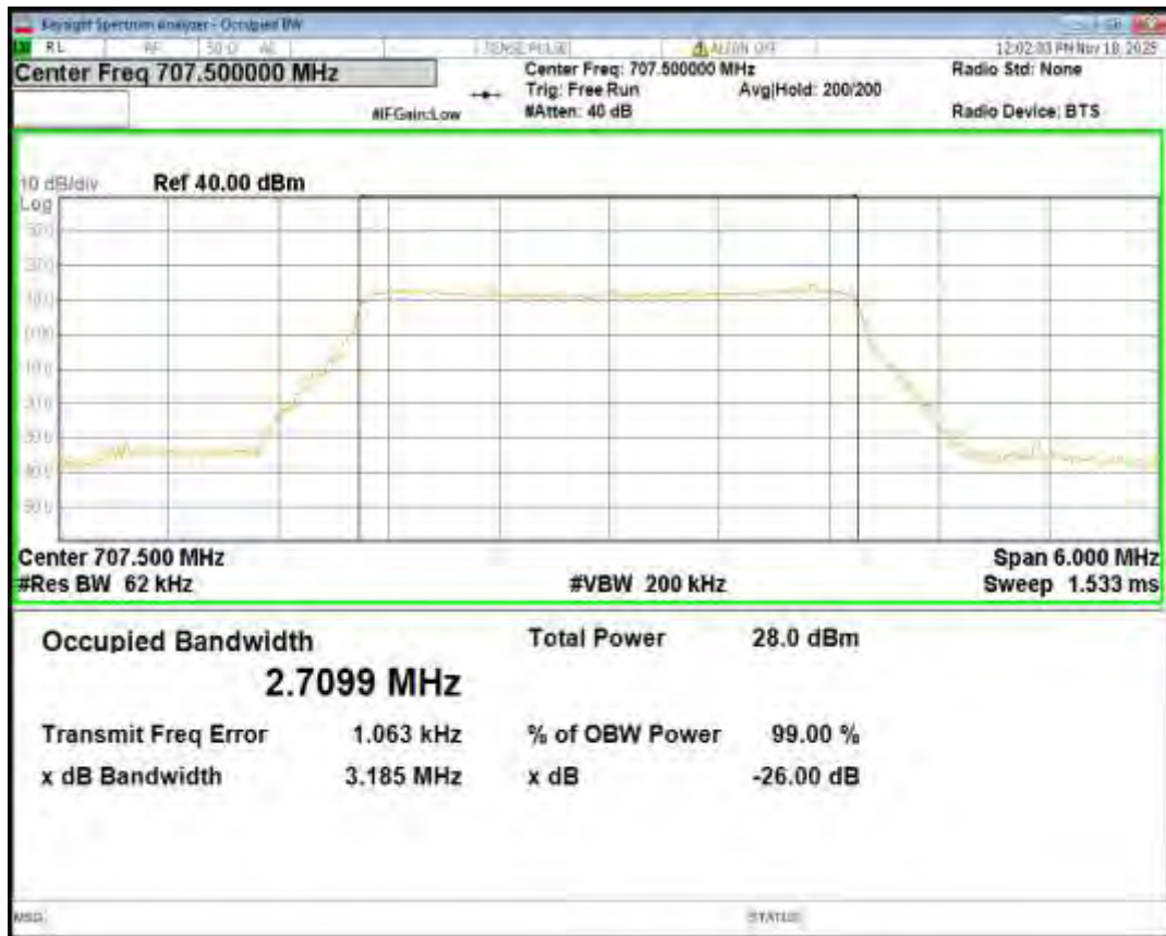
Band12 16QAM BW=3MHz Channel=23165 RB Size=15 Position=#0
