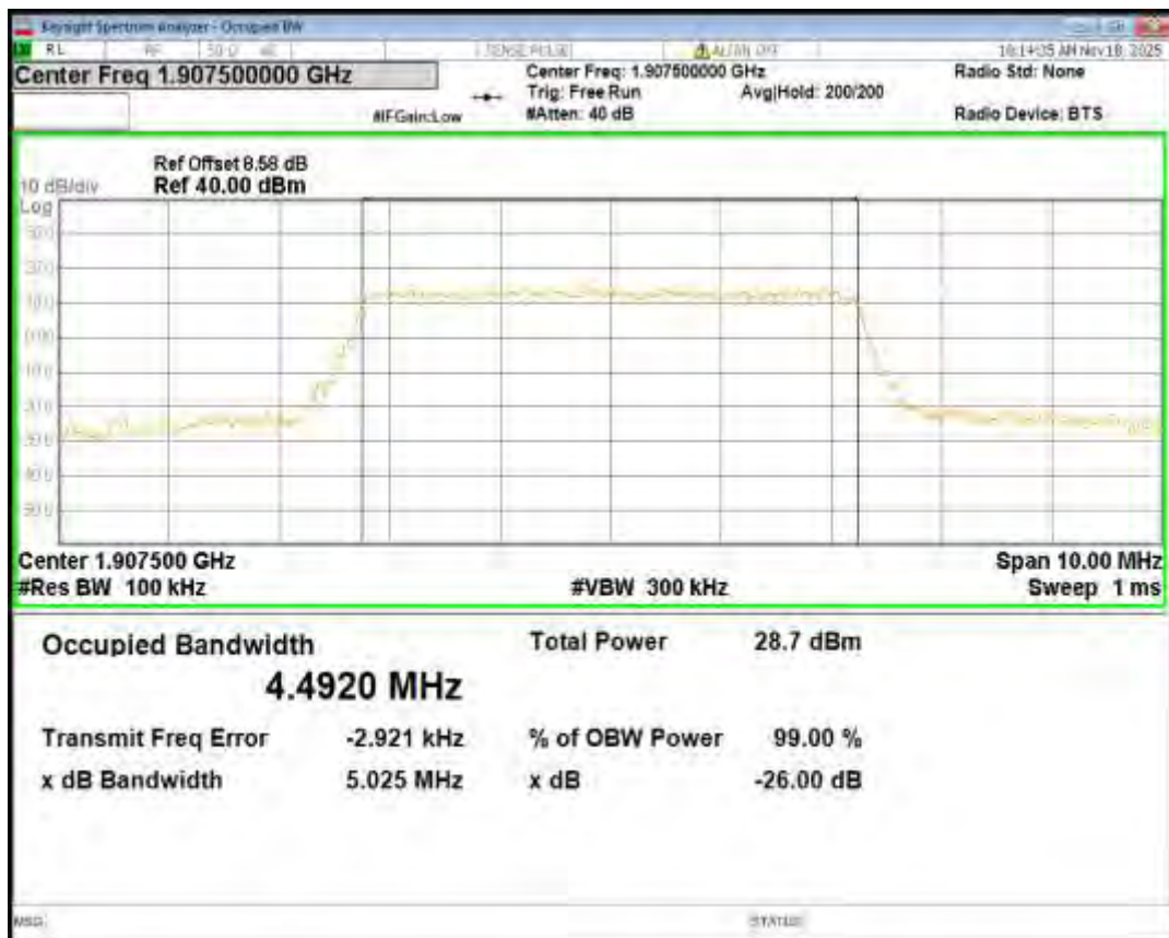
Band2 QPSK BW=1.4MHz Channel=18607 RB Size=6 Position=#0
