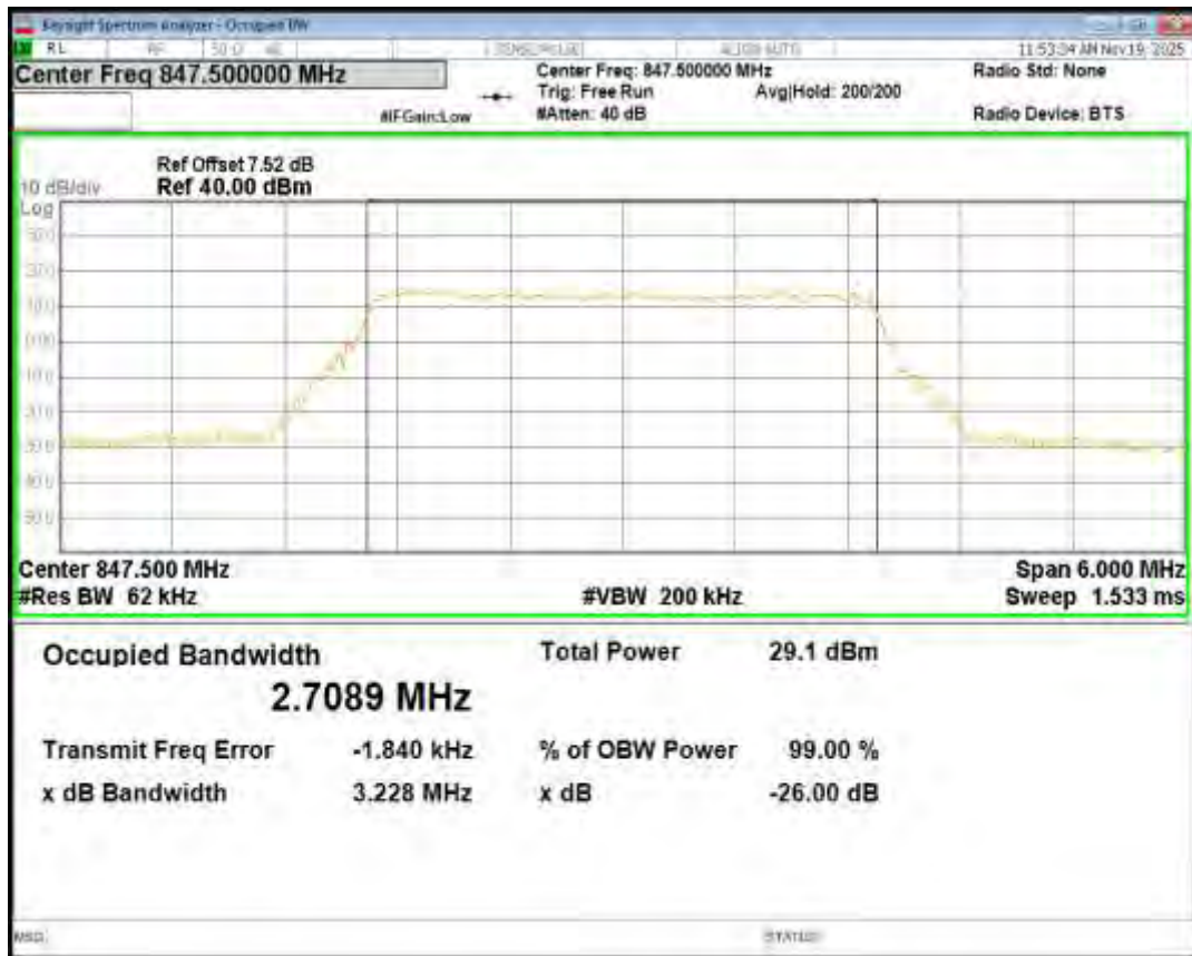
Band26(824-849) 16QAM BW=5MHz Channel=26915 RB Size=25 Position=#0
