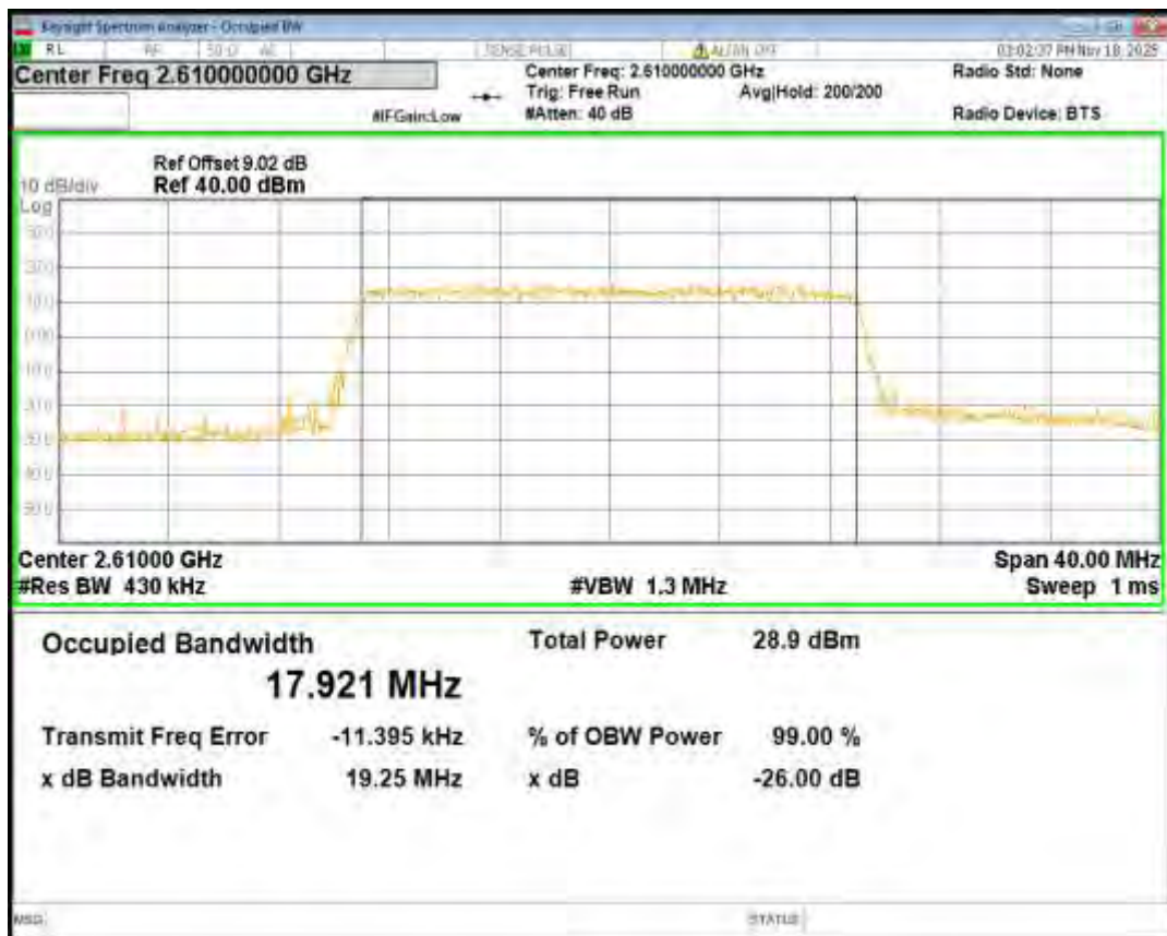
Band4 16QAM BW=1.4MHz Channel=19957 RB Size=6 Position=#0
