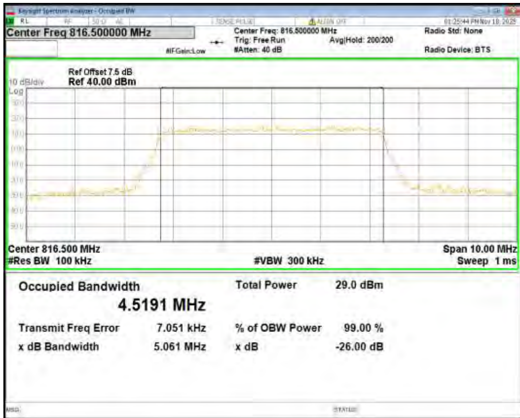
Band26(814-824) QPSK BW=5MHz Channel=26765 RB Size=25 Position=#0
