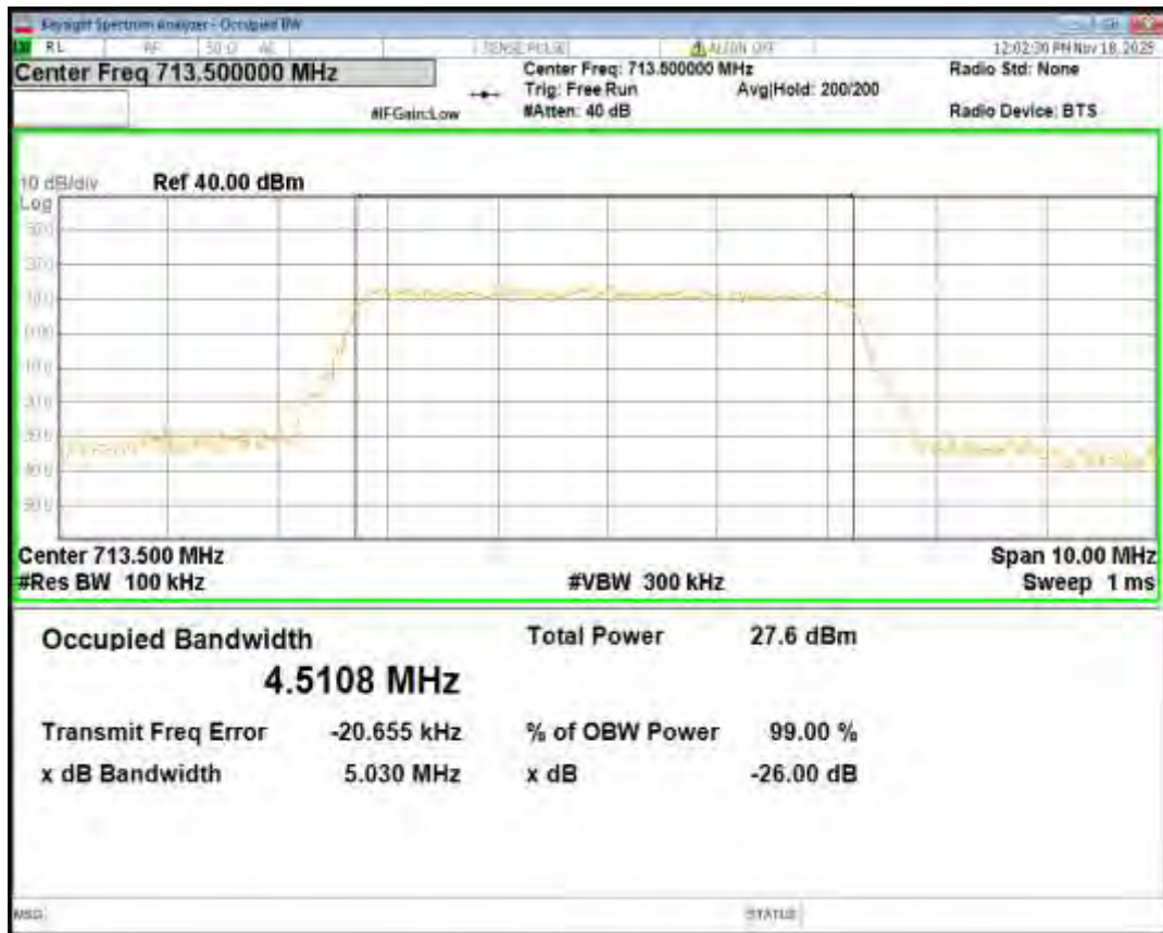
Band12 QPSK BW=1.4MHz Channel=23017 RB Size=6 Position=#0
