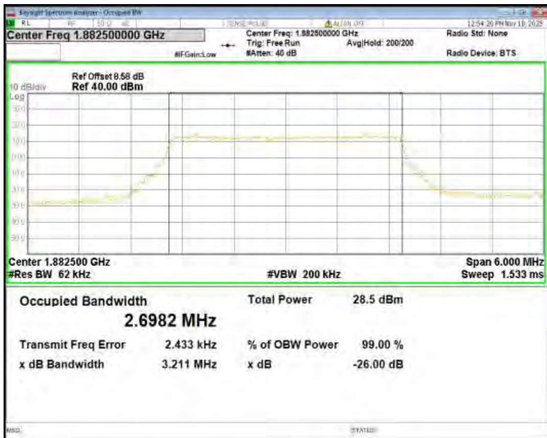
Band25 16QAM BW=3MHz Channel=26675 RB Size=15 Position=#0
