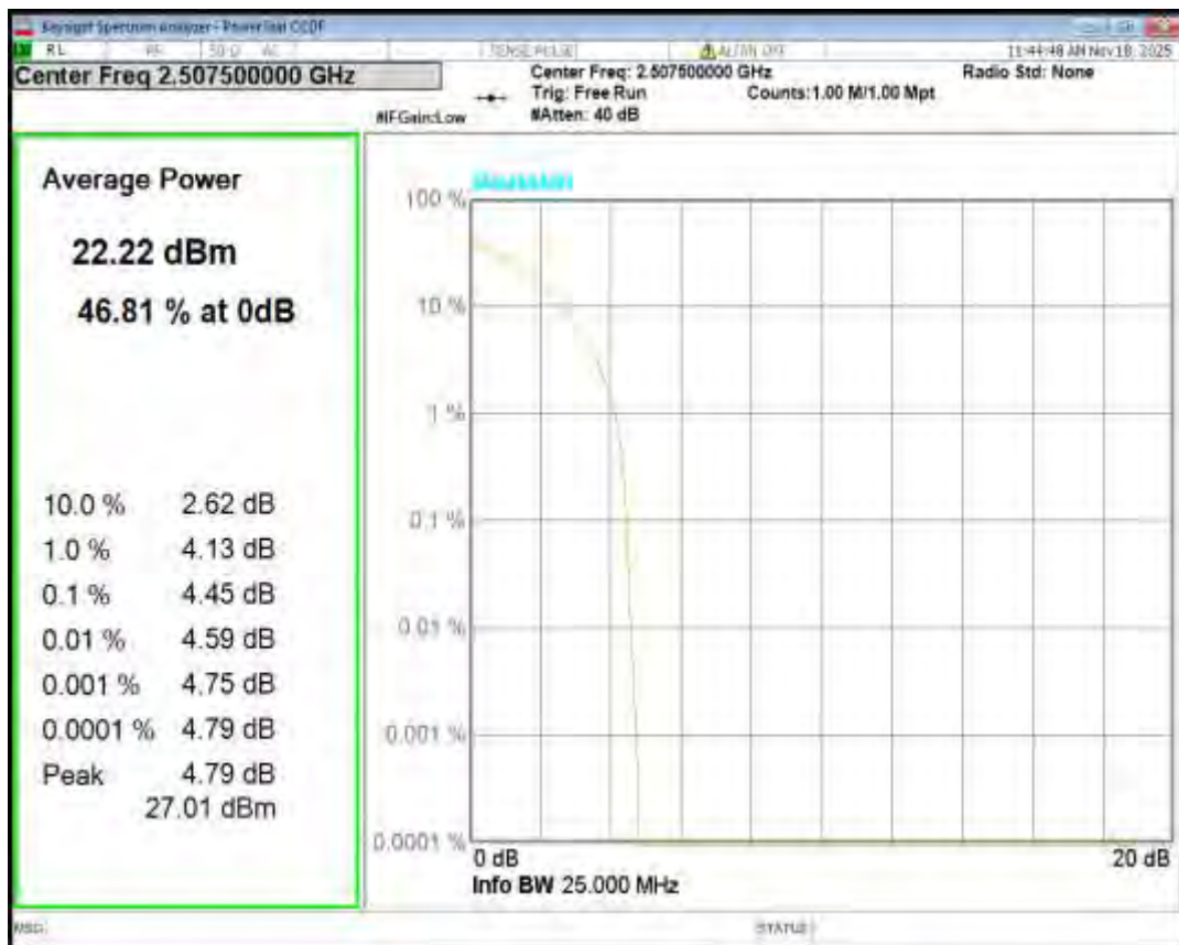
Band7 QPSK BW=15MHz Channel=21100 RB Size=1 Position=#0
