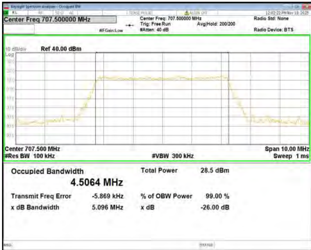
Band12 QPSK BW=5MHz Channel=23155 RB Size=25 Position=#0
