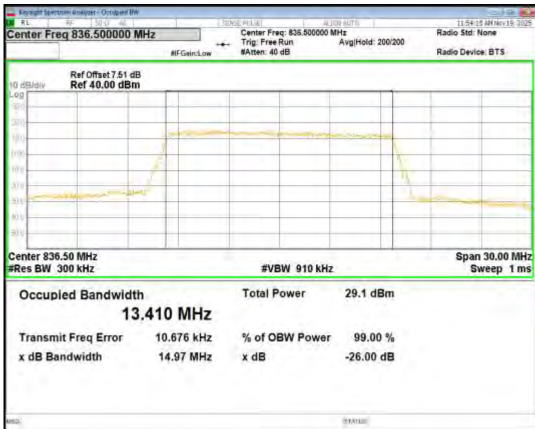
Band26(824-849) QPSK BW=15MHz Channel=26965 RB Size=75 Position=#0
