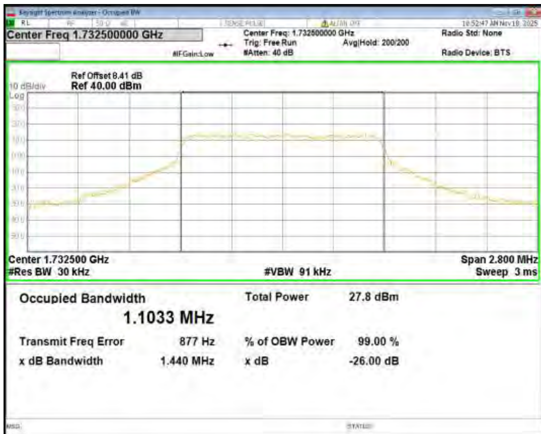
Band4 16QAM BW=1.4MHz Channel=20393 RB Size=6 Position=#0
