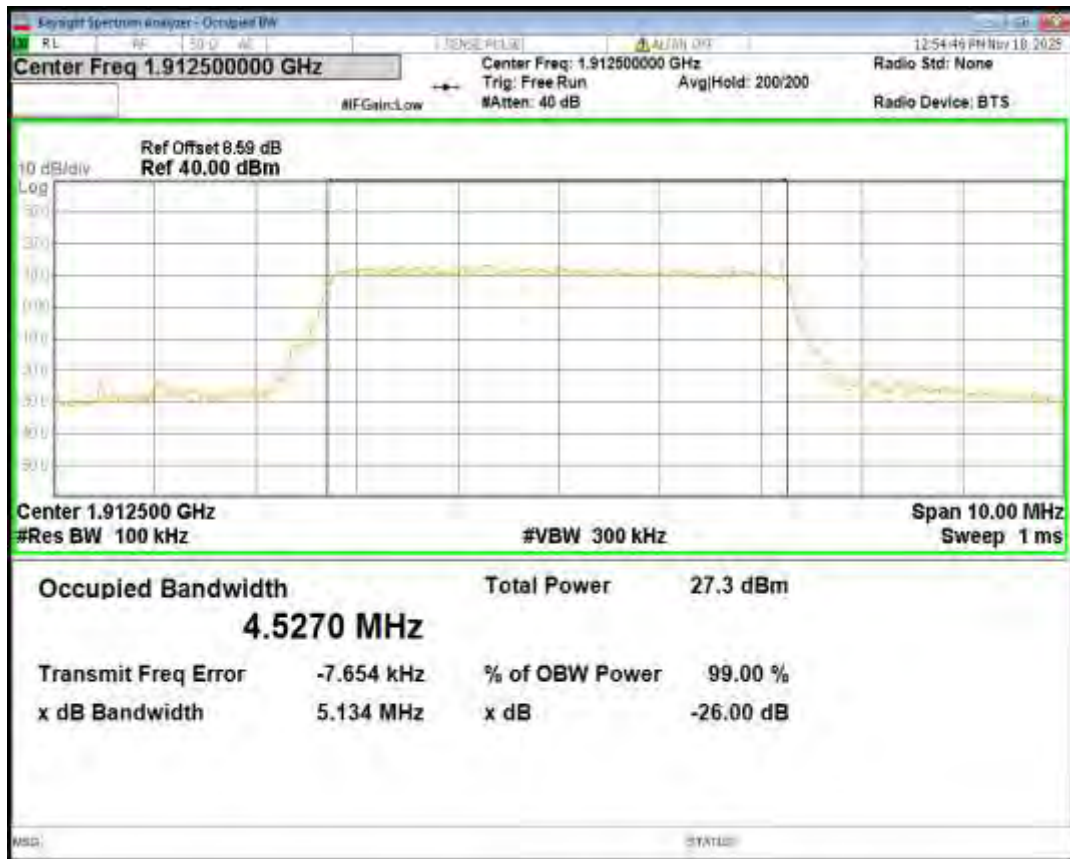
Band25 16QAM BW=5MHz Channel=26365 RB Size=25 Position=#0
