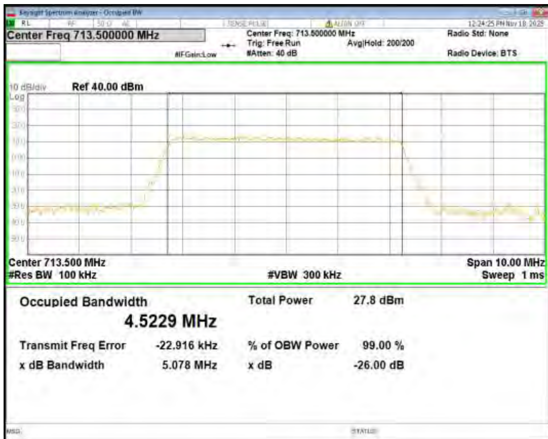
Band17 QPSK BW=5MHz Channel=23755 RB Size=25 Position=#0
