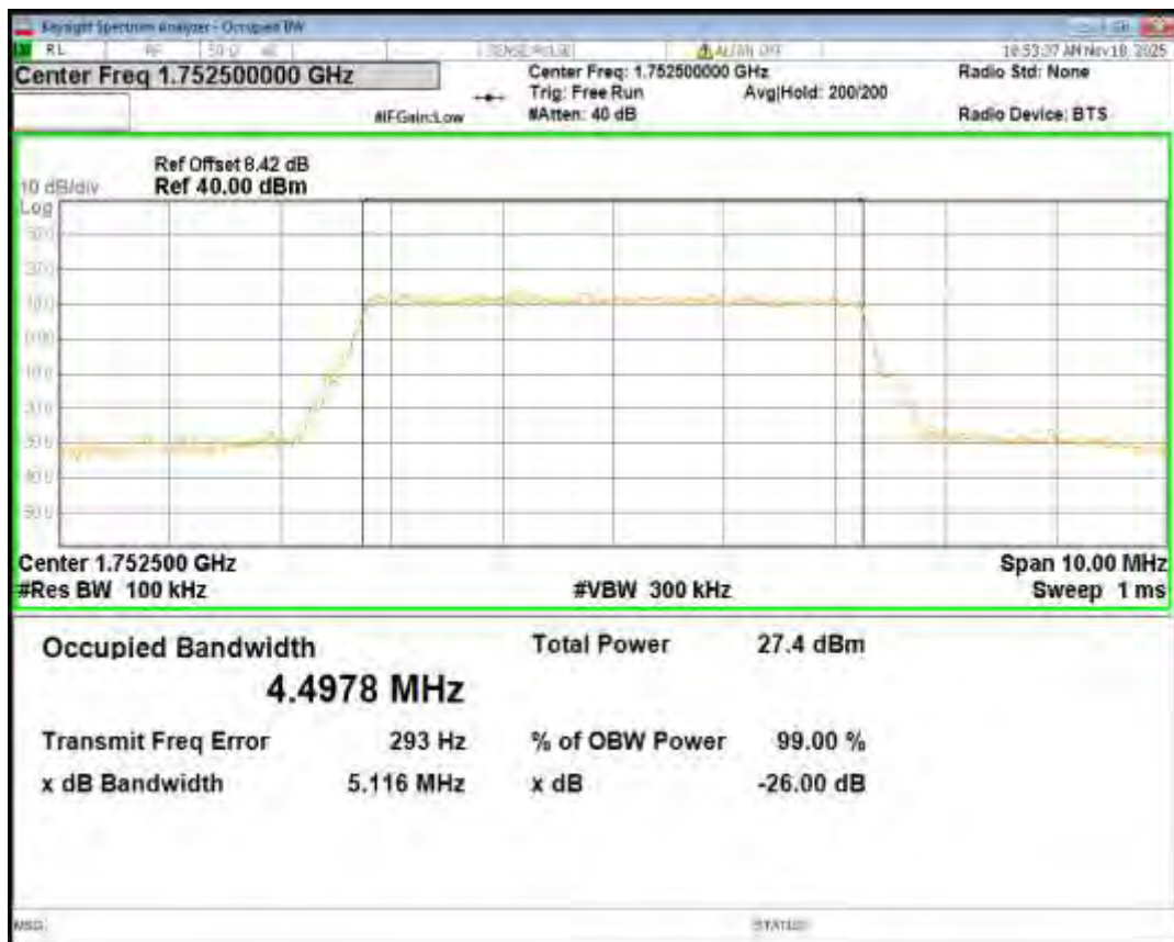
Band4 QPSK BW=1.4MHz Channel=19957 RB Size=6 Position=#0
