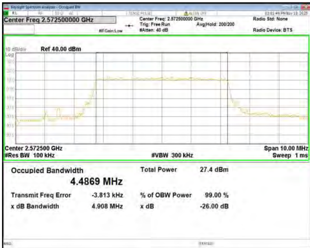
Band38 16QAM BW=5MHz Channel=38000 RB Size=25 Position=#0
