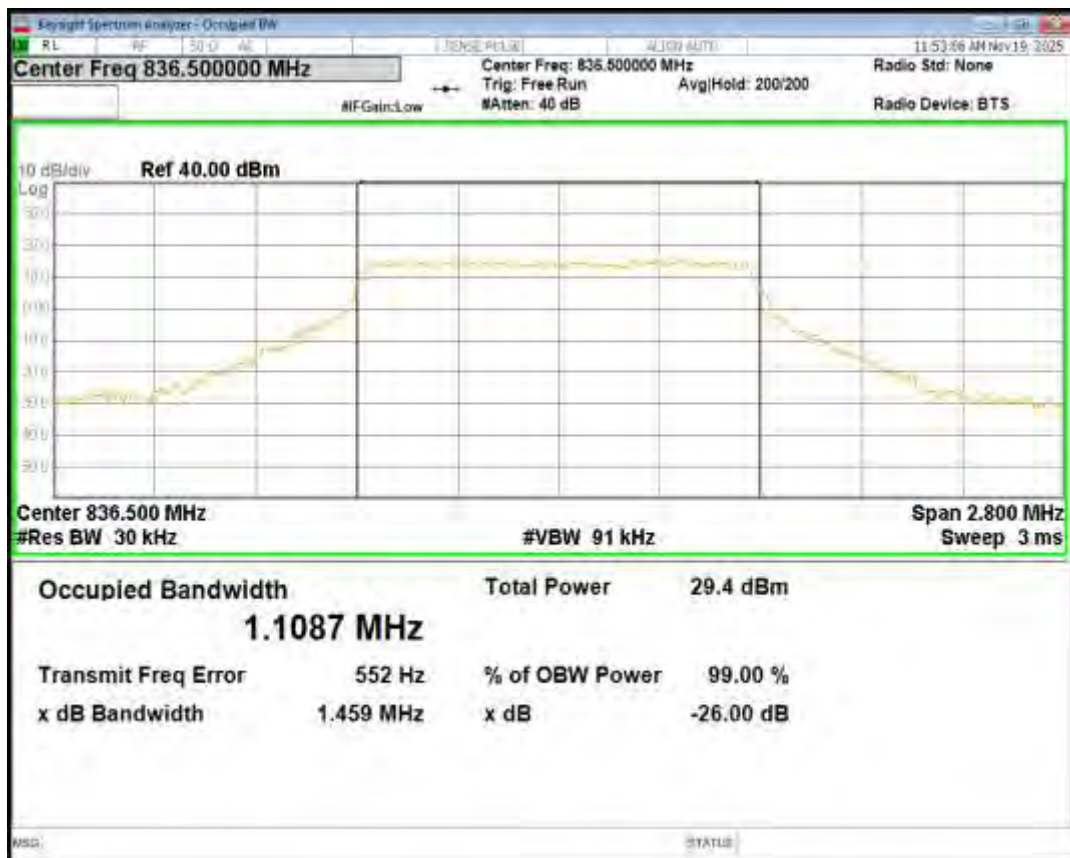
Band26(824-849) QPSK BW=1.4MHz Channel=27033 RB Size=6 Position=#0
