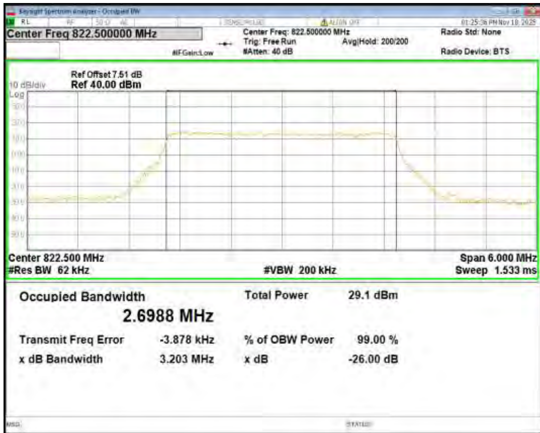
Band26(814-824) QPSK BW=5MHz Channel=26740 RB Size=25 Position=#0
