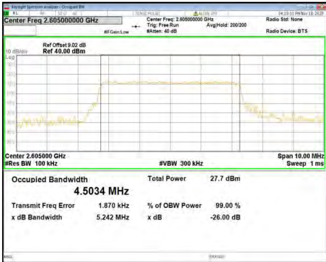
Band41(2555-2655) 16QAM BW=5MHz Channel=41215 RB Size=25 Position=#0
