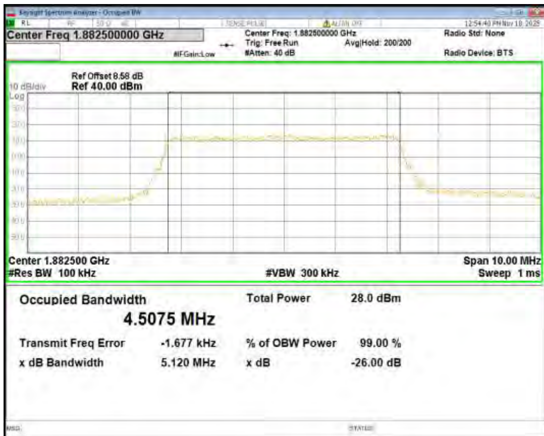
Band25 QPSK BW=1.4MHz Channel=26047 RB Size=6 Position=#0
