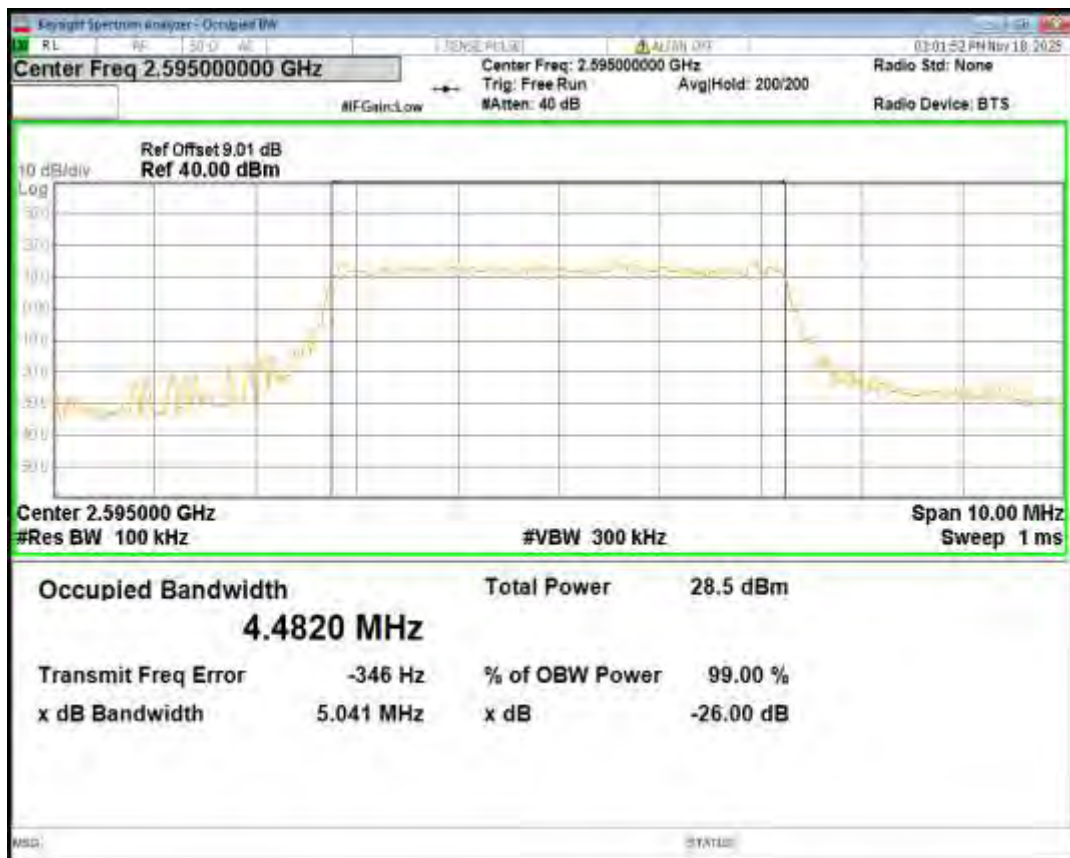
Band38 QPSK BW=5MHz Channel=38225 RB Size=25 Position=#0
