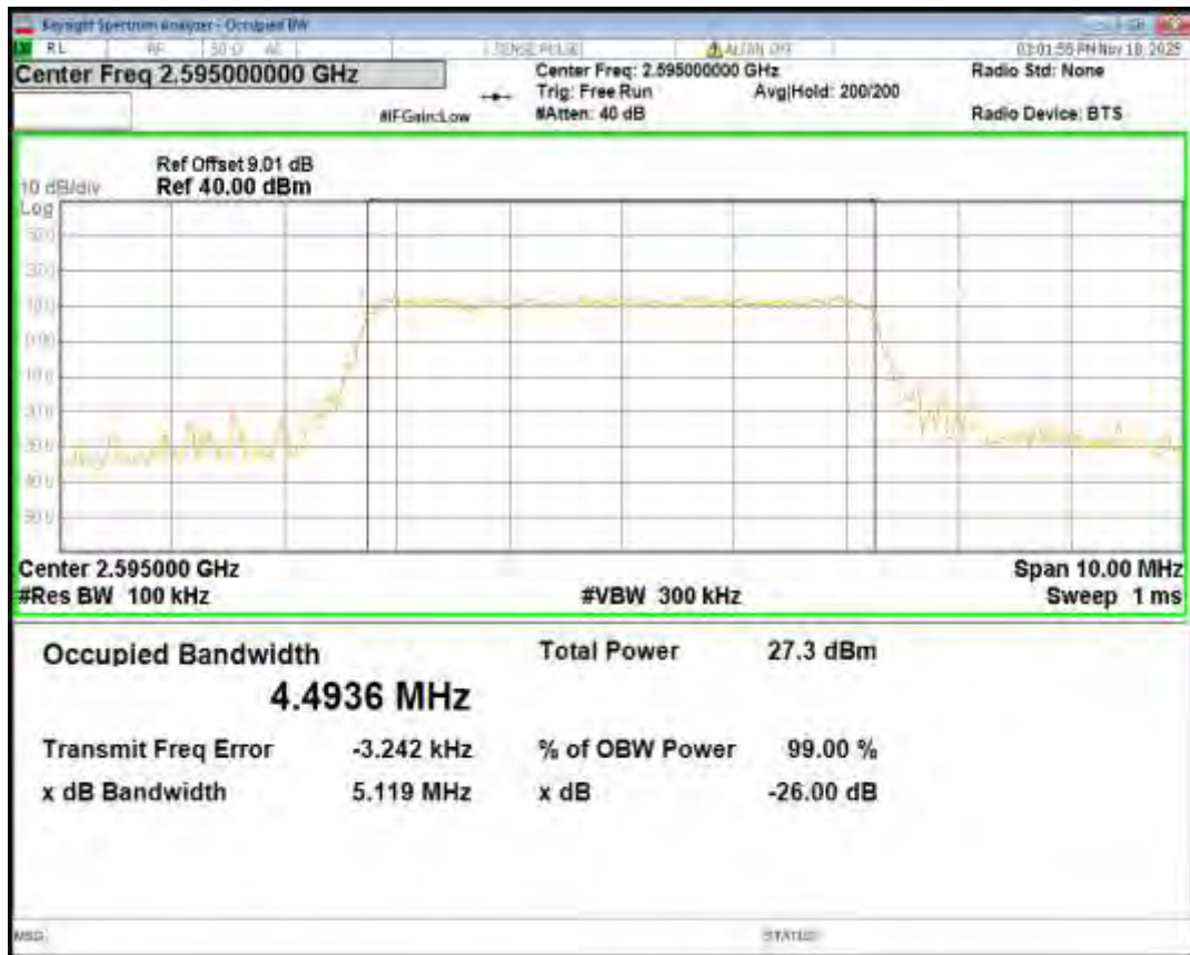
Band38 16QAM BW=5MHz Channel=38225 RB Size=25 Position=#0
