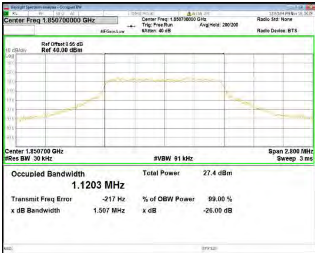
Band25 16QAM BW=1.4MHz Channel=26365 RB Size=6 Position=#0
