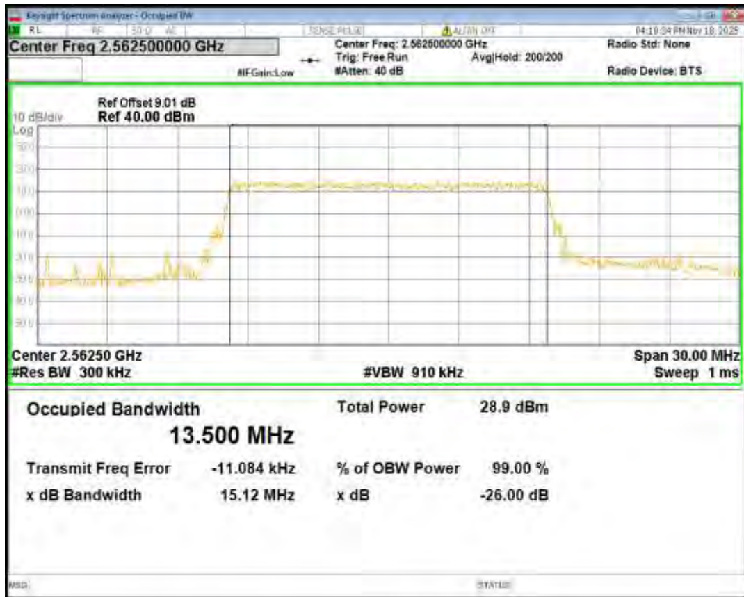
Band41(2555-2655) QPSK BW=15MHz Channel=40740 RB Size=75 Position=#0
