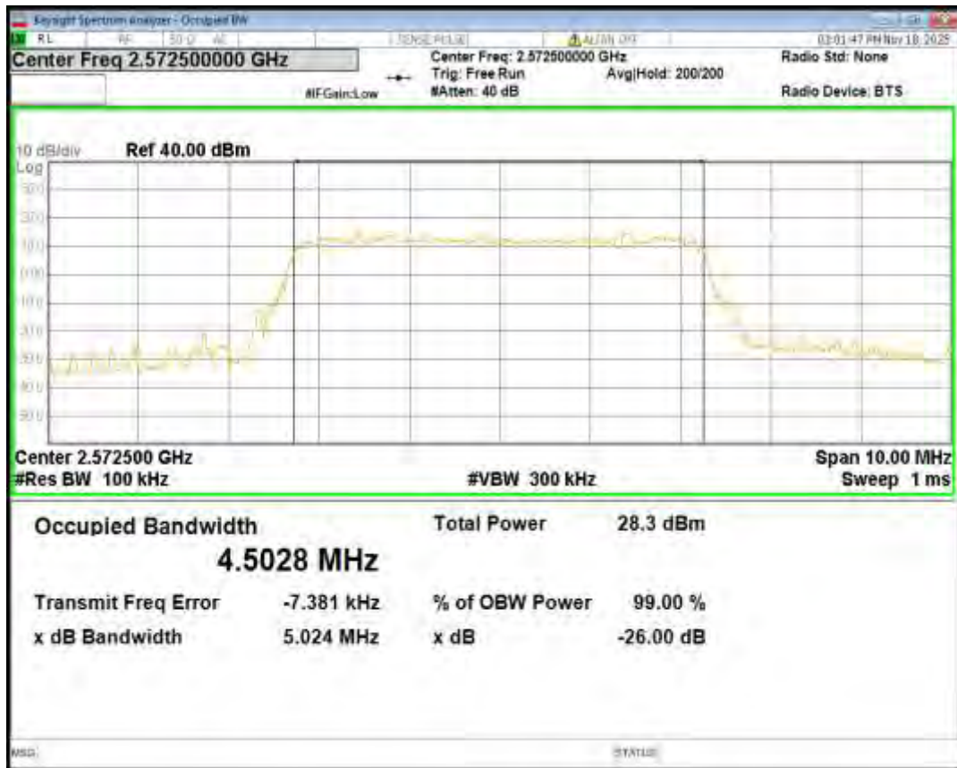
Band38 QPSK BW=5MHz Channel=38000 RB Size=25 Position=#0
