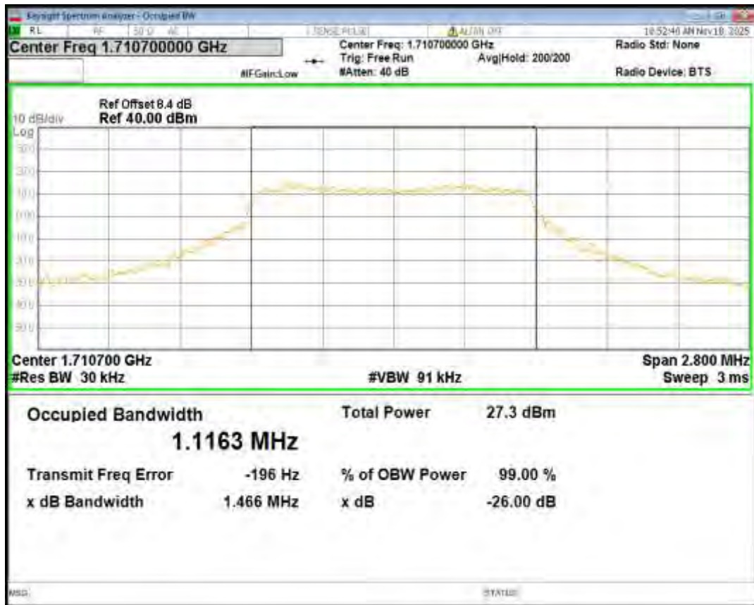
Band4 16QAM BW=1.4MHz Channel=20175 RB Size=6 Position=#0
