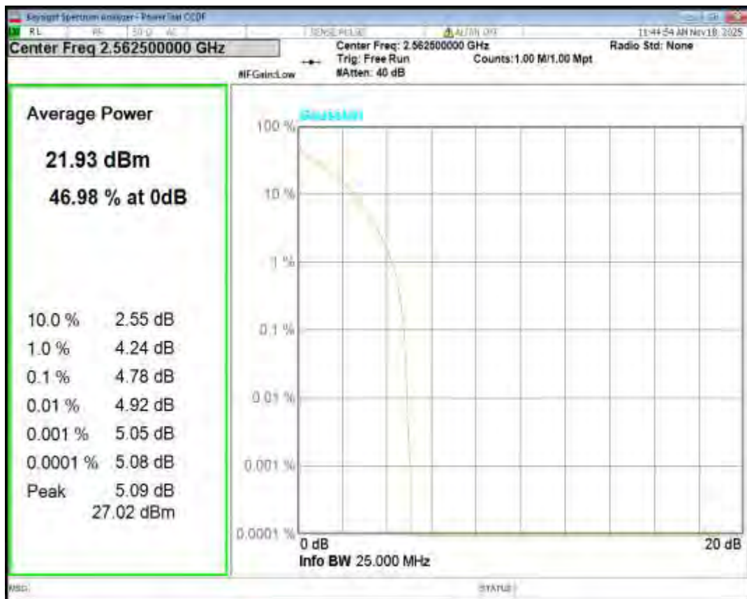
Band7 QPSK BW=20MHz Channel=20850 RB Size=1 Position=#0
