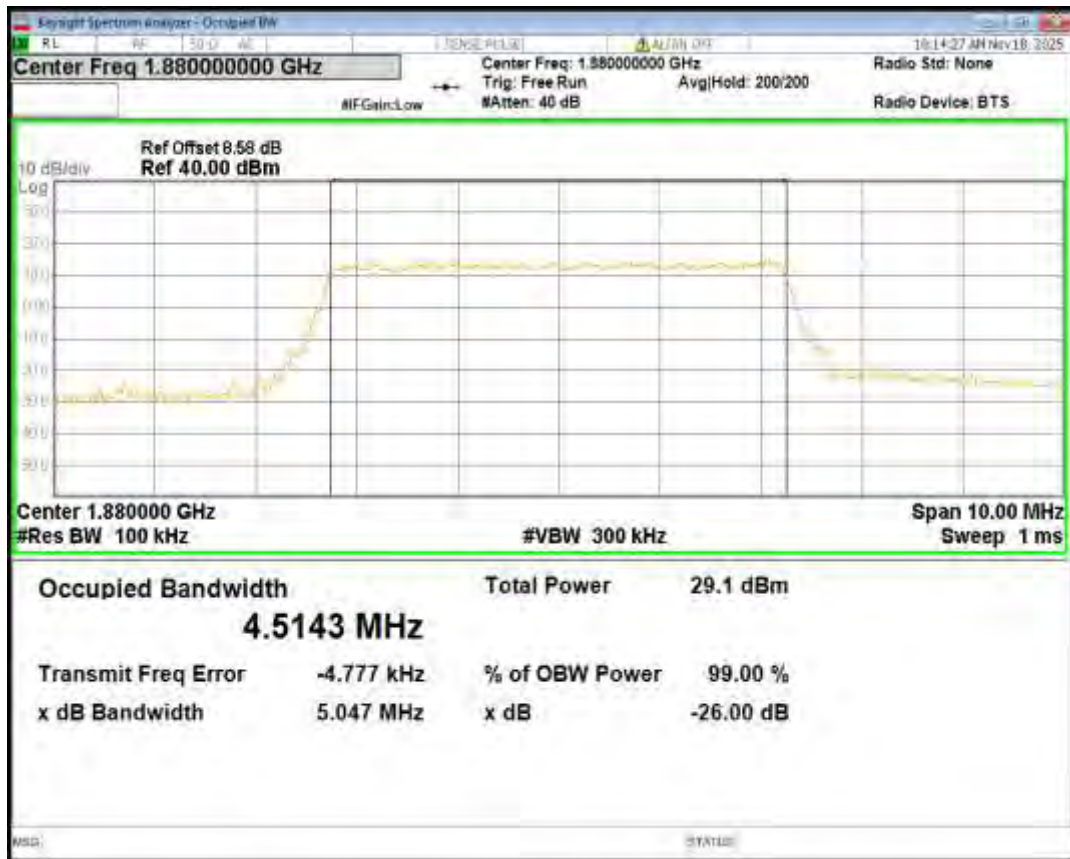
Band2 QPSK BW=3MHz Channel=19185 RB Size=15 Position=#0
