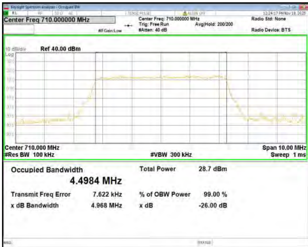
Band17 QPSK BW=5MHz Channel=23825 RB Size=25 Position=#0
