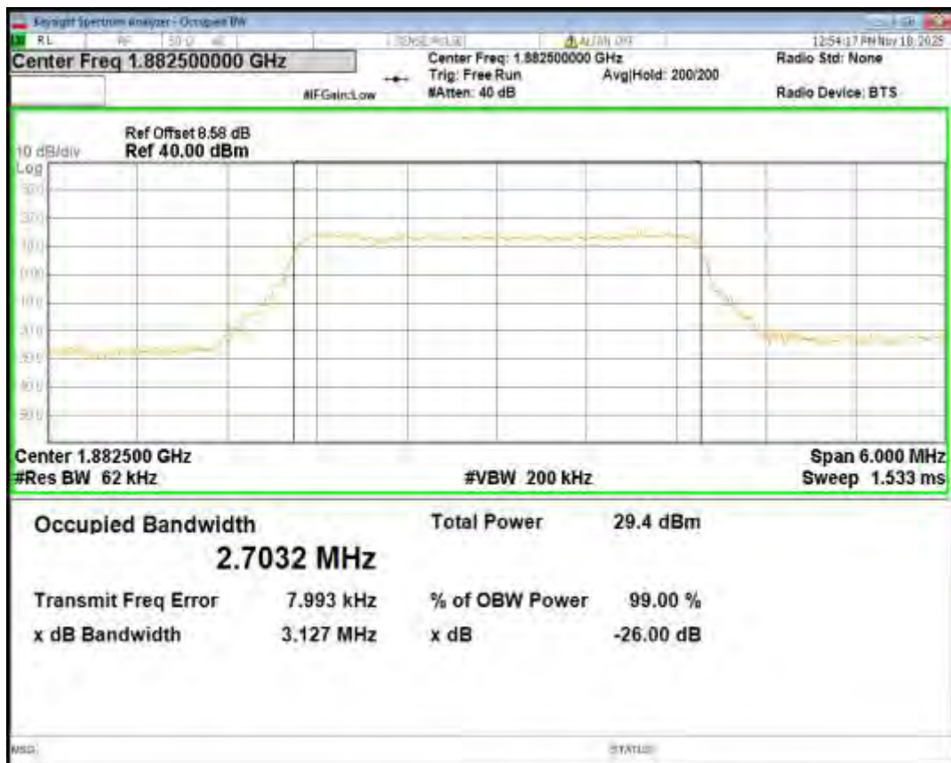
Band25 QPSK BW=3MHz Channel=26675 RB Size=15 Position=#0
