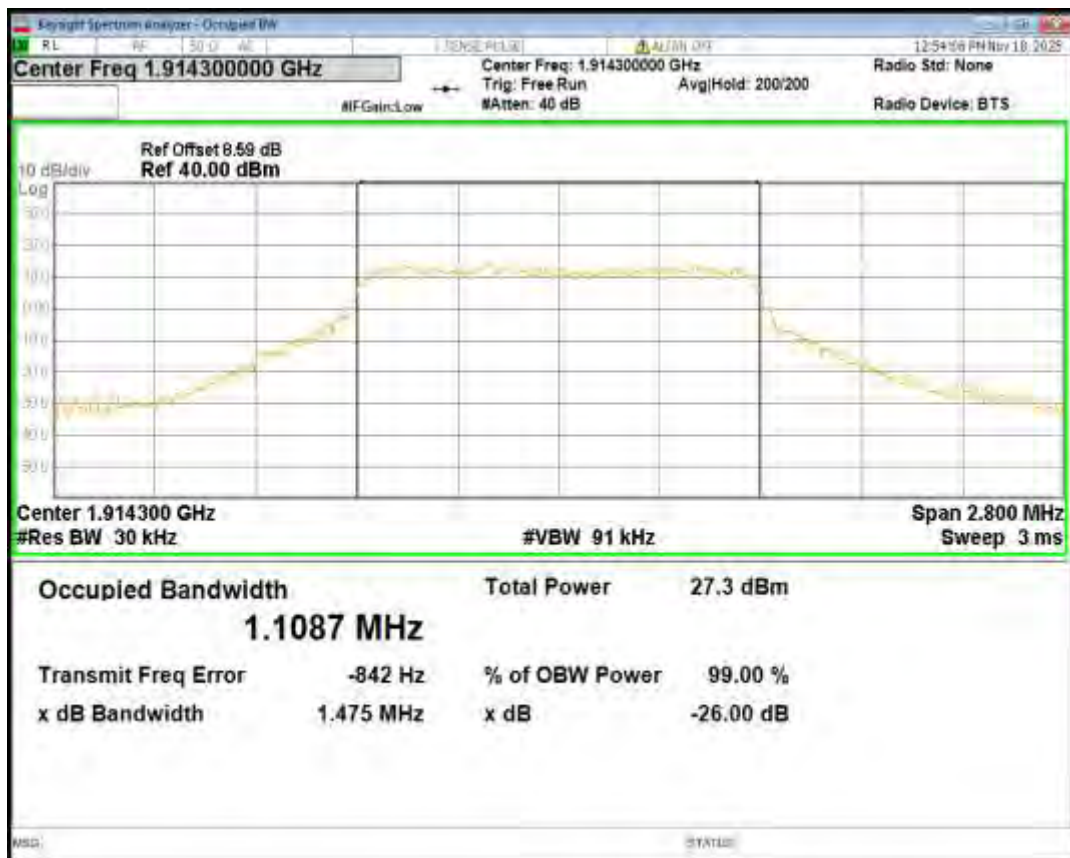
Band25 16QAM BW=3MHz Channel=26055 RB Size=15 Position=#0
