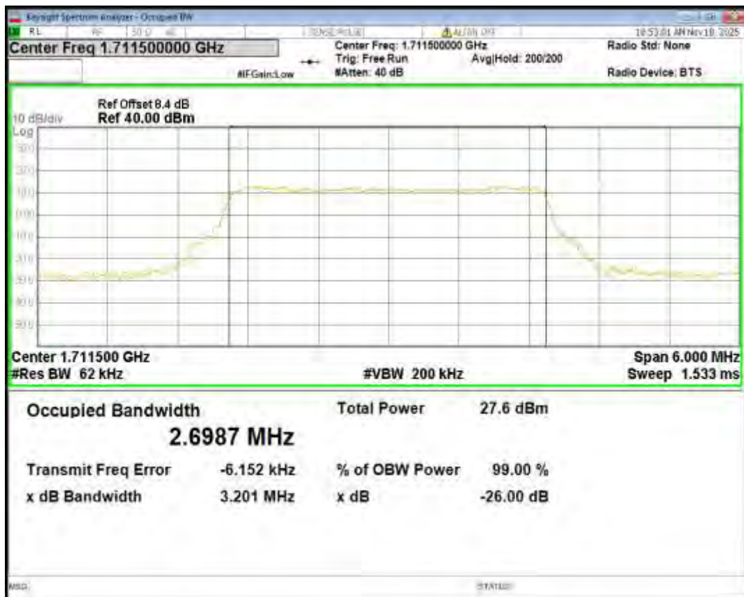
Band4 16QAM BW=3MHz Channel=20175 RB Size=15 Position=#0
