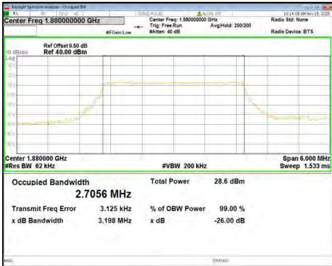
Band2 16QAM BW=3MHz Channel=19185 RB Size=15 Position=#0
