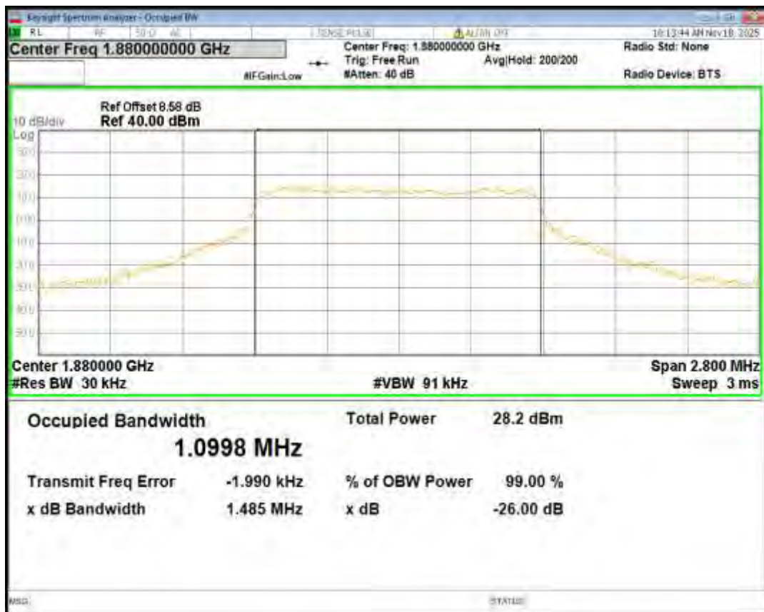
Band2 16QAM BW=1.4MHz Channel=19193 RB Size=6 Position=#0
