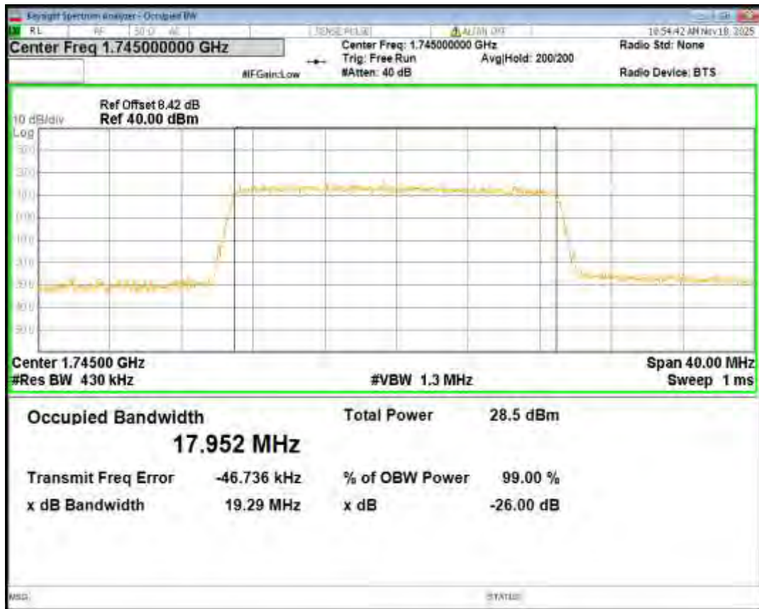
Band40(2305-2315) 16QAM BW=5MHz Channel=38725 RB Size=25 Position=#0
