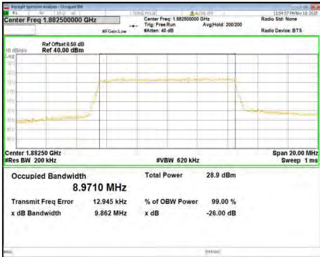
Band25 QPSK BW=10MHz Channel=26640 RB Size=50 Position=#0
