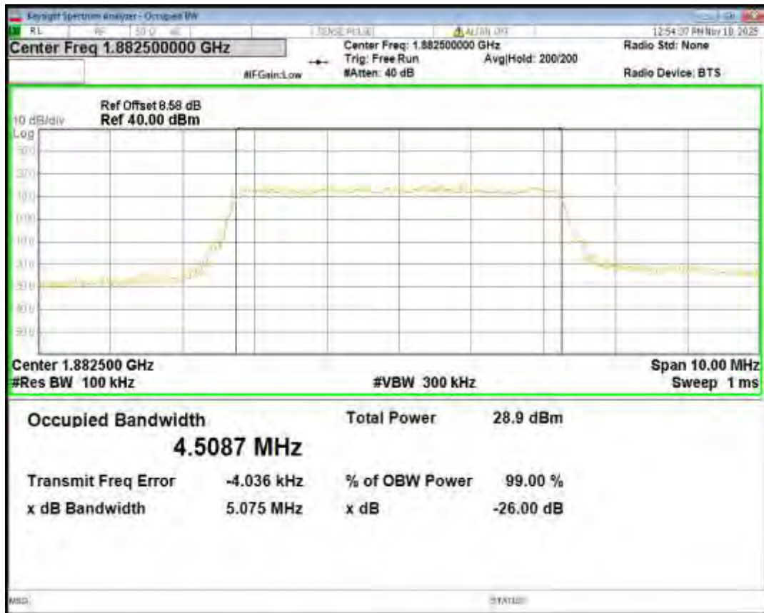
Band25 QPSK BW=3MHz Channel=26365 RB Size=15 Position=#0
