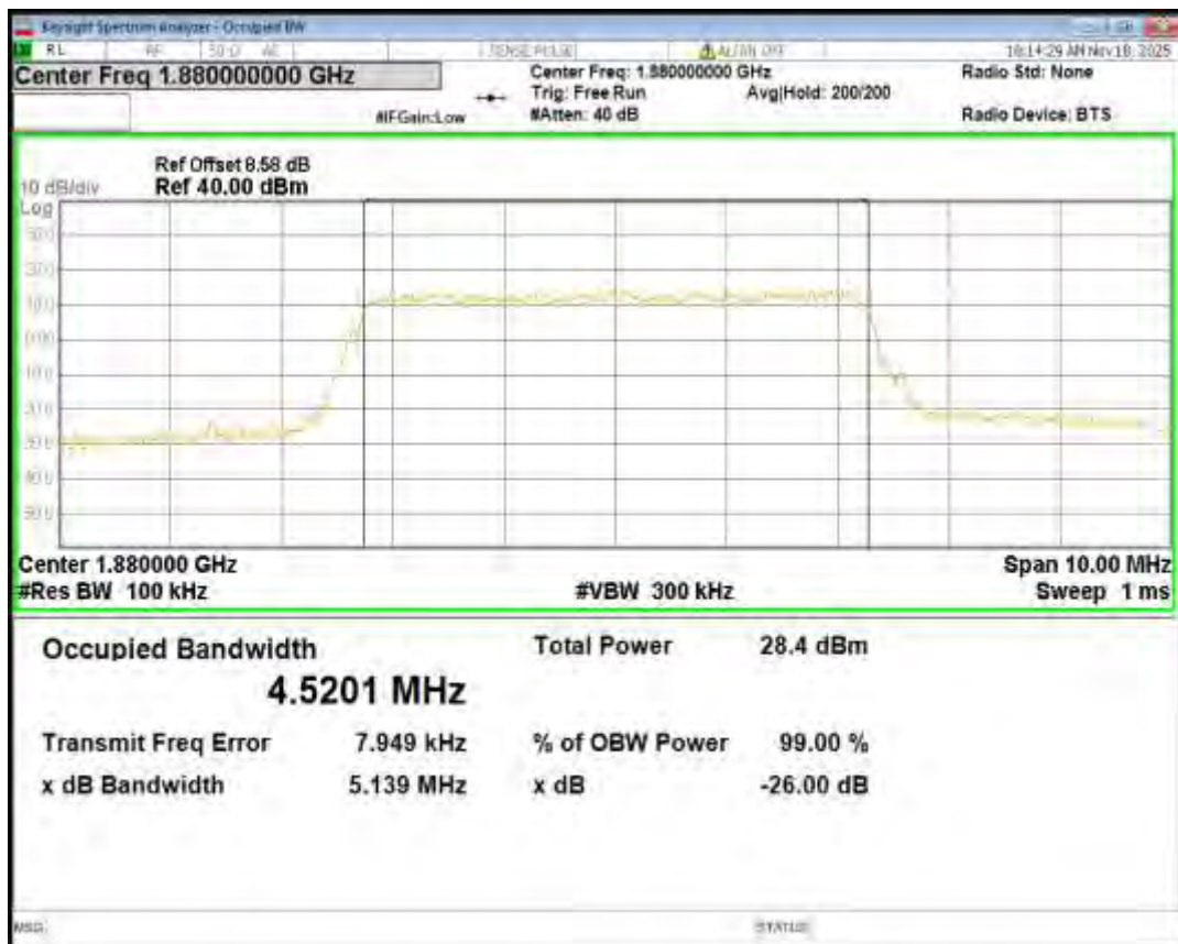
Band2 QPSK BW=1.4MHz Channel=18900 RB Size=6 Position=#0
