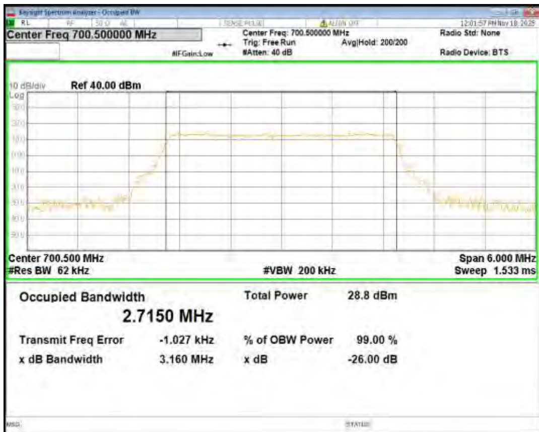
Band12 16QAM BW=3MHz Channel=23095 RB Size=15 Position=#0
