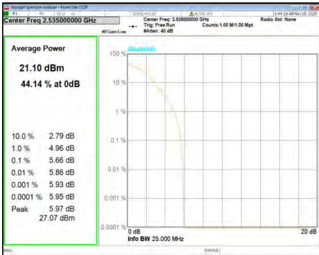
Band7 16QAM BW=5MHz Channel=21425 RB Size=1 Position=#0
