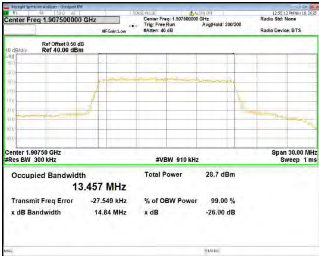
Band25 QPSK BW=20MHz Channel=26140 RB Size=100 Position=#0
