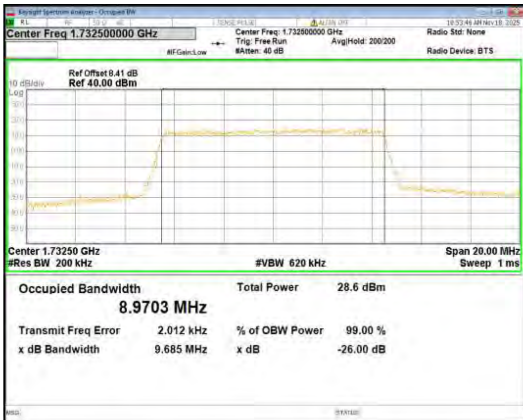
Band4 QPSK BW=10MHz Channel=20350 RB Size=50 Position=#0
