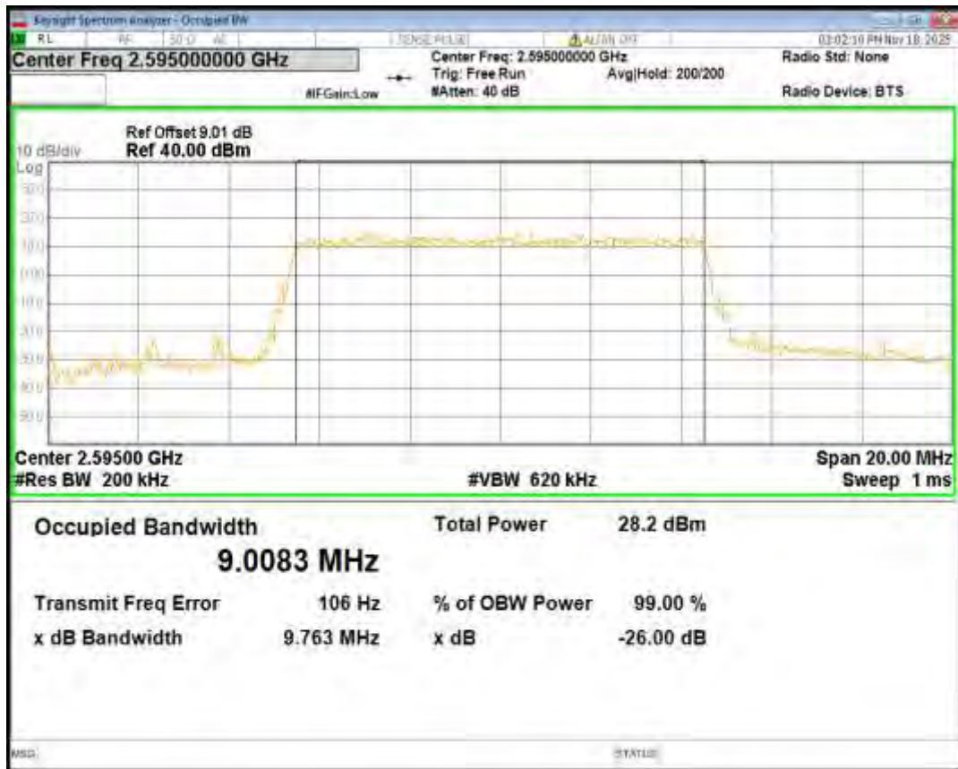
Band38 QPSK BW=10MHz Channel=38200 RB Size=50 Position=#0
