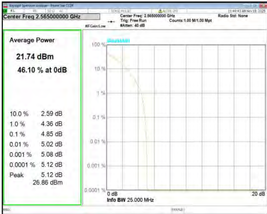
Band7 QPSK BW=15MHz Channel=20825 RB Size=1 Position=#0
