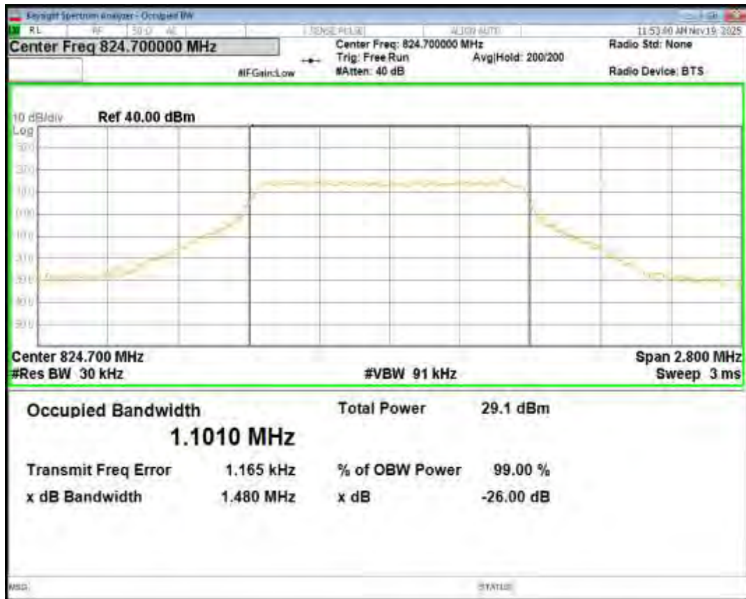
Band26(824-849) QPSK BW=1.4MHz Channel=26915 RB Size=6 Position=#0
