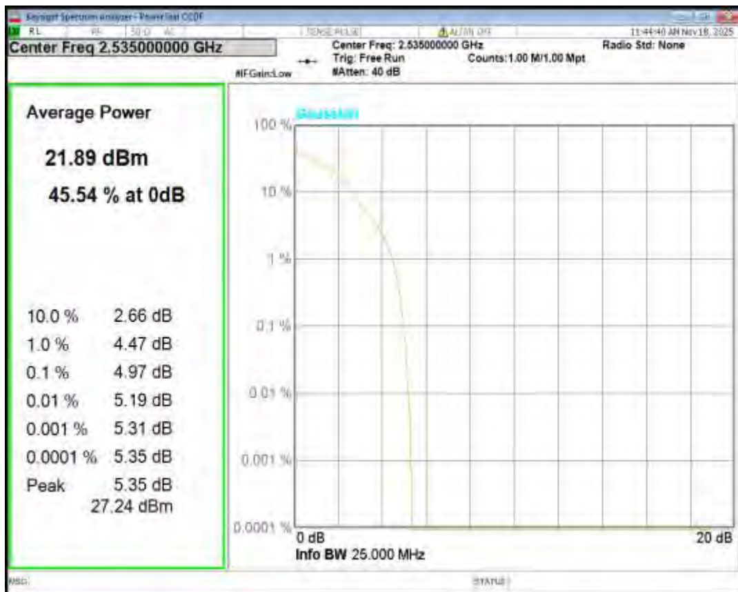
Band7 QPSK BW=10MHz Channel=21400 RB Size=1 Position=#0
