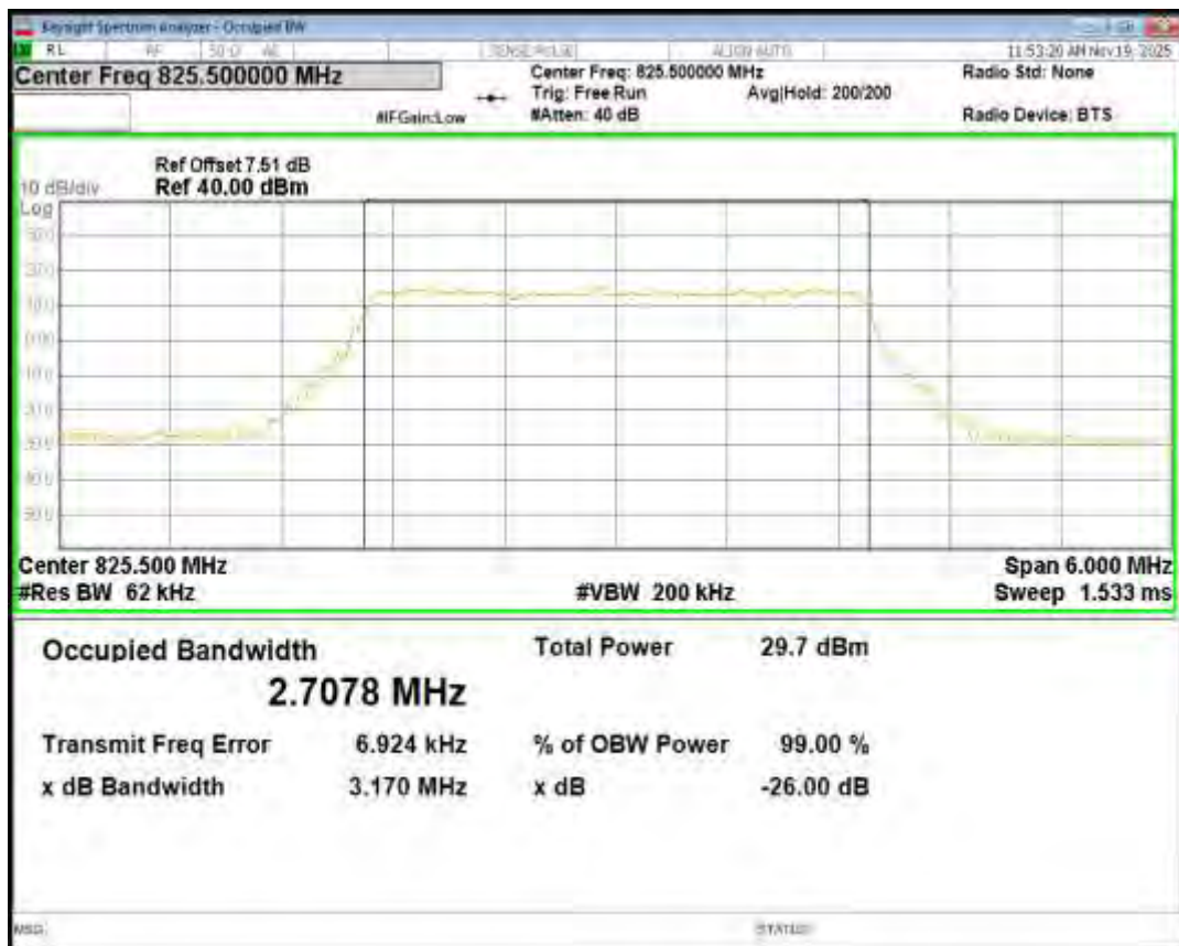
Band26(824-849) QPSK BW=3MHz Channel=26915 RB Size=15 Position=#0
