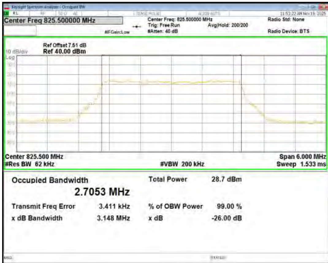
Band26(824-849) 16QAM BW=3MHz Channel=26915 RB Size=15 Position=#0
