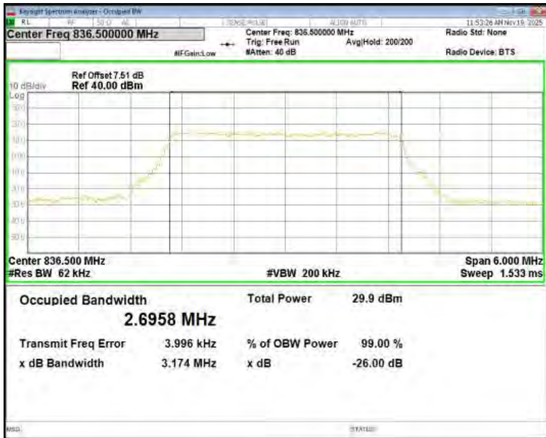
Band26(824-849) QPSK BW=3MHz Channel=27025 RB Size=15 Position=#0
