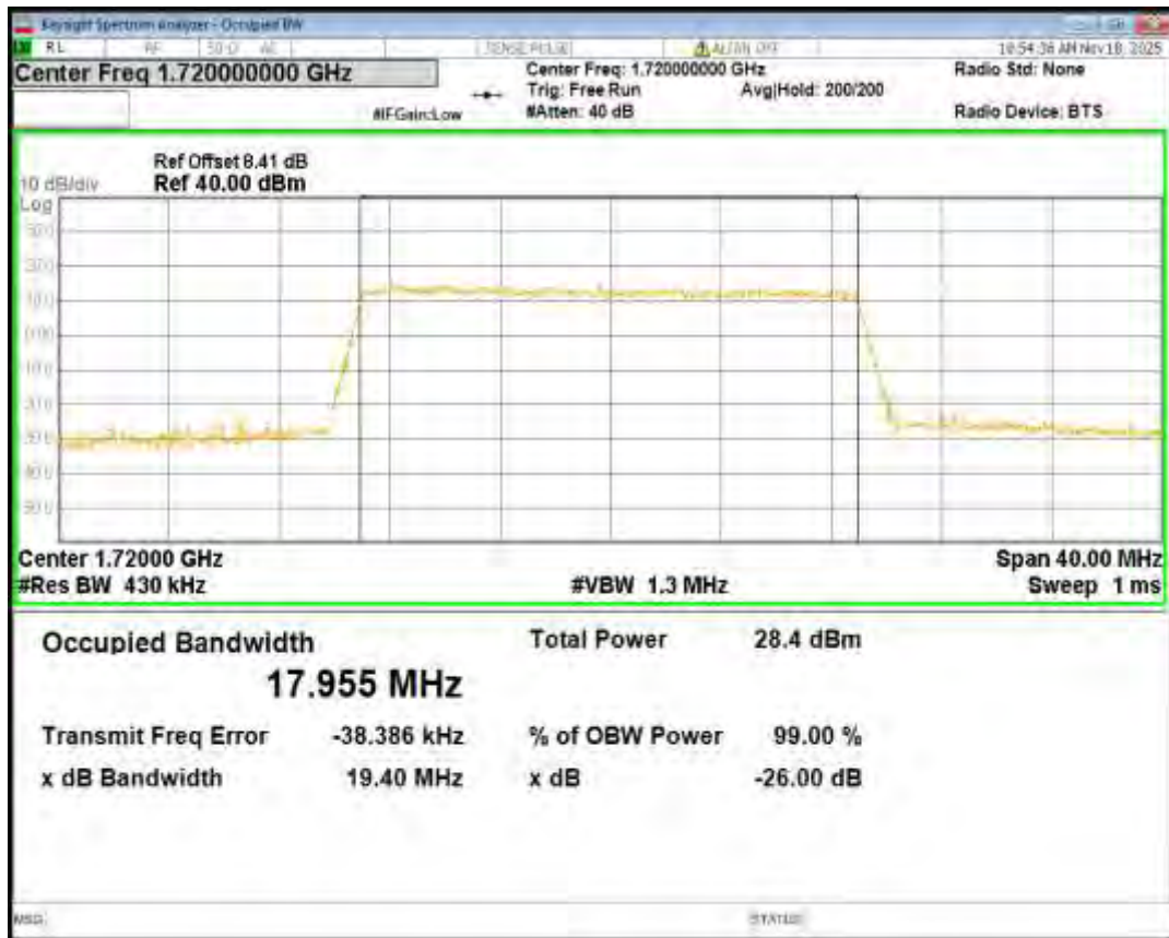
Band4 QPSK BW=20MHz Channel=20175 RB Size=100 Position=#0
