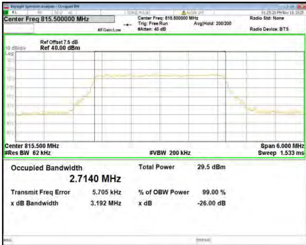
Band26(814-824) QPSK BW=3MHz Channel=26740 RB Size=15 Position=#0
