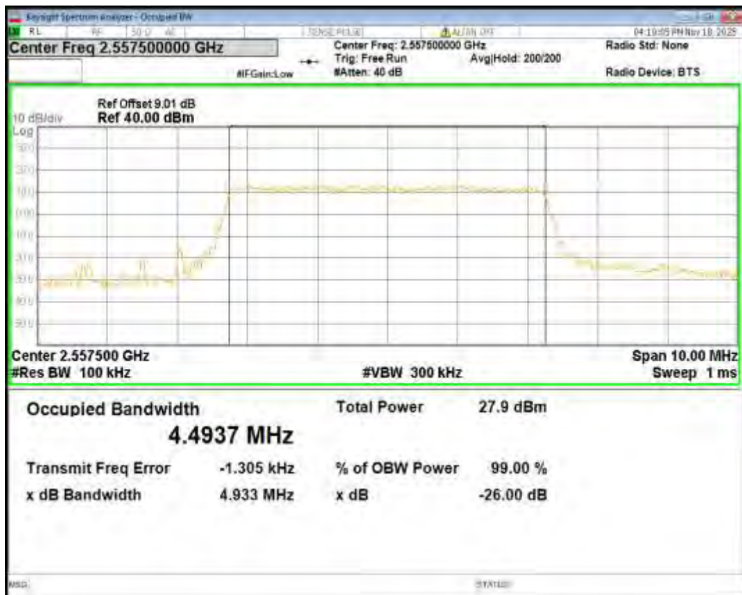
Band41(2555-2655) 16QAM BW=5MHz Channel=40740 RB Size=25 Position=#0
