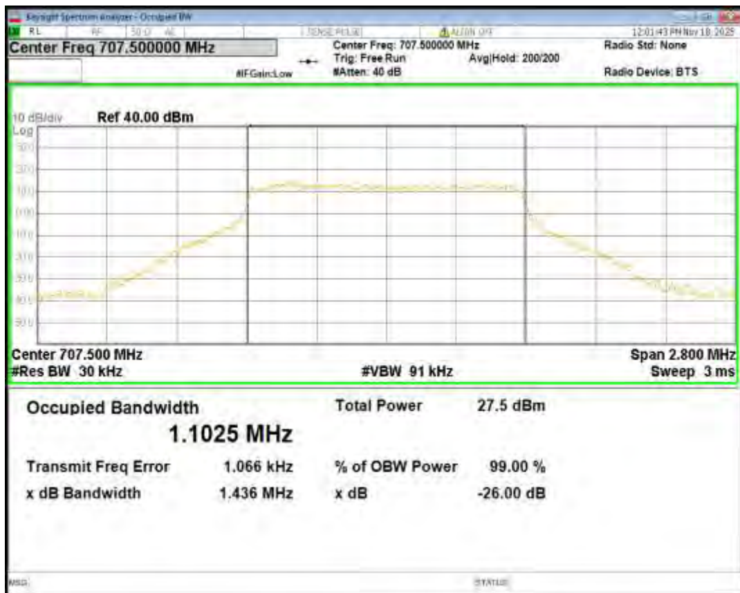
Band12 16QAM BW=1.4MHz Channel=23173 RB Size=6 Position=#0
